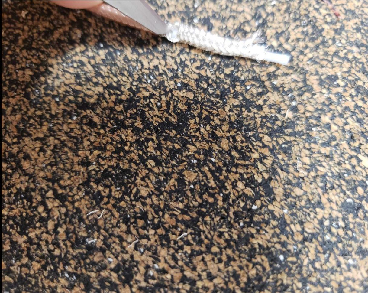
Carefully use an object such as the pen inkwell, antenna reflector or a hobby knife to slowly probe the center conductor and create a gap for you to pull the insulated center conductor through the braid as close to where the jacket ends.
