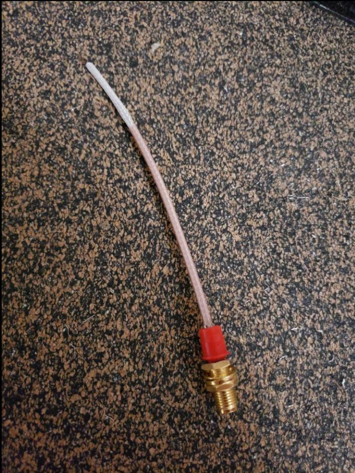
Properly completed matching section with the outer jacket of the RG-179 coaxial cable stripped at 57.6mm
