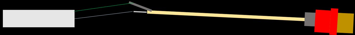
If your matching section is NOT preassembled with the shield and center conductor already separated, it should have a blue mark on the coax.
