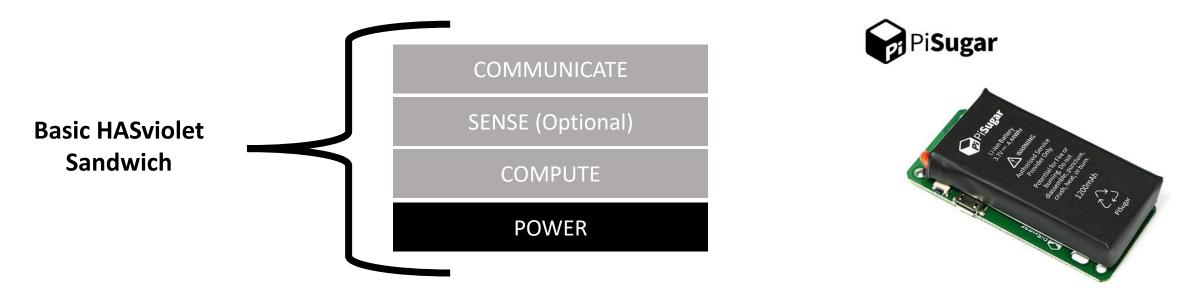
While a power bank can be used to power your device, be wary of stress on connectors to avoid damage of your Raspberry Pi Zero while using outside the home. More detail in <u>Addendum – Hardware – Power section</u>
