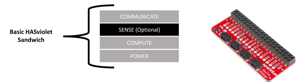
• A great feature of this approach is the 40-pin pass through style connector for use with a Raspberry Pi Zero
