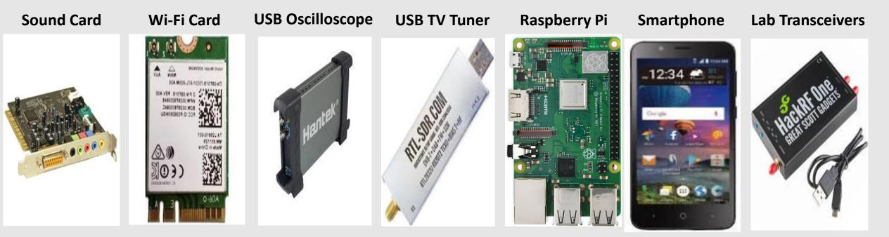
0 Hz to 500 kHz+ 2.3 GHz to 6 GHz 0 Hz to 60 MHz+ 0 Hz to 1.9 GHz+ 0 Hz to 1.5 GHz+ 0 Hz to ?? GHz 0 Hz to 6.0 GHz+
