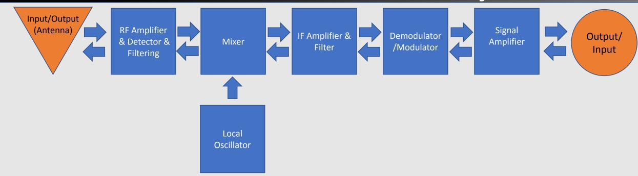
**Traditional Radio Systems** are limited to hardware features and functionality (e.g. <u>mixers</u>, <u>filters</u>, <u>amplifiers</u>, <u>modulators</u>/<u>demodulators</u>, <u>detectors</u>, etc.) There are applications where this still have benefits when very narrow needs are required.
