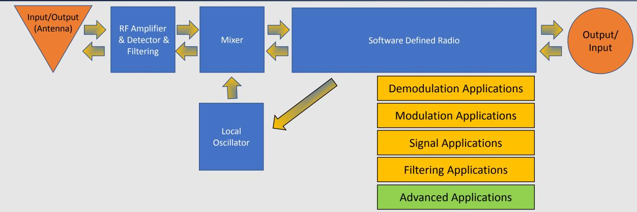
**Software-defined radio** (**SDR**) is a <u>radio communication</u> system where components that have been traditionally implemented in hardware (e.g. <u>mixers</u>, <u>filters</u>, <u>amplifiers</u>, <u>modulators/demodulators</u>, <u>detectors</u>, etc.) are instead implemented by means of software on a personal computer or <u>embedded system</u>.
