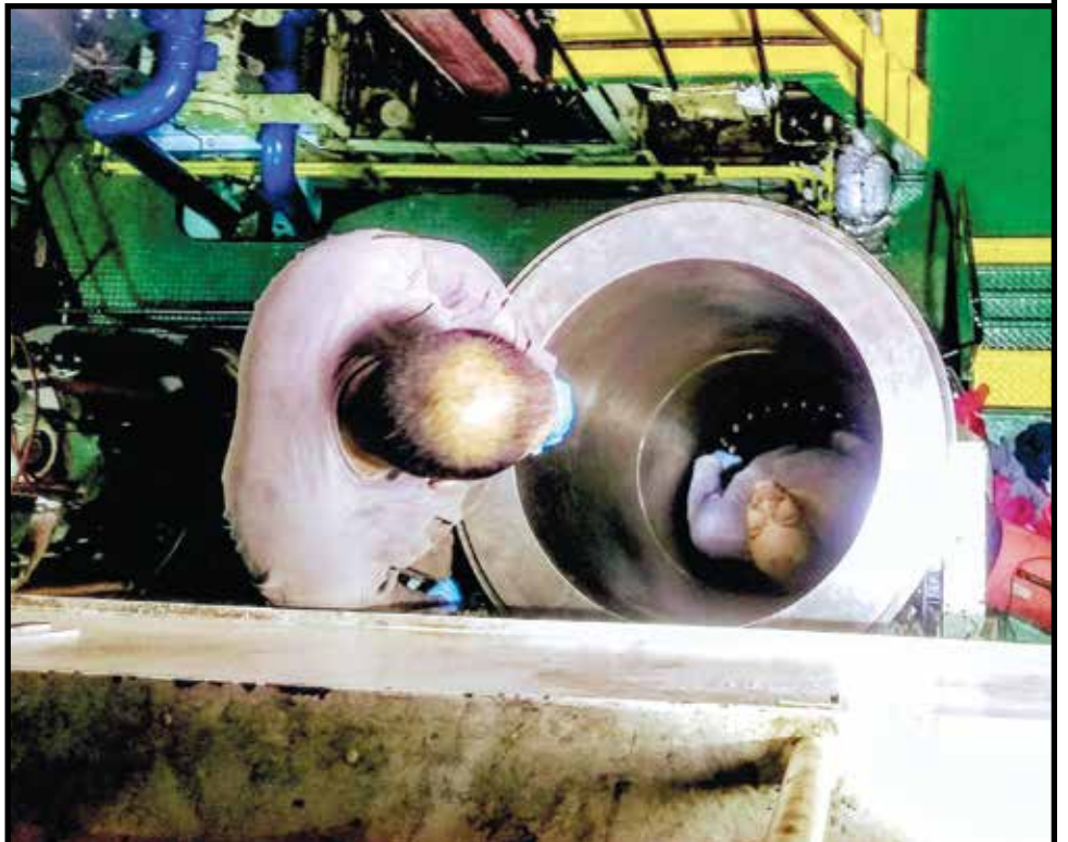
MV APL Saipan Wiper Tony Zarriello, JM-5329, is cleaning a cylinder liner with assistance from Junior Engineer Tony Grace, JM-5217.
