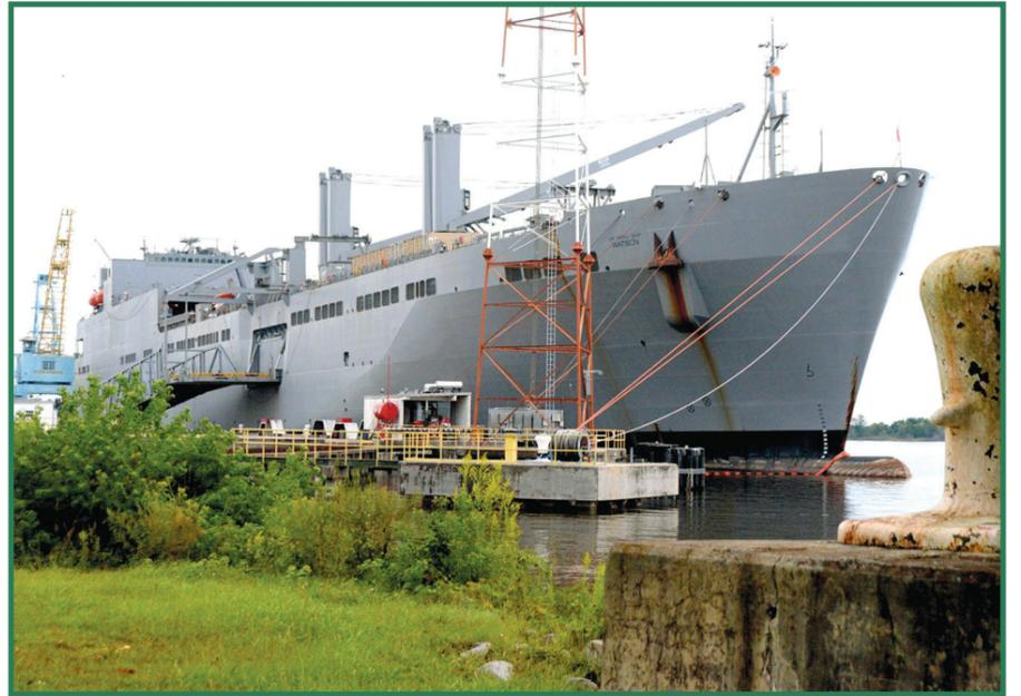
The *USNS Watson* pictured at Wharf Alpha, Naval Weapons Station-Joint Base Charleston, South Carolina. The large, medium-speed, roll-on roll-off (LMSR) vessels are ideal for the rapid loading and off-loading of Army wheeled and tracked vehicles, as well as other outsized Army equipment. A series of internal and external ramps makes this possible, and shipboard cranes allow cargo to be lifted without relying on local port infrastructure.
