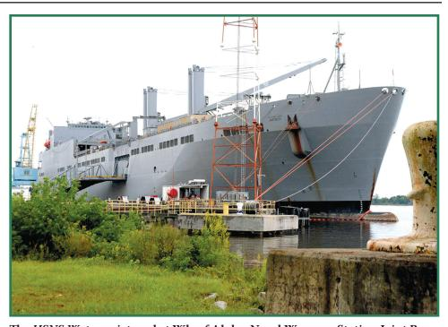
The USNS Watson pictured at Wharf Alpha, Naval Weapons Station-Joint Base Charleston, South Carolina. The large, medium-speed, roll-on roll-off (LMSR) vessels are ideal for the rapid loading and off-loading of Army wheeled and tracked vehicles, as well as other outsized Army equipment. A series of internal and external ramps makes this possible, and shipboard cranes allow cargo to be lifted without relying on local port infrastructure.
