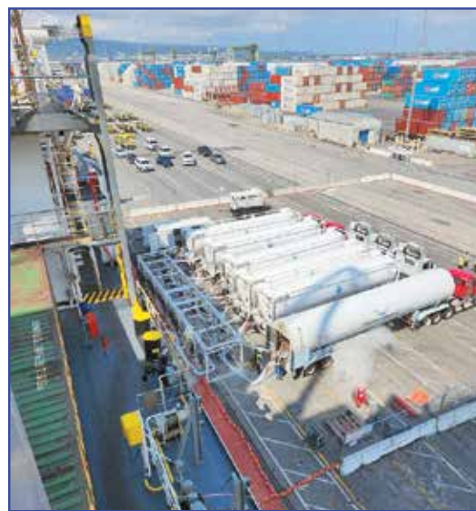
LNG tanker trucks in the Port of Long Beach refueling the MV Daniel K. Inouye.
