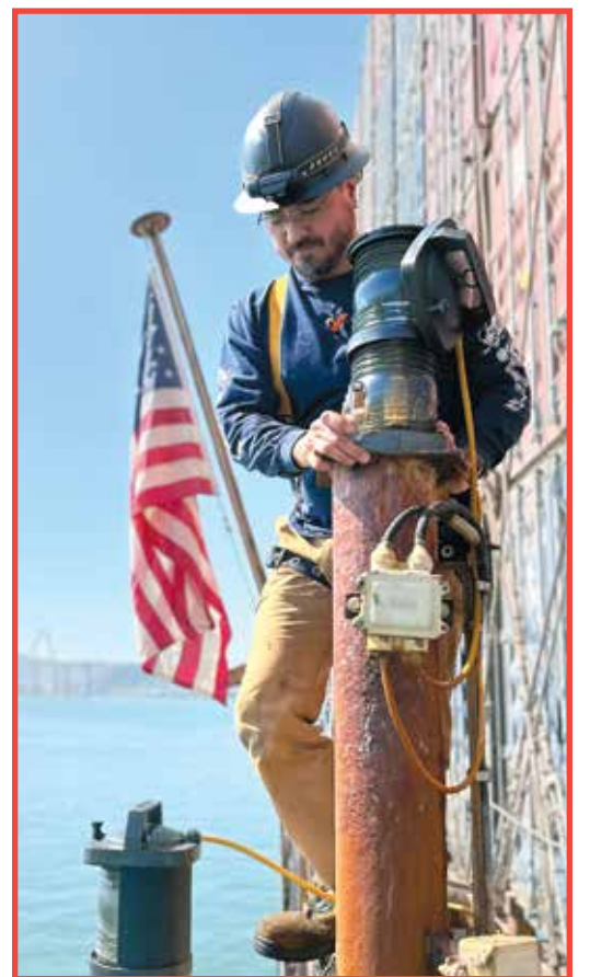
MV APL President FD Roosevelt ERJ John Ortiz, JM-5330, working on the stern anchor light in the Port of Oakland. The President FD Roosevelt is a 6600 TEU containership operated by APL Marine Services.
