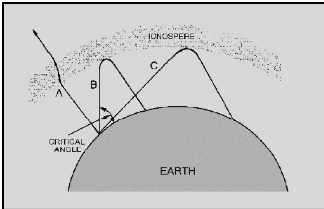
Figure 2-17 Different incident angles of radio waves
