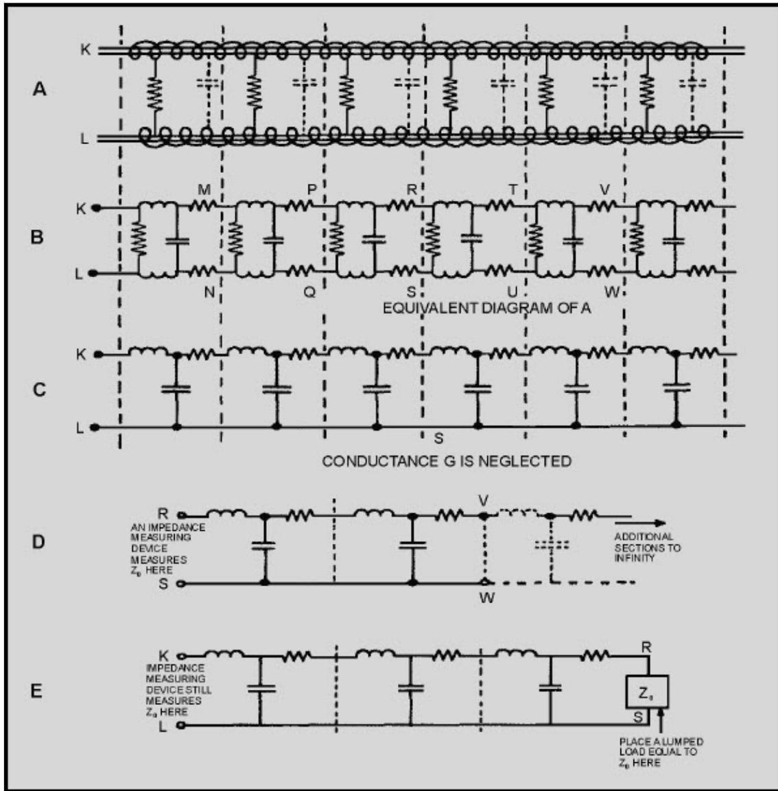
Figure 3-16 Characteristic impedance
