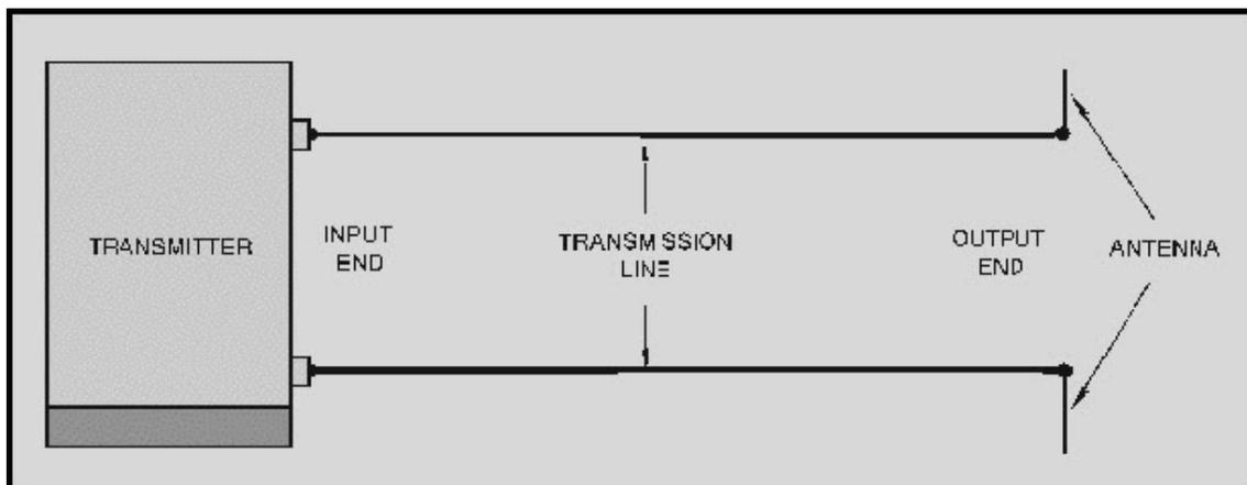
Figure 3-1 Basic transmission line
