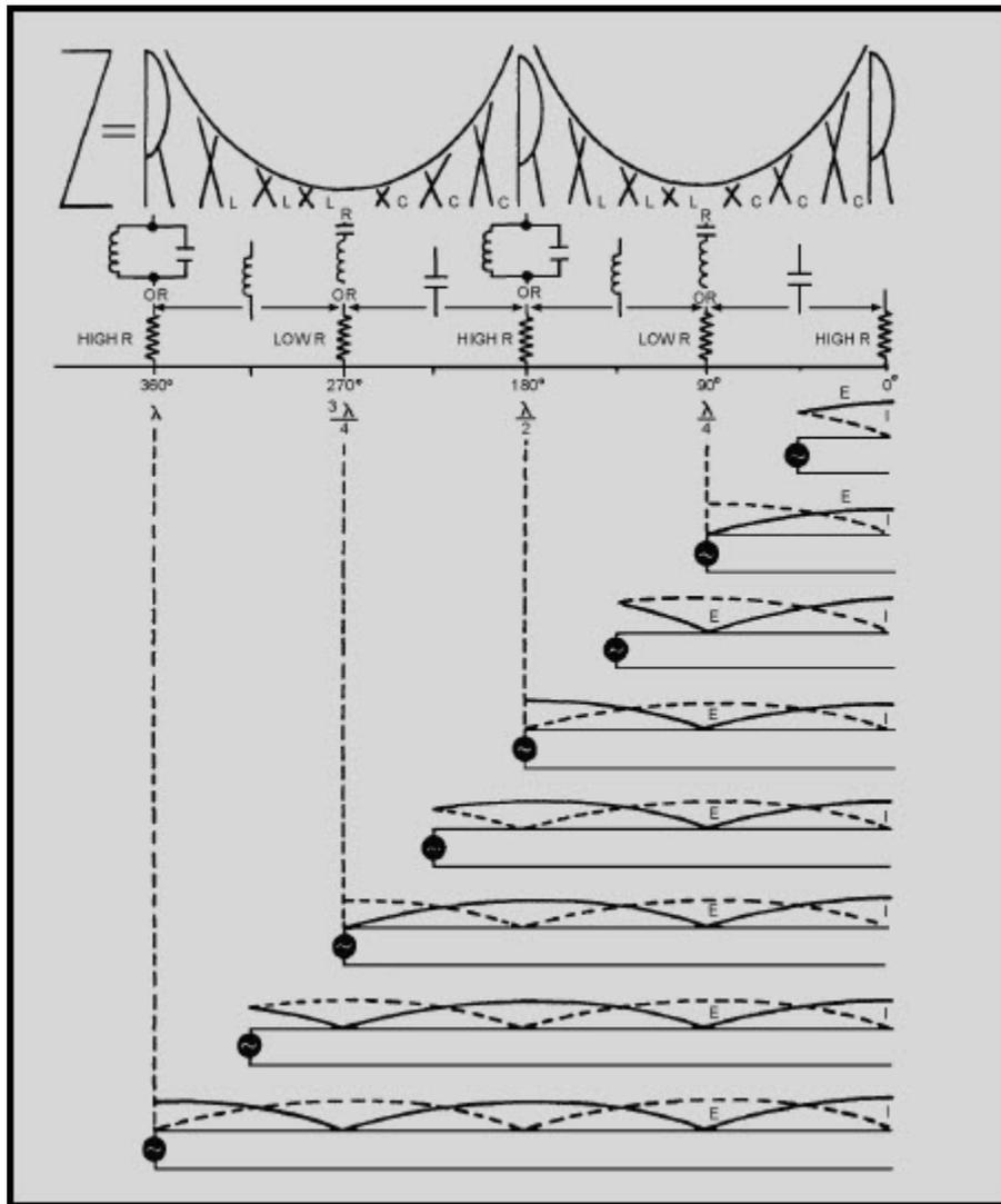
Figure 3-32 Voltage, current, and impedance on open line
