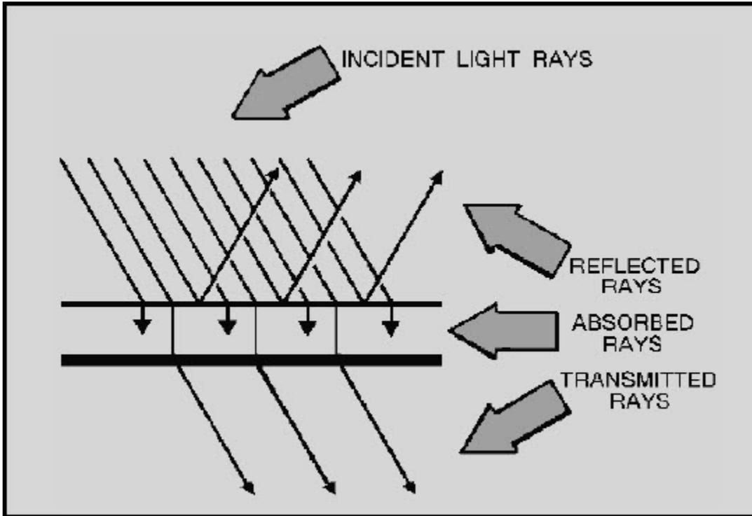
**Figure 1-19 Light waves reflected, absorbed, and transmitted**
