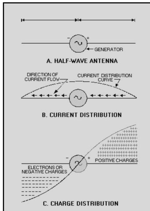
Figure 4-4 Current and voltage distribution on an antenna
