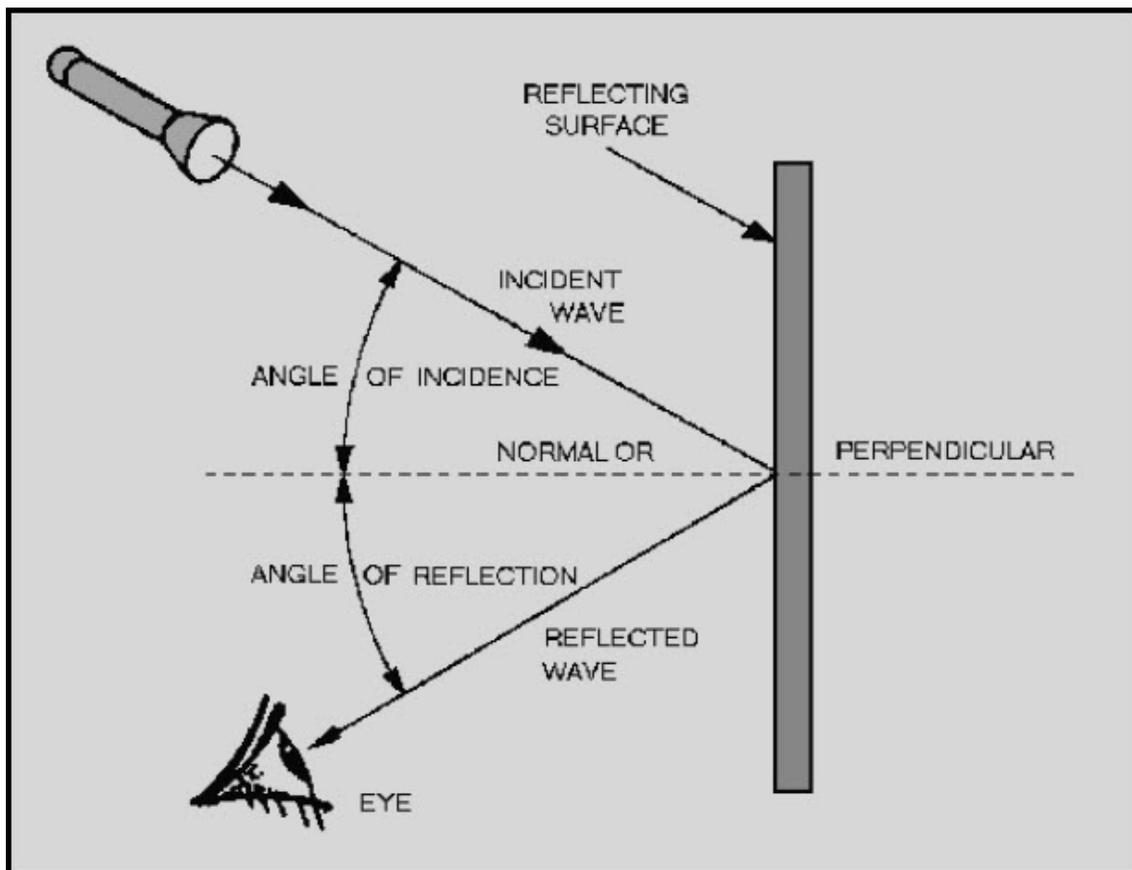
Figure 1-9 Reflection of a wave
