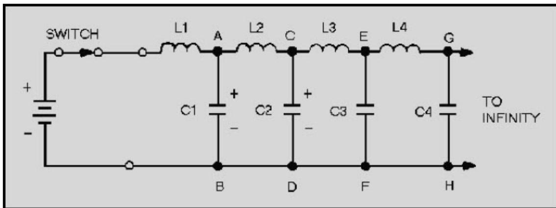
Figure 3-20 Dc applied to an equivalent transmission line
