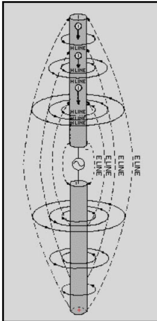
Figure 1-30 Relationship of E-lines, and current flow
