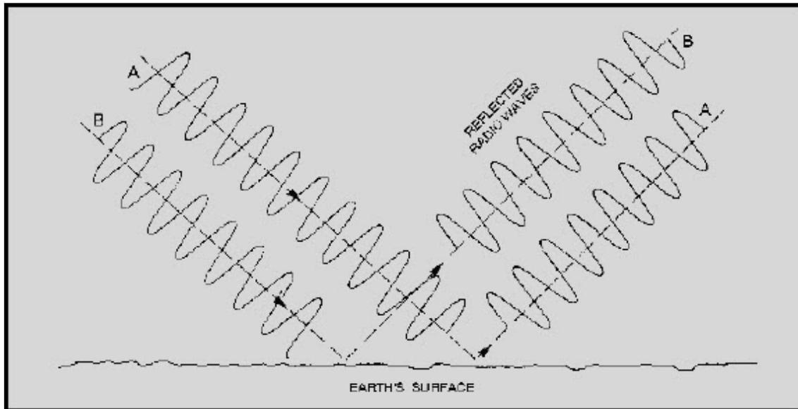
**Figure 2-7 Phase shift of reflected radio waves**
