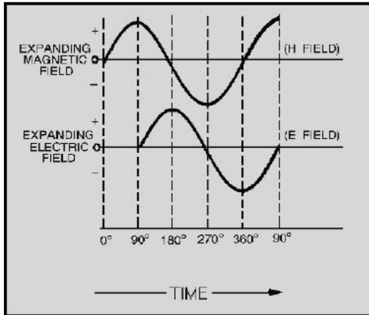
Figure 2-2 Phase relationship of induction field components
