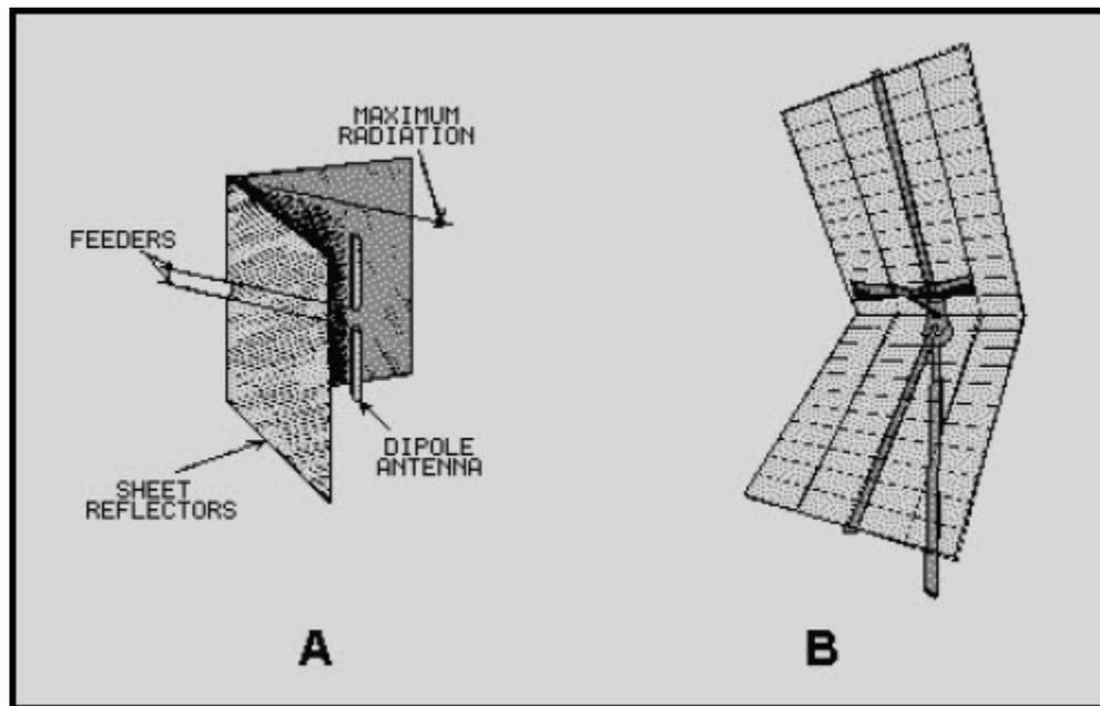
Figure 4-42 Corner-reflector antennas
