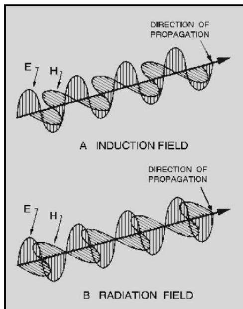
**Figure 2-4 E and H components of
