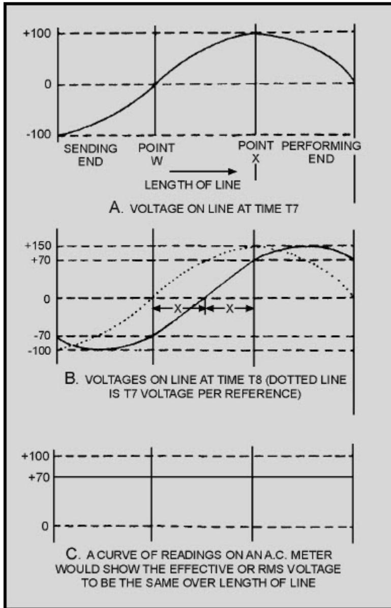
**Figure 3-22 Instantaneous voltages along a transmission line**
