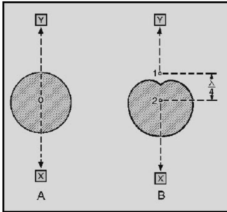
**Figure 4-21 Phasing of antenna in free space**
