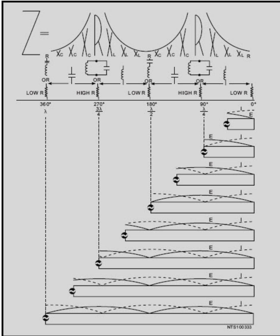
**Figure 3-33 Voltage, current, and impedance on shorted line**
