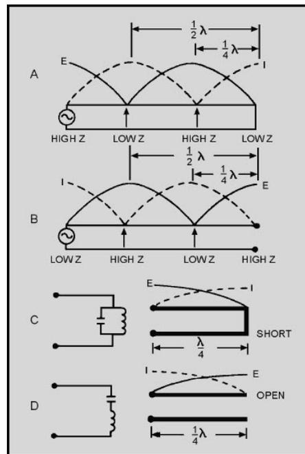
Figure 3-31 Sending-end impedance of various lengths and terminations
