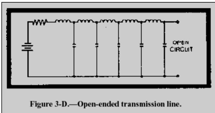
Figure 3-D.—Open-ended transmission line.
