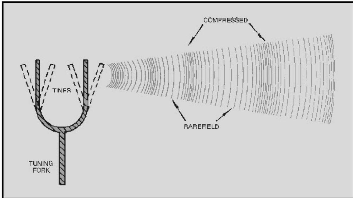
**Figure 1-5 Sound propagation by a tuning fork**
