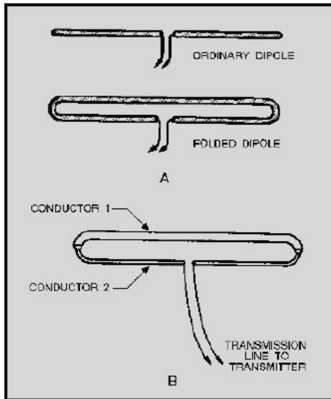
Figure 4-20 Folded-dipole antennas
