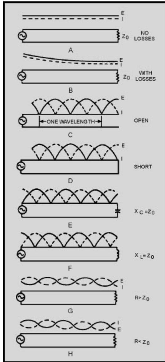
Figure 3-34 Effects of various terminations on standing waves
