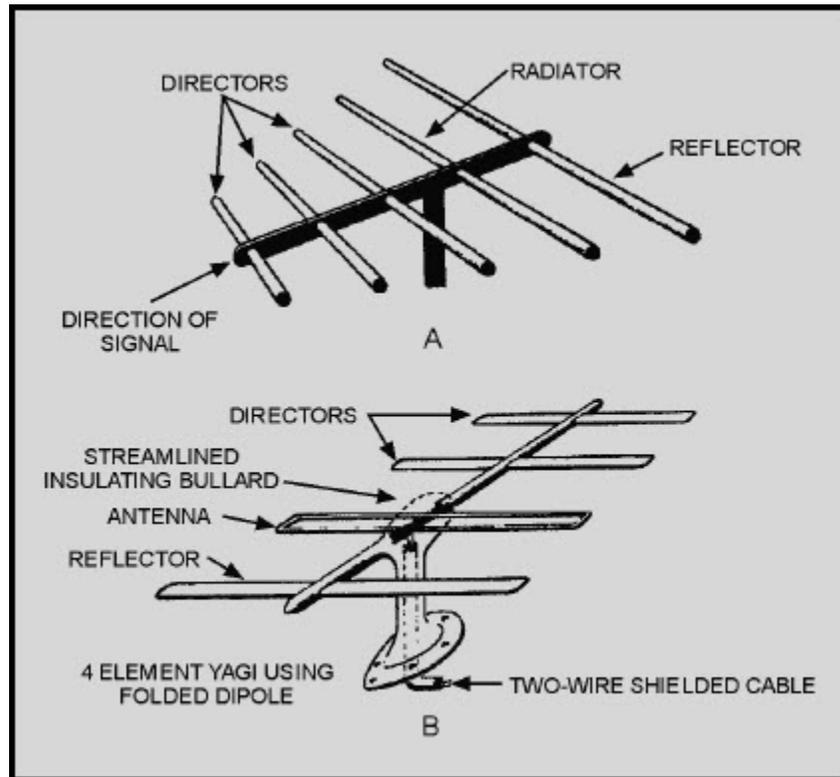
Figure 4-32 Yagi antenna
