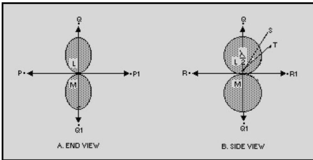
Figure 4-29 Parallel elements 180 degrees out of phase
