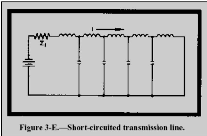
Figure 3-E.—Short-circuited transmission line.
