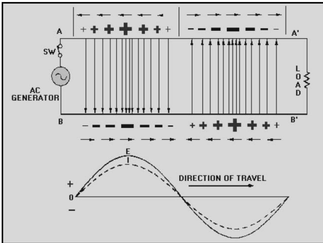
Figure 3-19 Ac voltage applied to a line
