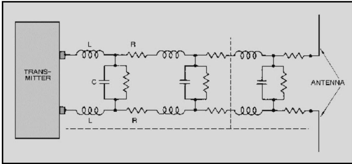
Figure 3-9 Equivalent circuit of a two-wire transmission line
