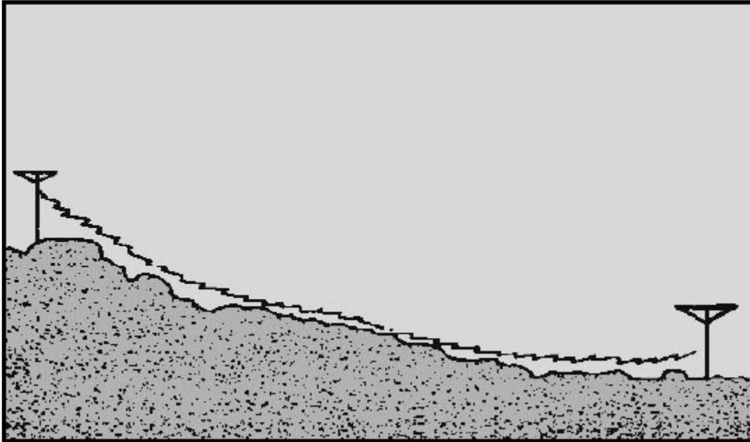
**Figure 2-12 Surface wave propagation**
