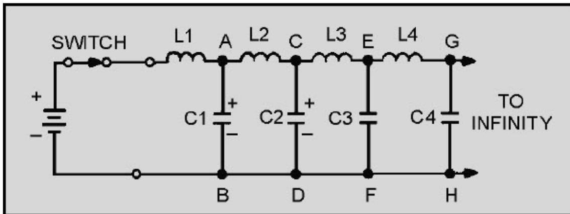
Figure 3-23 Dc applied to an equivalent transmission line
