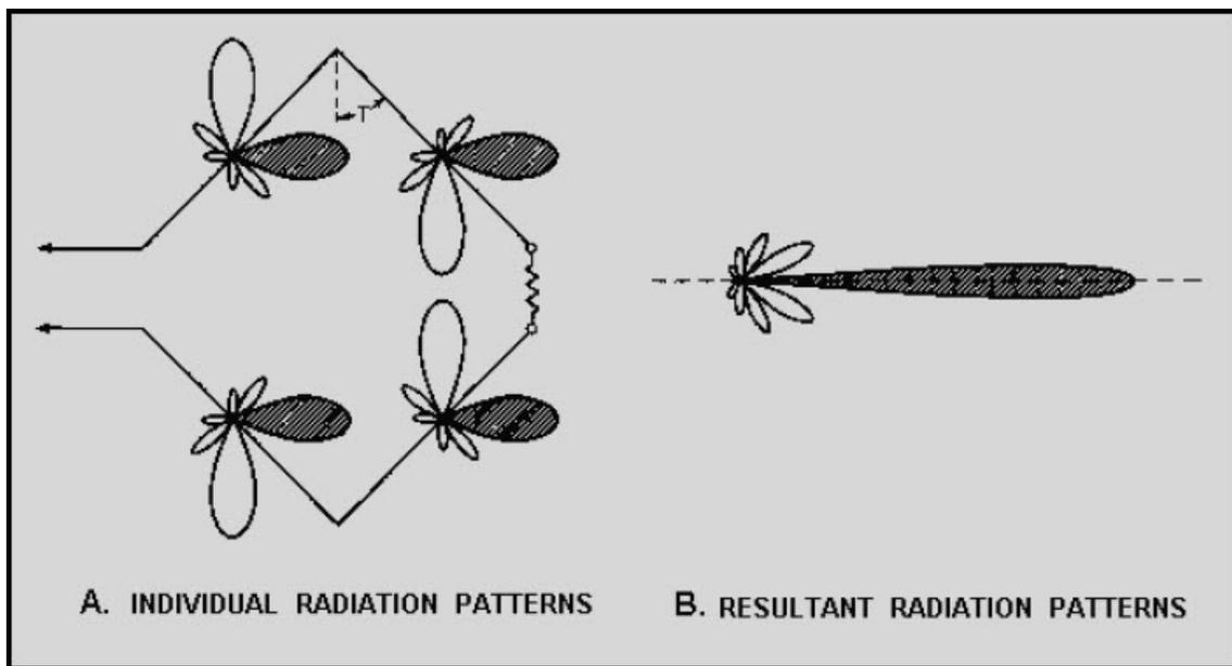
Figure 4-38 Formation of a rhombic antenna beam
