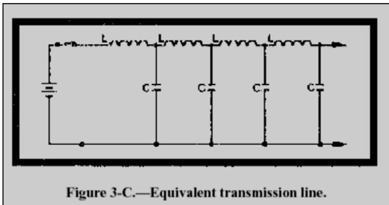
Figure 3-C.—Equivalent transmission line.
