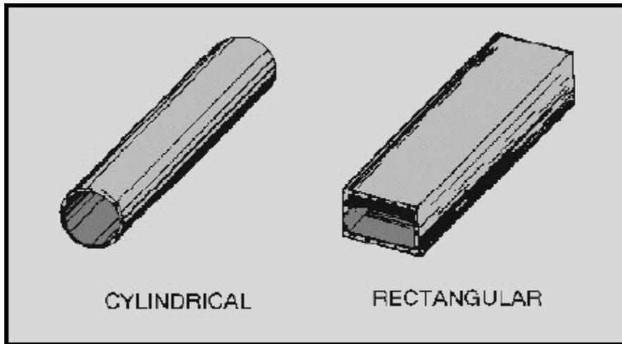
Figure 3-8 Waveguides
