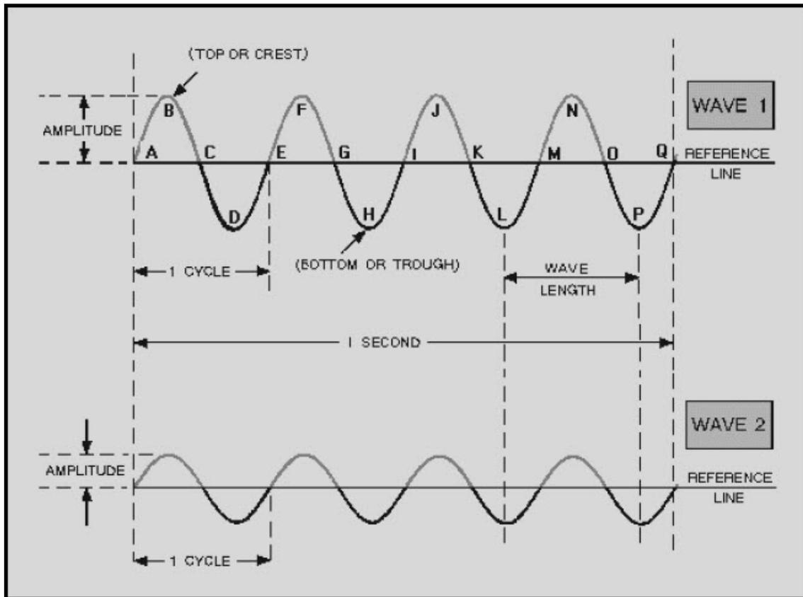
**Figure 1-7 Comparison of waves with different amplitudes**
