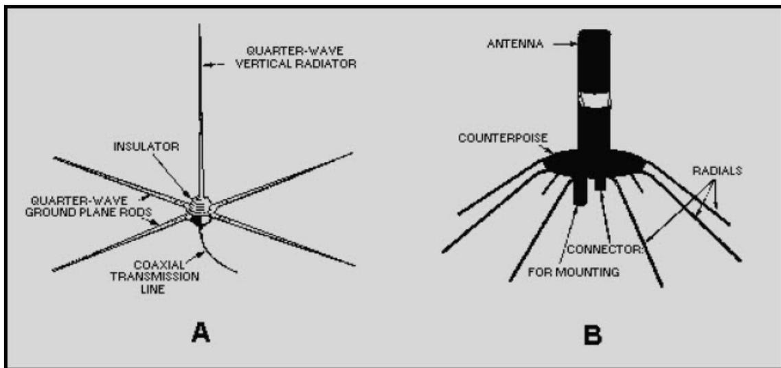
Figure 4-41 Ground-plane antennas
