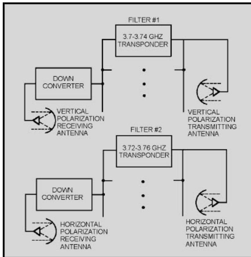
Figure 4-8 Satellite transmissions using polarized radiation
