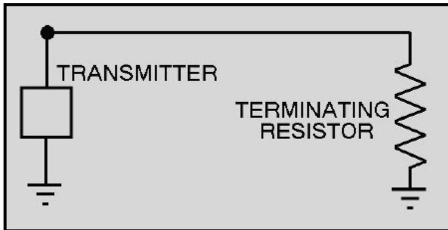
Figure 4-34 Beverage antenna
