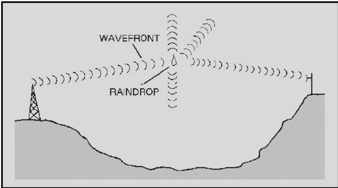
Figure 2-24 Rf energy losses from scattering
