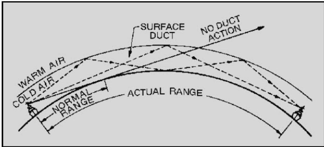
**Figure 2-25 Duct effect caused by temperature inversion**
