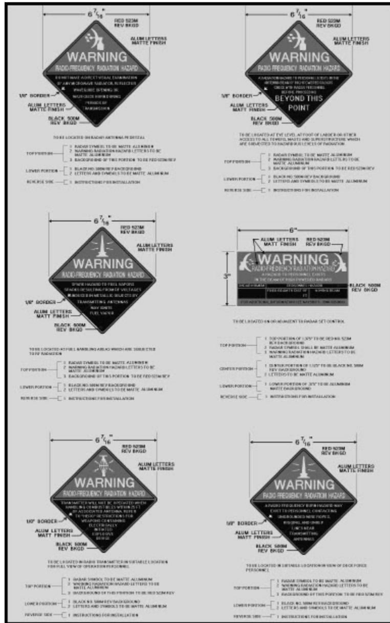
Figure 4-43 Examples of rf radiation warning signs
