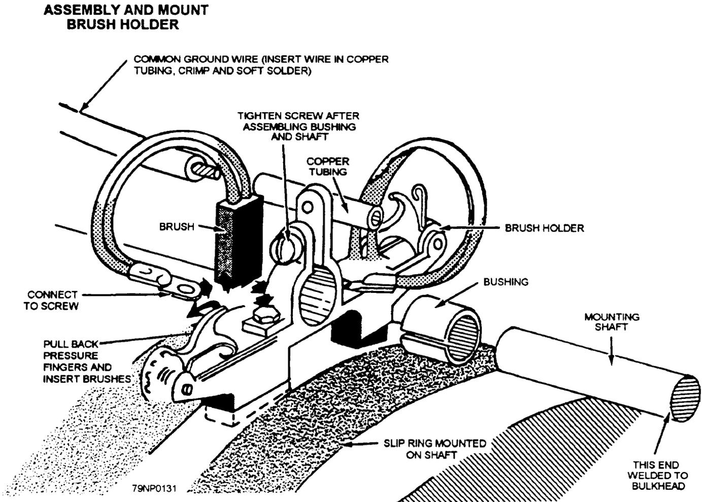
Figure 11-8.—Shaft grounding assembly.
