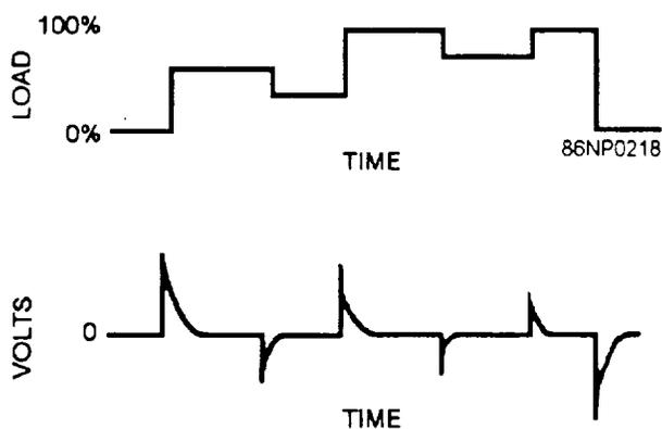
Figure 9-11.—Comparison of load pulse signals to load changes.
