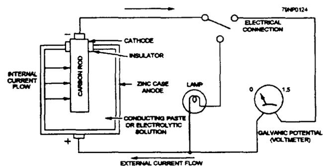
Figure 11-1.—Dry-cell battery circuit.
