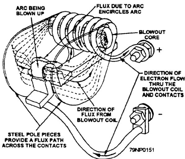
Figure 6-10.—Action of a magnetic blowout coil.
