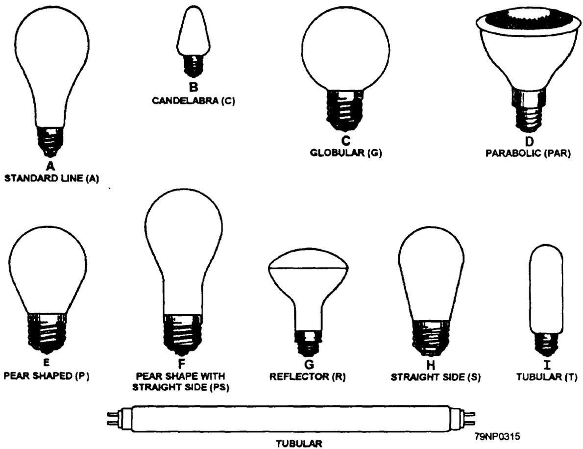
Figure 4-5.—Classification of lamps according to the shape of the bulb.
