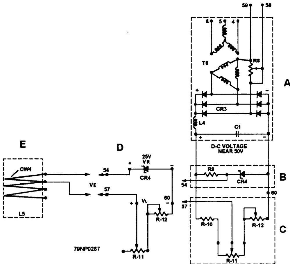
Figure 8-18.—Automatic voltage regulator.
