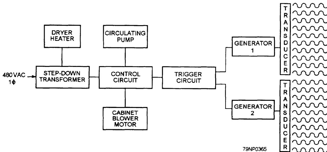
Figure 5-17.—Block diagram of ultrasonic cleaner.
