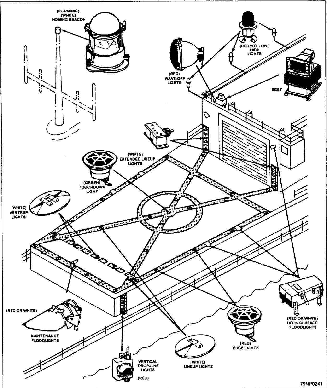
Figure 12-1.—Typical VLA installations with flight deck and hangar on 0-1, dual landing approach.
