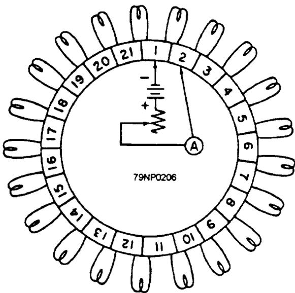
Figure 7-37.—Schematic of a simplex lap winding.
