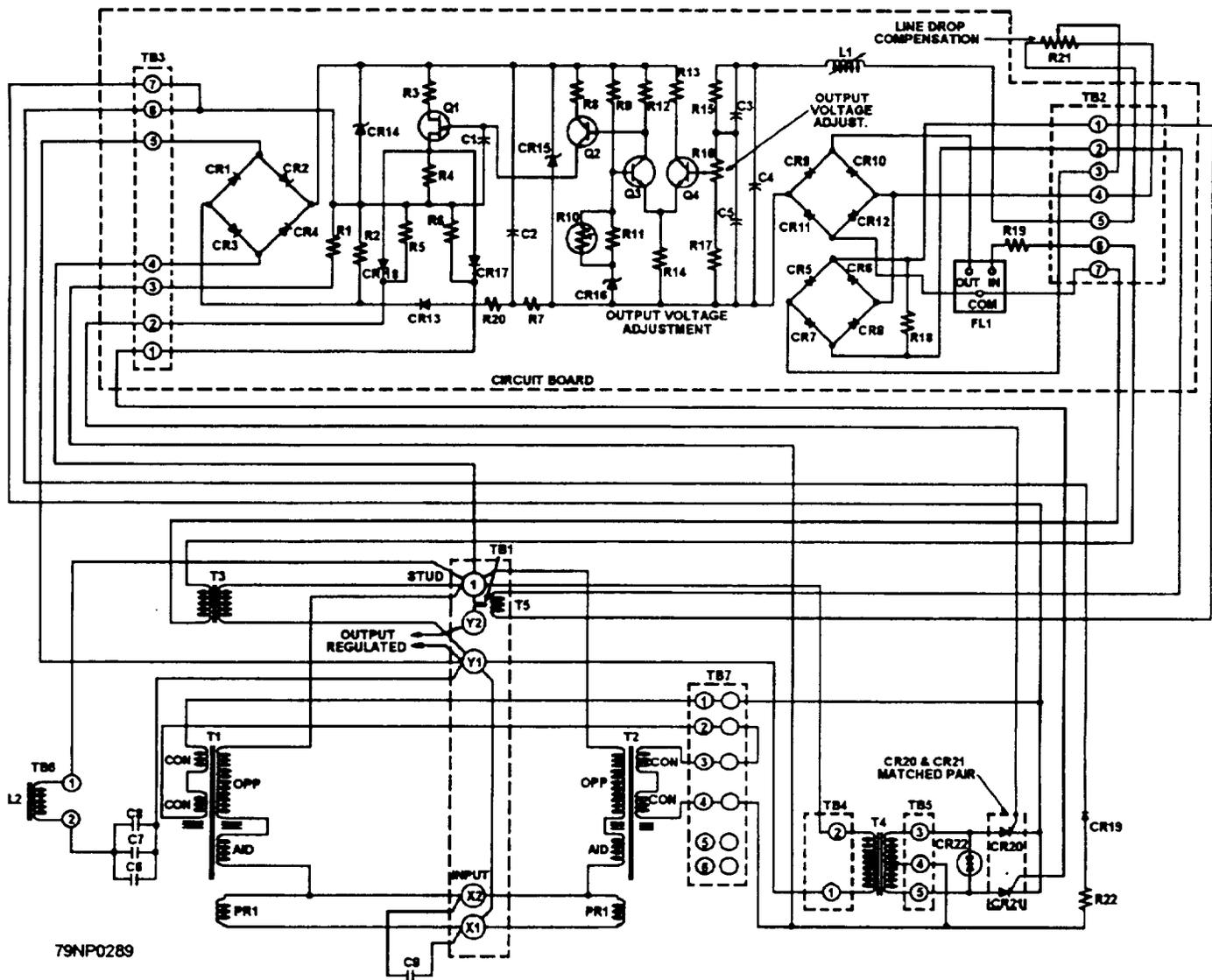
Figure 8-20.—SPR-400 line voltage regulator.
