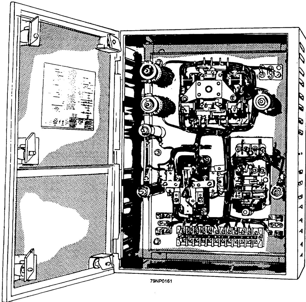
Figure 6-20.—A typical dc controller.
