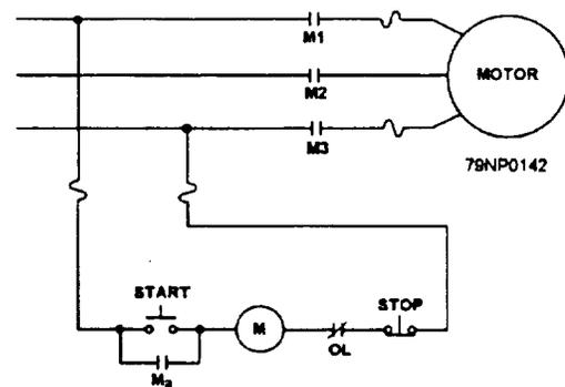
Figure 6-1.—Schematic of a simple across-the-line controller.
