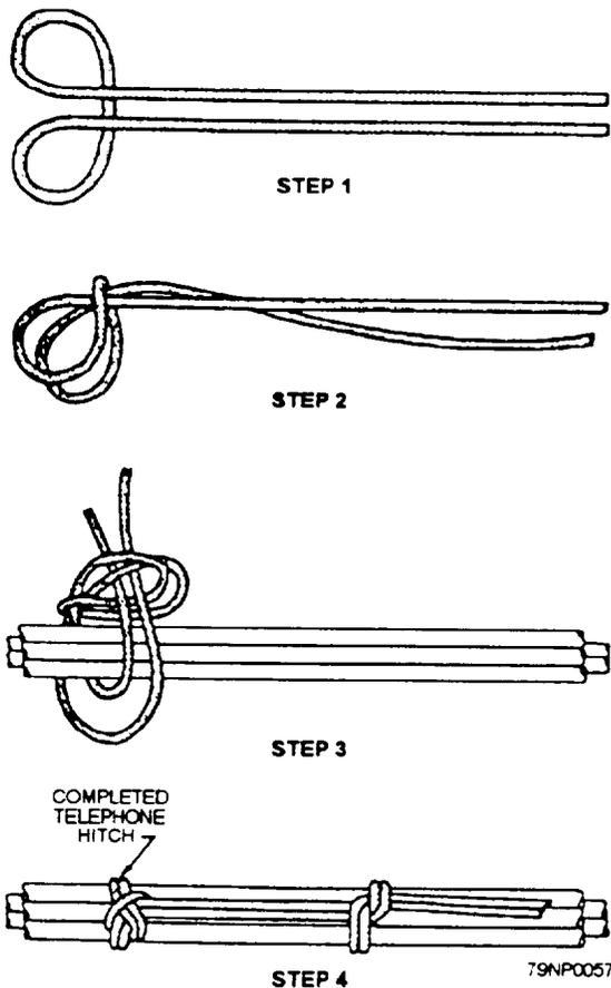
Figure 2-10.—Starting double lace with the telephone hitch.
