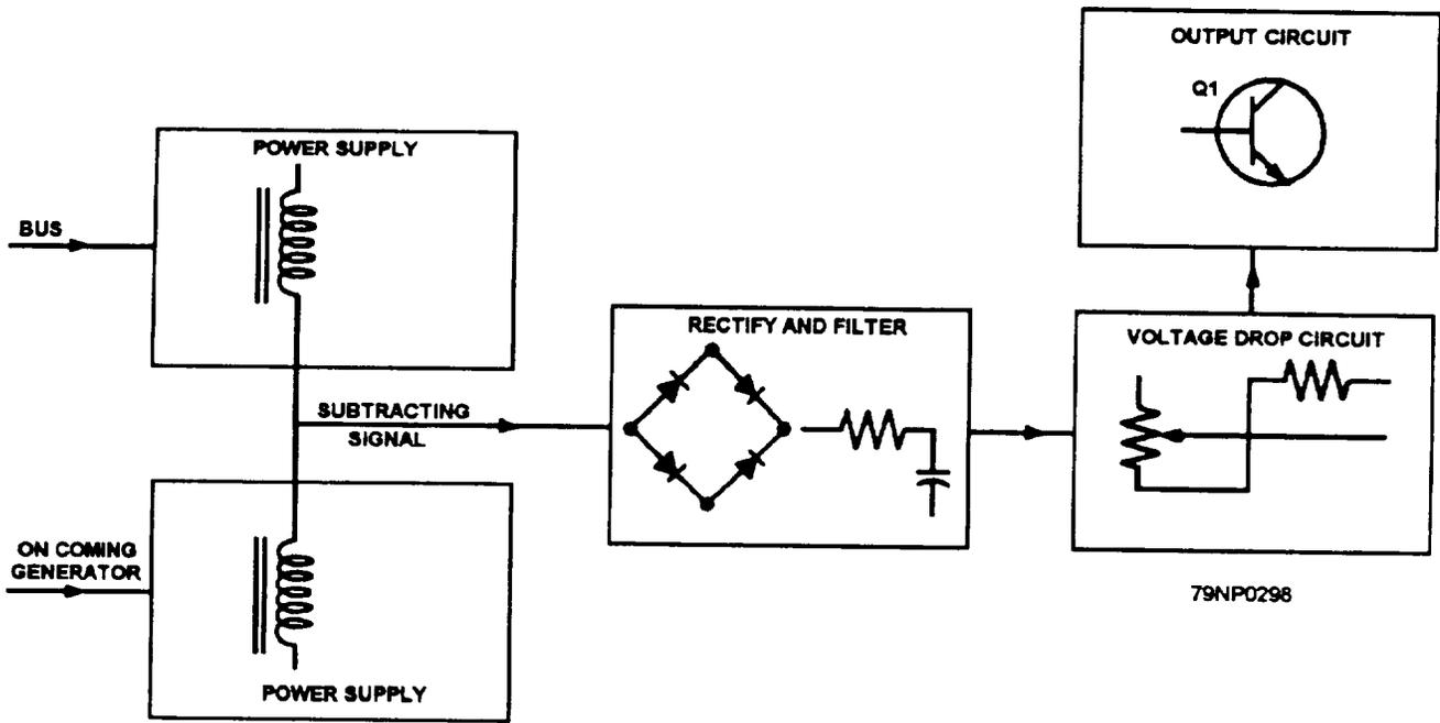
Figure 8-29.—Block diagram of phase difference monitoring circuit.
