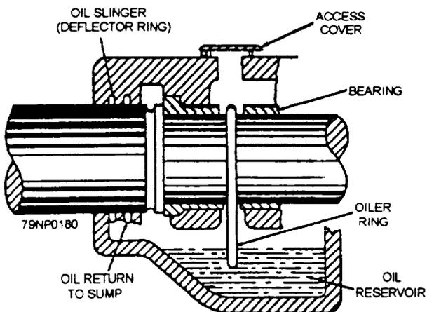
Figure 7-9.—Diagram of an oil-lubricated bearing.
