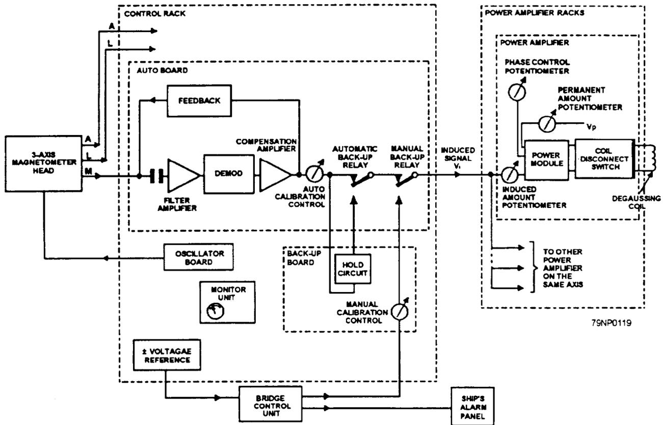
Figure 10-13.—Block diagram for type MDG degaussing system.
