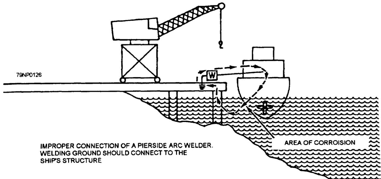
Figure 11-3.—Stray-current corrosion.
