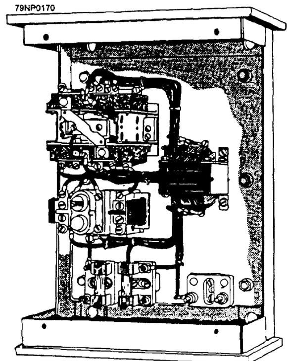
Figure 6-29.—Typical three-phase controller.
