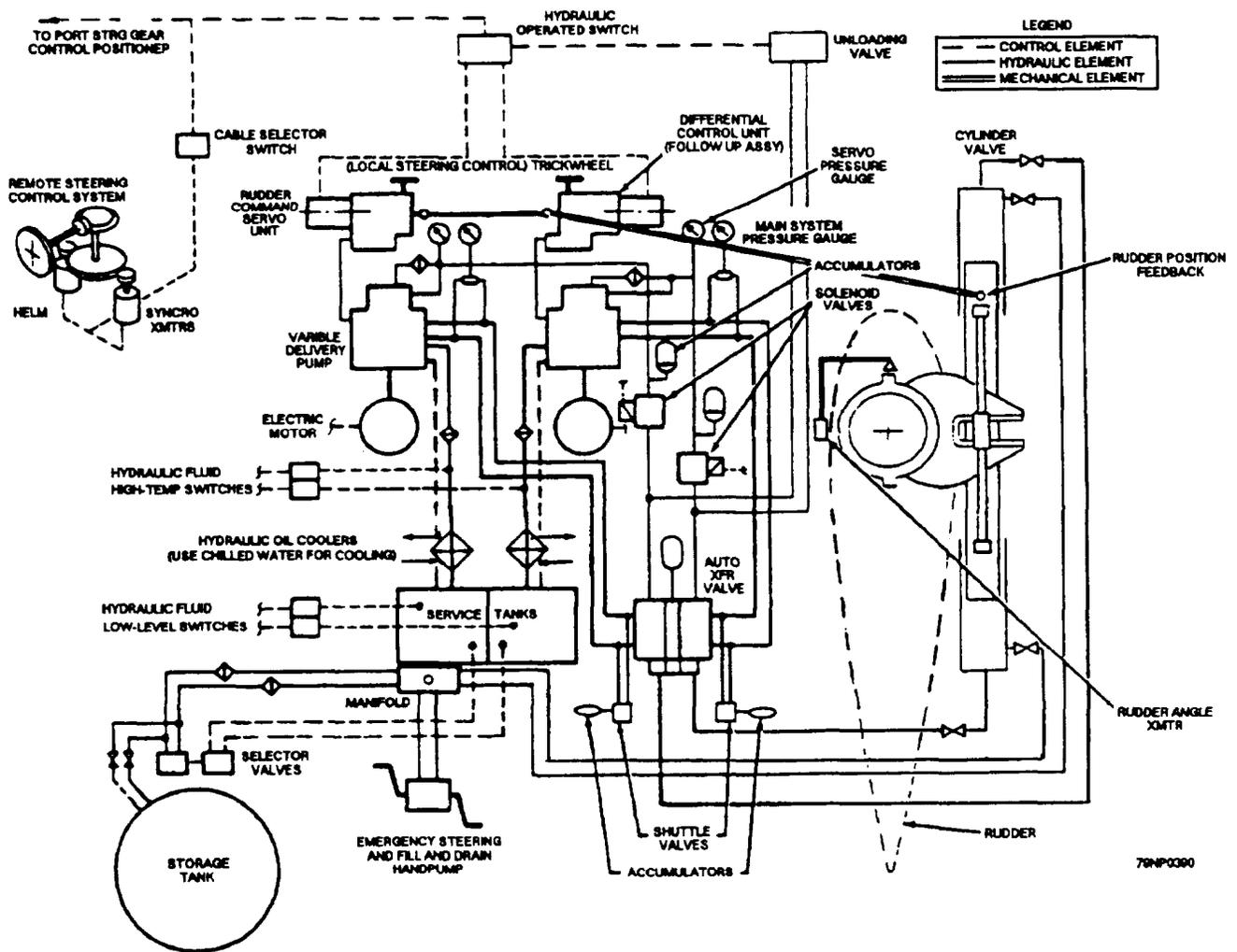
Figure 5-42.—Steering gear functional block diagram.
