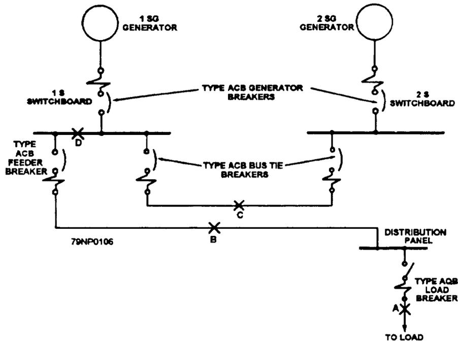
Figure 2-59.—Selected tripping of circuit breakers.
