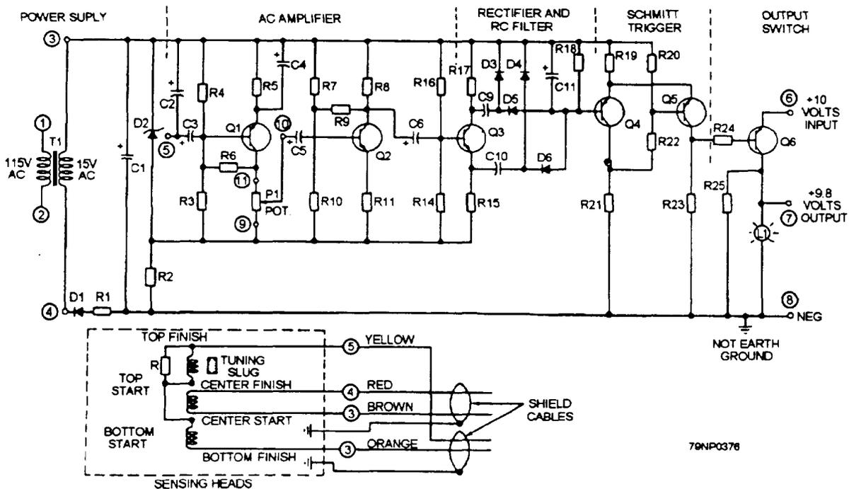
Figure 5-28.—Schematic diagram of a proximity limit switch.
