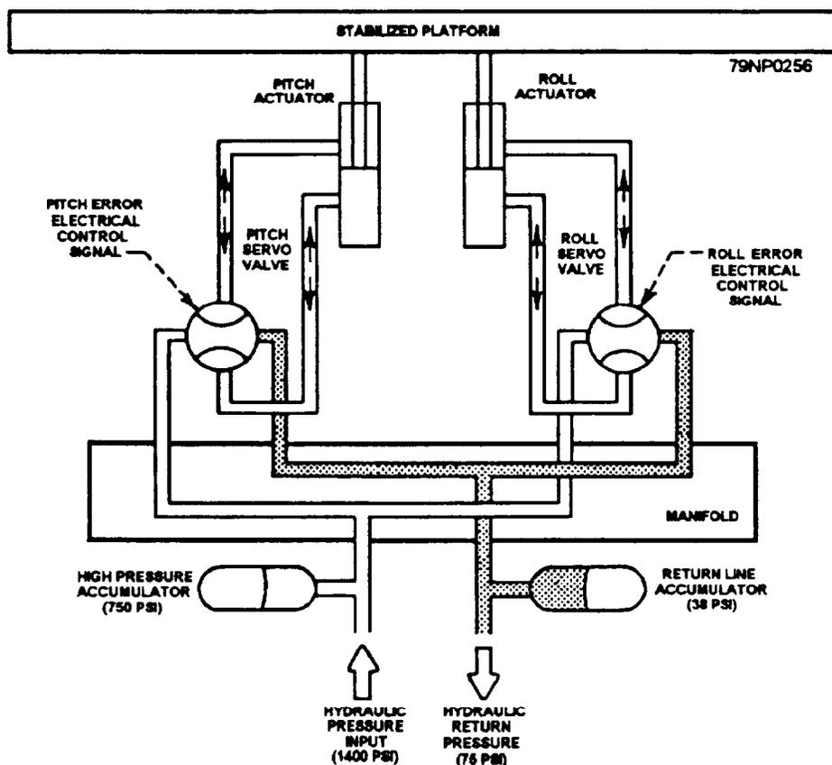
Figure 12-15.—Function diagram of the stabilized platform assembly.
