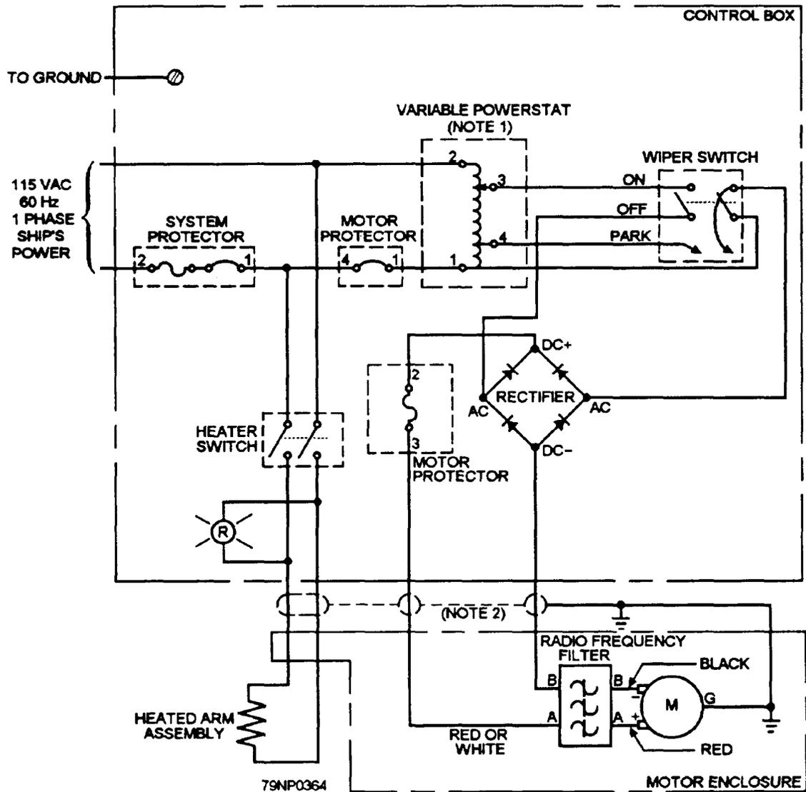
Figure 5-16.—Window wiper schematic.
