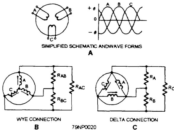
Figure 3-20.—Three-phase ac generator.
