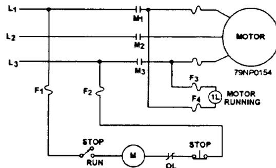
Figure 6-13.—Schematic of simple LVR controller.
