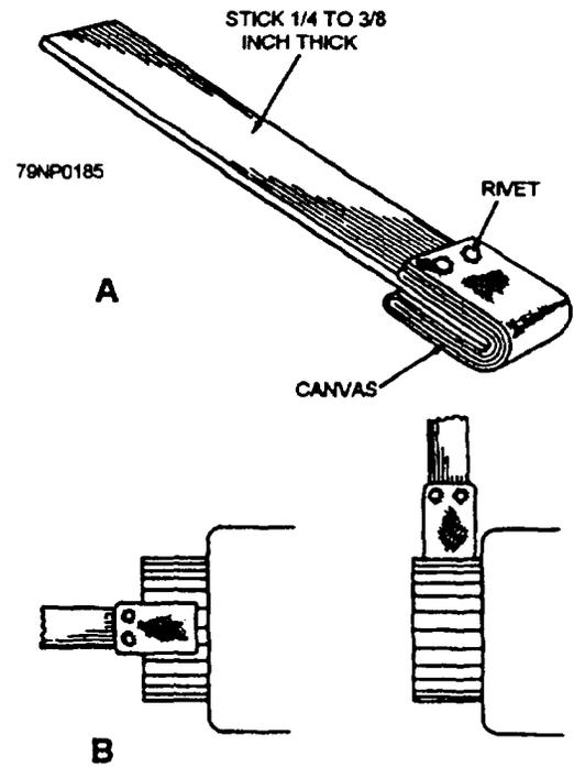
Figure 7-15.—Cleaning commutator or collector rings.
