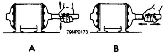
Figure 7-2.—Checking motor or generator shaft. (A) Vertical movements: (B) End-play movement.
