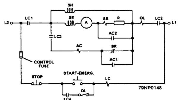
Figure 6-7.—Schematic of a dc resistor controller with one stage of acceleration.
