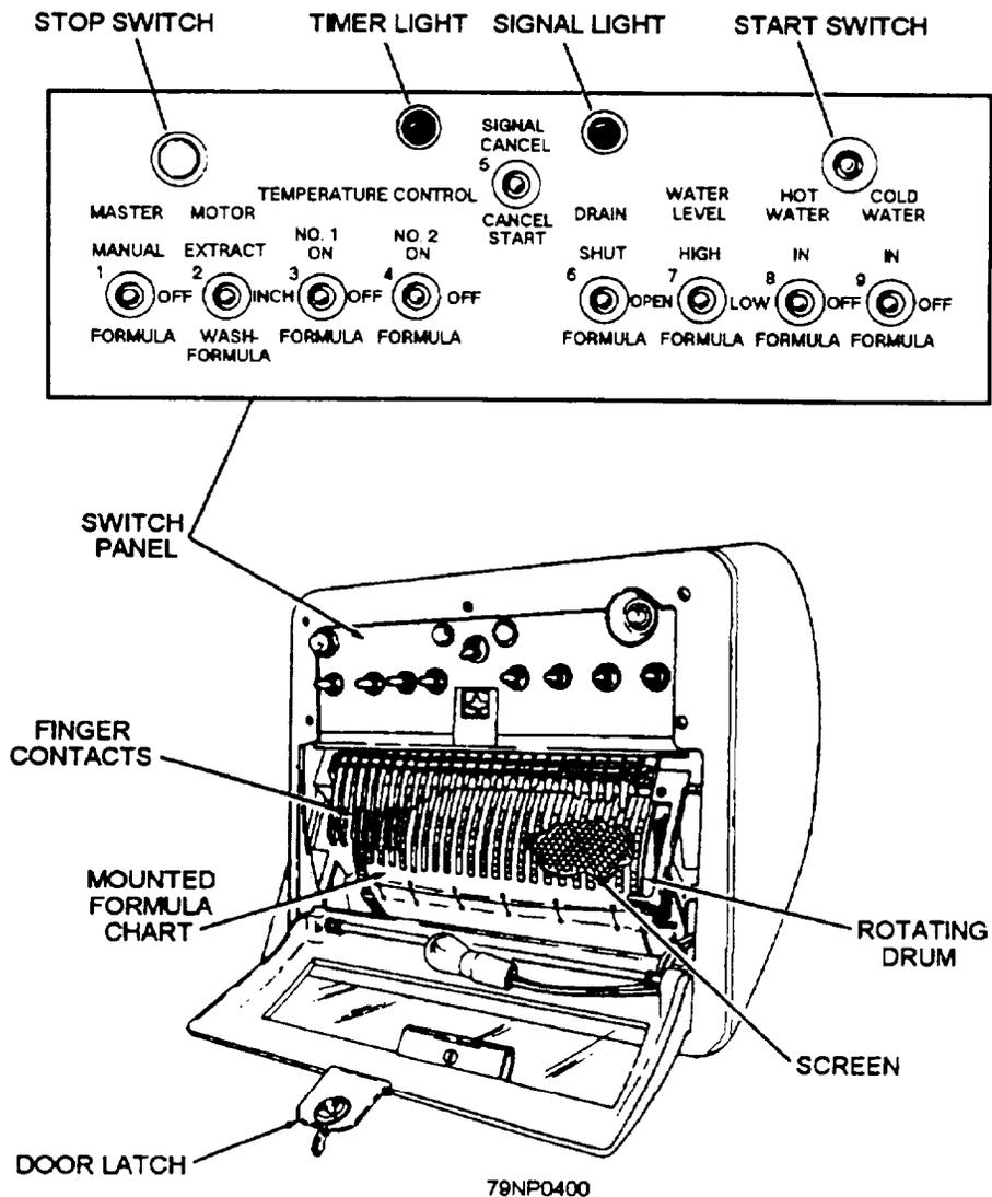
Figure 5-52.—A typical automatic control timer.
