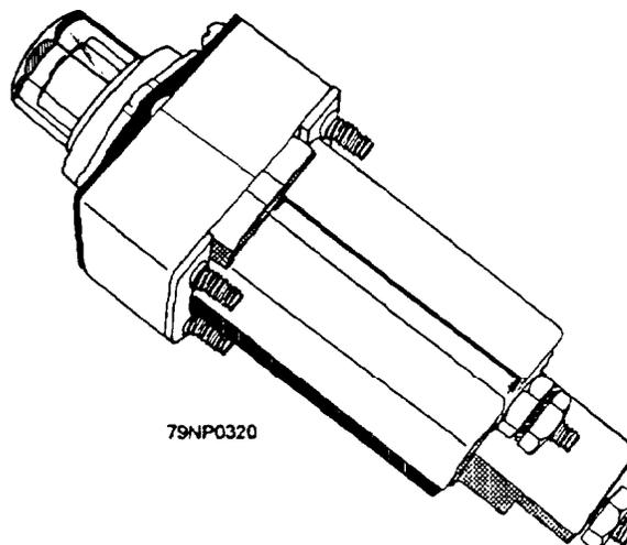
Figure 4-10.—Fuse holder with glow lamp.
