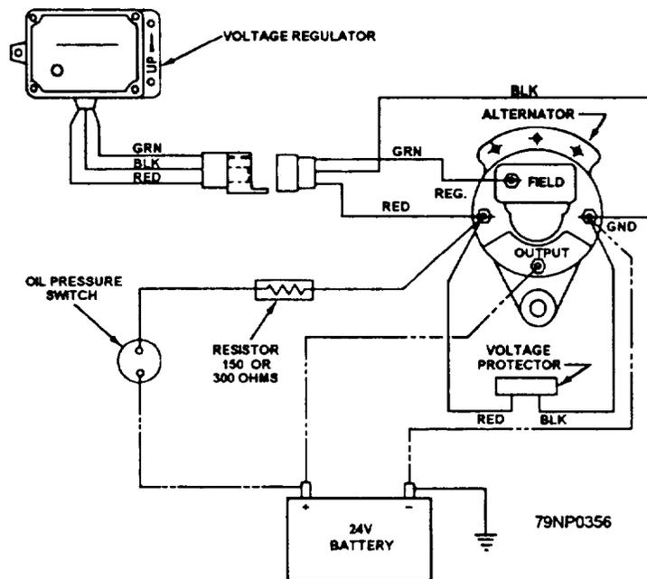
Figure 5-7.—A typical alternator electrical system wiring diagram.
