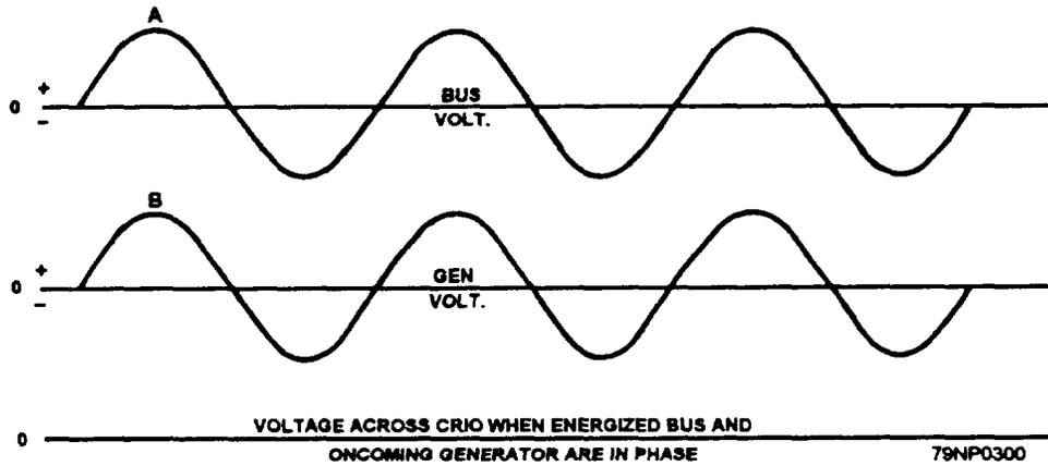
Figure 8-31.—Input voltage to CR10 (in phase).
