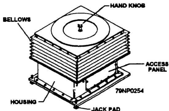
Figure 12-14.—stabilized platform assembly.
