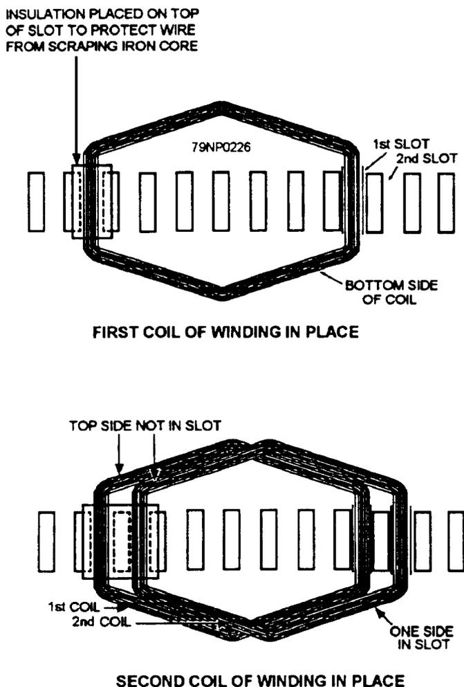
Figure 7-59.—Placing coil sides in slots.
