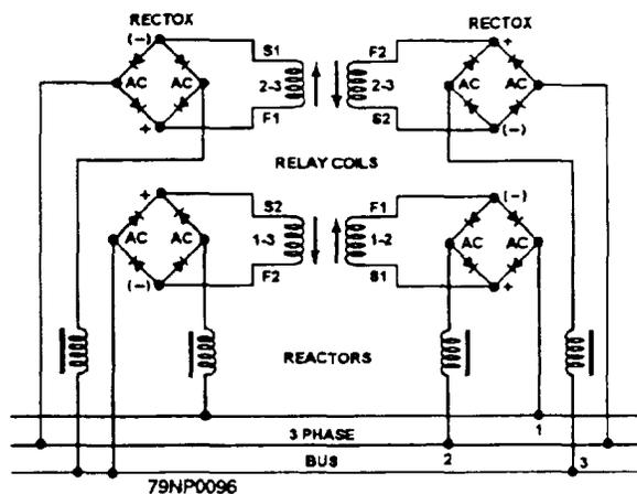
Figure 2-19.—Schematic wiring of a phase-failure relay.
