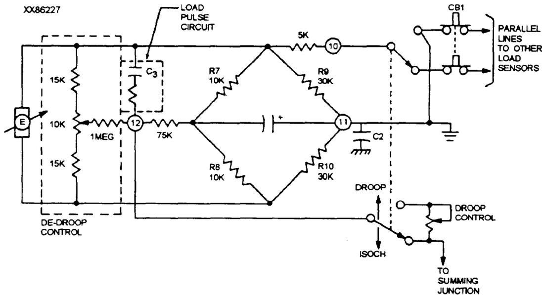
Figure 9-22.-Basic load sensor, single-unit configuration.
