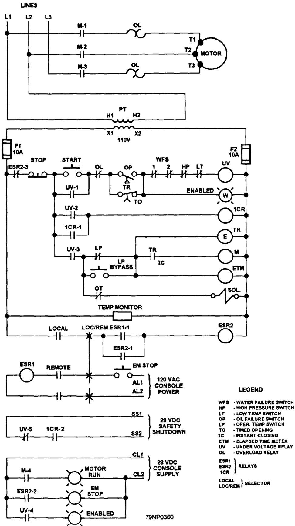
Figure 5-12.—80-ton air-conditioning compressor wiring diagram.
