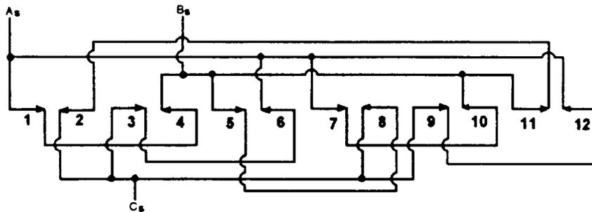
Figure 7-64.—Three-phase, four-pole, parallel-delta winding.
