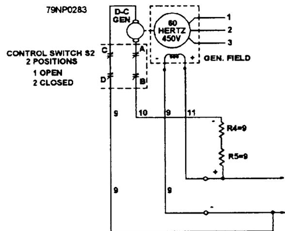
Figure 8-14.—Field-flashing circuit.
