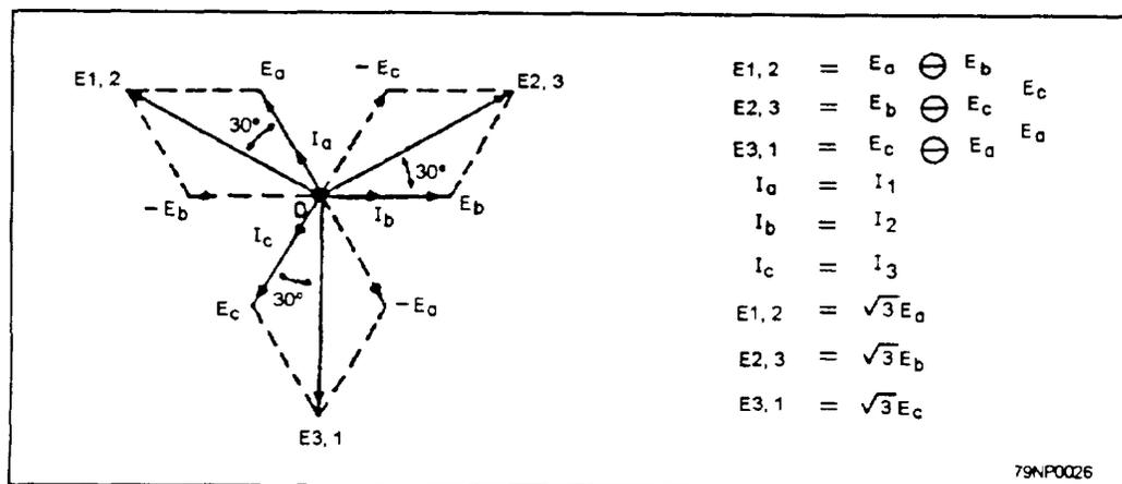
Figure 3-26.—Three-phase, wye-connected system.
