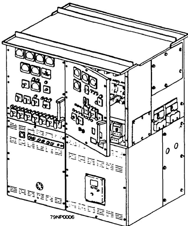
Figure 3-6.—1S Ship's service switchboard.
