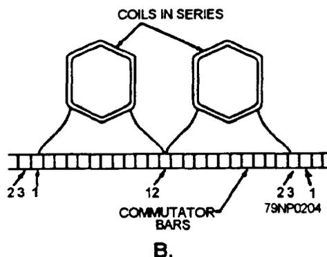
Figure 7-35.—Four-pole simplex wave windings.
