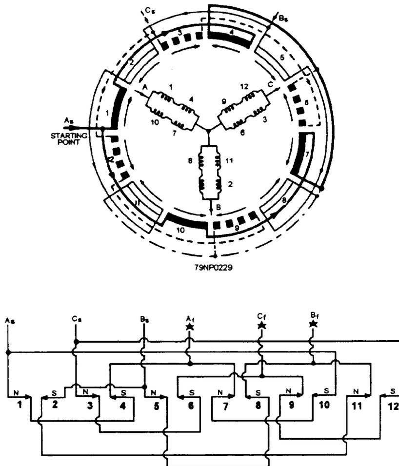
Figure 7-62.—Three-phase, four-pole, parallel-wye winding.
