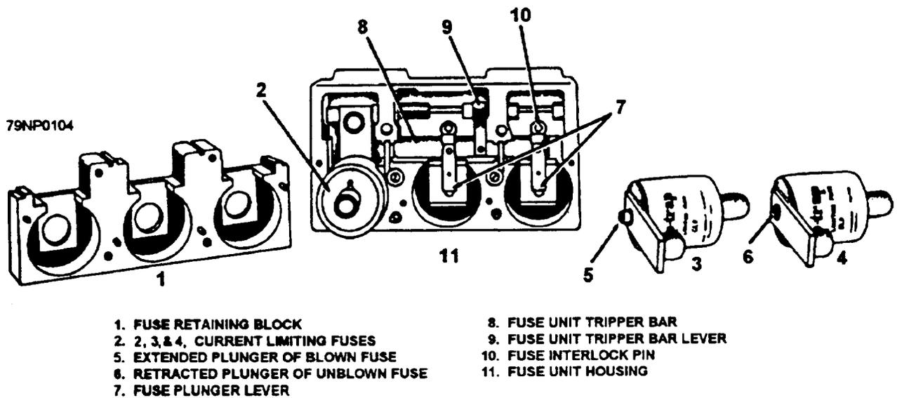
Figure 2-57.—Current-limiting fuse unit assembly.
