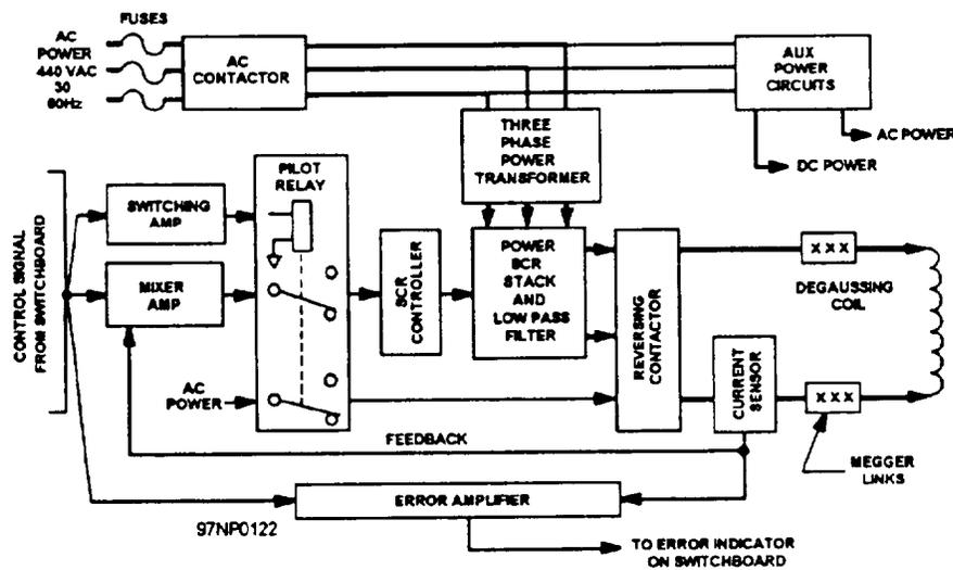
Figure 10-16.—Block diagram for a type SSM degaussing power supply.
