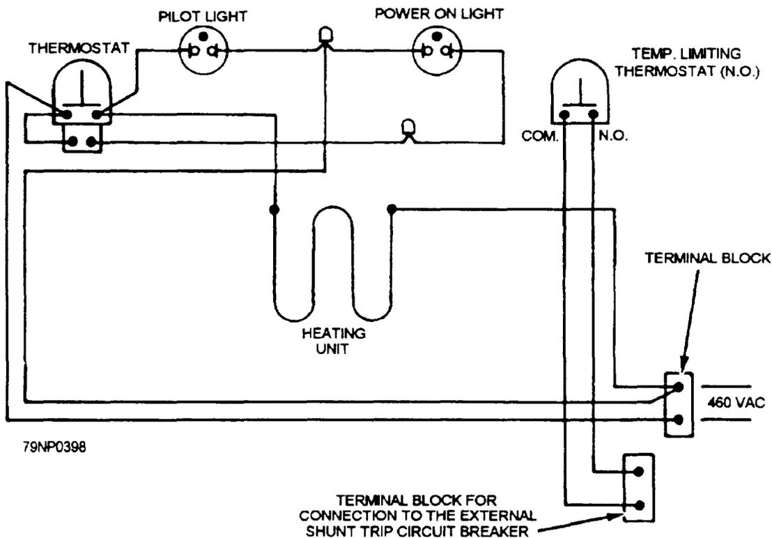
Figure 5-50.—Wiring diagram of the Mk 721 deep fat fryer.
