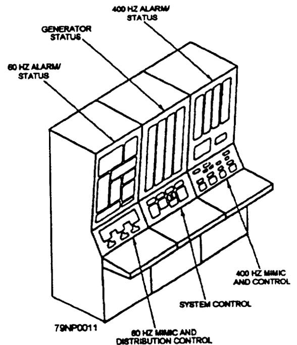
Figure 3-11.—Electric plant control console (EPCC).
