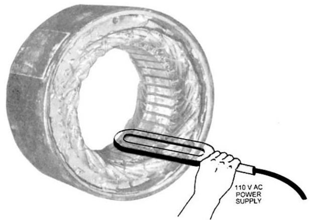
Figure 7-57.—Testing a three-phase stator for shorts.
