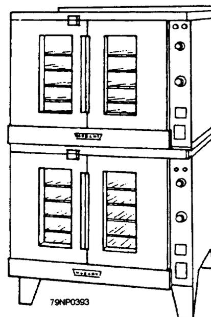
Figure 5-45.—M-series convection oven.
