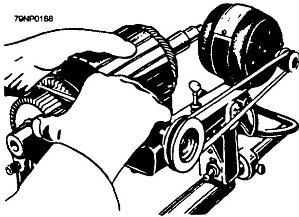
Figure 7-18.—Undercutting commutator mica with undercutter.
