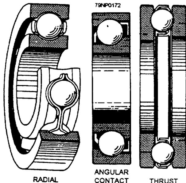
Figure 7-1.—Representative types of ball bearings.
