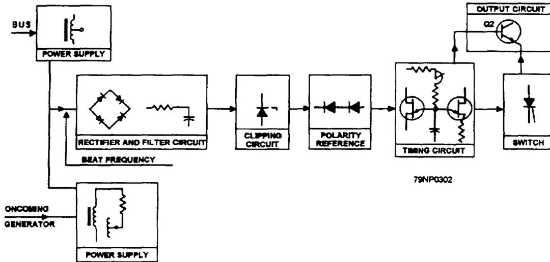
Figure 8-33.—Block diagram of frequency difference monitoring circuit.
