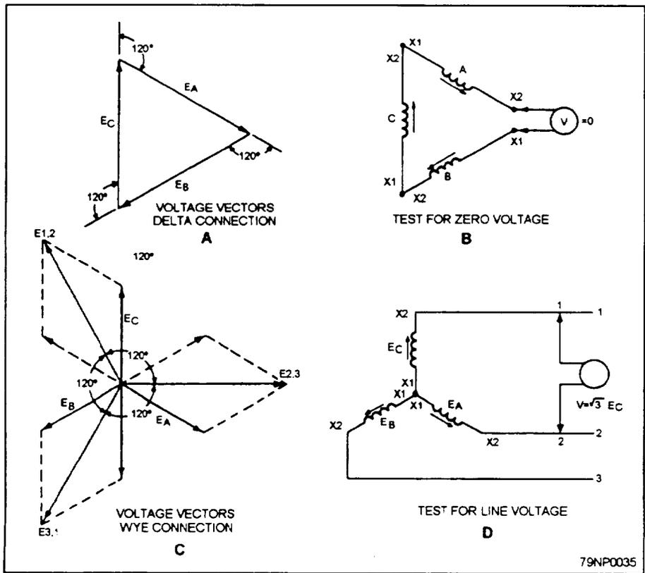
Figure 3-35.—Delta-connected transformer secondaries.
