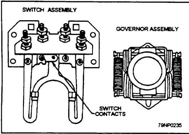
Figure 7-68.—Two major parts of a centrifugal switch.
