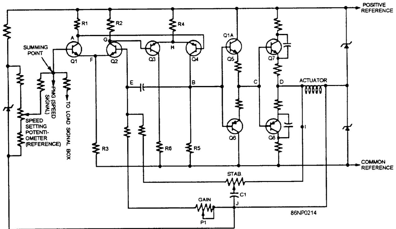
Figure 9-7.—EC-M control box, simplified schematic.
