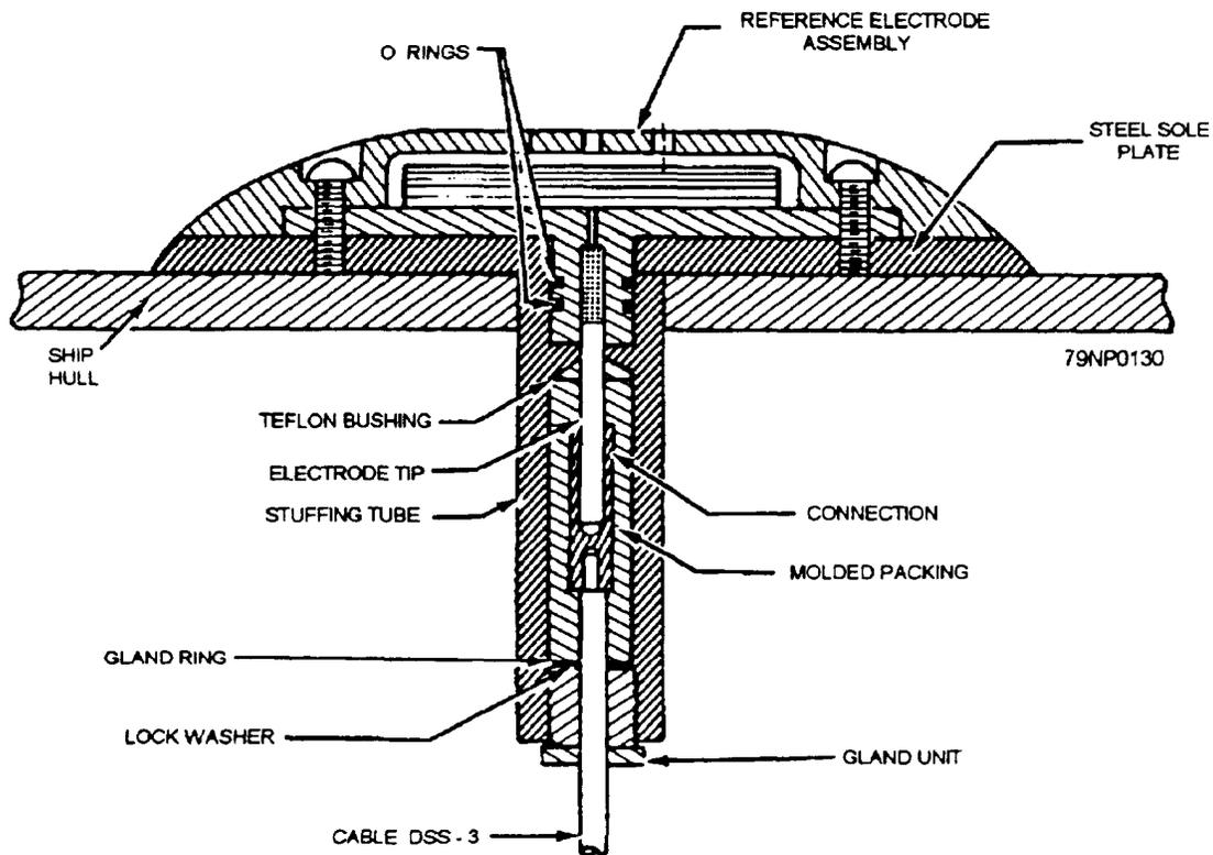
Figure 11-7.—Reference electrode assembly.
