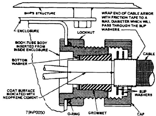
Figure 24.—Representative nylon stuffing tube installations.
