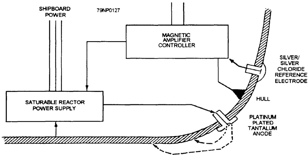
Figure 11-4.—Basic impressed current cathodic protection system.
