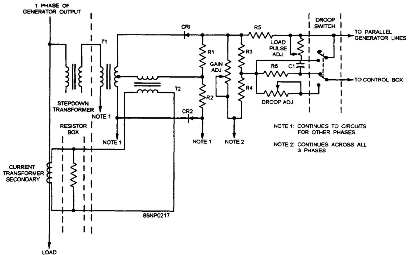
Figure 9-10.—Load signal box, simplified Schematic.
