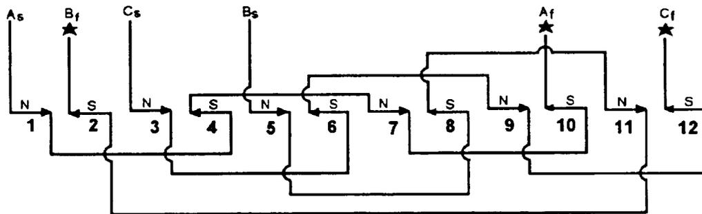
Figure 7-60.—Three-phase, four-pole, series-wye winding.
