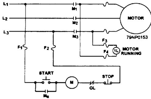
Figure 6-12.—Schematic of a simple LVP controller.
