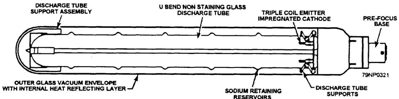
Figure 4-11.—A typical low-pressure sodium (LPS) lamp.
