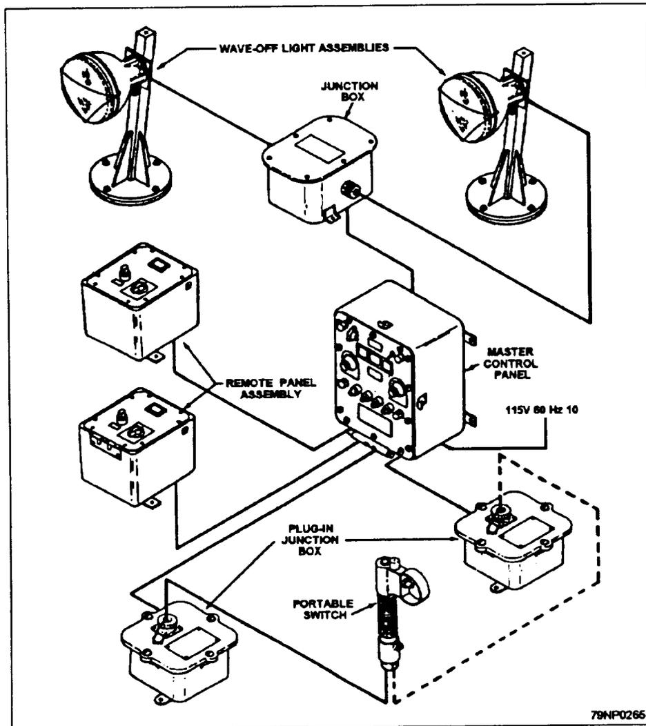
Figure 12-24.—Wave-off light system.
