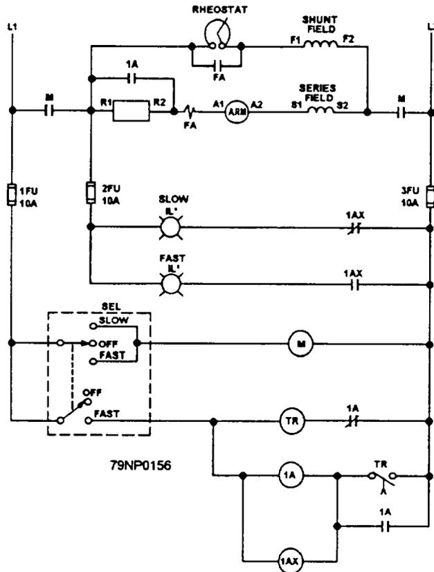
Figure 6-15.—A two-speed dc controller with shunt field rheostat.
