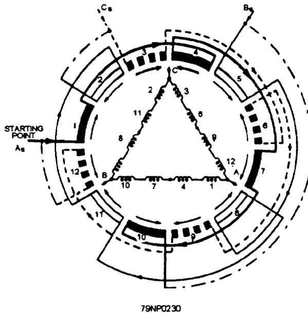
Figure 7-63.—Three-phase, four-pole, series-delta winding.
