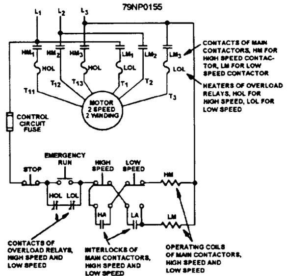
Figure 6-14.—Two-speed, ac controller.
