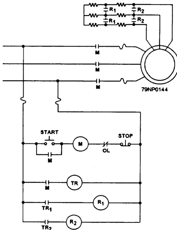
Figure 6-3.—Schematic of an ac secondary resistor controller.
