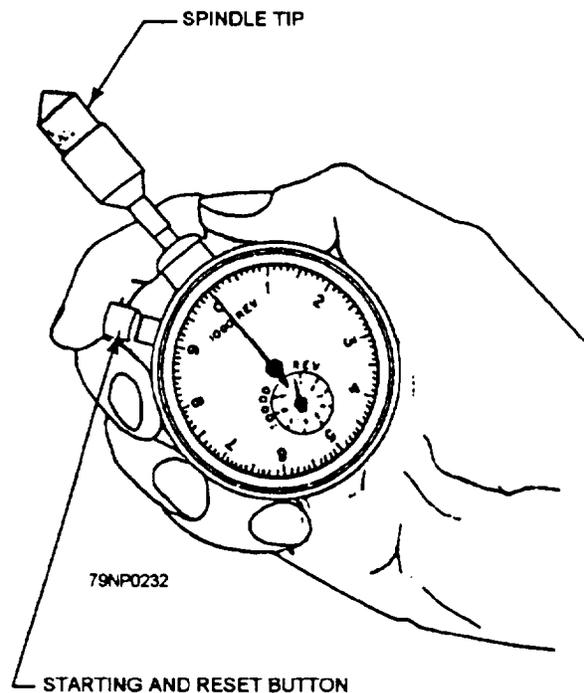
Figure 7-65—A chronometric tachometer.
