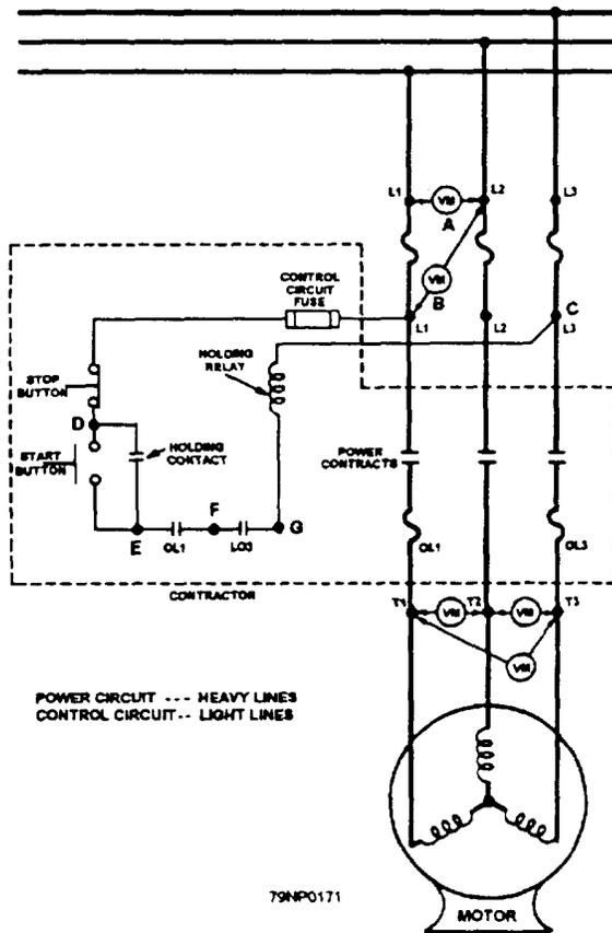
Figure 6-30.—Troubleshooting a three-phase magnetic line starter.
