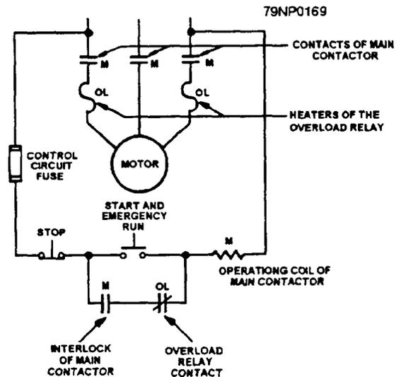
Figure 6-28.—Schematic of controller with start-emergency run push button.
