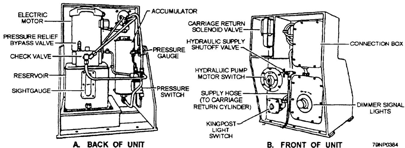
Figure 5-36.—Carriage return hydraulic power unit: A. Back of unit; B. Front of unit.
