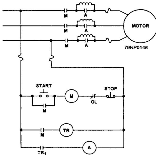
Figure 6-5.—Schematic of a reactor controller.
