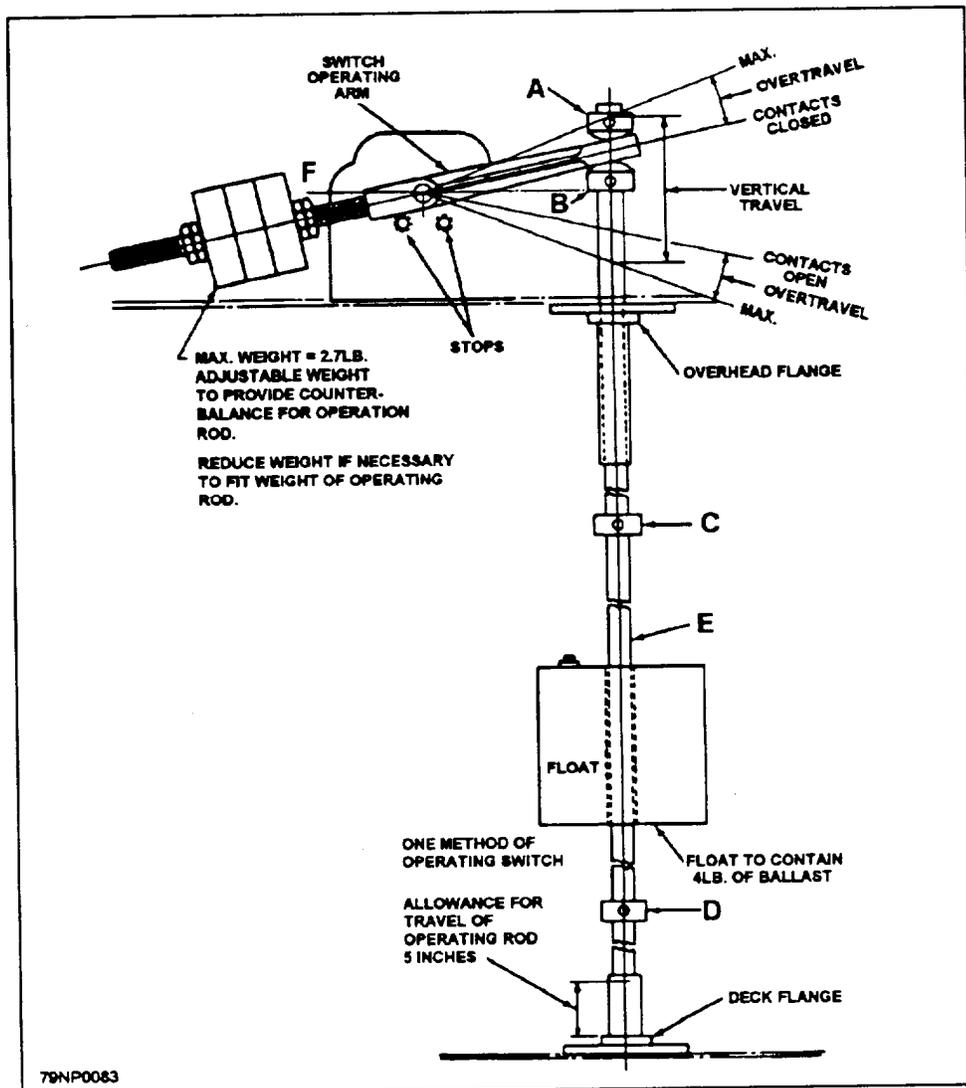
Figure 2-36.—A float switch tank installation.
