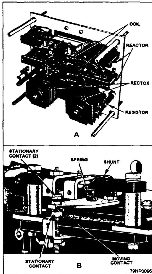
Figure 2-48.—A phase-failure relay.
