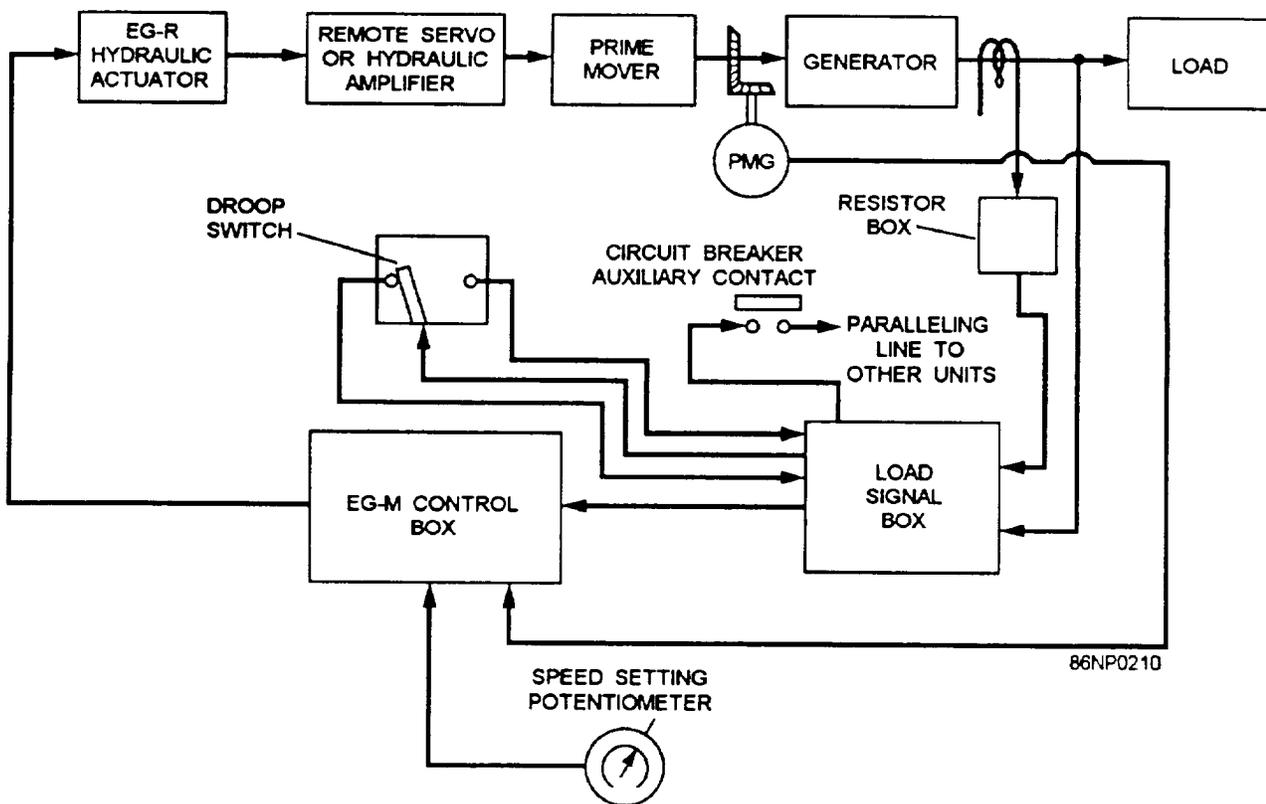
Figure 9-3.—Electrohydraulic load-sensing governor system, block diagram.
