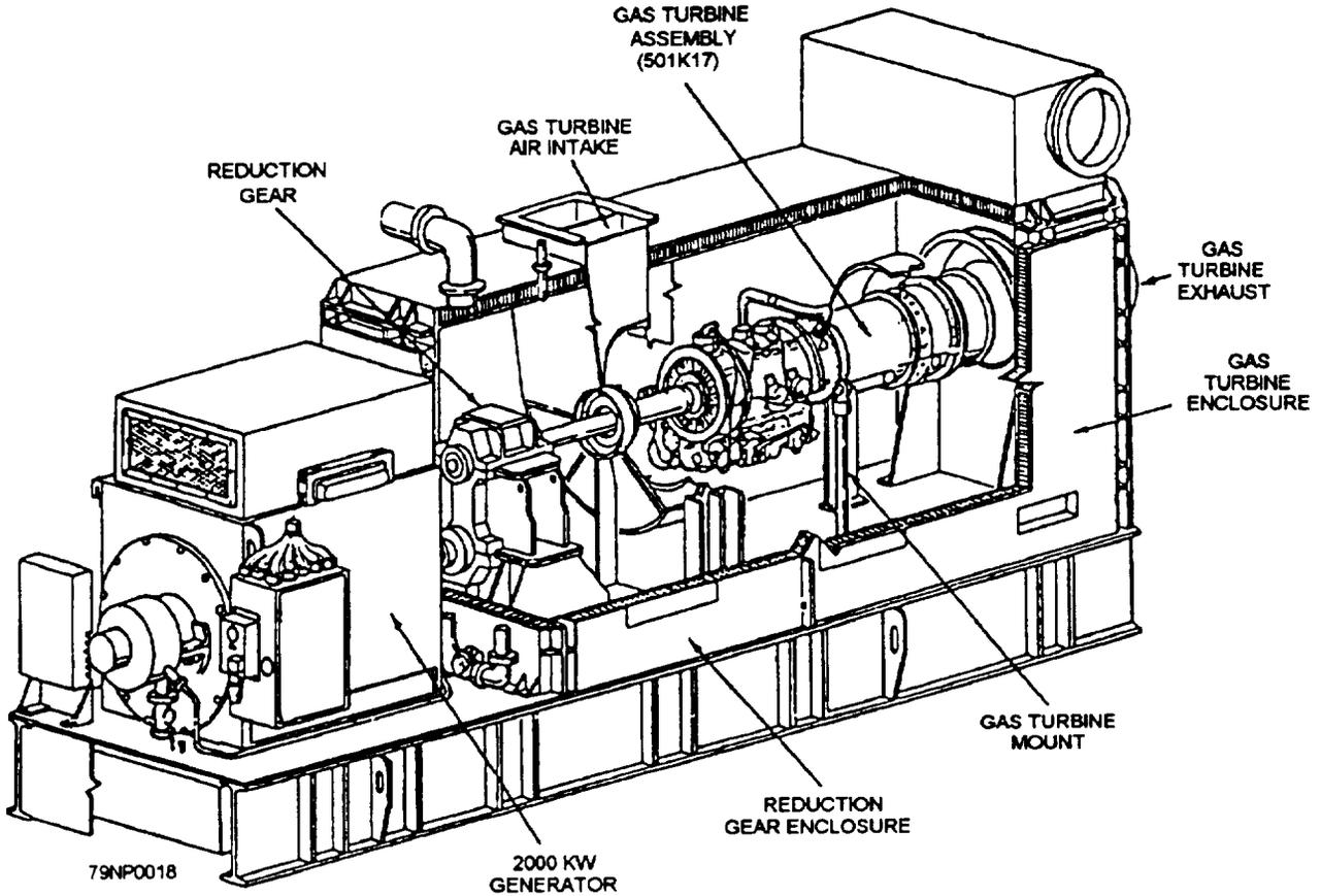
Figure 3-18.—Model 104 gas turbine generator set.
