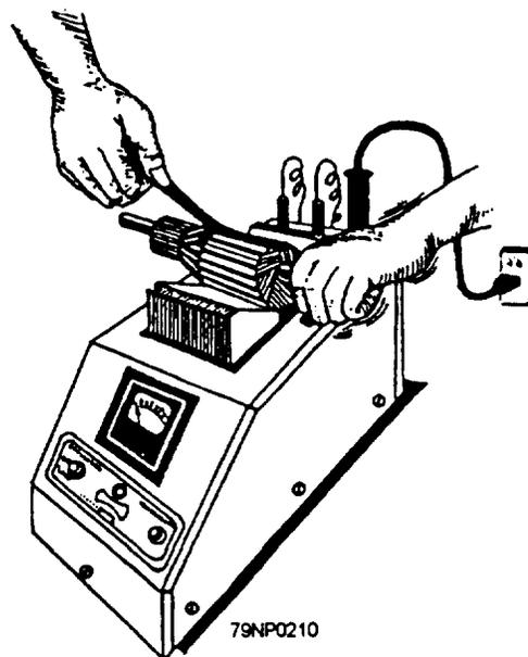
Figure 7-41.—Checking armature shorts with a growler.
