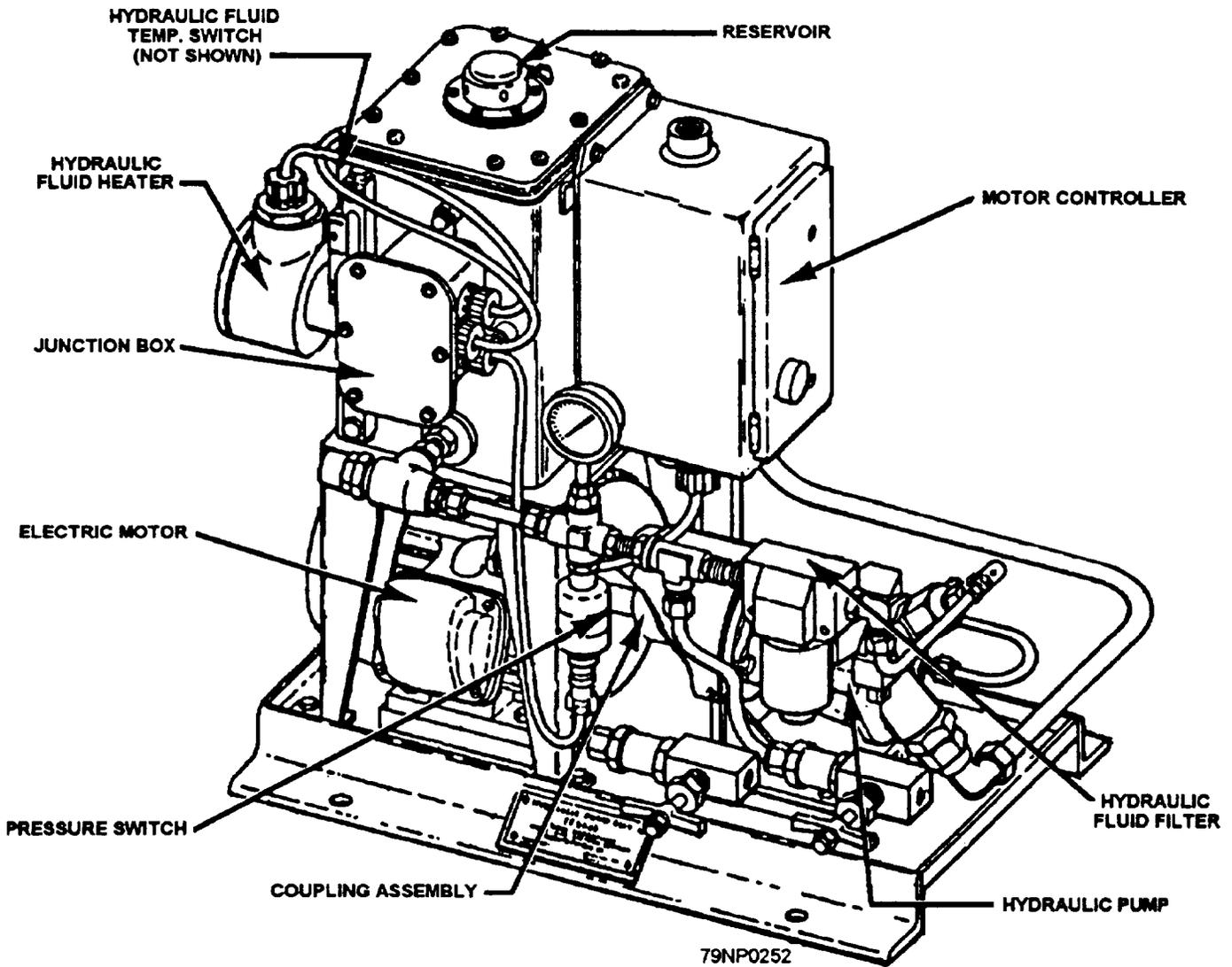
Figure 12-12.—Hydraulic pump assembly.
