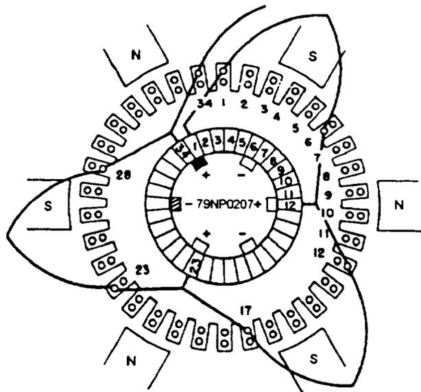
Figure 7-38.—Portion of a six-pole simplex wave winding.
