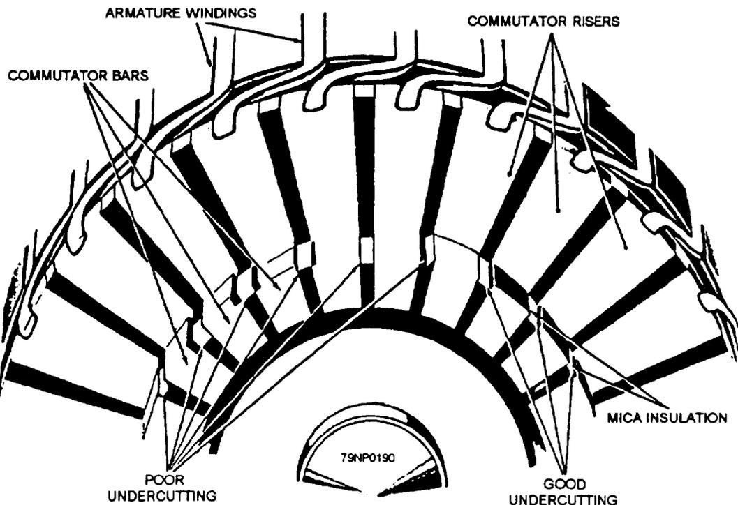
Figure 7-20.—Example of good and poor undercutting.
