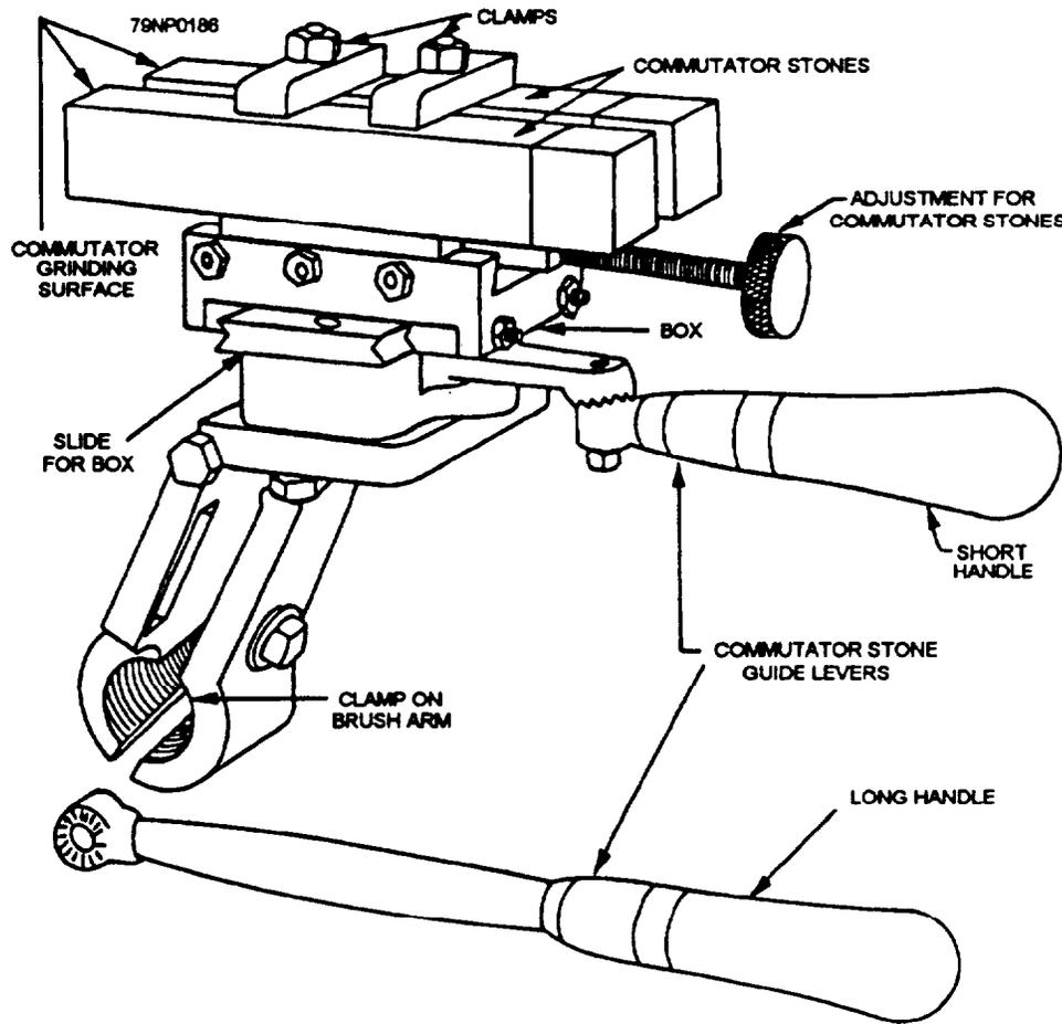
Figure 7-16.—Commutator dressing stone tool.
