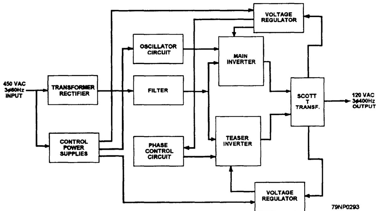
Figure 8-24.—Static converter, simplified block diagram.
