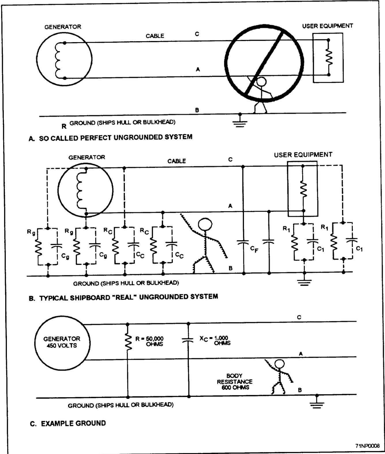
Figure 1-2.—DANGEROUS! BEWARE! Shipboard ungrounded electrical distribution systems are DEADLY.
