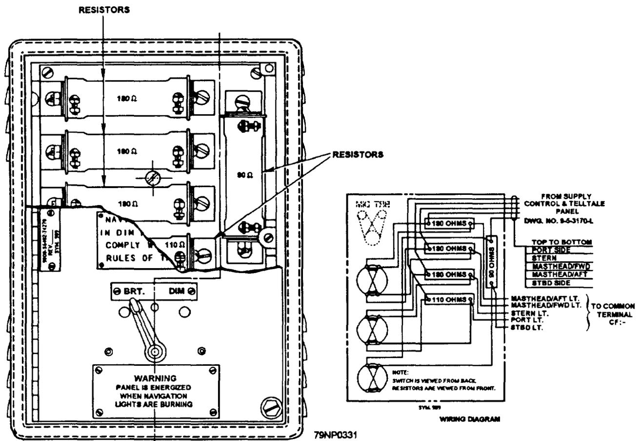
Figure 4-22.—Dimmer control panel, symbol 989.
