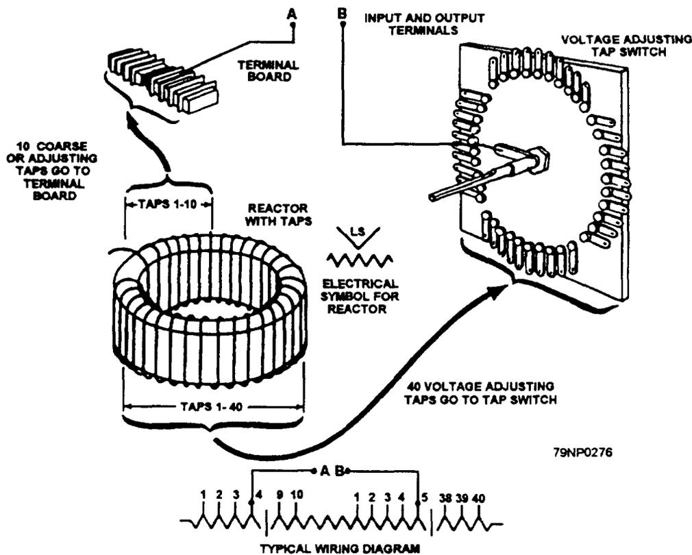
Figure 8-7.—Voltage-adjusting unit.
