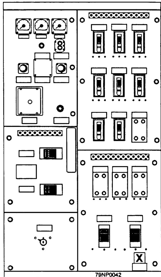
Figure 3-42.—400-hertz switchboard.
