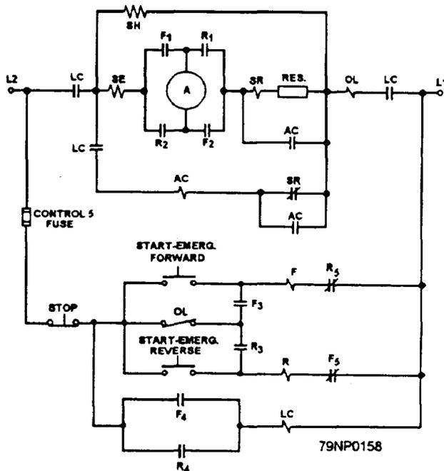
Figure 6-17.—Reversing dc controller.
