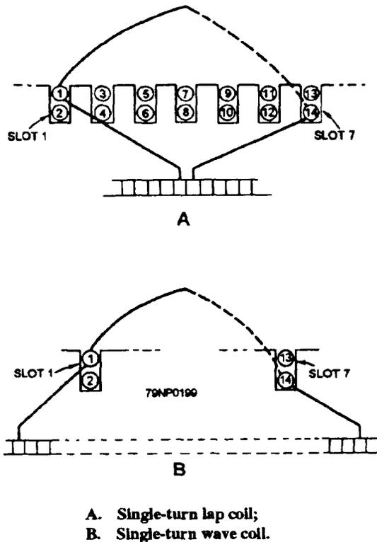
Figure 7-30.—Classification of armature windings.
