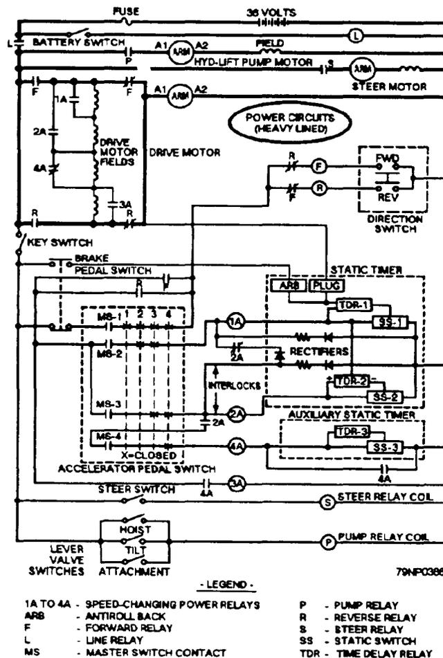
Figure 5-38.—Wiring diagram of an electric forklift.
