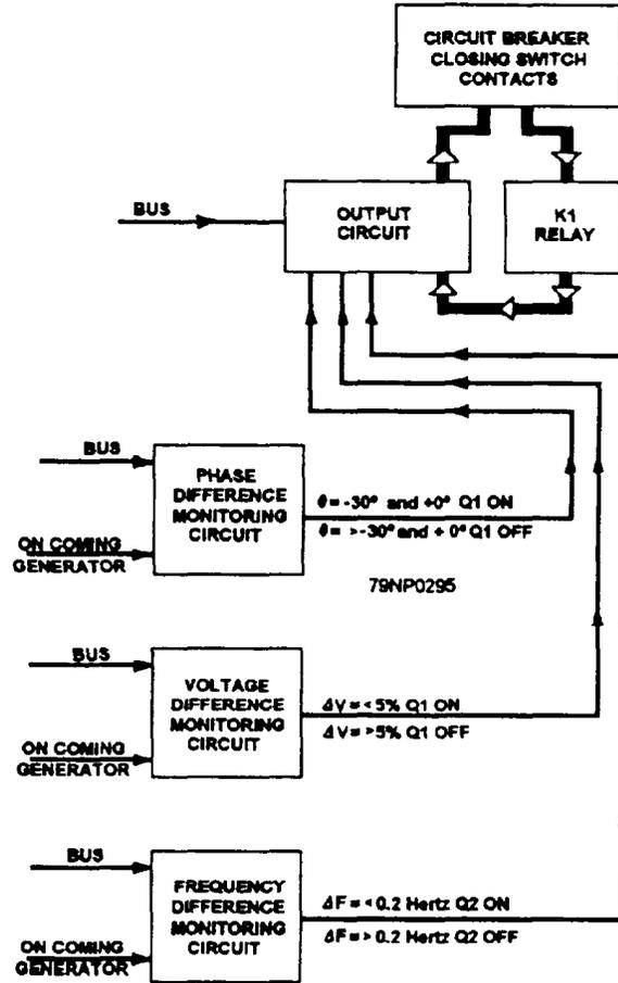
Figure 8-26.—Block diagram of synchronizing monitor.
