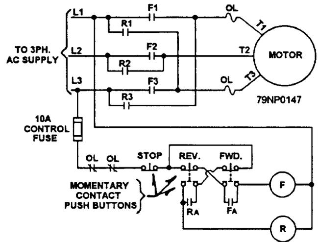
Figure 6-6.—Schematic of a reversing ac controller.
