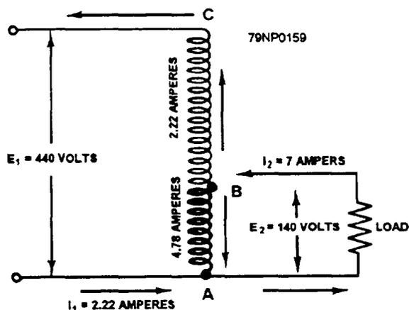
Figure 6-18.—Single-phase autotransformer.
