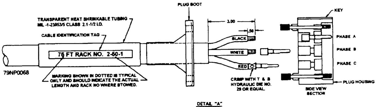
Figure 2-21.—New method of preparing casualty power cable ends.
