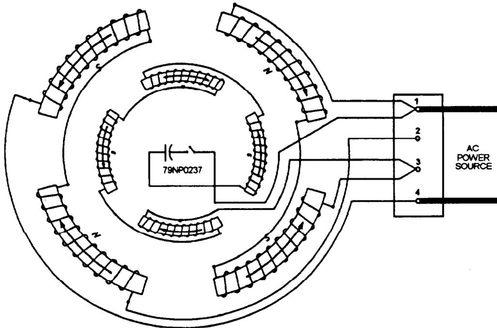
Figure 7-70.—Single-phase, capacitor-start, inductor-run motor diagram.
