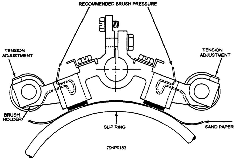
Figure 7-13.—Detail of brush rigging with sandpaper in position.
