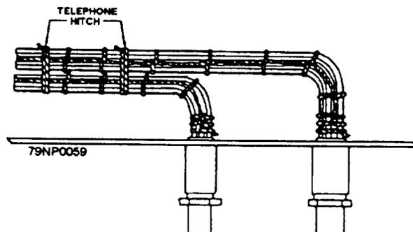
Figure 2-12.—Binding cable groups with the telephone hitch.
