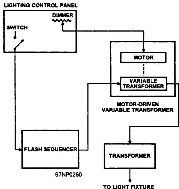
Figure 12-19.—Simplified interconnection of line-up lights.
