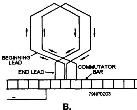
Figure 7-34.—Simplex lap windings.
