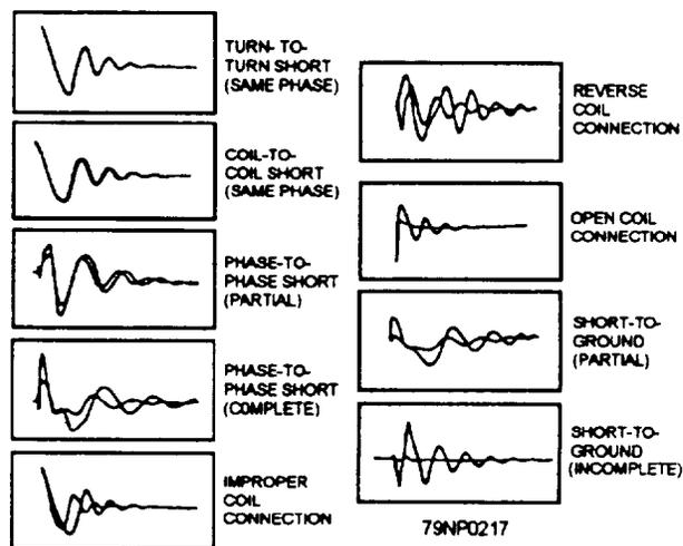
Figure 7-48.—Representative surge test waveforms.
