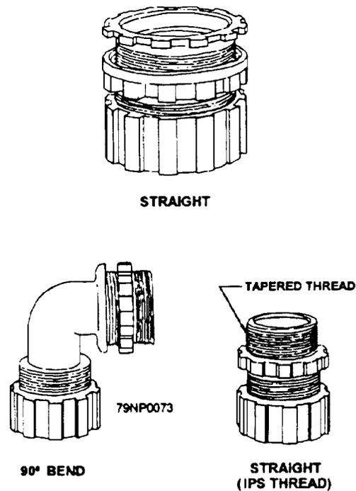
Figure 2-26.—Nylon Stuffing tubes.
