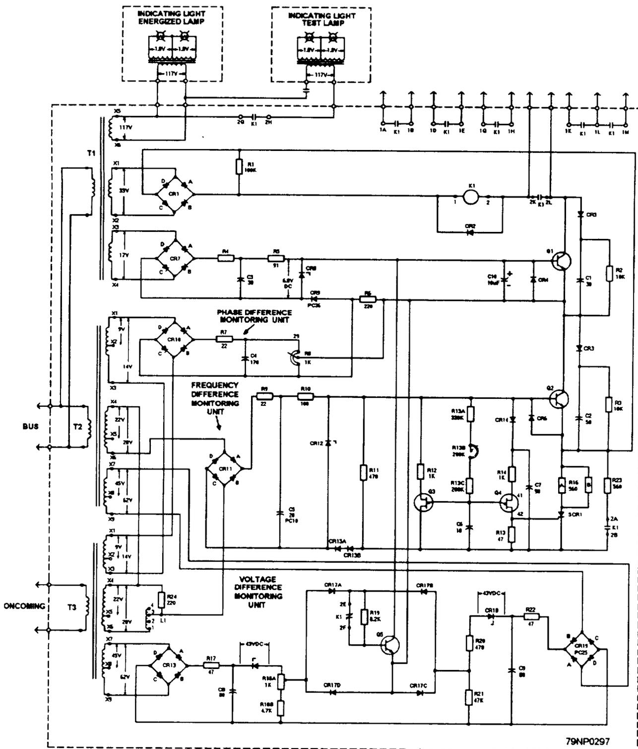
Figure 8-28.—Synchronizing monitor.
