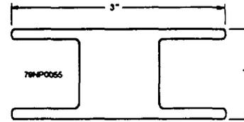
Figure 2-8.—A lacing shuttle.
