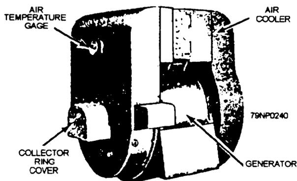
Figure 7-73.—Generator equipped with an air cooler.
