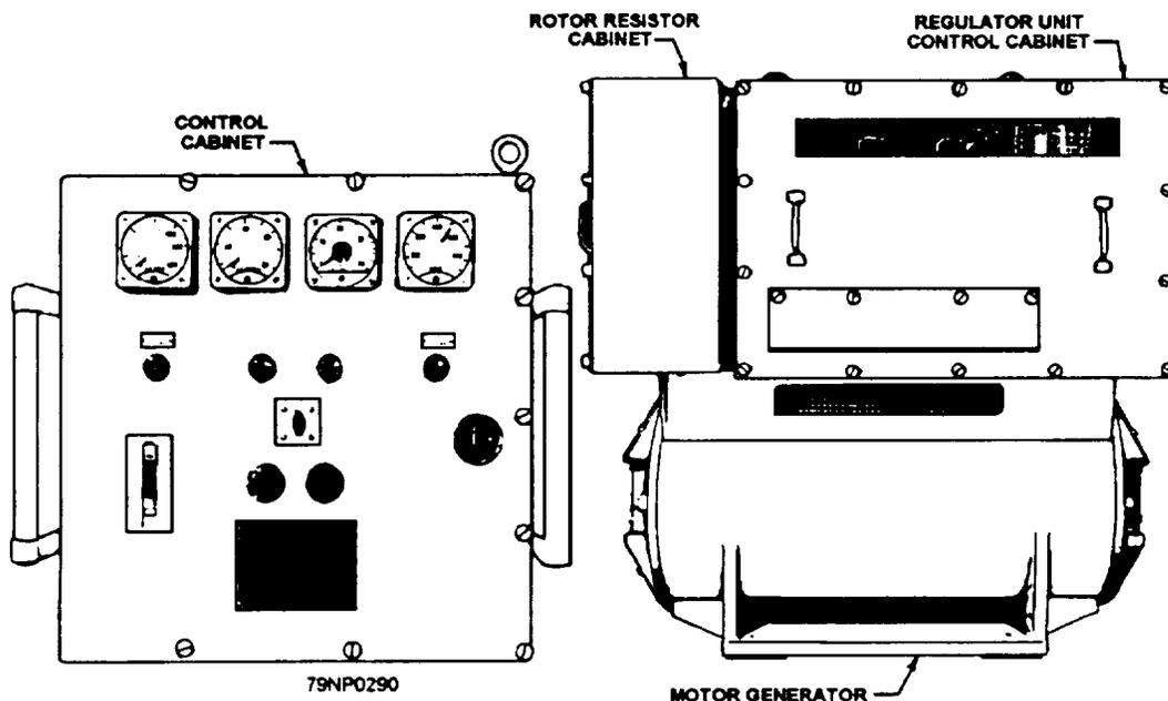
Figure 8-21.—Motor-generator set with control equipment.
