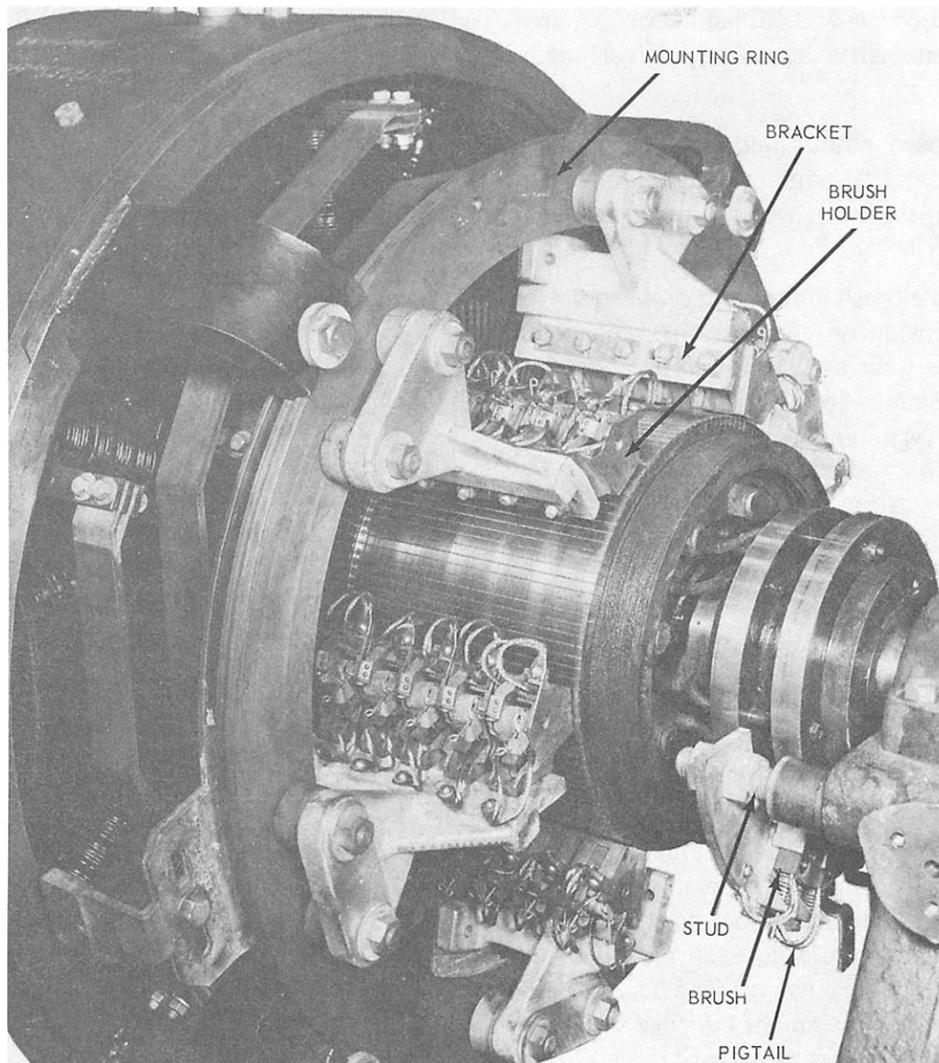
**Figure 7-10.—Brush holder and brush rigging assembly.**
