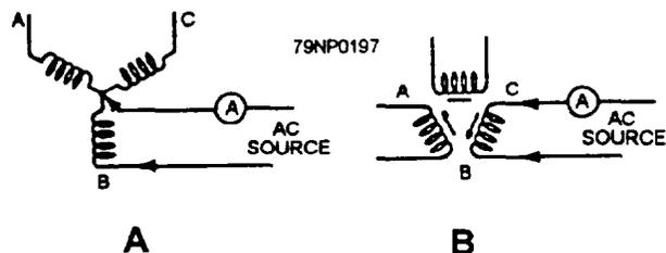
Figure 7-28.—Balanced current test for shorted phase.
