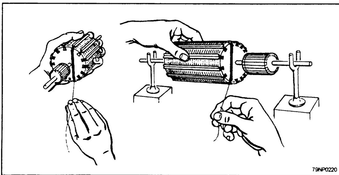
Figure 7-52.—Winding armatures by hand.
