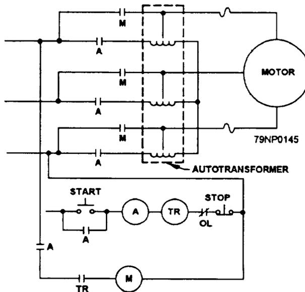
Figure 6-4.—Schematic of an autotransformer controller.
