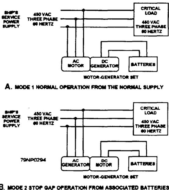
Figure 8-25.—No-break power supply, block diagram.
