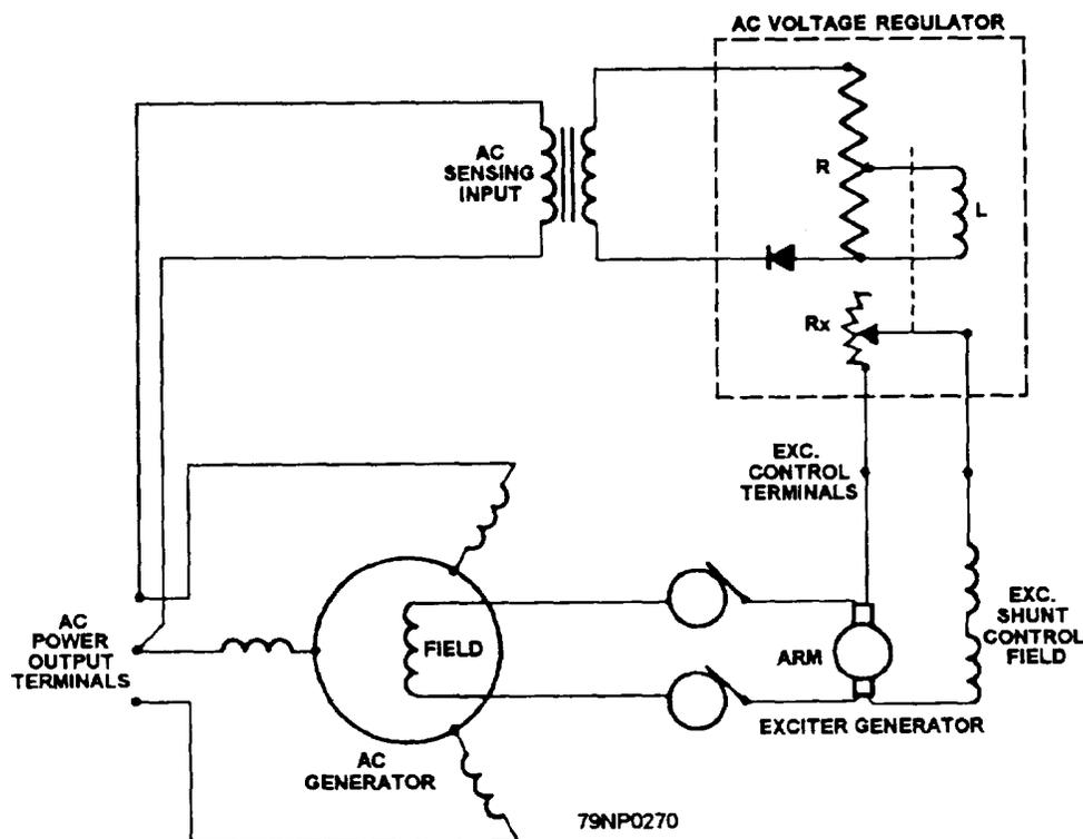
Figure 8-1.—Simplified voltage regulator circuit.
