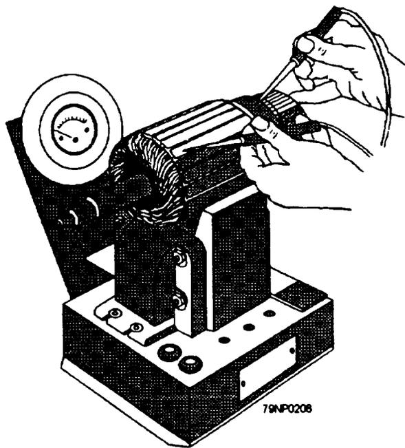
Figure 7-39.—Testing an armature for grounds.
