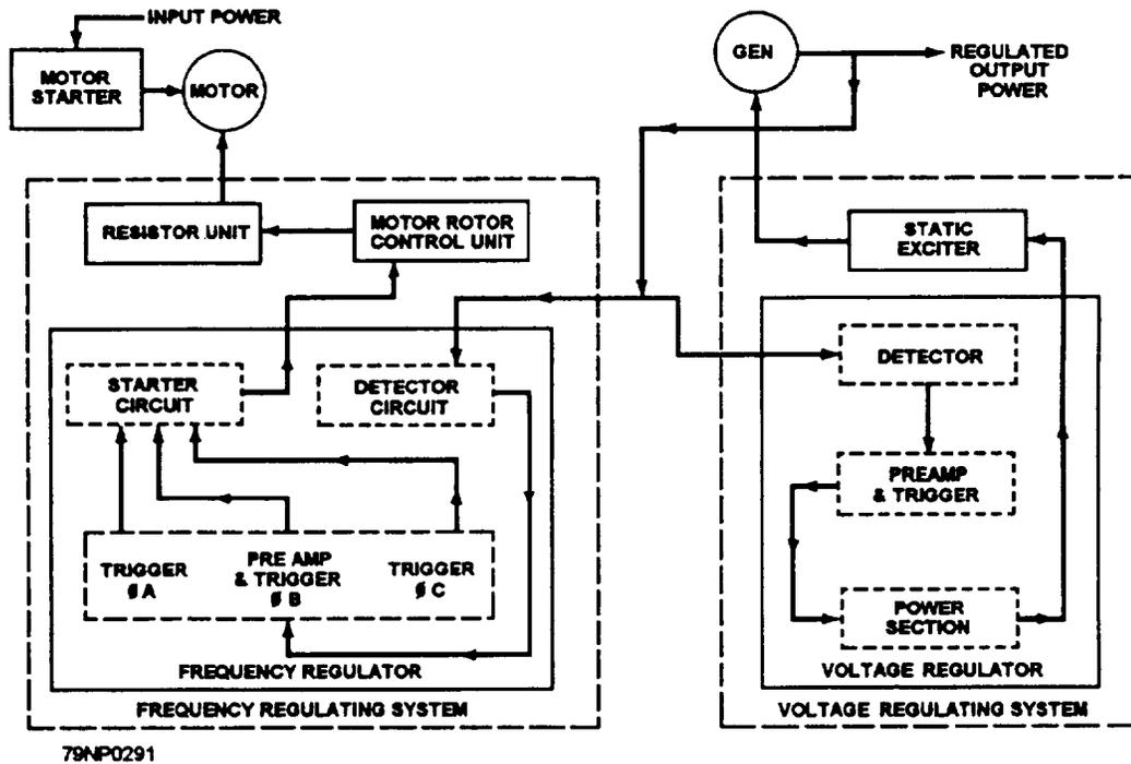
Figure 8-22.—Motor-generator set simplified block diagram.
