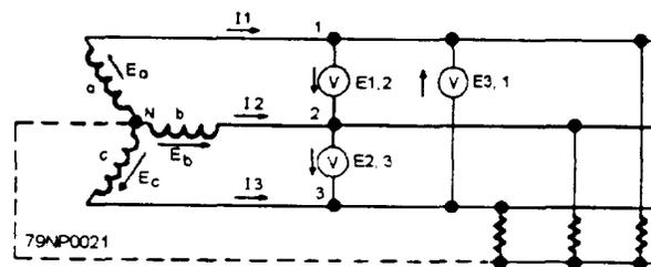
Figure 3-21.—Three-phase, ac generator showing neutral connection.
