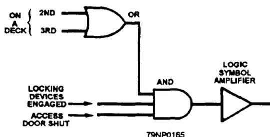
Figure 6-24.—Basic logic circuit.
