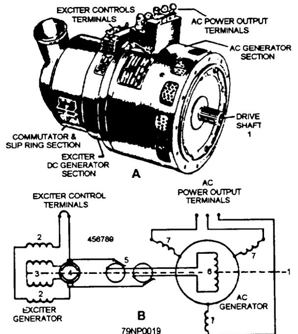
Figure 3-19.—An ac generator and schematic.
