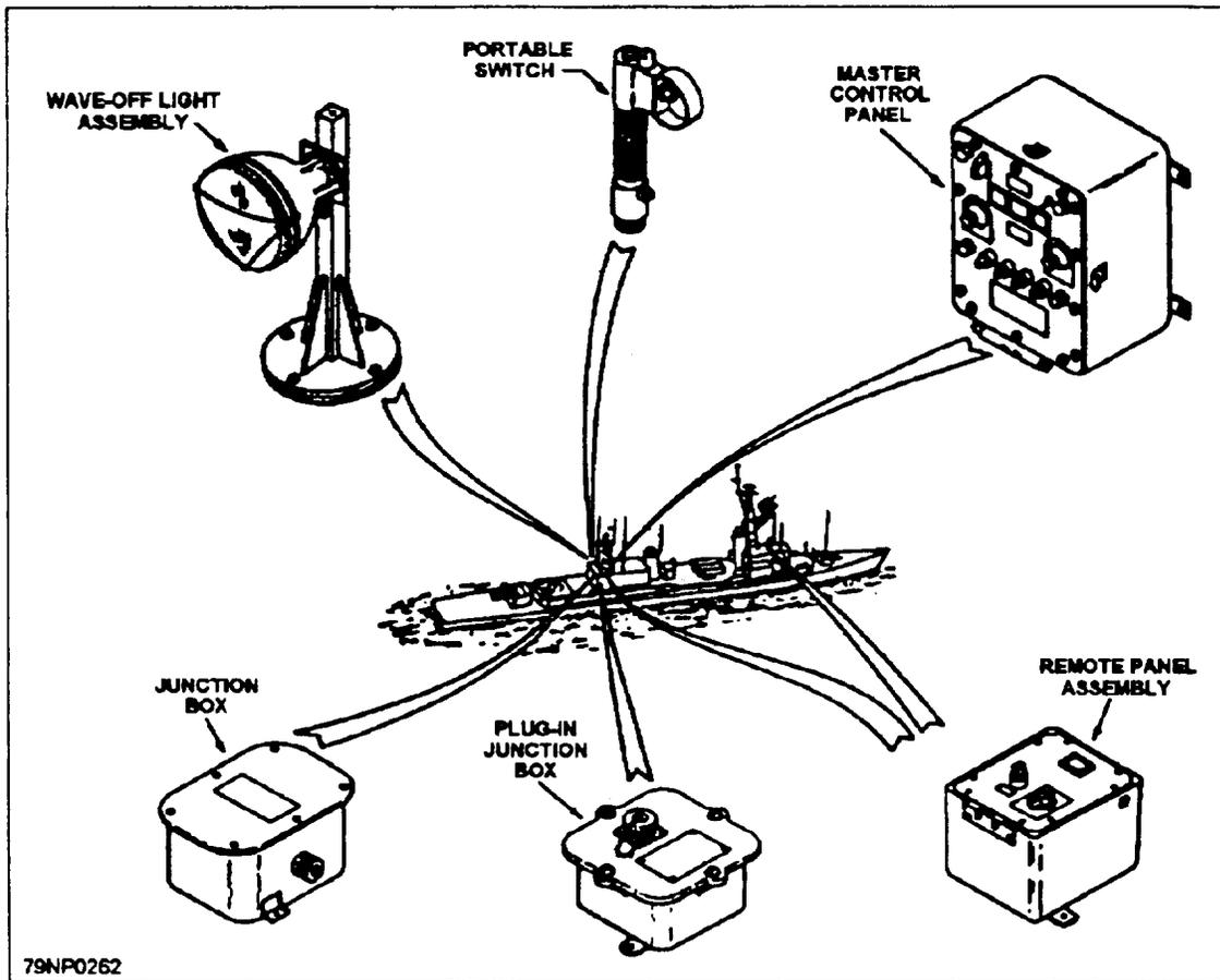
Figure 12-21.—Wave-off light system.
