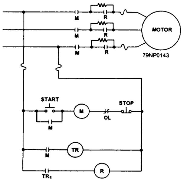
Figure 6-2.—Schematic of an ac primary resistor controller.
