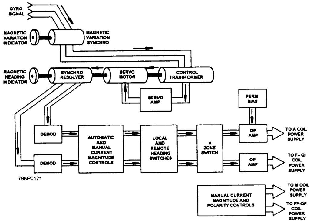
Figure 10-15.—Block diagram for an SSM degaussing switchboard.
