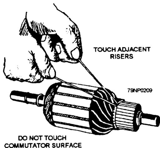
Figure 7-40.—Testing armature coils for an open circuit.
