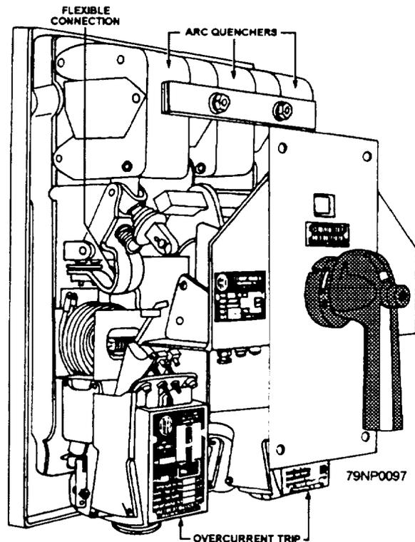
Figure 2-50.—Type ACB circuit breaker.
