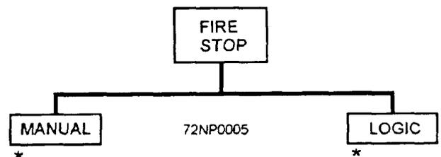
\* IF BATTLE OVERRIDE IS ON, LOGIC WILL NOT ALLOW THE FIRE STOP SEQUENCE TO STOP THE ENGINE.
