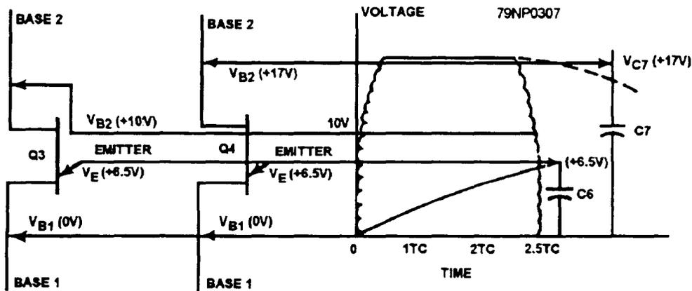
Figure 8-38.—Firing sequence for Q3.
