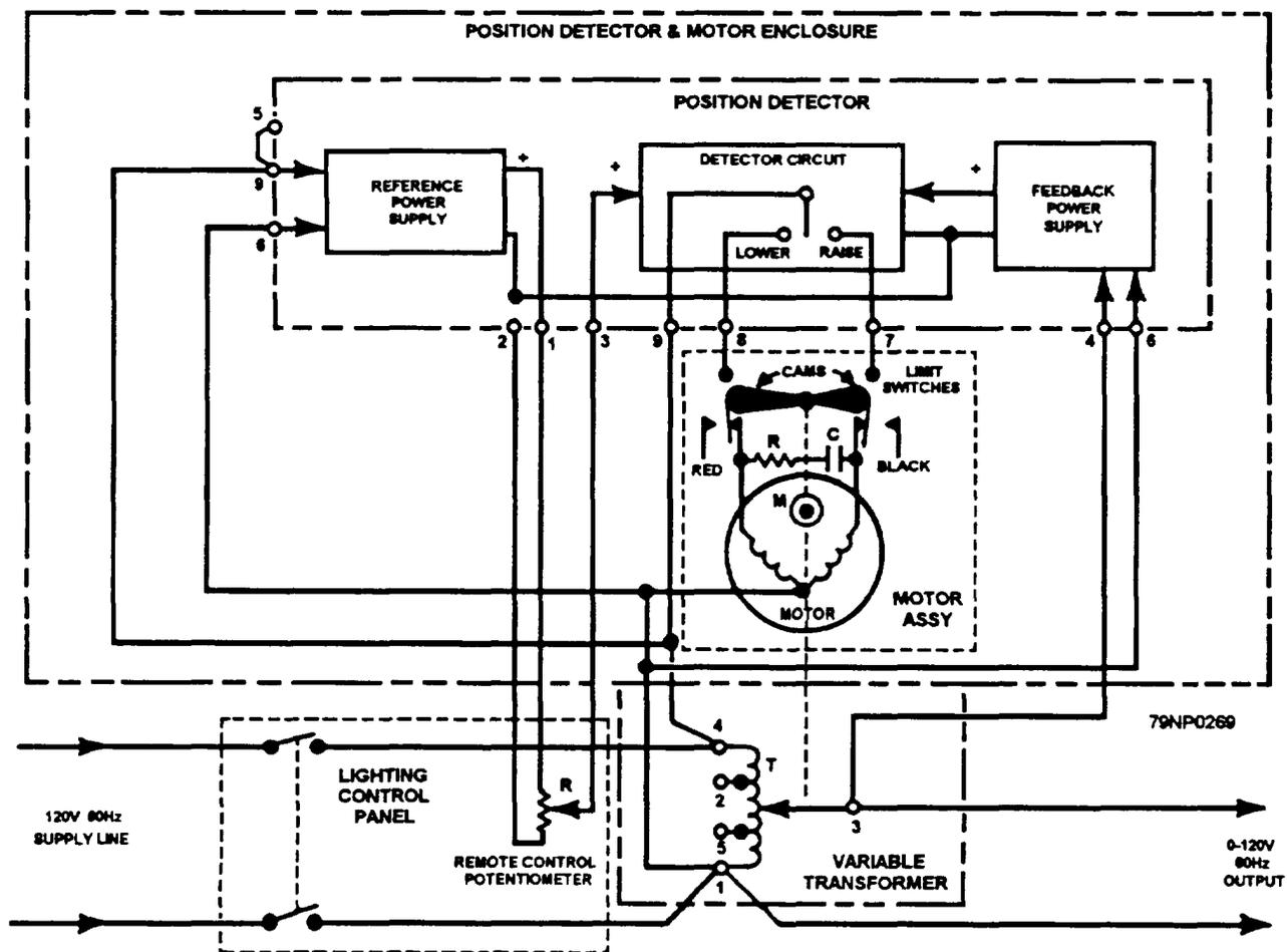
Figure 12-28.—Motor-driven remote variable transformer circuit diagram.
