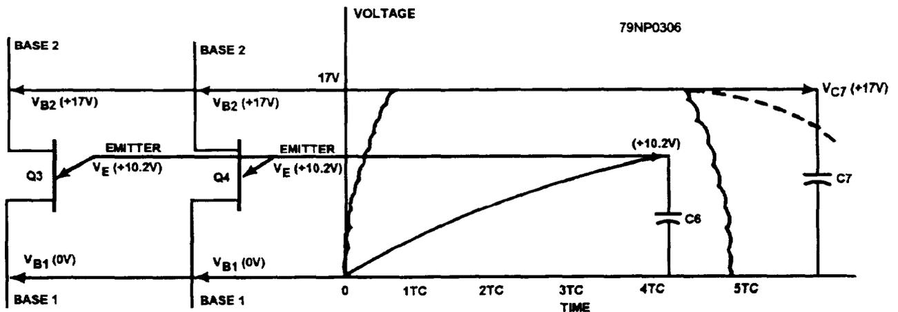
Figure 8-37.—Firing sequence for Q4.
