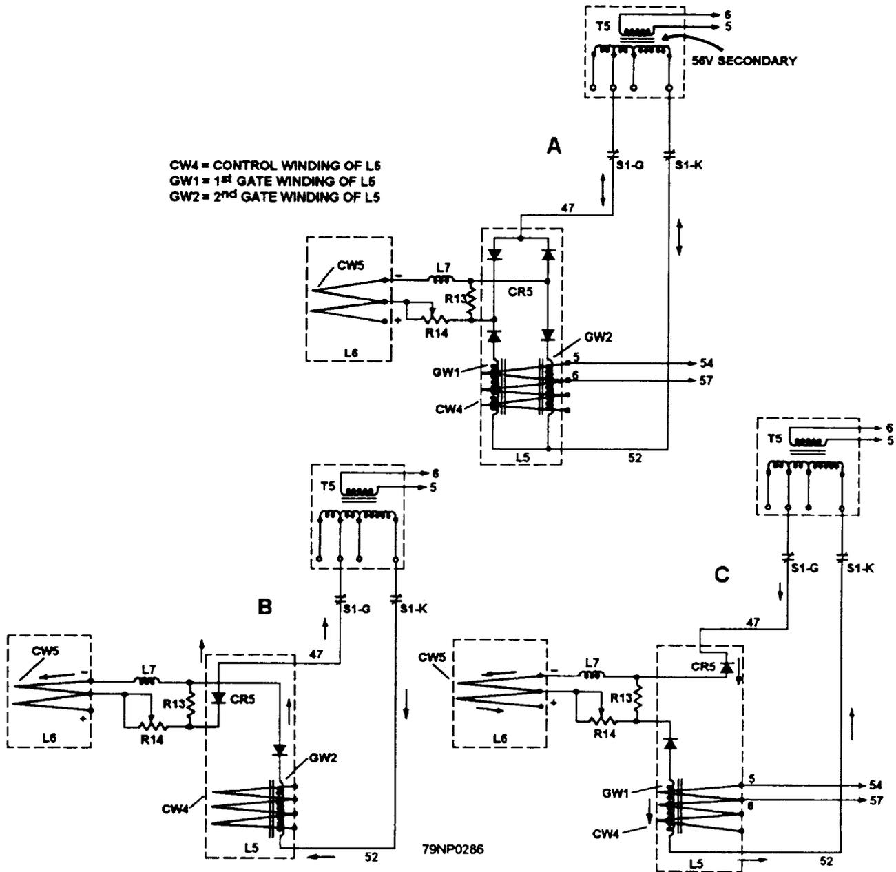
Figure 8-17.—First-stage magnetic amplifier.
