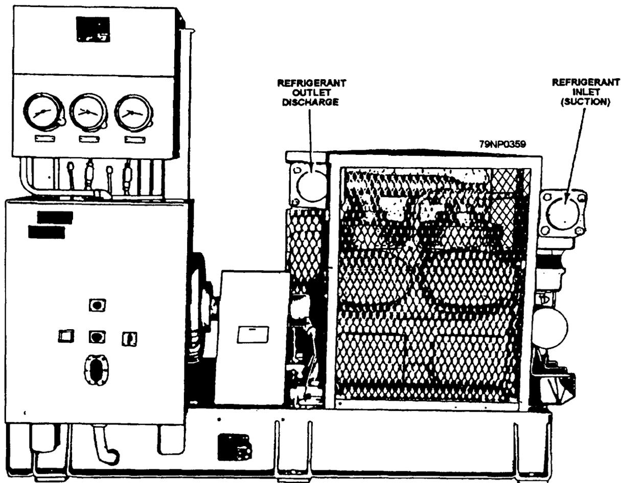
Figure 5-11.—80-ton compressor unit assembly.
