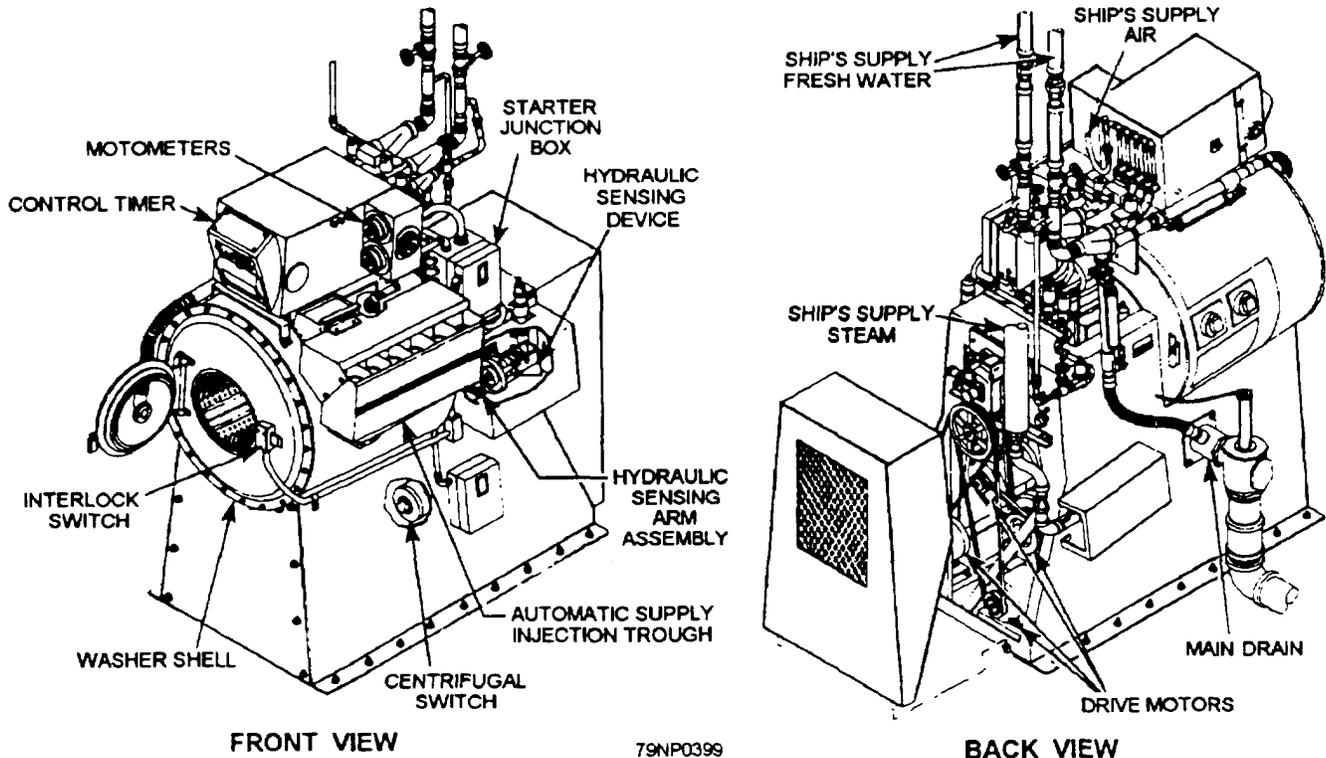
Figure 5-51.—A typical washer-extractor installation.
