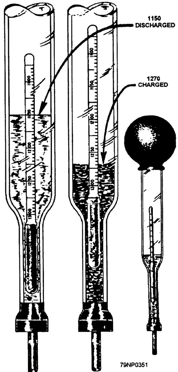
Figure 5-2.—Type-B hydrometer.
