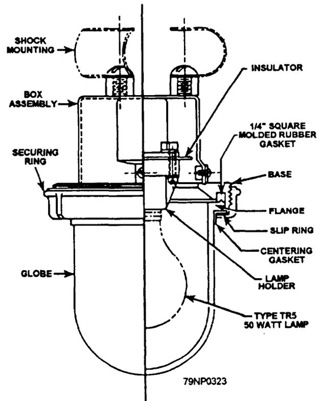
Figure 4-14.—A symbol 92.2 watertight fixture.
