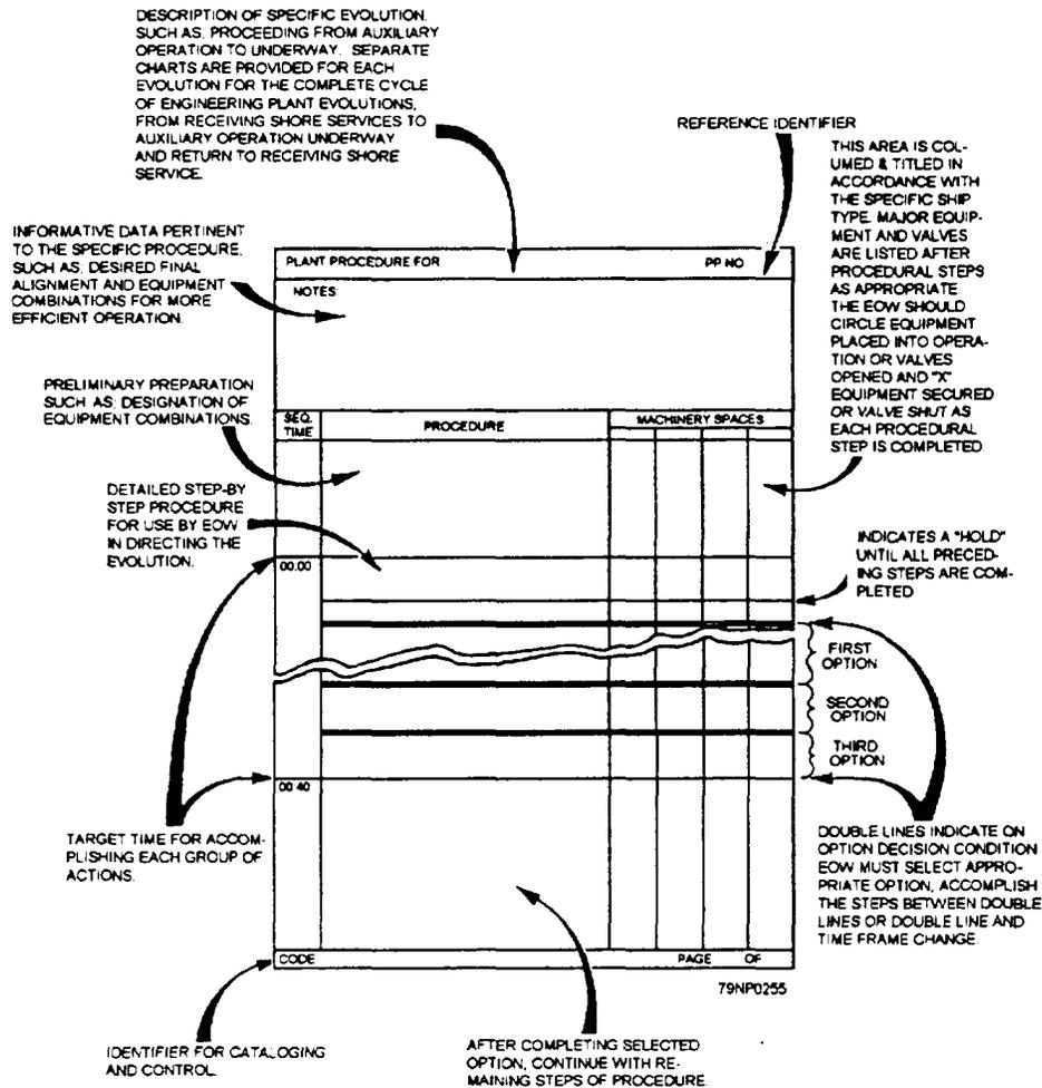
Figure 14-1. Sample plant procedure chart.
