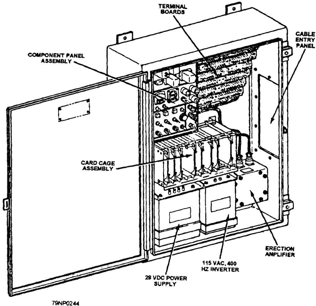
Figure 12-4.—Electronic enclosure assembly.
