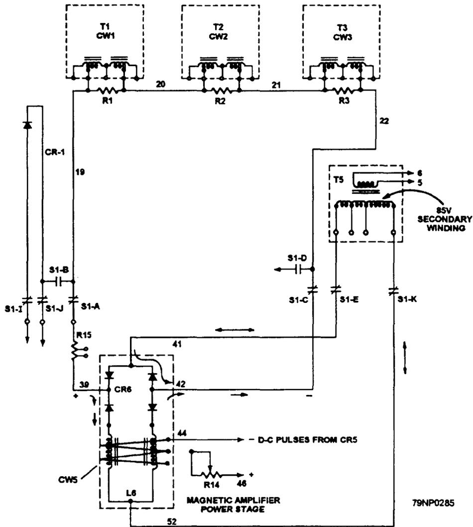
Figure 8-16.—Final-stage magnetic amplifier.
