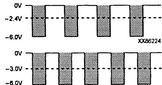
NOTE: BASIC ENVELOPE DEVELOPED ACROSS A4A1R1. DASHED LINE INDICATES AVERAGE FILTERED DC VOLTAGE OUTPUT. SHADED AREA EMPHASIZES EQUAL AREA PULSES.
