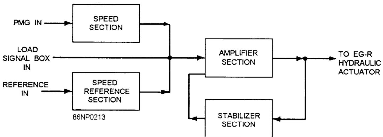
Figure 9-6.—EG-M control box, block diagram.
