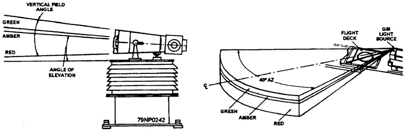
Figure 12-2.—Glide slope indicator and light beam.
