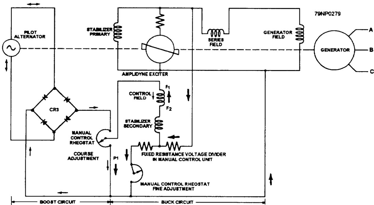
Figure 8-10.—Manual control circuit.
