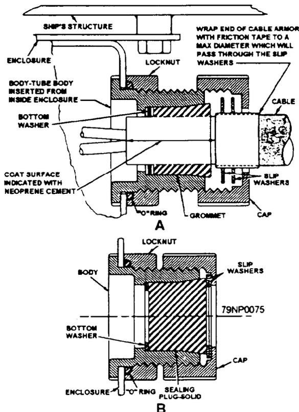
Figure 2-28.—Representative nylon stuffing tube installations.
