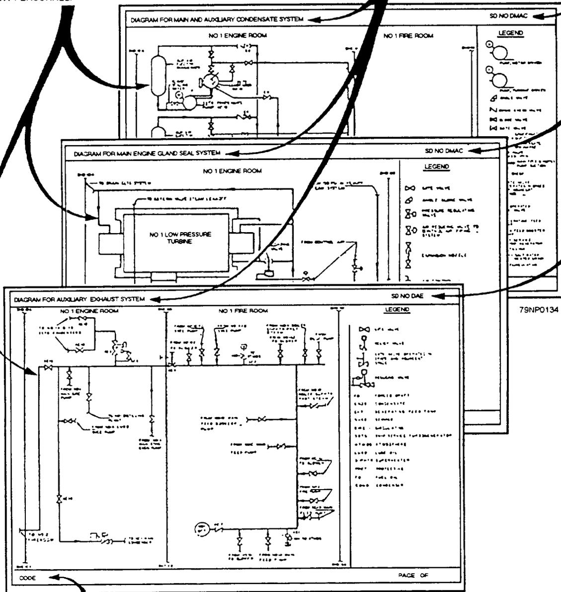
ALPHA/NUMERIC IDENTIFICATION CODES ARE NOTED ON EACH DIAGRAM TO FACILITATE CATALOGING AND CONTROL
