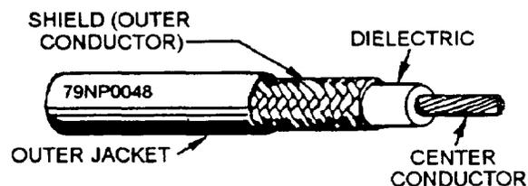
Figure 2-2—Construction of flexible RF transmission line.
