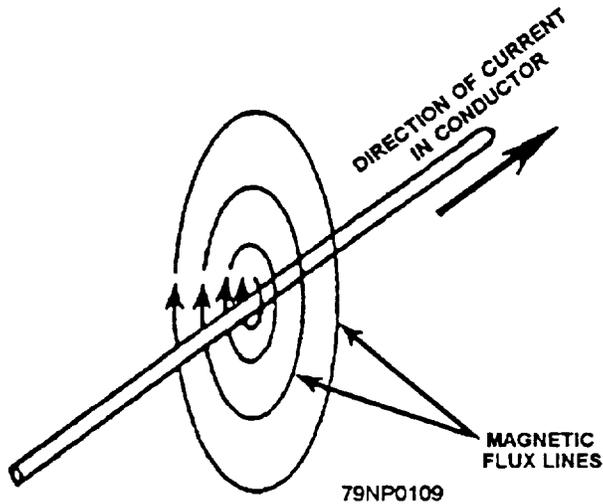
Figure 10-3.—Magnetic field around a current-carrying conductor.
