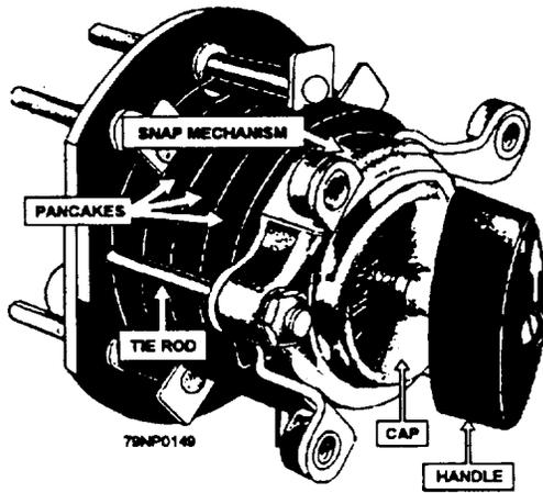
Figure 6-8.—Rotary snap switch.
