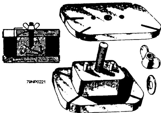
Figure 7-53.—Coil form for field coils.
