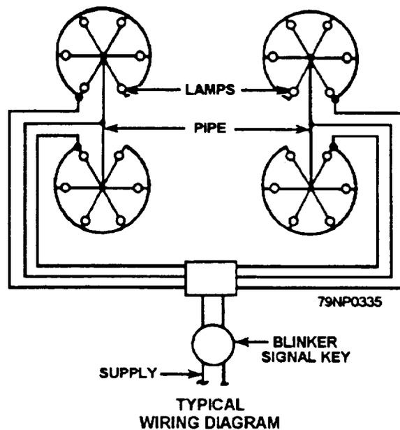
Figure 4-26.—Blinker light fixture.
