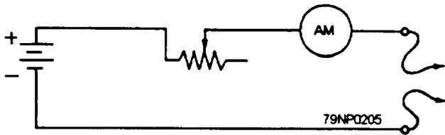
Figure 7-36.—Test circuit for measuring armature resistance.
