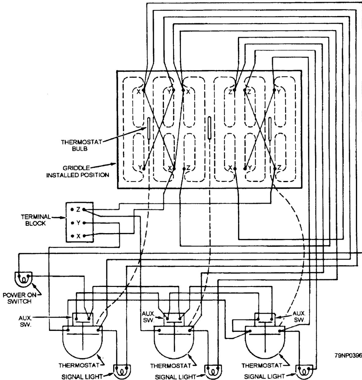
Figure 5-48.—Electric griddle wiring diagram.
