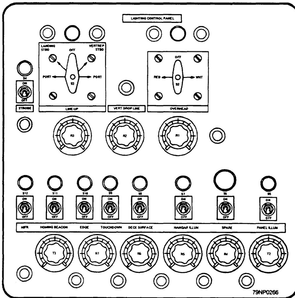
Figure 12-25.—Lighting control panel.
