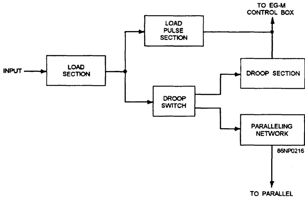
Figure 9-9.—Load signal box, block diagram.
