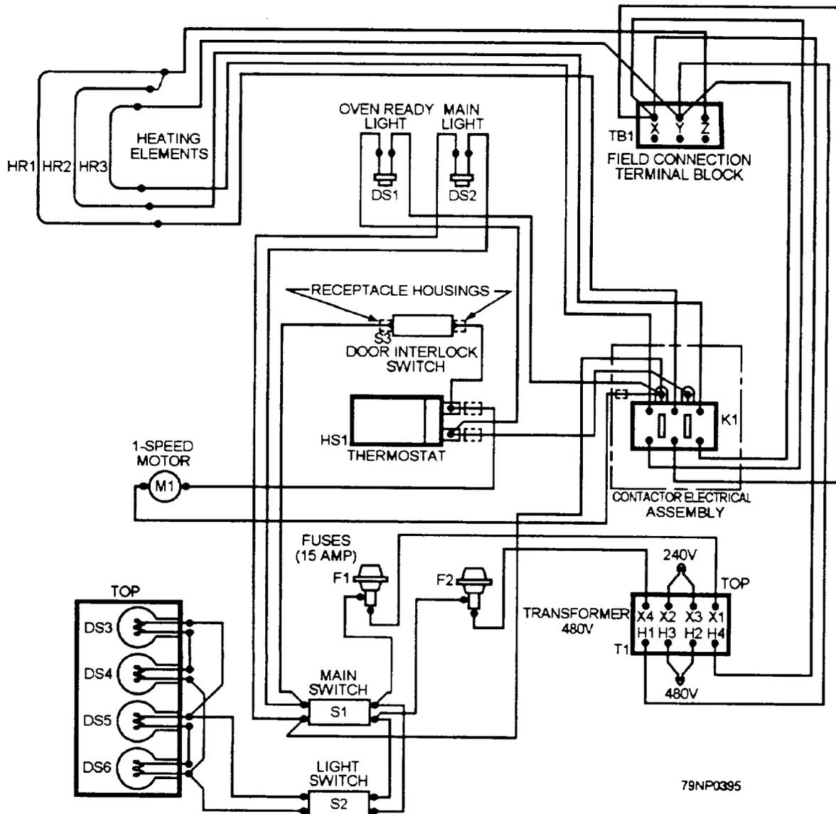
Figure 5-46.—Wiring diagram of M-series oven.
