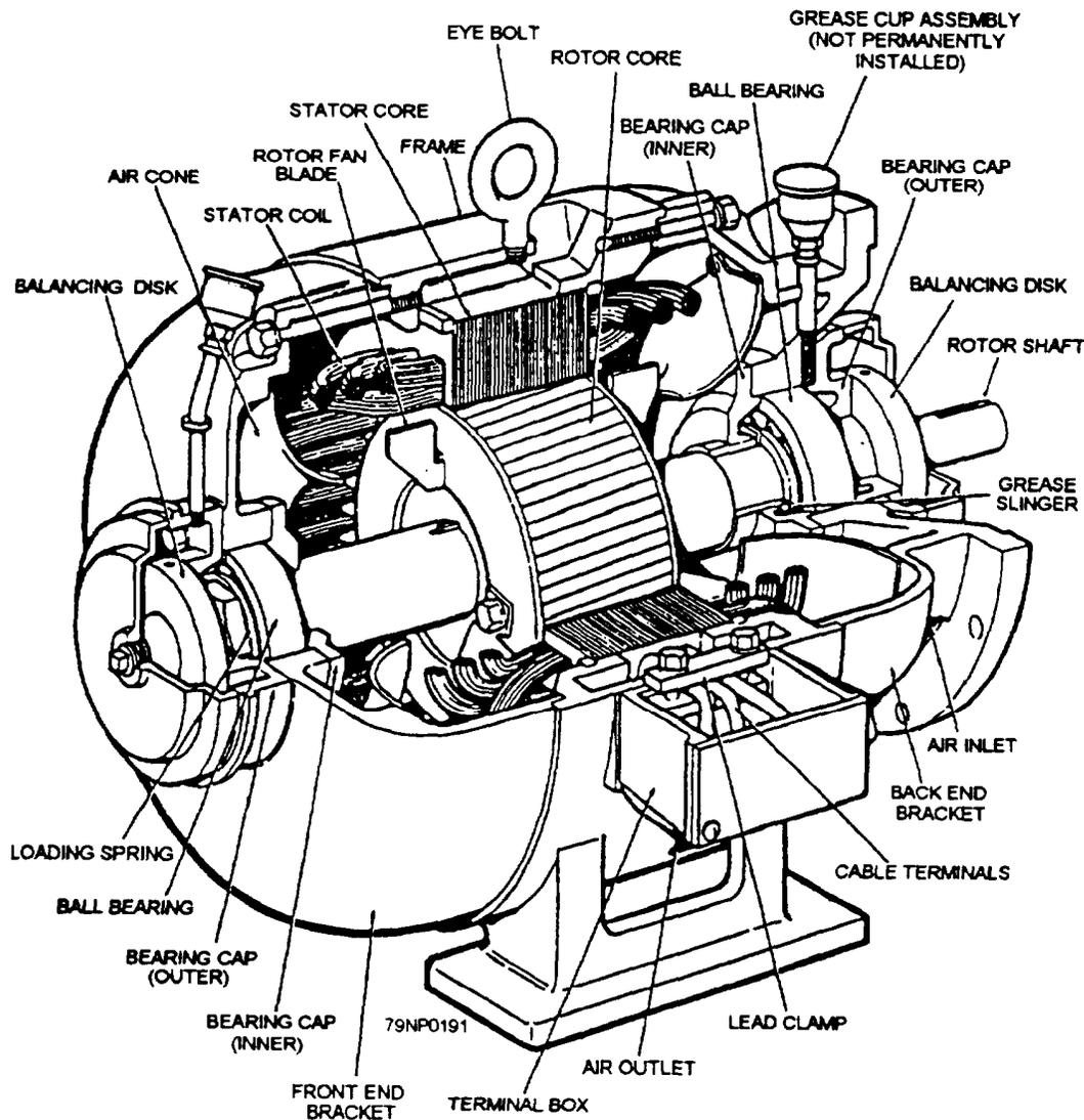
Figure 7-21.—Typical ac motor.
