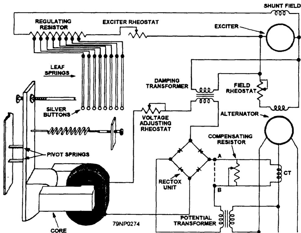
Figure 8-5.—A Silverstat voltage regulator on an ac generator.
