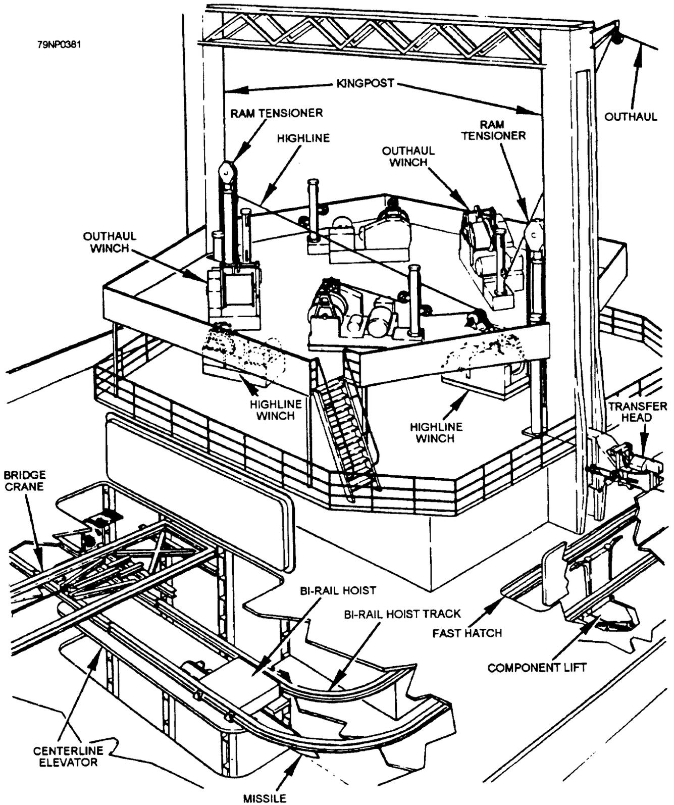
Figure 5-33.—Top view of AE UNREP system (view looking aft).
