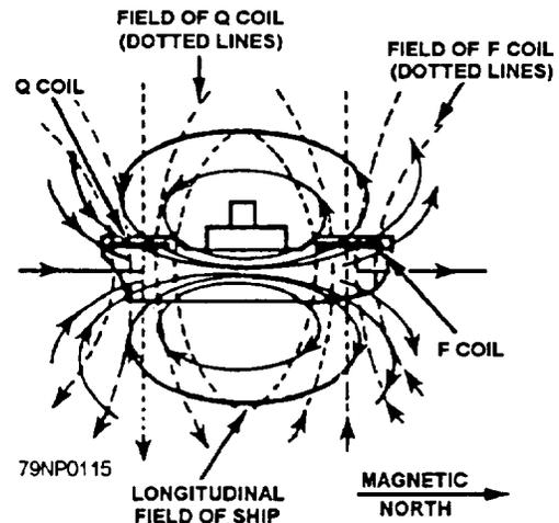
Figure 10-9.—Longitudinal field of ship and neutralizing fields of F and Q coils.
