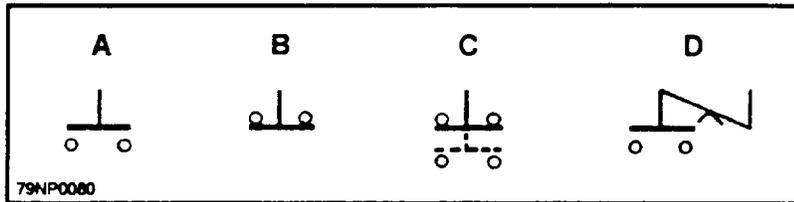
Figure 2-33.—Manually operated contacts.
