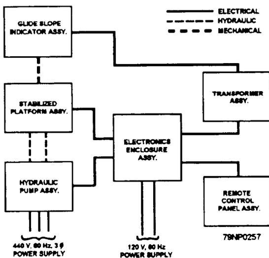
Figure 12-16.—Stabilized glide slope indicator—block diagram.
