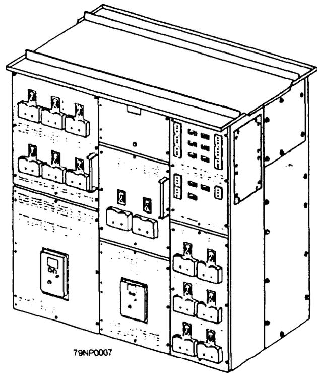
Figure 3-7.—1SA Ship's service switchboard.
