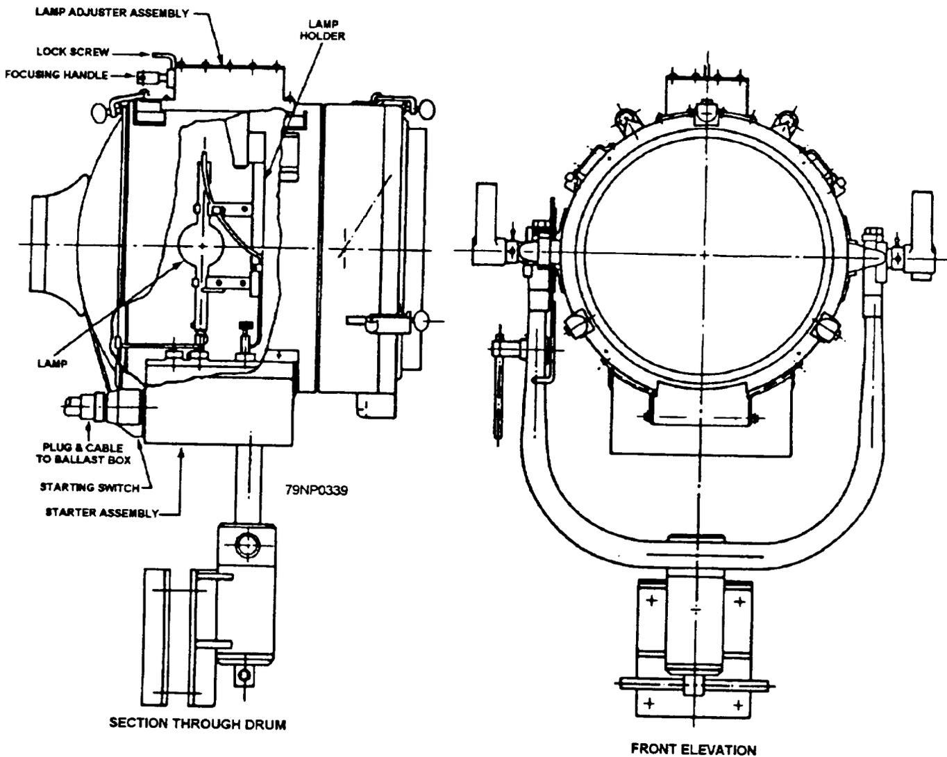
Figure 4-30.—A 12-inch incandescent searchlight converted to use a mercury-xenon arc lamp.
