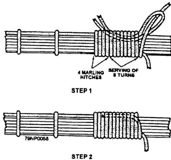
Figure 2-11.—The loop method of terminating the lace.
