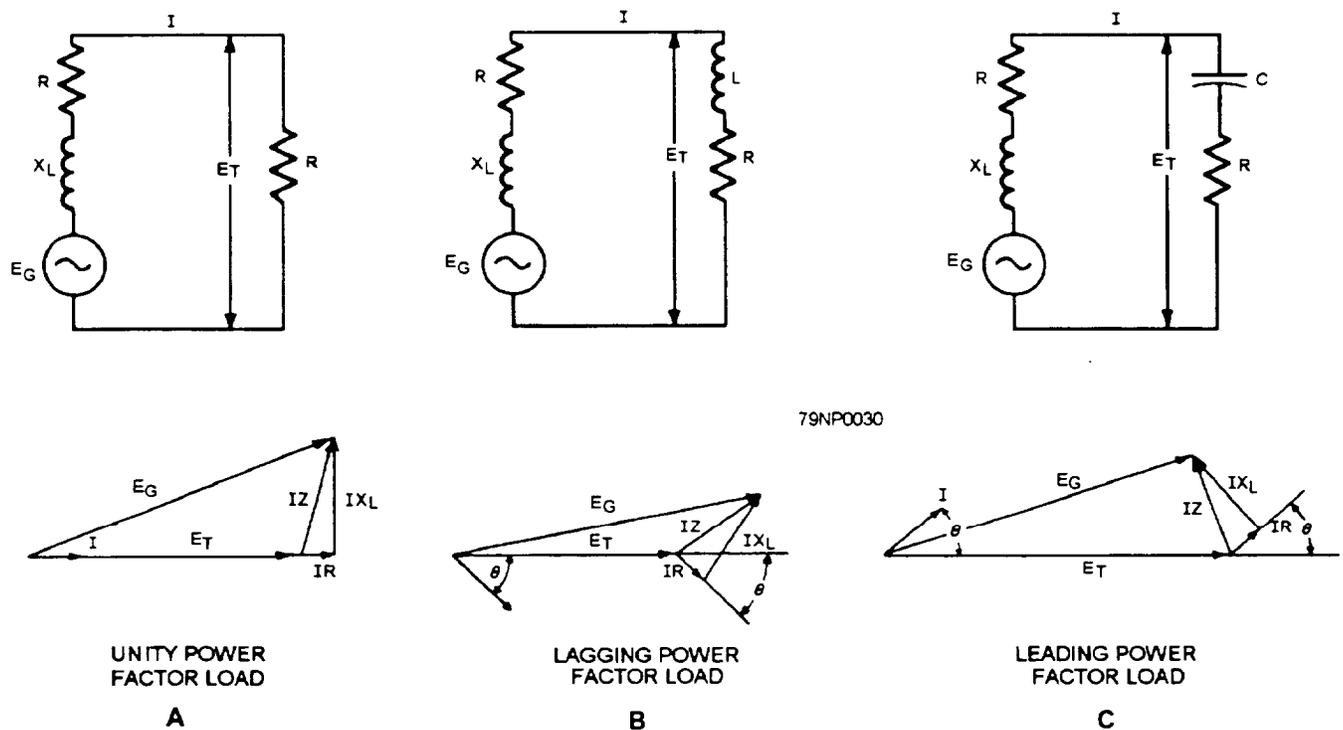
Figure 3-30.—The ac generator voltage characteristics.
