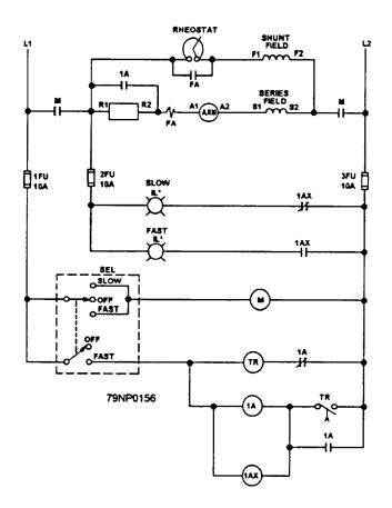
Figure 6-15.-A two-speed de controller with shunt field rheostat.
