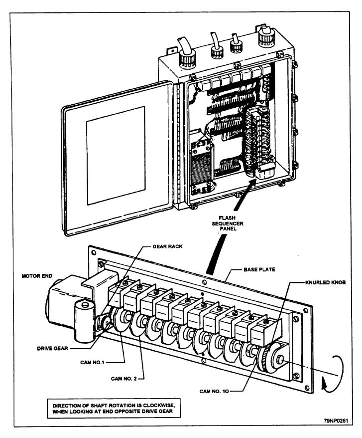
Figure 12-20.—Flash sequencer panel and timer assembly.
