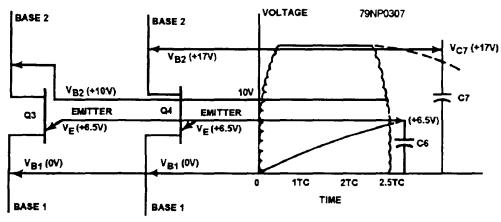
Figure 8-38.—Firing sequence for Q3.
