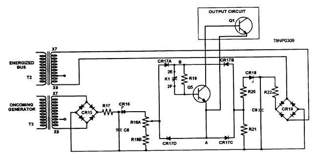
Figure 8-40.—Schematic diagram of voltage difference monitoring circuit.
