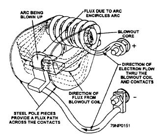
Figure 6-10.—Action of a magnetic blowout coil.
