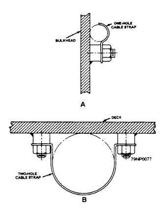
Figure 2-30.—Single cable strap application.
