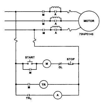
Figure 6-5.—Schematic of a reactor controller.
