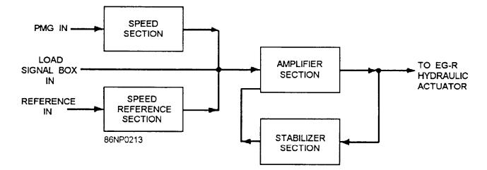
Figure 9-6.-EG-M control box, block diagram.
