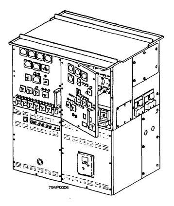
Figure 3-6.—1S Ship's service switchboard.
