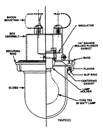
Figure 4-14.—A symbol 92.2 watertight fixture.
