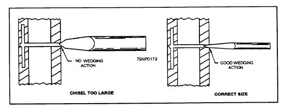
Figure 7-8.—Cracking seized inner ring of bearing.
