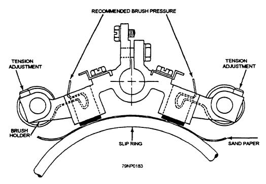
Figure 7-13.—Detail of brush rigging with sandpaper in position.
