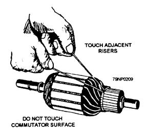
Figure 7-40.—Testing armature coils for an open circuit.
