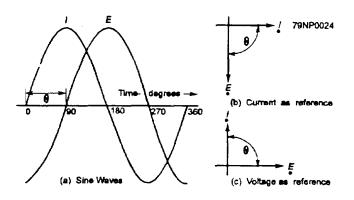
Figure 3-25.—Waves and vectors of alternating current and voltage in a circuit containing only capacitance.
