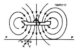
Figure 10-6.—Magnetic field due to the vertical magnetization of the ship.
