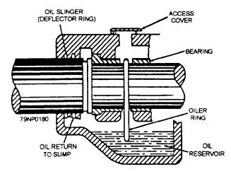
Figure 7-9.—Diagram of an oil-lubricated bearing.
