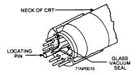
Figure 1-17.—Cathode-ray tube base structure.
