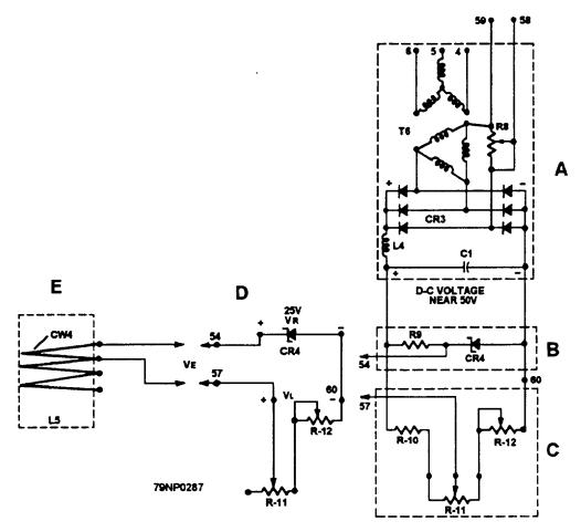
Figure 8-18.—Automatic voltage regulator.
