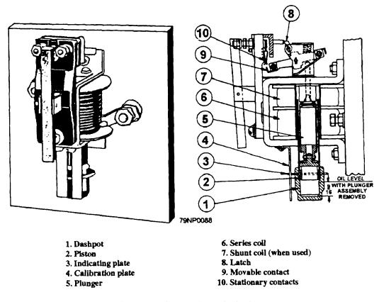
Figure 2-41.—A magnetic overload relay.
