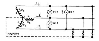
Figure 3-21.—Three-phase, ac generator showing neutral connection.
