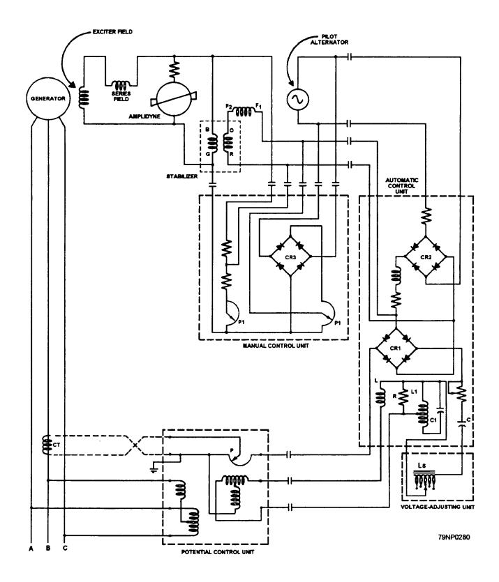
Figure 8-11.—Schematic diagram of amplidyne voltage regulator installation.
