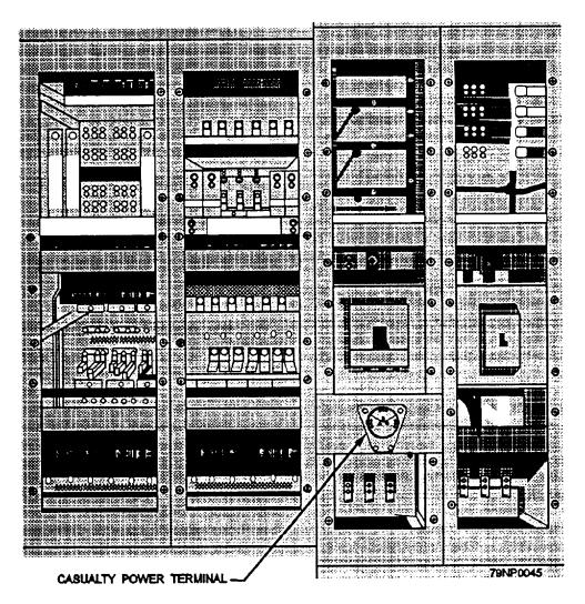
Figure 3-45.-Rear of switchboard showing casualty power terminal.
