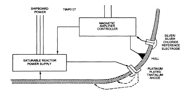
Figure 11-4.-Basic impressed current cathodic protection system.
