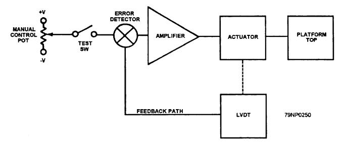
Figure 12-10.-LVDT servo loop.
