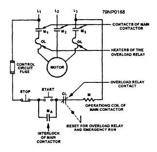
Figure 6-27.—Schematic of controller with reset-emergency lever or rod.
