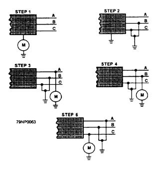
Figure 2-16.—Measuring circuit insulation resistance.
