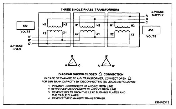
Figure 4-3.—Delta-delta transformer connections.
