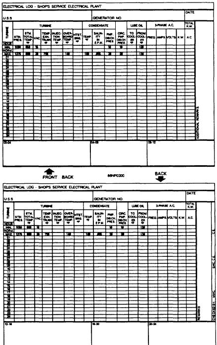
Figure 13-7.-Electrical Log-Ship's Service Electric Plant.
