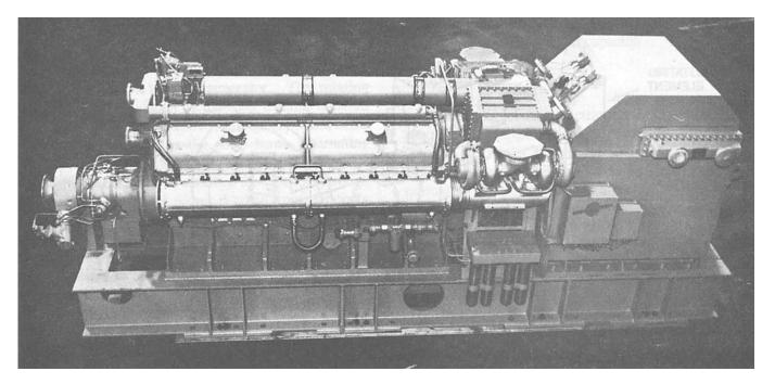
Figure 3-16.—Low-speed, engine-driven ac generator.
