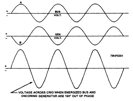
Figure 8-32.-Input voltage to CR10 (180° out of phase).
