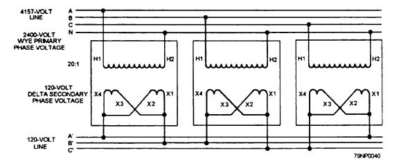
Figure 3-40.-Wye-delta transformer connections.
