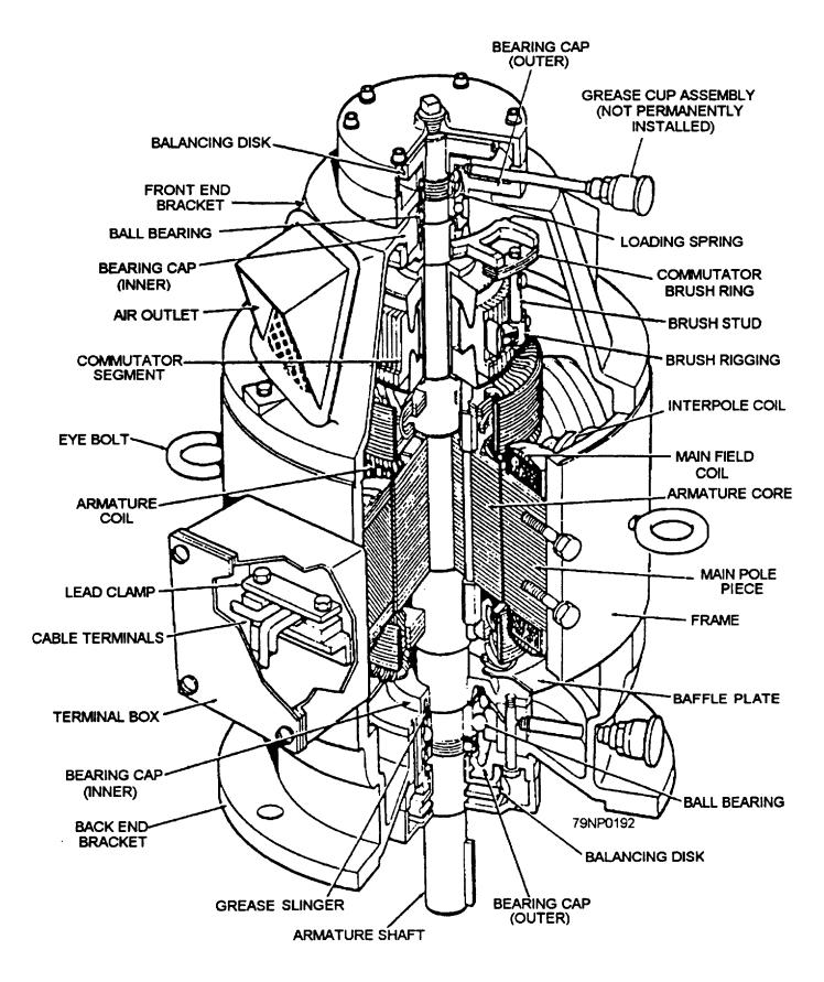
Figure 7-22.—Typical dc Motor.
