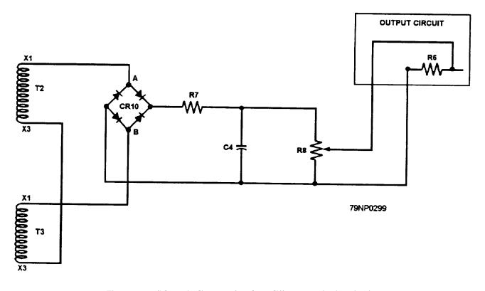
Figure 8-30.-Schematic diagram of a phase differnce monitoring circuit.
