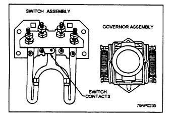
Figure 7-68.—Two major parts of a centrifugal switch.
