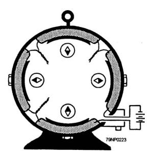
Figure 7-55.—Testing the polarity of field coils.
