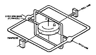
Figure 12-17.-Vertical gyro-simplified schematic.
