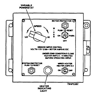
Figure 5-14.—Control box assembly.
