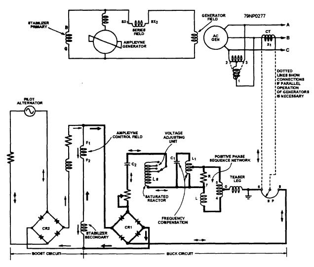
Figure 8-8.—Automatic control circuit.
