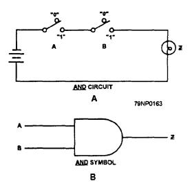
Figure 6-22.—AND symbol and circuit.
