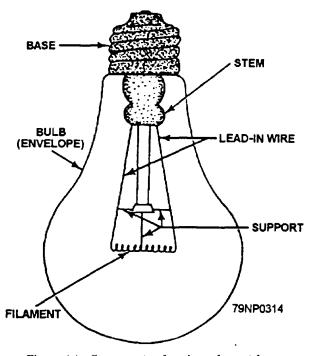
Figure 4-4.—Components of an incandescent lamp.
