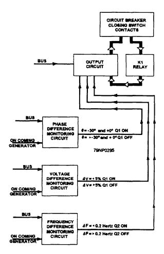
Figure 8-26.—Block diagram of synchronizing monitor.
