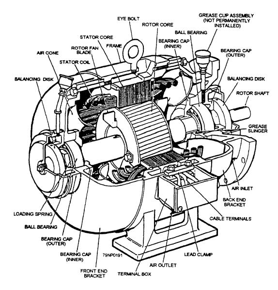
Figure 7-21.—Typical ac motor.
