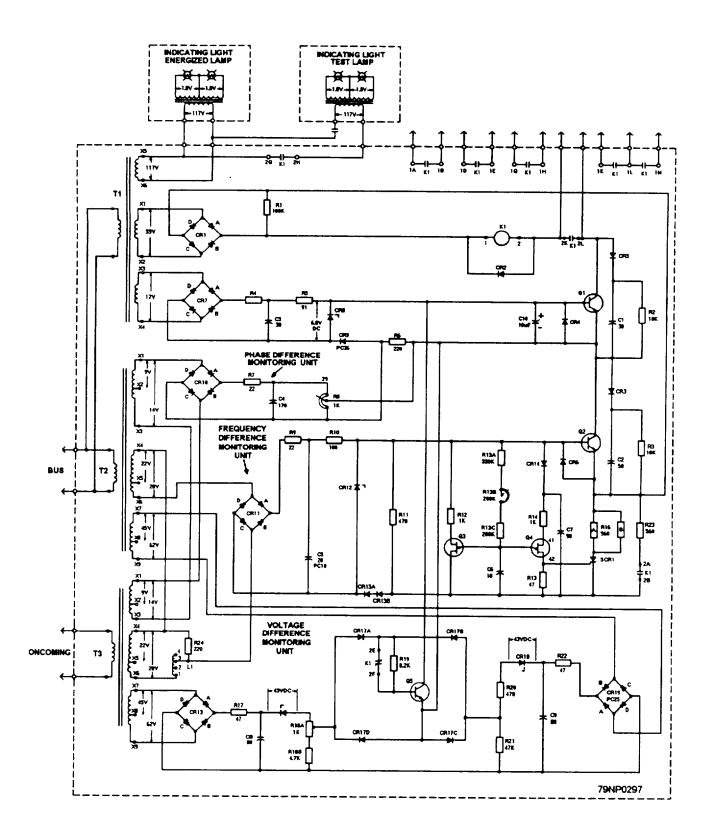
Figure 8-28.—Synchronizing monitor.
