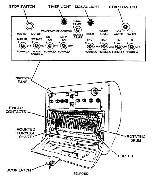
Figure 5-52.—A typical automatic control timer.
