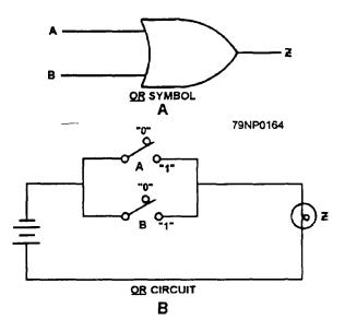
Figure 6-23.—OR symbol and circuit.
