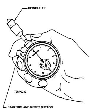
Figure 7-65-A chronometric tachometer.
