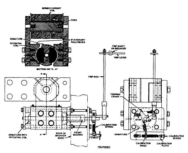
Figure 2-46.-Mechanical construction of an dc reverse-current relay.
