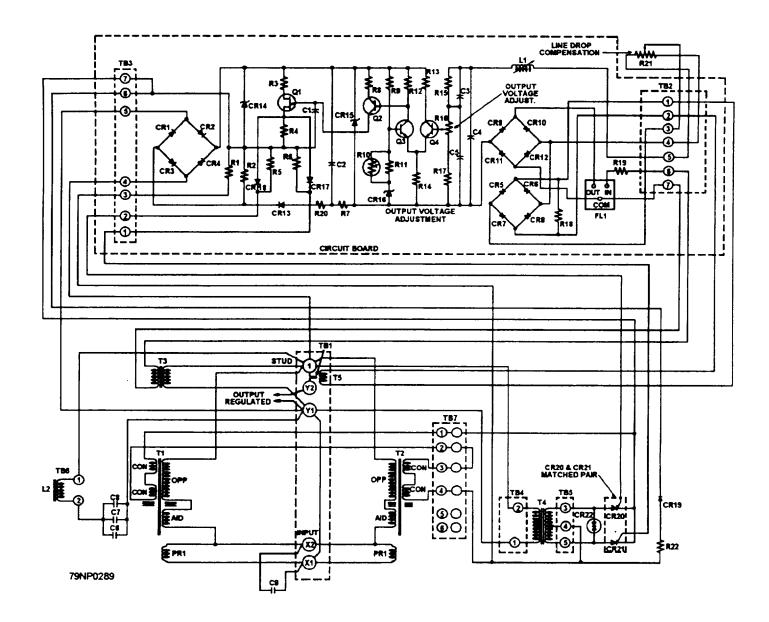
Figure 8-20.—SPR-400 line voltage regulator.
