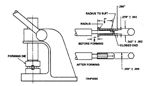
Figure 2-19.—Method of securing a copper ferrule to a conductor.
