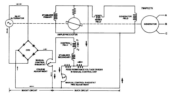
Figure 8-10.—Manual control circuit.
