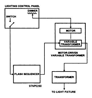
Figure 12-19.-Simplified interconnection of line-up lights.
