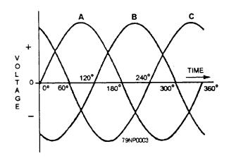
Figure 3-3.—Sine curve for three-phase circuit.
