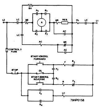
Figure 6-17.—Reversing dc controller.
