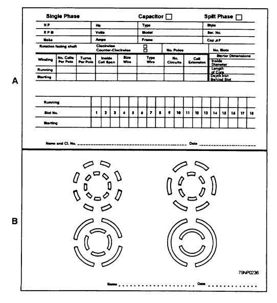
Figure 7-69.—Single-phase motor data card. (A) Front side; (B) back side.
