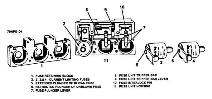
Figure 2-57.—Current-limiting fuse unit assembly.
