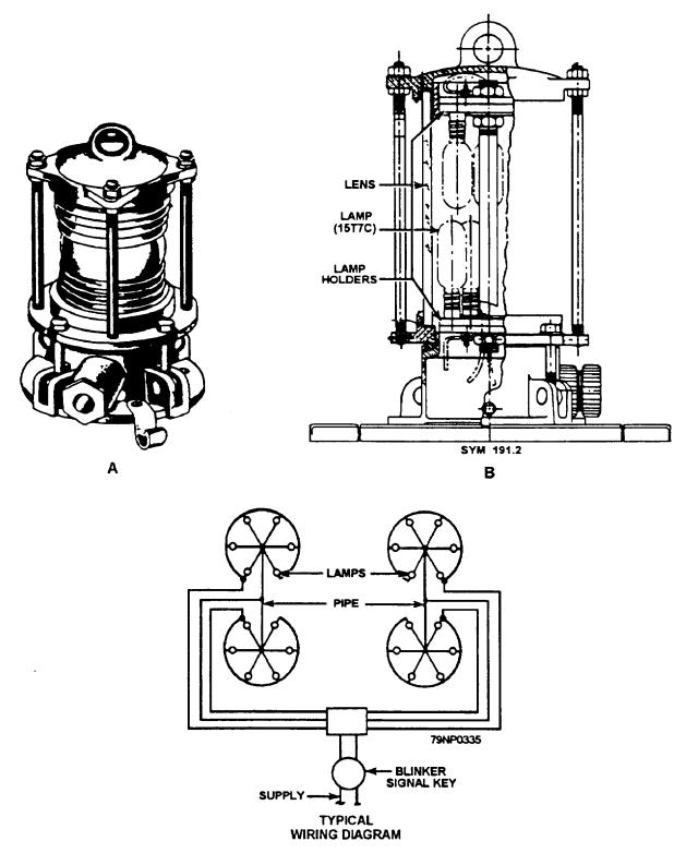
Figure 4-26.—Blinker light fixture.
