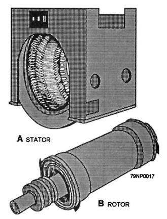
Figure 3-17.—High-speed, steam turbine-driven ac generator.
