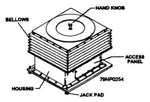
Figure 12-14.-stabilized platform assembly.
