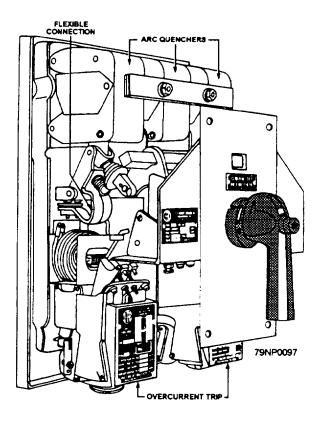
Figure 2-50.—Type ACB circuit breaker.
