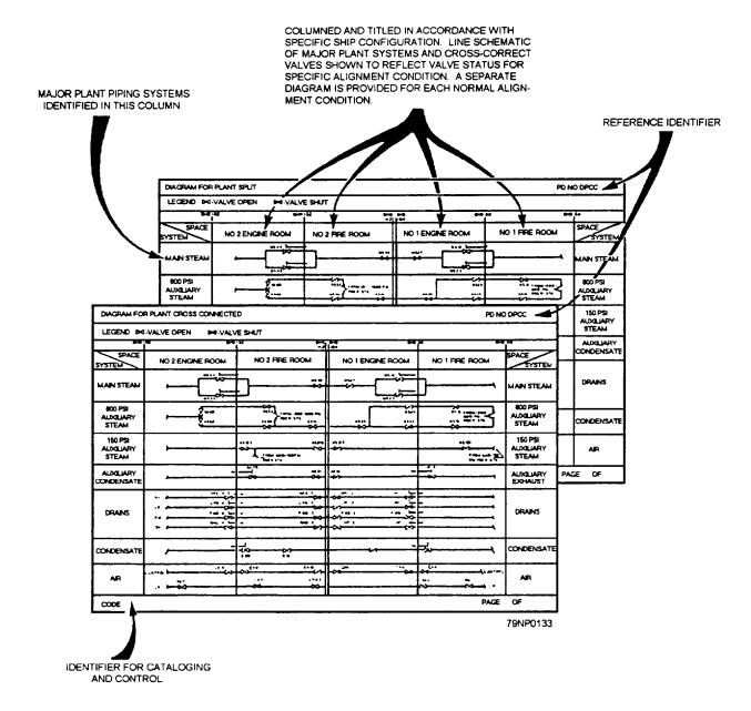
Figure 14-3.—Sample preferred alignment diagrams.
