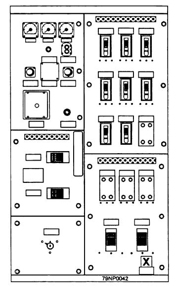
Figure 3-42.—400-hertz switchboard.
