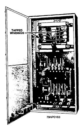
Figure 6-19.—Autotransformer controller.
