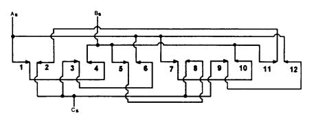
Figure 7-64.-Three-phase, four-pole, parallel-delta winding.
