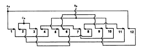
Figure 7-63.—Three-phase, four-pole, series-delta winding.
