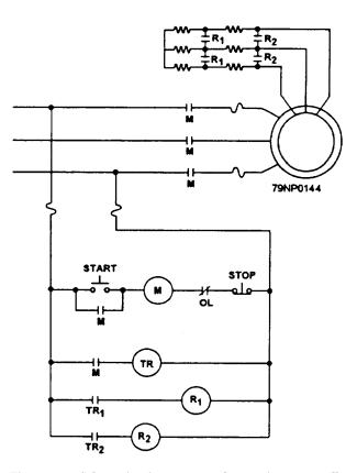
Figure 6-3.—Schematic of an ac secondary resistor controller.
