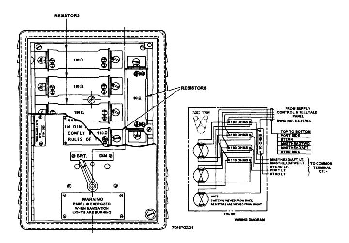
Figure 4-22.—Dimmer control panel, symbol 989.
