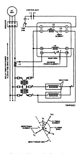
Figure 2-45.—Schematic wiring diagram of an ac reverse-power relay.
