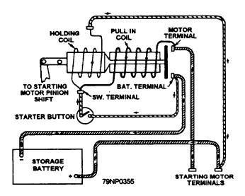
Figure 5-6.—Solenoid switch diagram.
