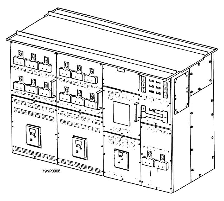
Figure 3-8.—1SB Ship's service switchboard.
