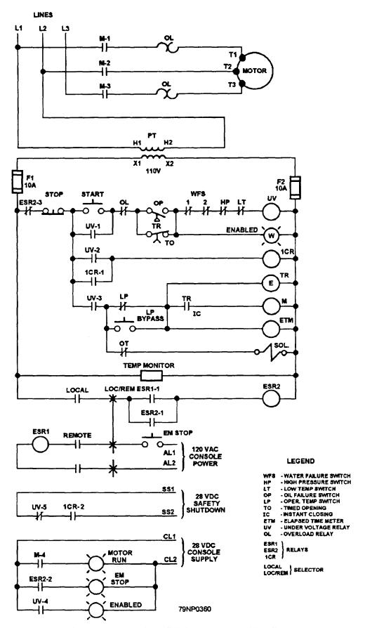
Figure 5-12.—80-ton air-conditioning compressor wiring diagram.
