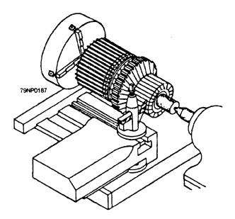
Figure 7-17.—Truing a commutator by turning.
