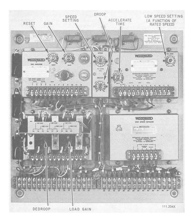
Figure 9-14.—2301 load - and speed-sensing control.
