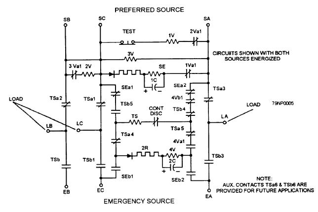
Figure 3-5.—Schematic diagram of the A-2 ABT.
