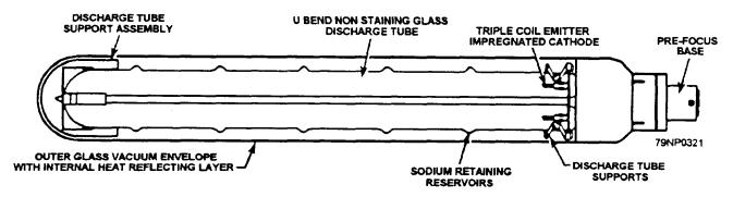
Figure 4-11.--A typical low-pressure sodium (LPS) lamp.
