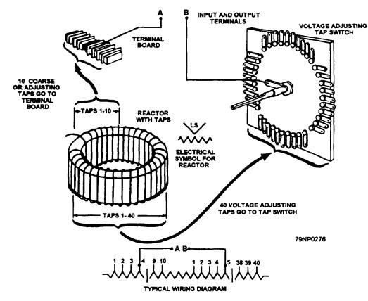
Figure 8-7.-Voltage-adjusting unit.
