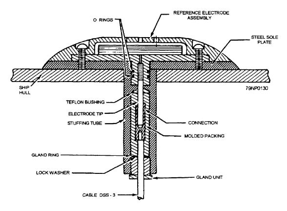
Figure 11-7.-Reference electrode assembly.
