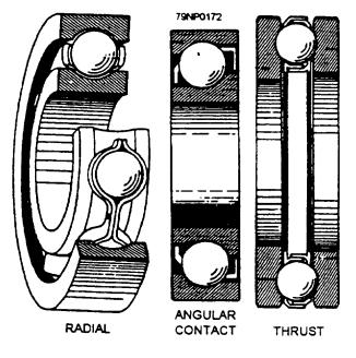
Figure 7-1.—Representative types of ball bearings.
