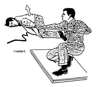
Figure 1-9.—Pushing a victim away from a power line.
