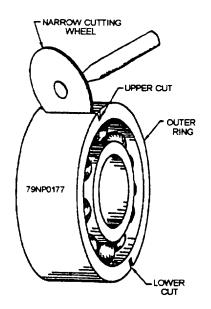
Figure 7-6.—Removing seized outer ring of bearing.
