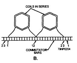
Figure 7-35.—Four-pole simplex wave windings.
