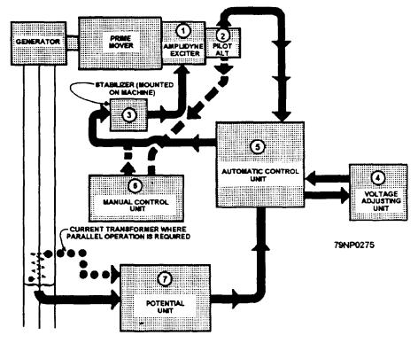
Figure 8-6.-Block diagram of an amplidyne voltage regulator system.
