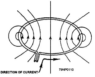
Figure 10-4.—Magnetic field of a current-carrying coil.
