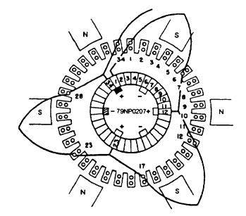
Figure 7-38.—Portion of a six-pole simplex wave winding.
