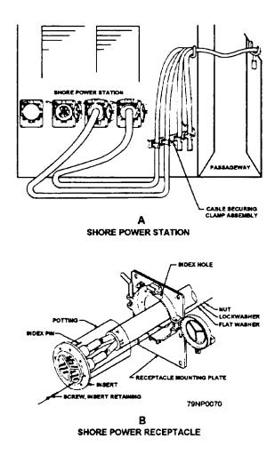
Figure 2-23.—Shore-power station and receptacle assembly.
