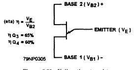
Figure 8-36.—Unijunction transistor.
