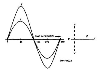
Figure 3-23.—Waves and vectors of alternating current and voltage in a circuit containing only resistance.
