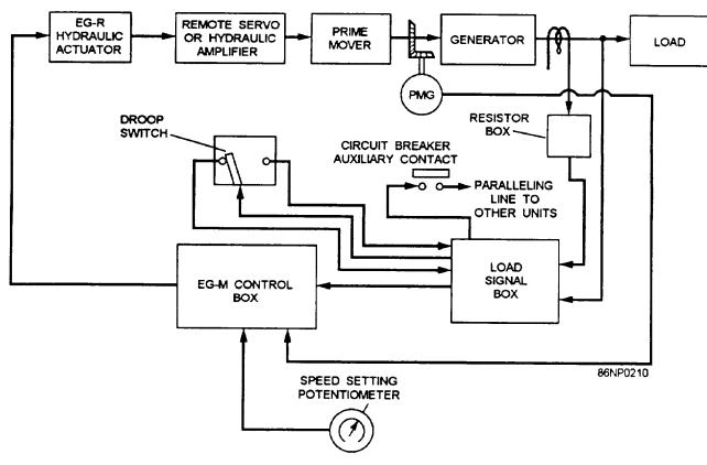
Figure 9-3.-Electrohydraulic load-sensing governor system, block diagram.
