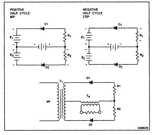
"Reprinted with permission of Woodward Governor Company, 1994" Figure 9.21—Equivalent single-phase circuit.
