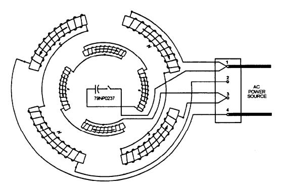
Figure 7-70.-Single-phase, capacitor-start, inductor-run motor diagram.
