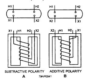
Figure 3-41.—Polarity markings for large transformers.
