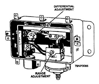
Figure 2-39.—A pressure-operated switch.
