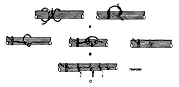
Figure 2-9.—Lacing procedure.
