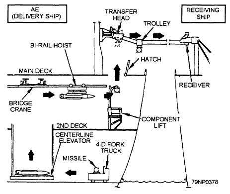
Figure 5-30.-UNREP system equipment used to move a missile from storage to the receiving ship.
