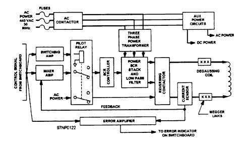
Figure 10-16.—Block diagram for a type SSM degaussing power supply.
