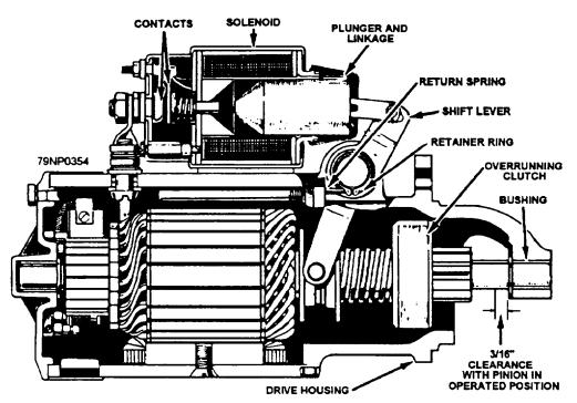
Figure 5-5.—Starting motor with an overrunning clutch drive and a solenoid-operated switch.
