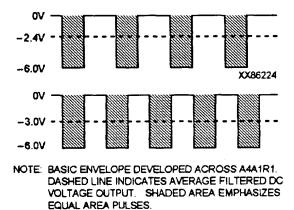
"Reprinted with permission of Woodward Governor Company, 1994" Figure 9-19.—Speed sensor output voltage.
