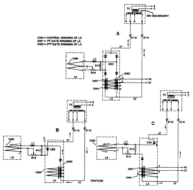
Figure 8-17.-First-stage magnetic amplifier.
