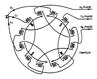
Figure 7-61.—Three-phase, four-pole, series-wye winding showing the four poles.
