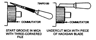
Figure 7-19.—Undercutting mica with a hacksaw blade.
