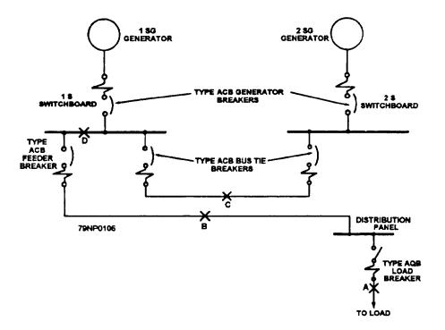
Figure 2-59.—Selected tripping of circuit breakers.
