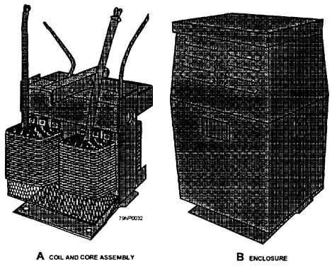
Figure 3-32.—Single-phase transformer.
