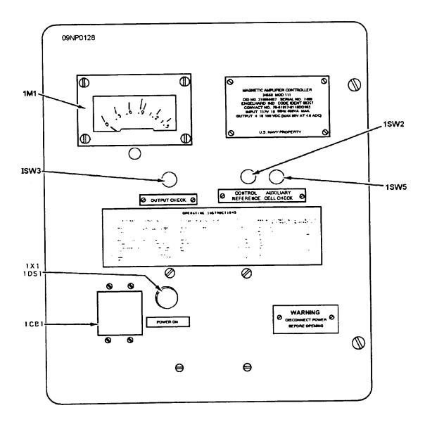
Figure 11-5.—Magnetic amplifier controller Mod III.
