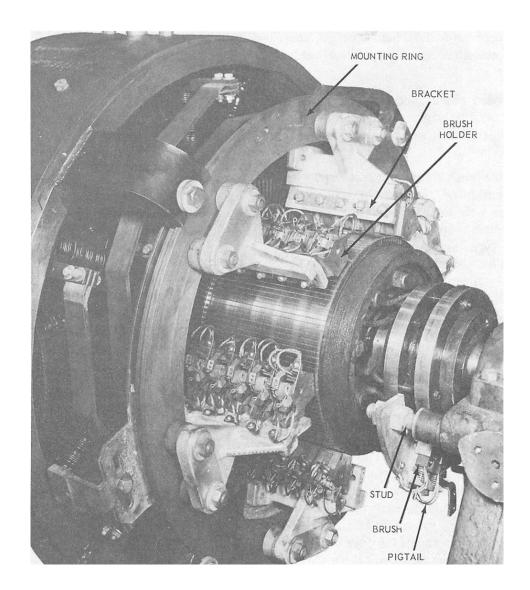
Figure 7-10.—Brush holder and brush rigging assembly.
