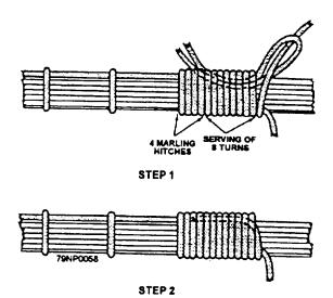
Figure 2-11.—The loop method of terminating the lace.
