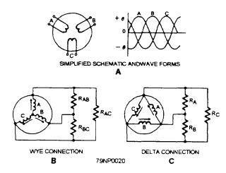
Figure 3-20.—Three-phase ac generator.
