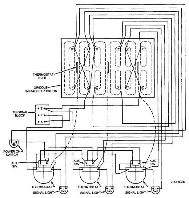
Figure 5-48.-Electric griddle wiring diagram.
