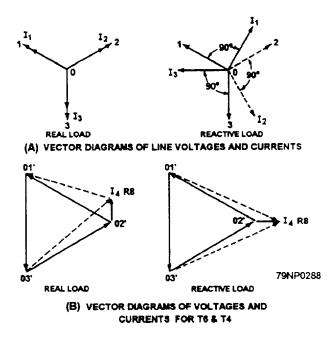
Figure 8-19.- Vector diagrams of reactive droop circuit-
