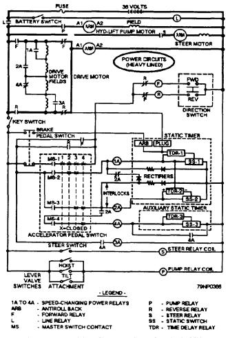
Figure 5-38.-Wiring diagram of an electric forklift.
