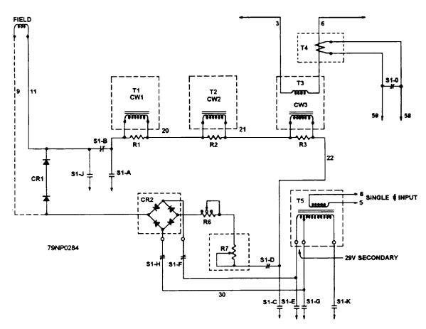
Figure 8-15.-Manual voltage control circuits.
