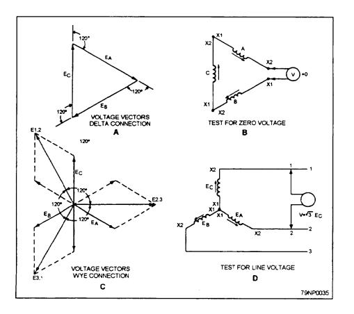
Figure 3-35.—Delta-connected transformer secondaries.
