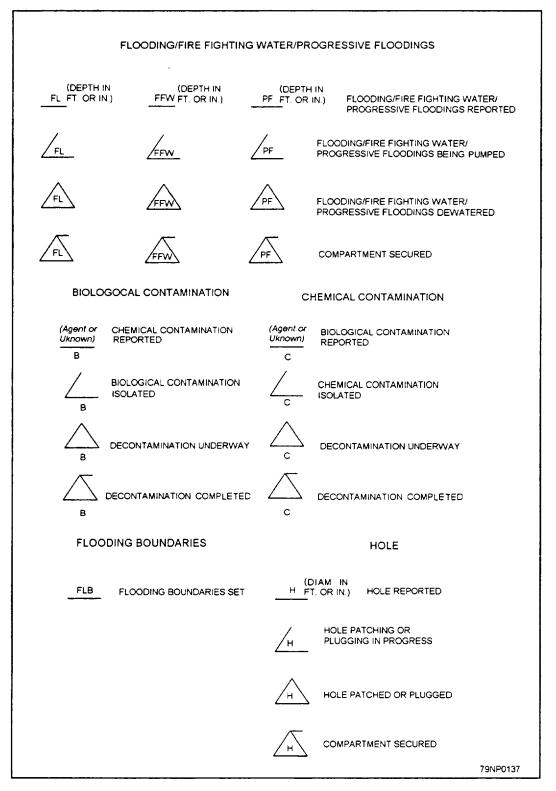
Figure 14-7.-Navy standard damage control symbology.
