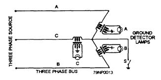
Figure 3-13.—An ac ground detector lamp circuit.
