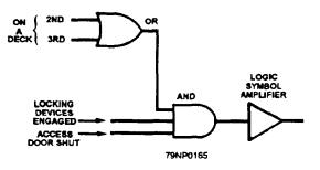
Figure 6-24.—Basic logic circuit.
