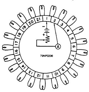
Figure 7-37.—Schematic of a simplex lap winding.
