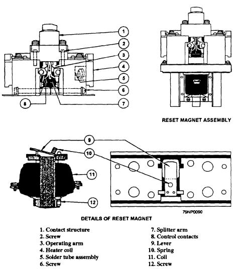
Figure 2-43.-An adjustable thermal overload relay and a reset magnet assembly.
