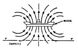
Figure 10-7.—Magnetic field produced by the M coil.
