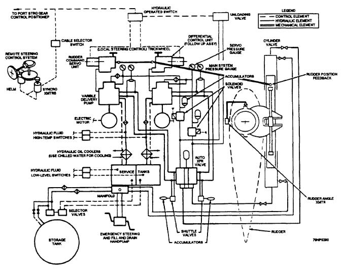
Figure 5-42.-Steering gear functional block diagram.
