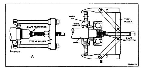
Figure 7-5.—Bearing pullers.
