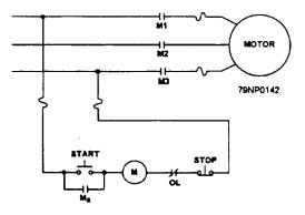
Figure 6-1.—Schematic of a simple across-the-line controller.
