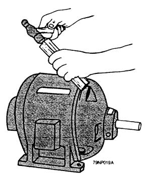
Figure 7-24.—Parting end bells with a hammer and a wood block.
