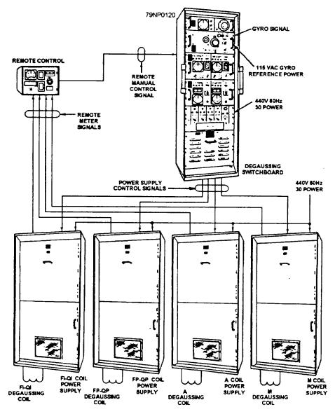
Figure 10-14.-SSM automatic degaussing equipment.
