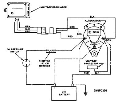
Figure 5-7.--A typical alternator electrical system wiring diagram.
