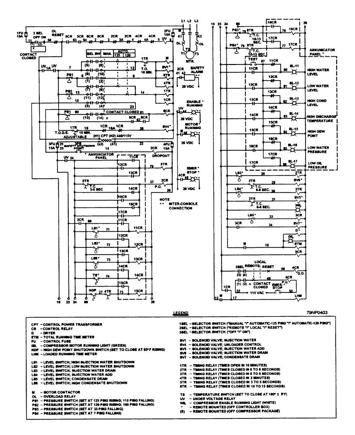
Figure 5-9.—Air compressor schematic diagram.
