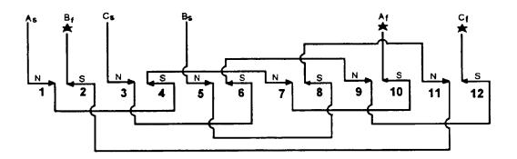
Figure 7-60.-Three-phase, four-pole, series-wye winding.
