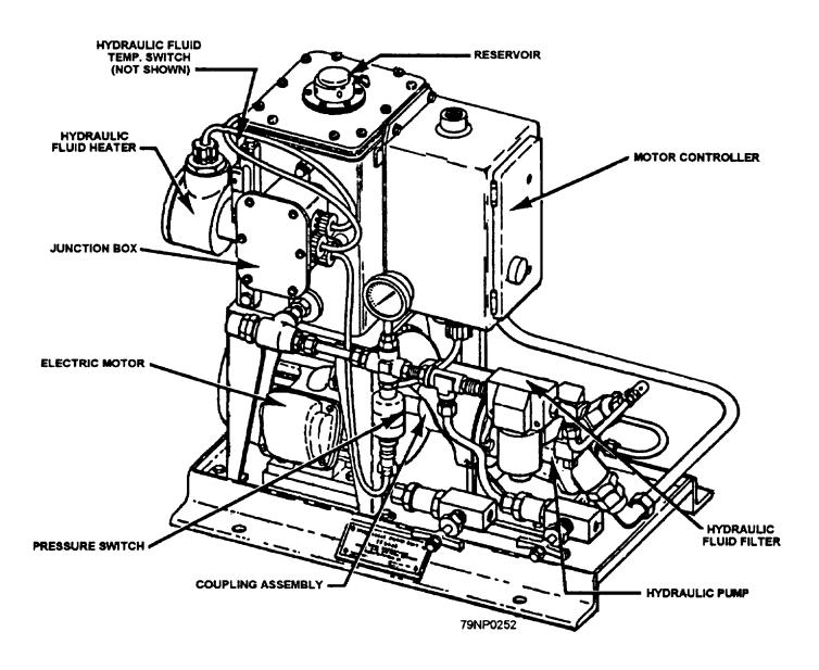
Figure 12-12.—Hydraulic pump assembly.
