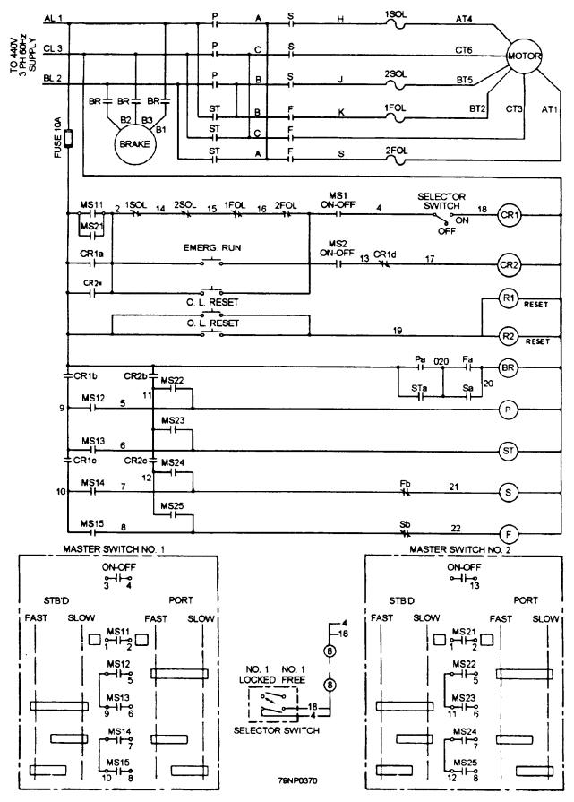
Figure 5-22.—Reversing across-the-line starter for a two-speed anchor windlass.
