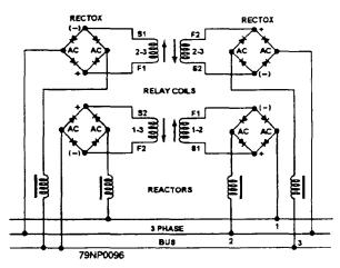
Figure 2-19.—Schematic wiring of a phase-failure relay.
