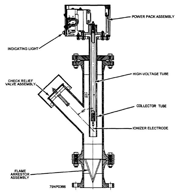
Figure 5-18.—Vent fog precipitator.
