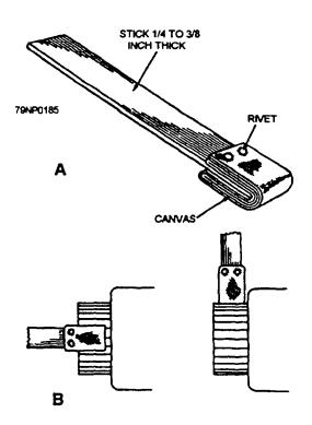
Figure 7-15.—Cleaning commutator or collector rings.
