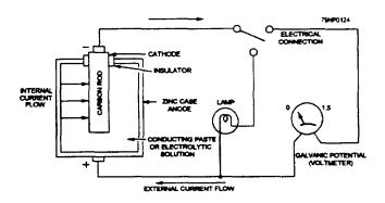
Figure 11-1.—Dry-cell battery circuit.
