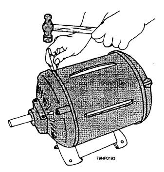
Figure 7-23.-Marking a motor frame and end bell.
