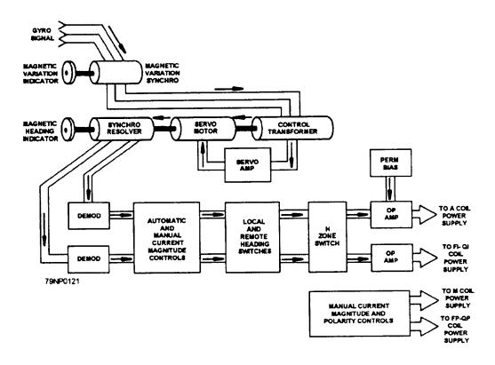
Figure 10-15.—Block diagram for an SSM degaussing switchboard.
