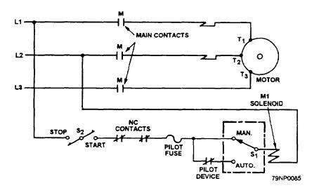
Figure 2-38.—A representative pilot device control circuit.
