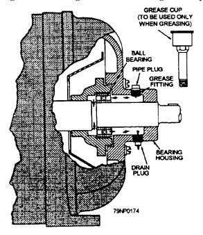
Figure 7-3.—Grease-lubricated ball bearings.
