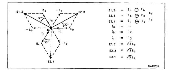
Figure 3-26.-Three-phase, wye-connected system.
