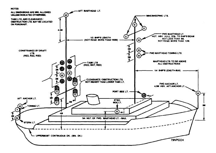
Figure 4-15.—General arrangement of lights for navigation.
