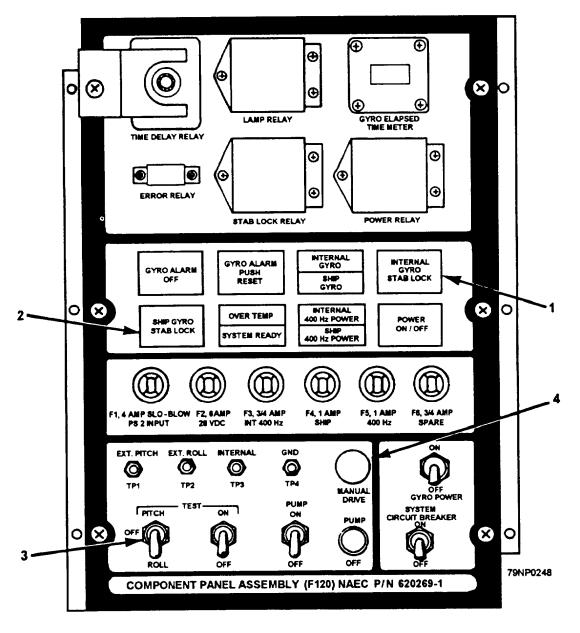
1. Internal Gyro Stab Lock switch-indicator
