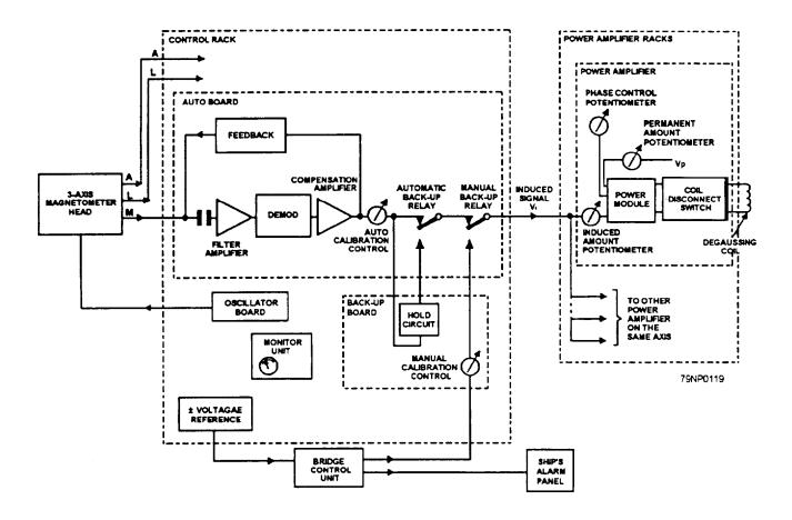
Figure 10-13.—Block diagram for type MDG degaussing system.
