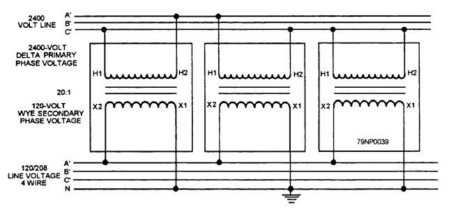
Figure 3-39.—Delta-wye transformer connections.
