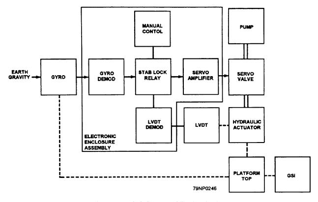
Figure 12-6.—Block diagram-stabilization circuits.
