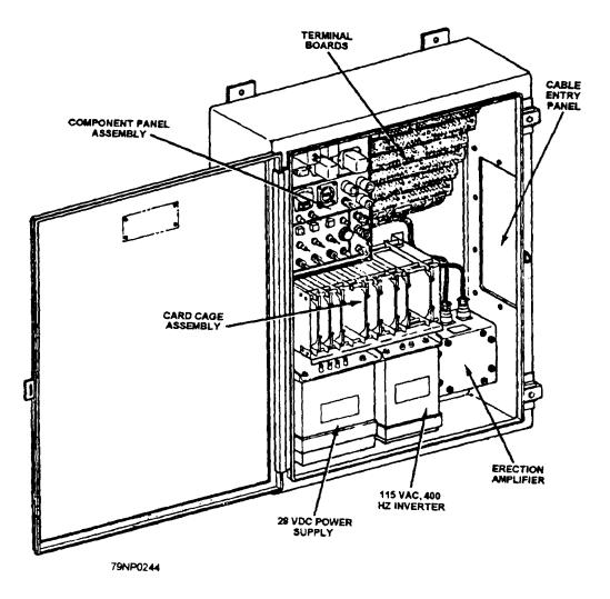
Figure 12-4.—Electronic enclosure assembly.
