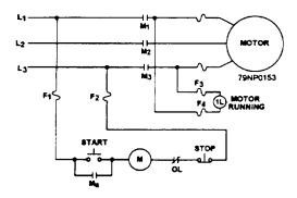
Figure 6-12.—Schematic of a simple LVP controller.
