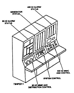
Figure 3-11.—Electric plant control console (EPCC).
