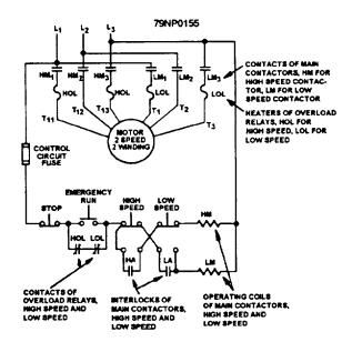
Figure 6-14.-Two-speed, ac controller.
