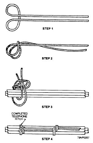
Figure 2-10.—Starting double lace with the telephone hitch.
