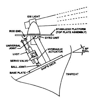
Figure 12-7.—Stabilized platform assembly-functional diagram.
