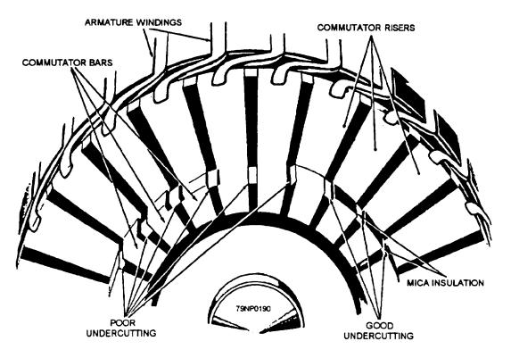
Figure 7-20.-Example of good and poor undercutting.
