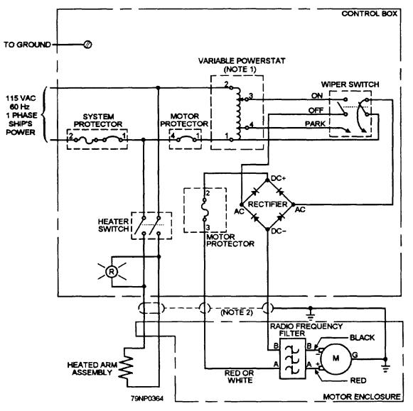
Figure 5-16.—Window wiper schematic.
