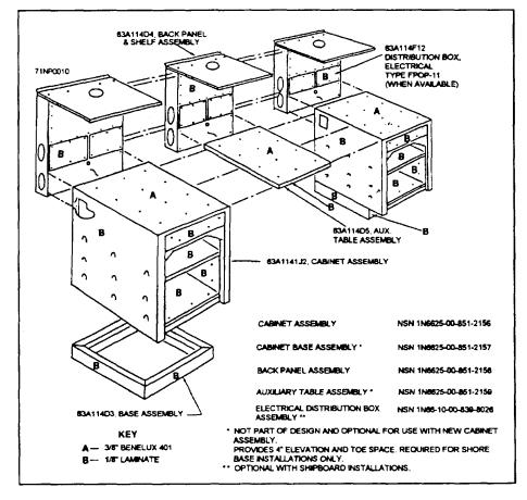
Figure 1-4.—A typical electric workbench.
