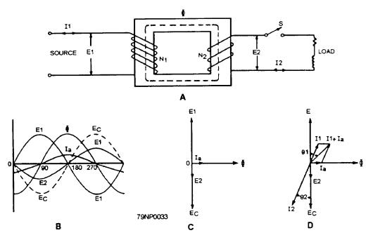
Figure 3-33.-Constant-potential transformer.
