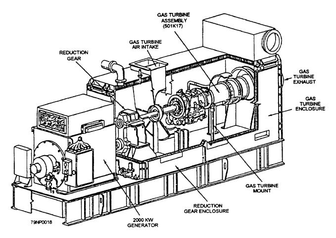
Figure 3-18.-Model 104 gas turbine generator set.
