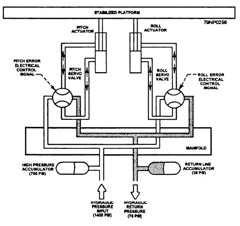
Figure 12-15.—Function diagram of the stabilized platform assembly.
