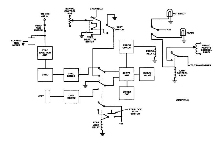
Figure 12-9.-Stabilization control circuits-signal flow.
