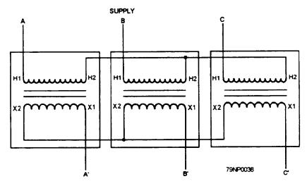
Figure 3-38.-Wye-wye transformer connections.
