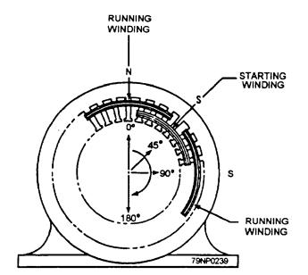
Figure 7-72.--A four-pole, split-phase motor.
