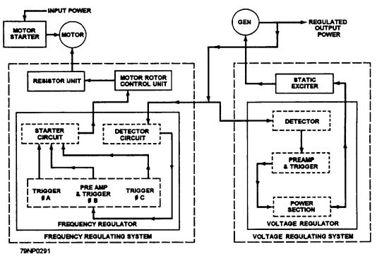
Figure 8-22.-Motor-generator set simplified block diagram.
