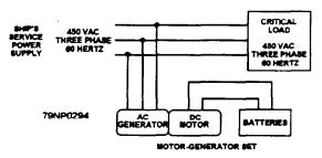
B. MODE 2 STOP GAP OPERATION FROM ASSOCIATED BATTERIES
