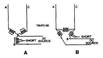
Figure 7-27.—Compass test for shorted pole-phase groups.
