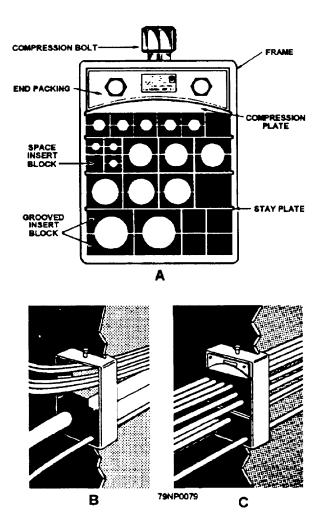
Figure 2-32.-Modular cable supports.
