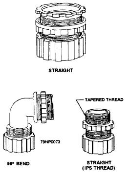
Figure 2-26.-Nylon Stuffing tubes.
