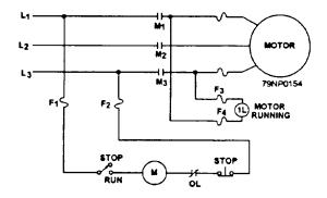
Figure 6-13.—Schematic of simple LVR controller.
