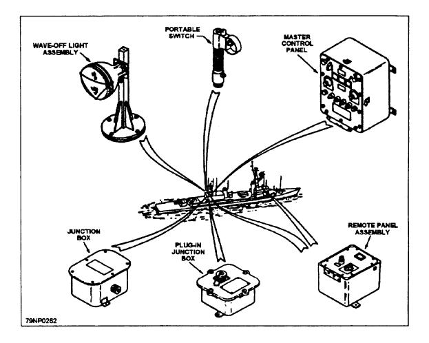
Figure 12-21.-Wave-off light system.
