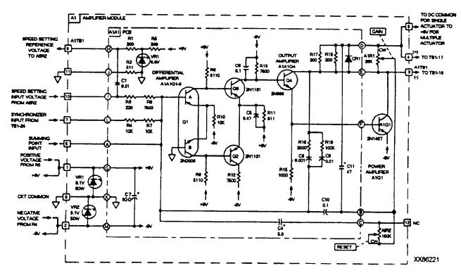
Figure 9-16.—Amplifier schematic.
