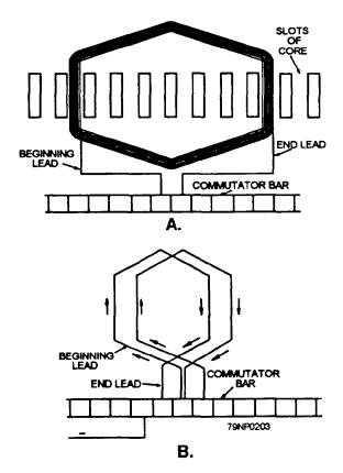
Figure 7-34.—Simplex lap windings.
