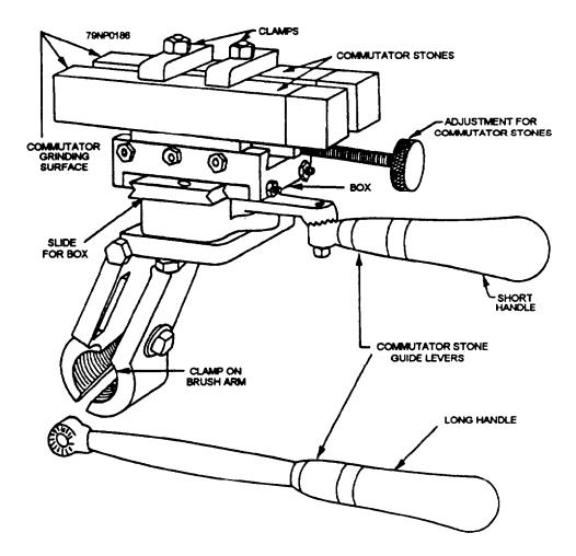
Figure 7-16.—Commutator dressing stone tool.
