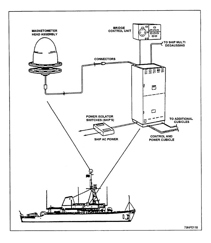
Figure 10-12.—Type MDG automatic degaussing equipment.
