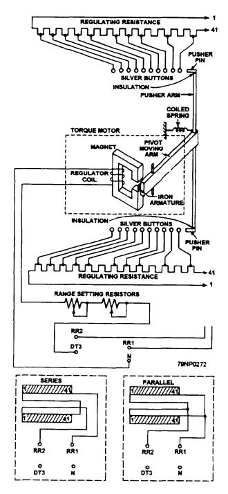
Figure 8-3.—Control element of a direct-acting voltage regulator.
