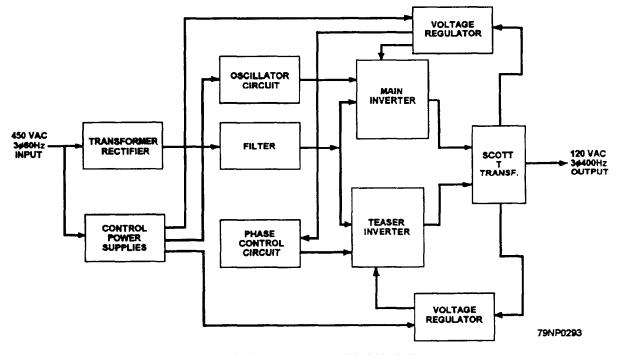
Figure 8-24.-Static converter, simplified block diagram.
