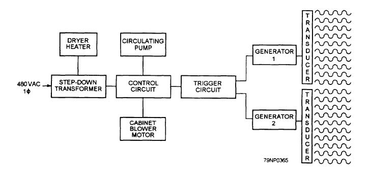
Figure 5-17.—Block diagram of ultrasonic cleaner.
