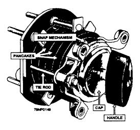
Figure 6-8.—Rotary snap switch.
