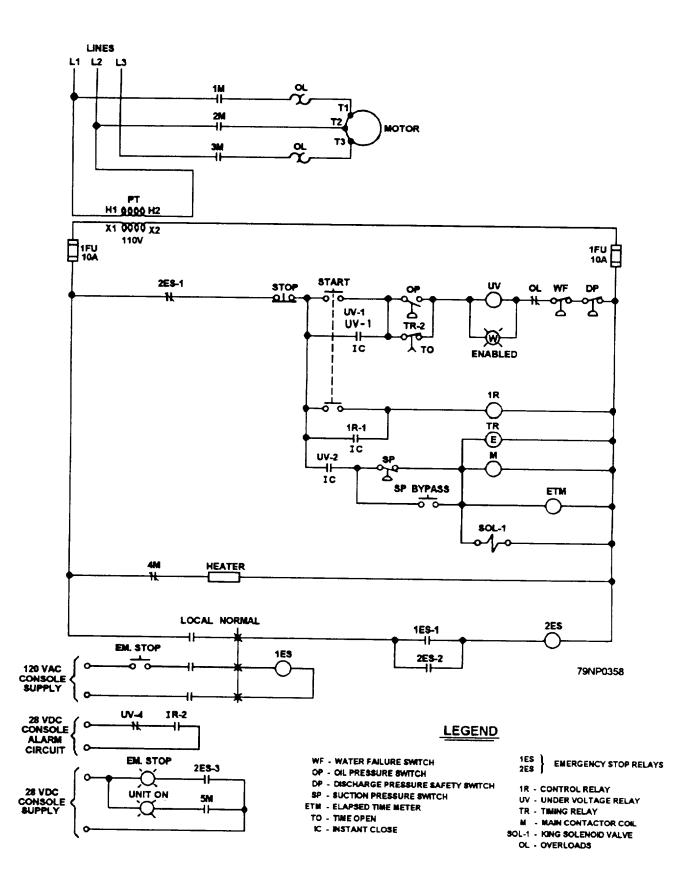
Figure 5-10.-Refrigeration plant wiring diagram.
