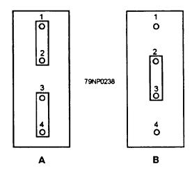
Figure 7-71.—Connecting bars. (A) Low voltage input; (B) High voltage input.
