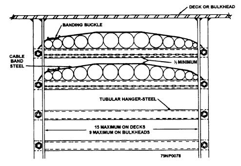
Figure 2-31.—Cables installed in a cable rack.
