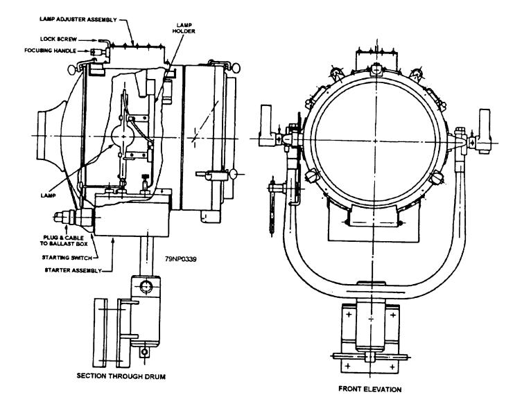
Figure 4-30.-A 12-inch incandescent searchlight converted to use a mercury-xenon arc lamp.
