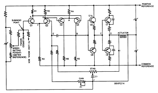
Figure 9-7.-EC-M control box, simplified schematic.
