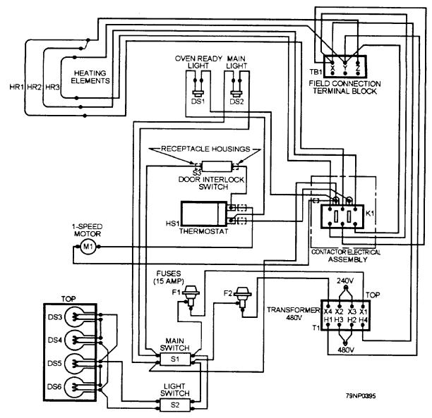
Figure 5-46.—Wiring diagram of M-series oven.
