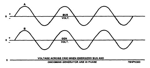
Figure 8-31.—Input voltage to CR10 (in phase).
