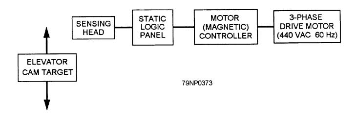
Figure 5-25.—Block diagram of electronic controlled elevator system.
