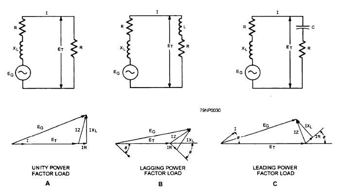
Figure 3-30.—The ac generator voltage characteristics.
