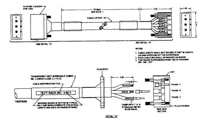
Figure 2-21.-New method of preparing casualty power cable ends.
