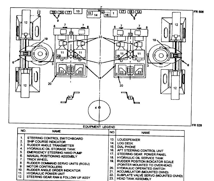
Figure 5-40.—Steering gear room (plan view).
