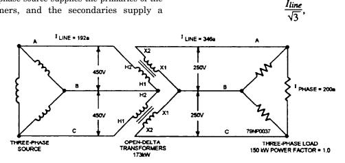
Figure 3-37.—Open-delta transformer connection.
