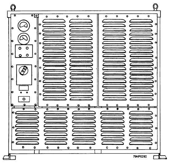
Figure 8-23.—Static converter, front view.
