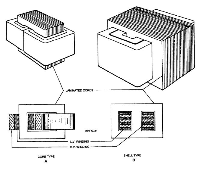
Figure 3-31.—Types transformer construction.
