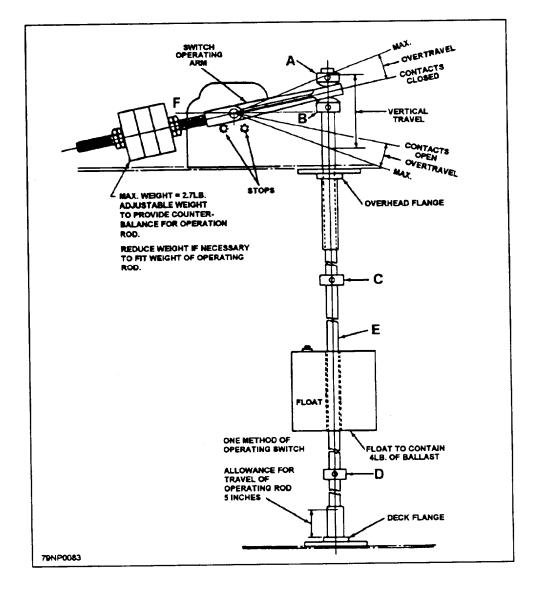
Figure 2-36.—A float switch tank installation.
