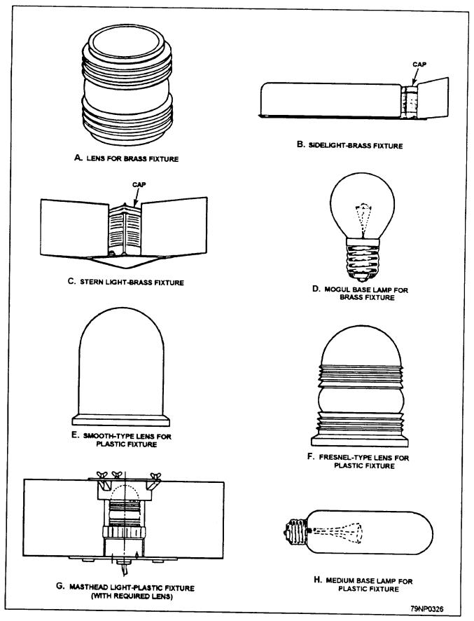
Figure 4-17.-Navigation light fixtures, lamps, and lenses.
