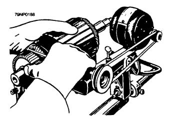
Figure 7-18.—Undercutting commutator mica with undercutter.
