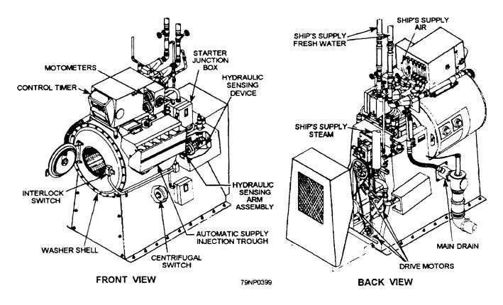
Figure 5-51.—A typical washer-extractor installation.
