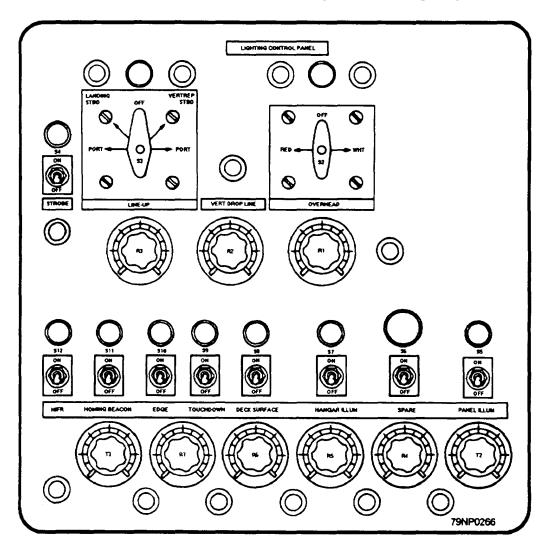
Figure 12-25.—Lighting control panel.
