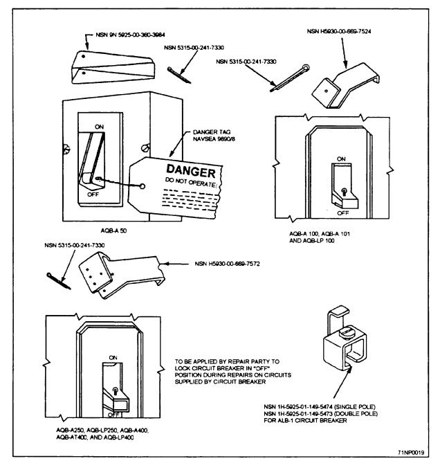
Figure 1-20.—Handle-locking devices for circuit breakers.
