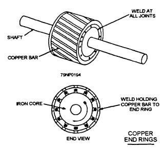
Figure 7-25.—Squirrel-cage rotor.
