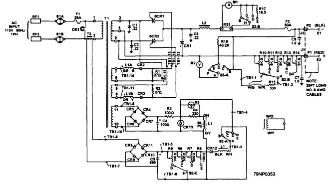
Figure 5-4-Battery charger wiring diagram.
