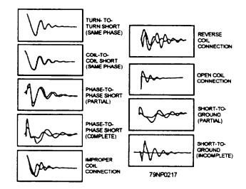
Figure 7-48.—Representative surge test waveforms.
