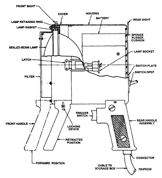
Figure 4-27.-Multipurpose signal light, symbol 106.1.
