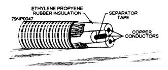
Figure 2-1.—Construction of low-smoke cable (typical).
