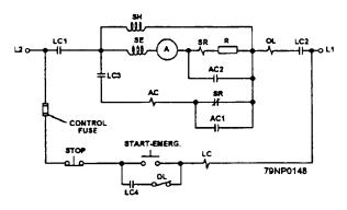
Figure 6-7.—Schematic of a dc resistor controller with one stage of acceleration.
