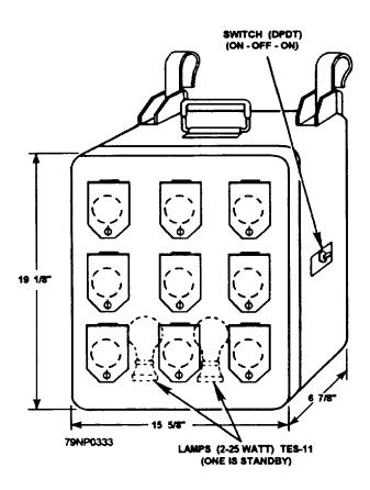
Figure 4-24.—Station marker box, symbol 285.
