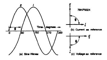
Figure 3-24.—Waves and vectors of alternating current and voltage in a circuit containing only inductance.
