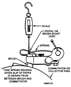
Figure 7-11.-Measuring brush tension.
