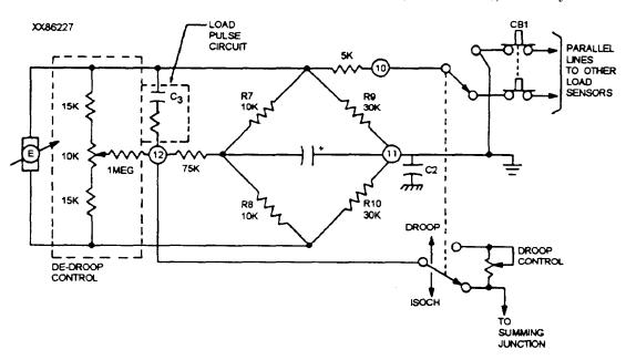
"Reprinted with permission of Woodward Governor Company, 1994" Figure 9-22.-Basic load sensor, single-unit configuration.
