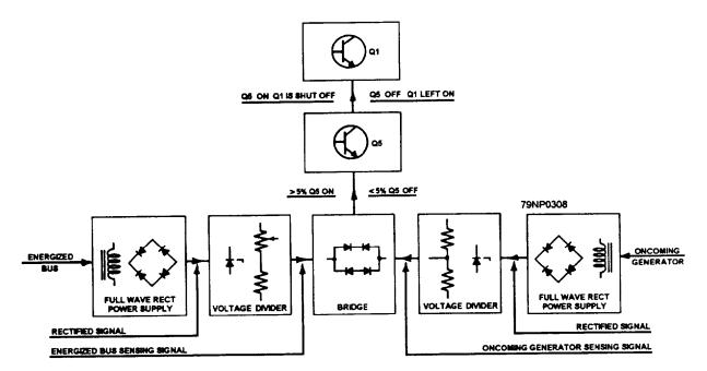
Figure 8-39.-Block diagram of voltage difference monitoring circuit.
