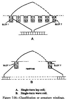
Figure 7-50.—Classification of armature windings.
