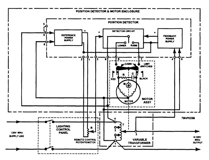
Figure 12-28.-Motor-driven remote variable transformer circuit diagram.
