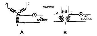
Figure 7-28.-Balanced current test for shorted phase.
