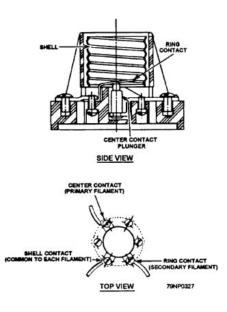
Figure 4-18.—New navigation light fixture lamp holder wiring diagram.
