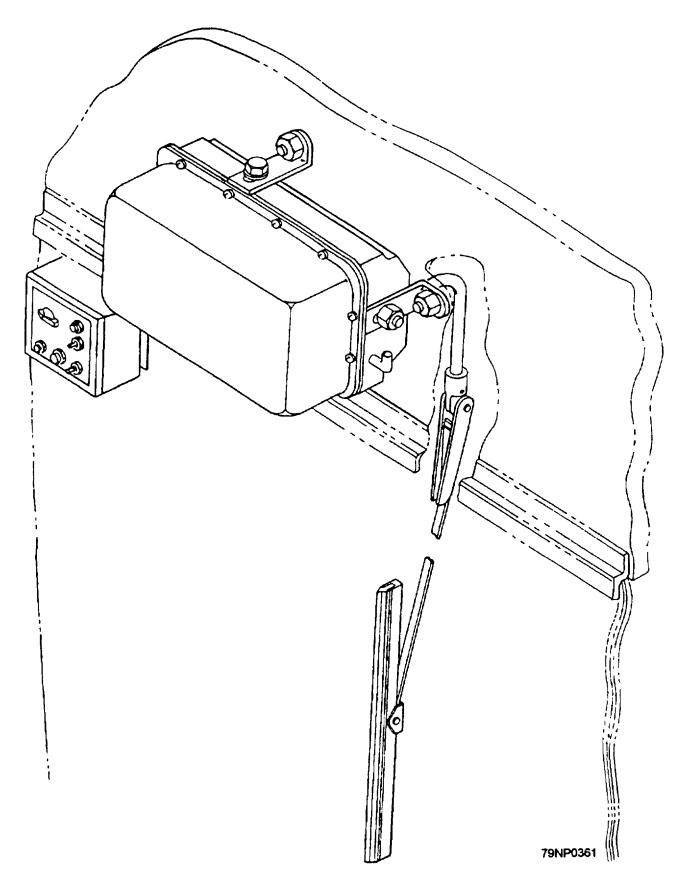
Figure 5-13.—Pendulum window wiper.
