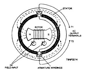
Figure 3-14.—Essential parts of a rotating-field generator.
