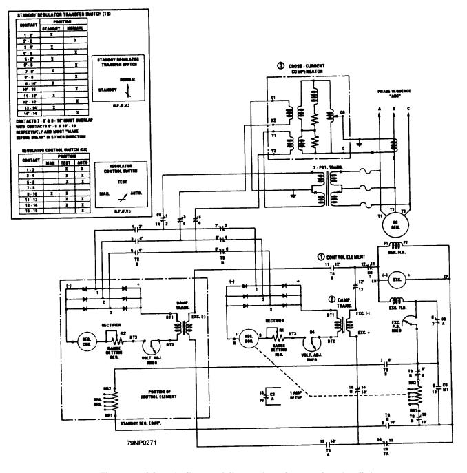
Figure 8-2.-Schematic diagram of direct acting voltage regulator installation.
