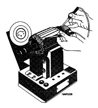
Figure 7-41.—Checking armature shorts with a growler.
