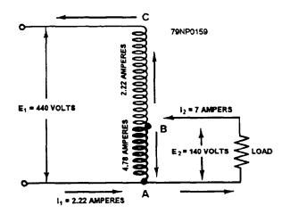
Figure 6-18.—Single-phase autotransformer.
