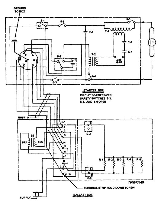
Figure 4-31.-Wiring diagram for an early model 12-inch mercury-xenon arc searchlight.
