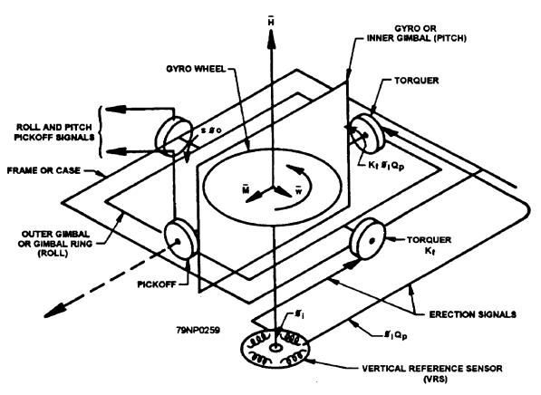
Figure 12-18.-Vertical gyro-line schematic diagram.
