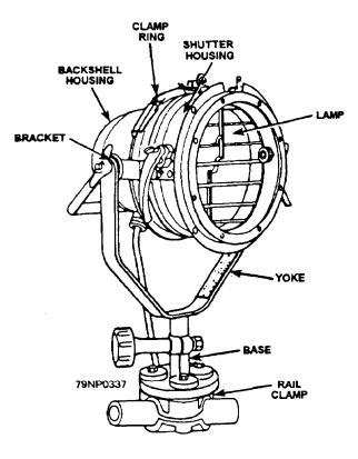
Figure 4-28.—An 8-inch, 60-hertz, sealed-beam searchlight.
