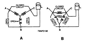
Figure 7-29.—Ohmmeter test for open circuits.
