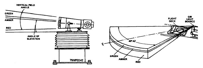
Figure 12-2.—Glide slope indicator and light beam.
