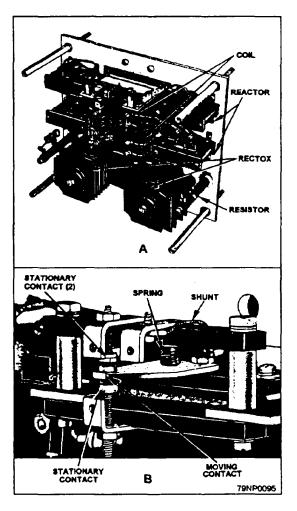
Figure 2-48.—A phase-failure day.
