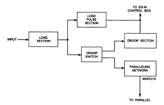
Figure 9-9.-Load signal box, block diagram.
