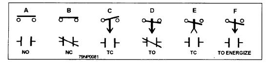
Figure 2-34.—Electrically operated contacts.
