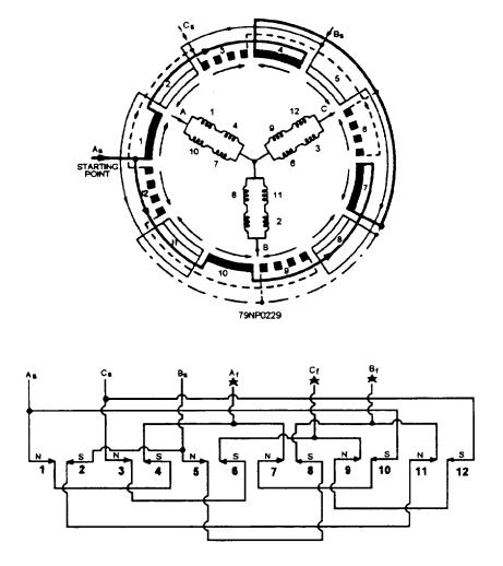
Figure 7-62.-Three-phase, four-pole, parallel-wye winding.
