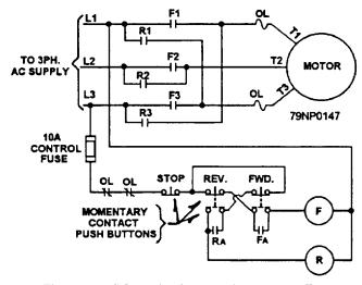
Figure 6-6.—Schematic of a reversing ac controller.
