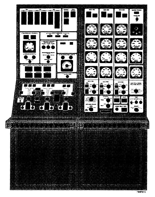
Figure 3-12.-EPCC showing distribution and system status and control sections.
