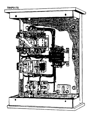
Figure 6-29.—Typical three-phase controller.
