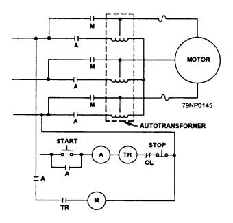
Figure 6-4.—Schematic of an autotransformer controller.
