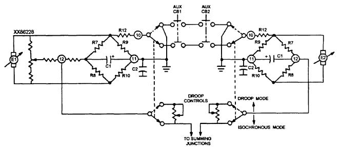
"Reprinted with permission of Woodward Governor Company, 1994" Figure 9-23.—Basic load sensor, parallel unit configuration.
