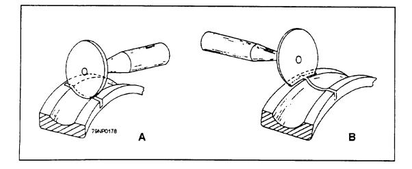
Figure 7-7.-Removing seized inner ring of bearing.
