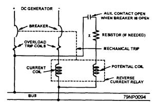
Figure 2-47.—A dc reverse-current connection.
