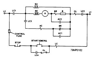
Figure 6-21.—A dc controller with one stage of acceleration.
