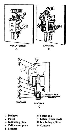
Figure 2-42.-Two ac overload relays.
