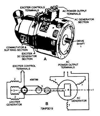
Figure 3-19.—An ac generator and schematic.
