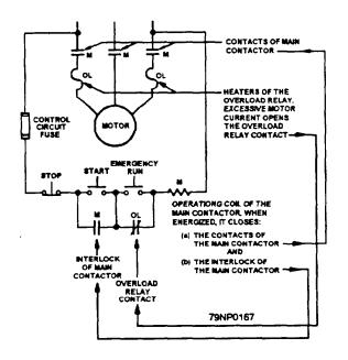
Figure 6-26.—Schematic of controller with emergency run push button.
