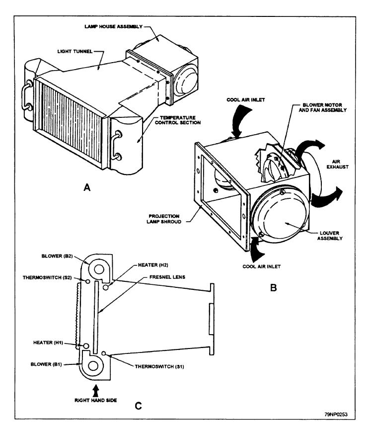
Figure 12-13.-A. Glide slope Indicator; B. Lamp house assembly; C. Temperature control section.
