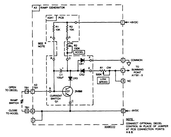
"Reprinted with permission of Woodward Governor Company, 1994" Figure 9-17.-Ramp generator schematic.
