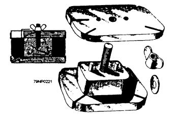
Figure 7-53.—Coil form for field coils.
