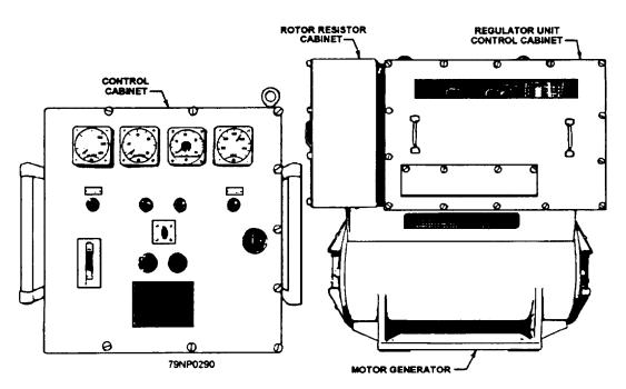
Figure 8-21.-Motor-generator set with control equipment.
