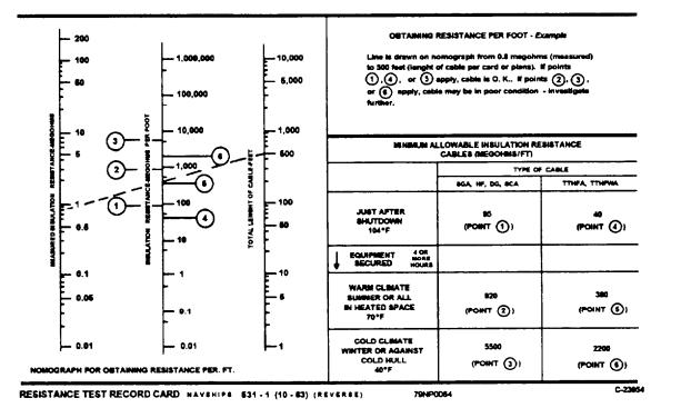
Figure 2-17.-Nomograph for obtaining resistance per foot.
