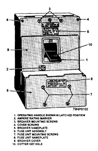
Figure 2-55.—AQB-LF250 complete circuit breaker, front view.
