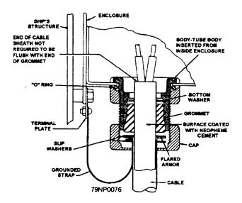
Figure 2-29.-Nylon stuffing tube grounded installation.
