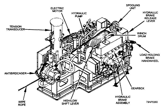
Figure 5-32.—Parts of the inhaul/outhaul winch.
