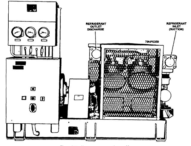
Figure 5-11.—80-ton compressor unit assembly.
