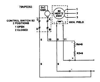
Figure 8-14.—Field-flashing circuit.
