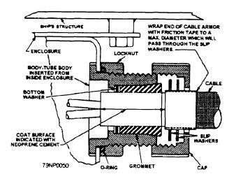
Figure 24.-Representative nylon stuffing tube installations.
