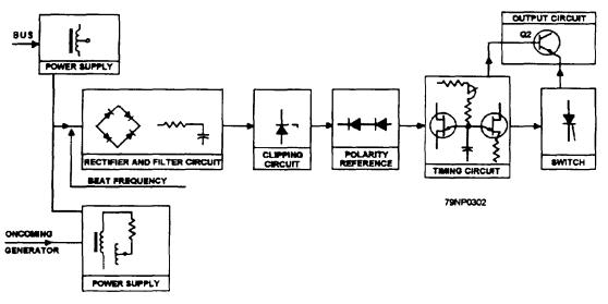
Figure 8-33.-Block diagram of frequency difference monitoring circuit.
