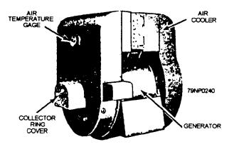
Figure 7-73.—Generator equipped with an ailr cooler.
