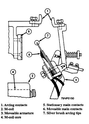
Figure 6-9.—Detailed view of arcing contacts.
