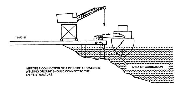
Figure 11-3.—Stray-current corrosion.
