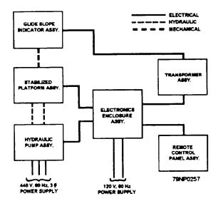
Figure 12-16.—Stabilized glide slope indicator—block diagram.
