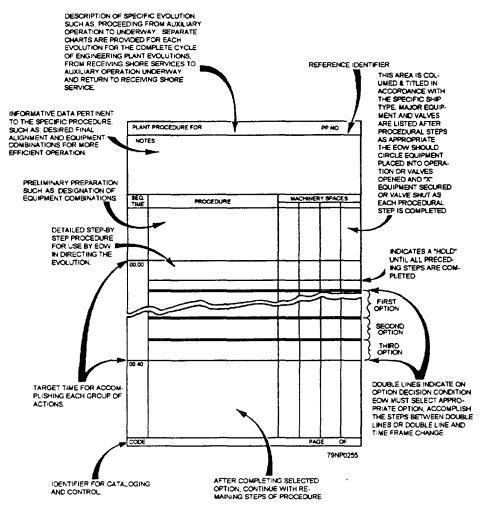
Figure 14-1.-Sample plant procedure chart.
