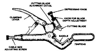
Figure 2-3.—Cable stripper.
