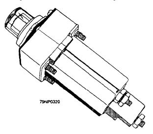
Figure 4-10.—Fuse holder with glow lamp.
