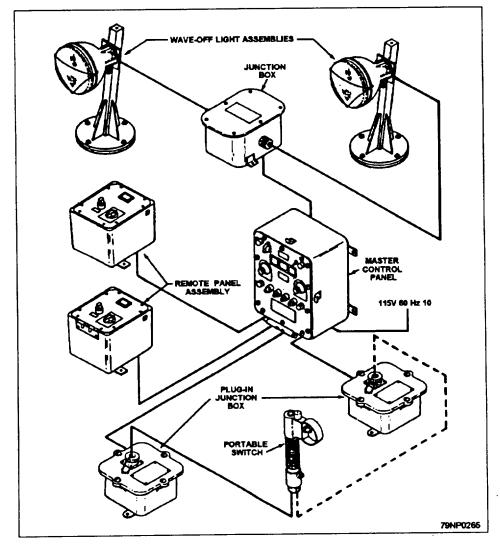
Figure 12-24.-Wave-off light system.
