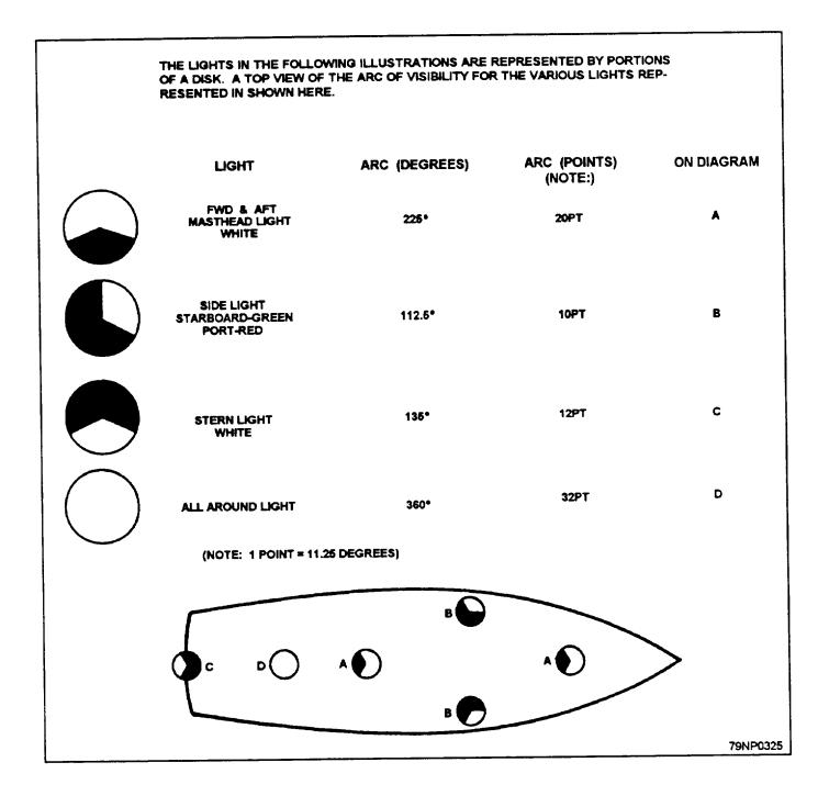
Figure 4-16.—Arc of visibility for navigation lights.
