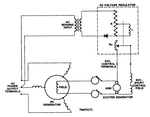
Figure 8-1.-Simplified voltage regulator circuit.
