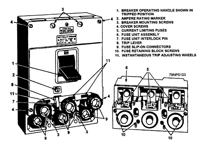
Figure 2-56.—Complete circuit breaker, front view, with fuse unit removed.
