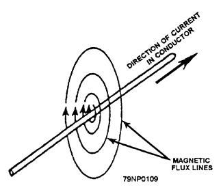
Figure 10-3.—Magnetic field around a current-carrying conductor.
