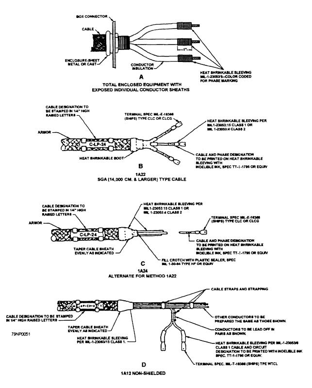
Figure 2-5.—Protecting cable ends.
