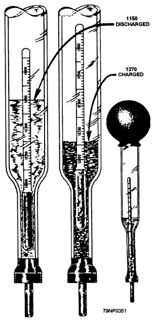
Figure 5-2.—Type-B hydrometer.
