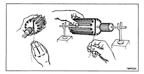
Figure 7-52.-Winding armatures by hand.
