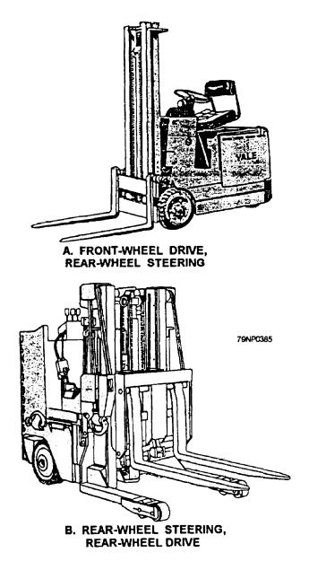
Figure 5-37.—Electric forklift trucks.
