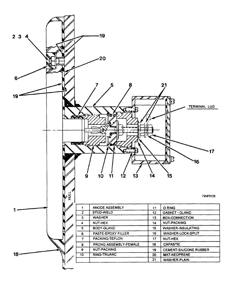
Figure 11-6.—Anode assembly.
