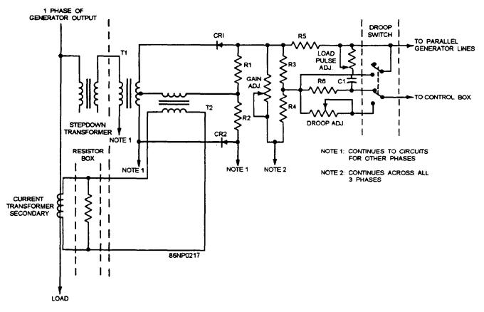
Figure 9-10.-Load signal box, simplified Schemstic.
