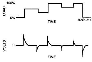
Figure 9-11.—Comparison of load pulse signals to load changes.
