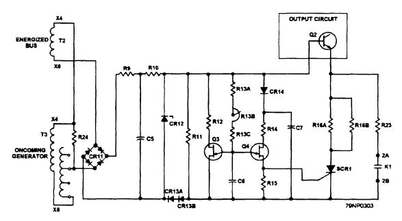
Figure 8-34.—Schematic diagram of frequency difference monitoring circuit.
