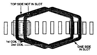
SECOND COIL OF WINDING IN PLACE
