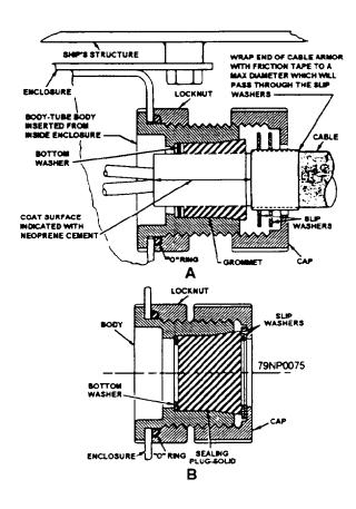
Figure 2-28.—Representative nylon stuffing tube installations.
