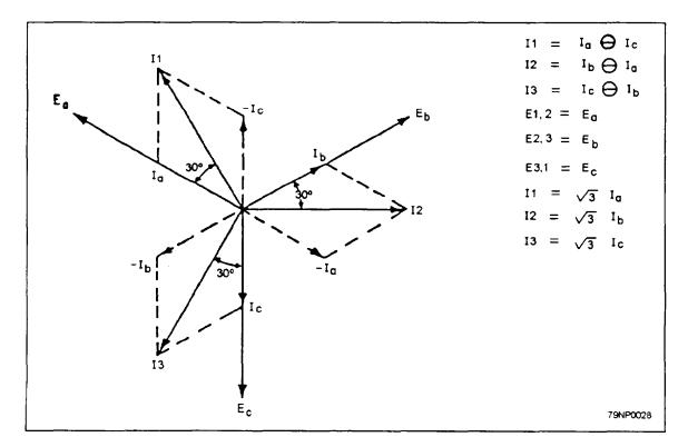
Figure 3-28.-Three-phase delta/connected system.
