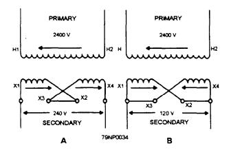
Figure 3-34.-Single-phase transformer connections.
