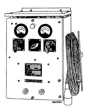
Figure 5-3.—Front view of Battery charger, model 24-302-BN-1.
