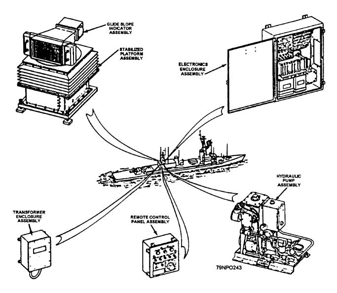
Figure 12-3.-Stabilized glide slope indicator system
