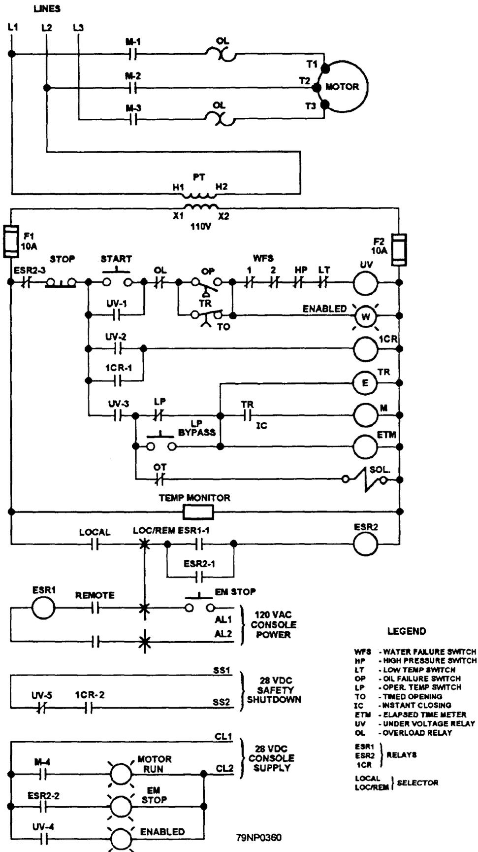
Figure 5-12.—80-ton air-conditioning compressor wiring diagram.
