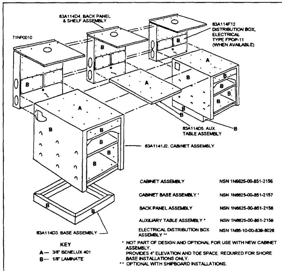
Figure 1-4.—A typical electric workbench.
