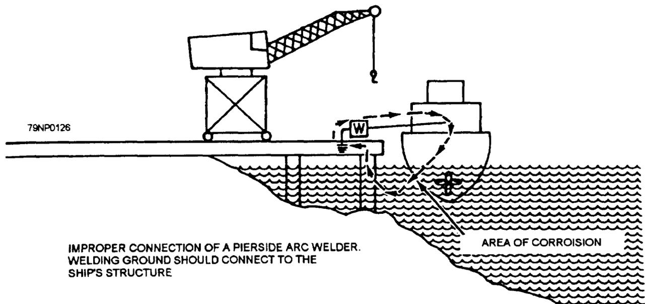
Figure 11-3.—Stray-current corrosion.
