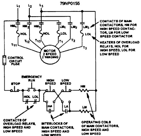
Figure 6-14.—Two-speed, ac controller.
