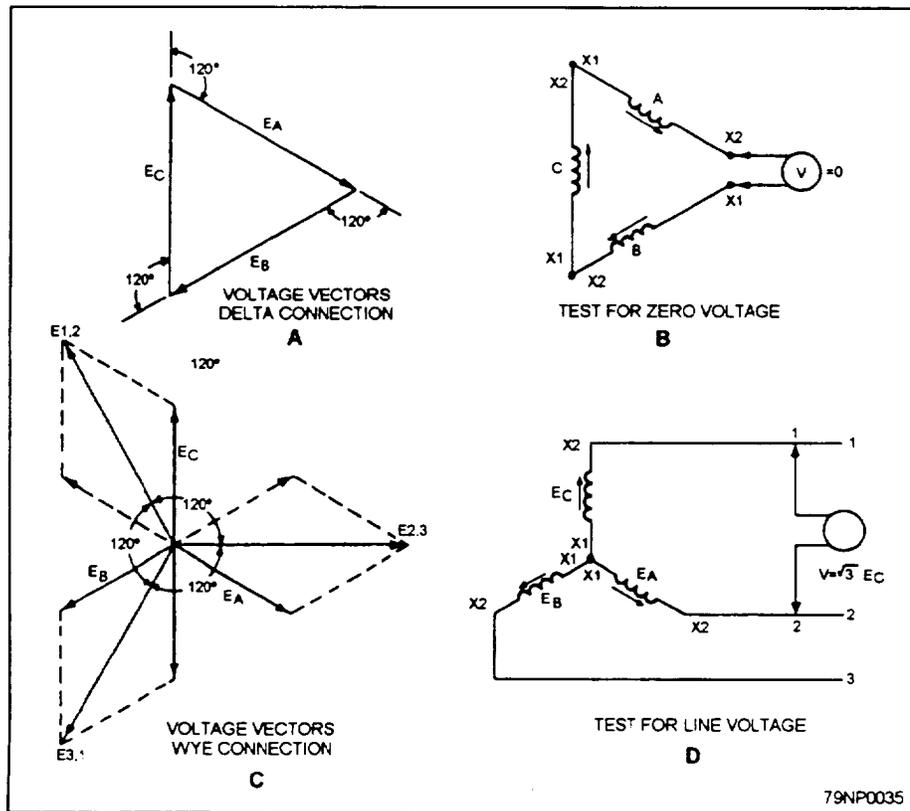
Figure 3-35.—Delta-connected transformer secondaries.
