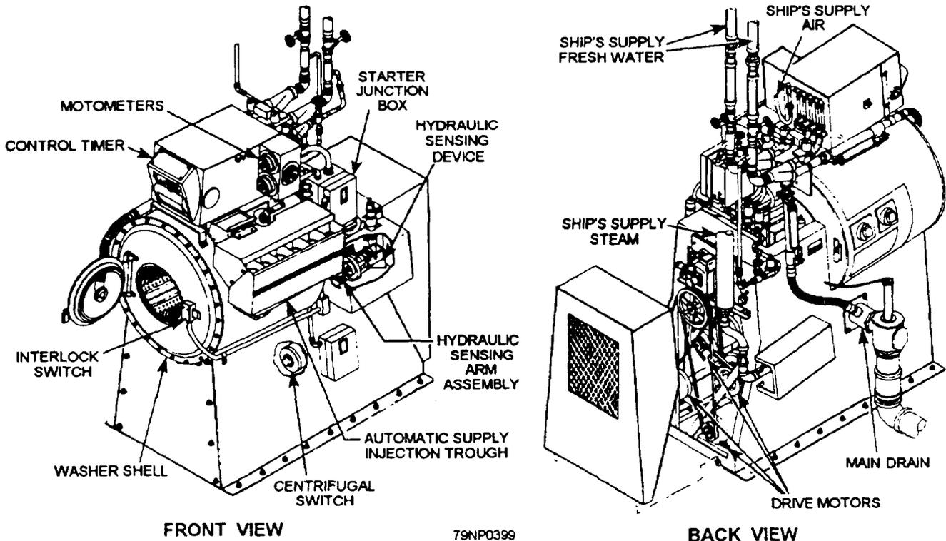
Figure 5-51.—A typical washer-extractor installation.
