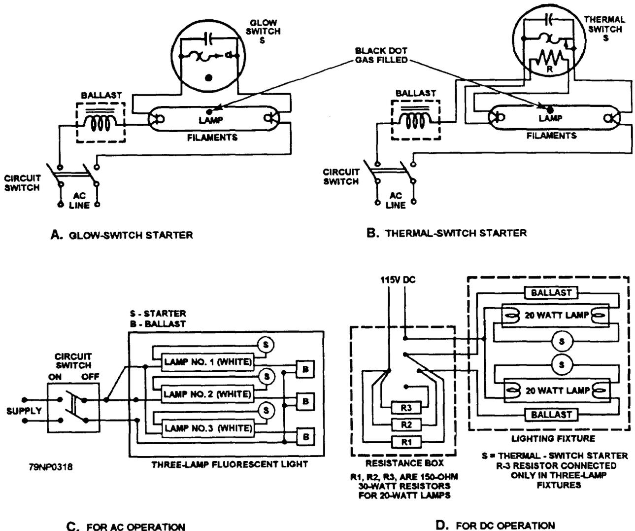
Figure 4-8.—Fluorescent lamps with auxiliary equipment.
