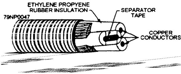
Figure 2-1.—Construction of low-smoke cable (typical).
