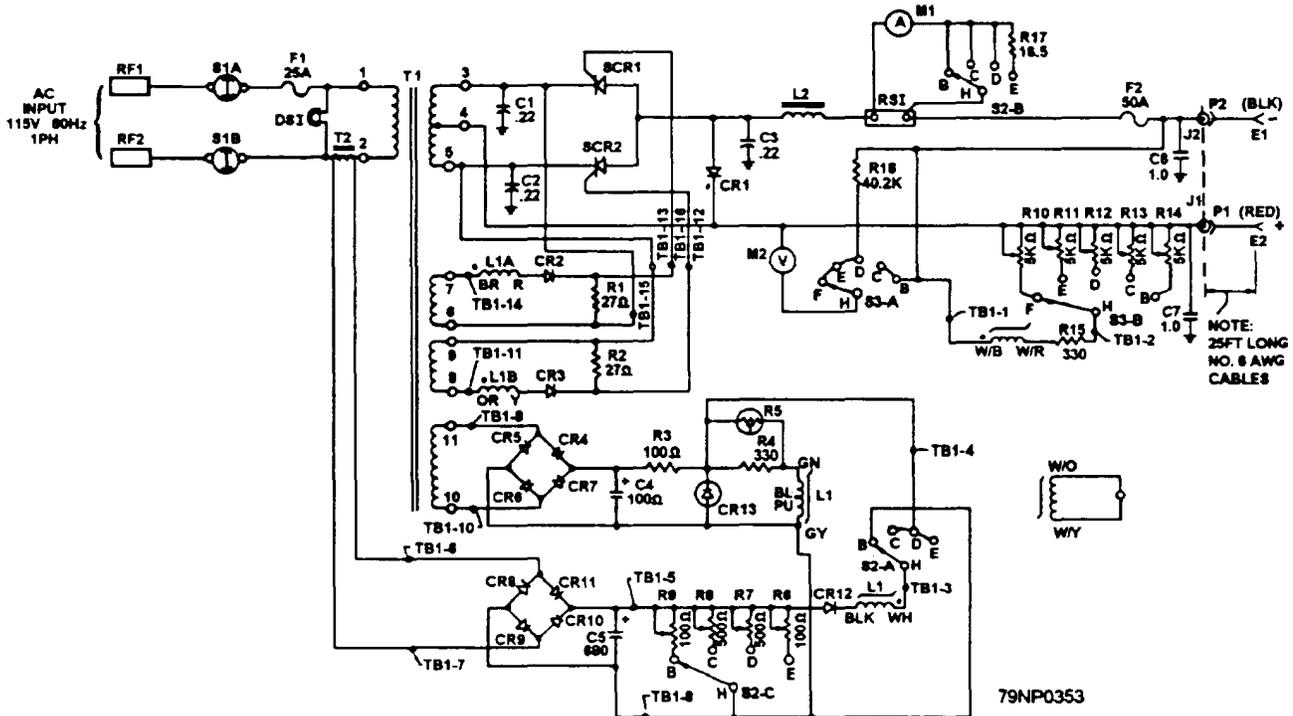
Figure 5-4—Battery charger wiring diagram.
