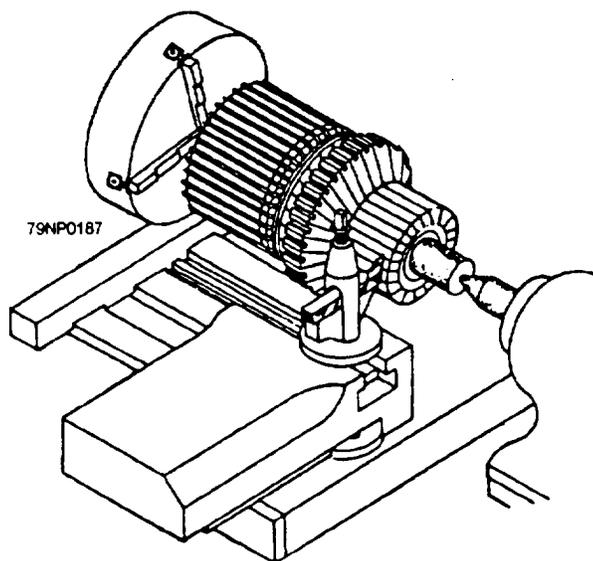
Figure 7-17.—Truing a commutator by turning.
