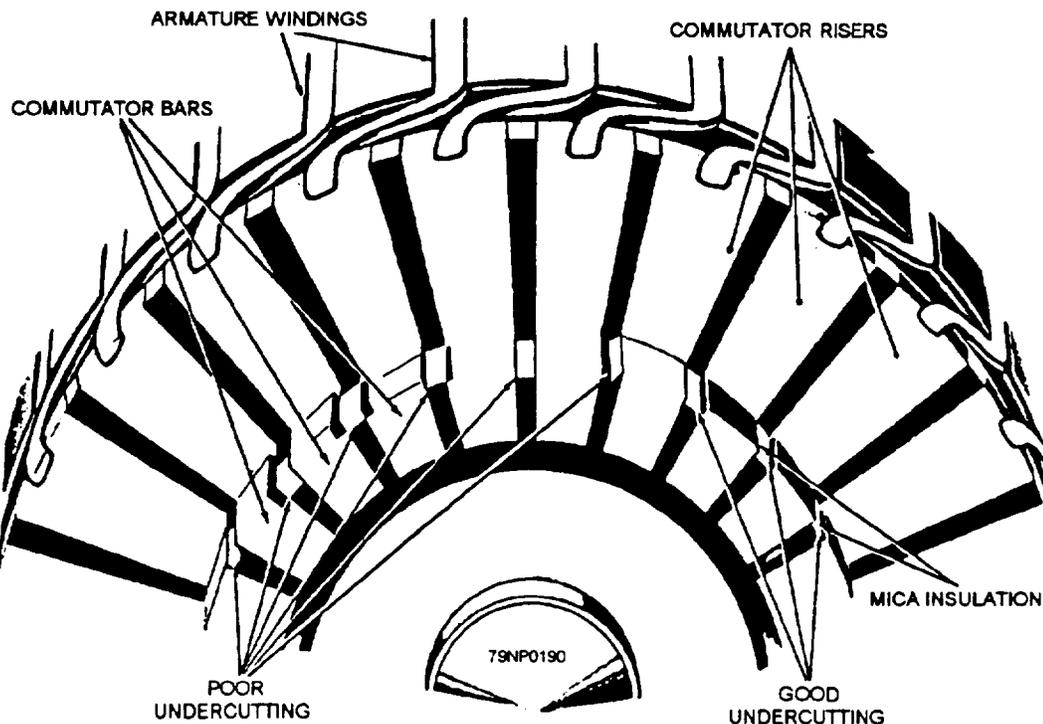
Figure 7-20.—Example of good and poor undercutting.
