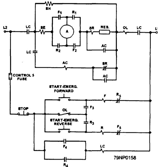
Figure 6-17.—Reversing dc controller.
