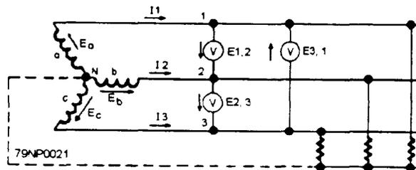
Figure 3-21.—Three-phase, ac generator showing neutral connection.
