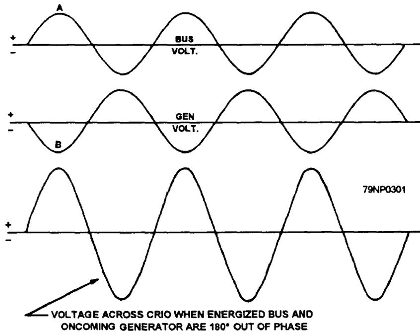
Figure 8-32.—Input voltage to CR10 ( $180^\circ$  out of phase).
