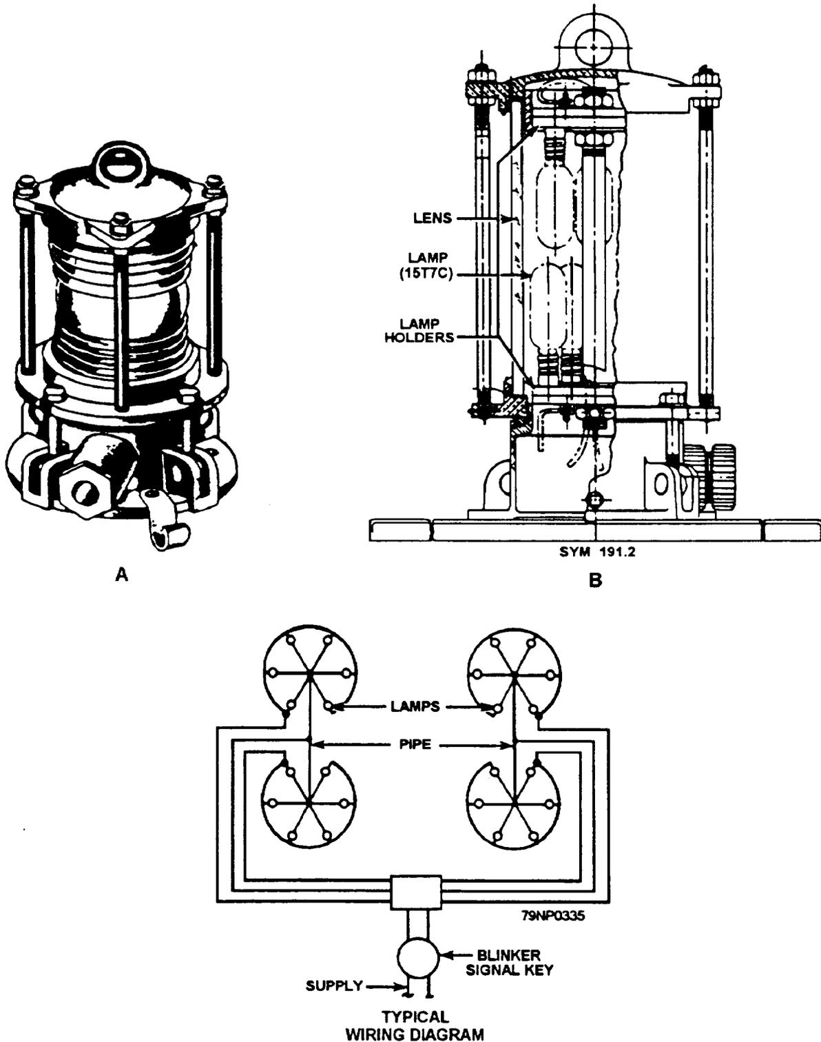
Figure 4-26.—Blinker light fixture.
