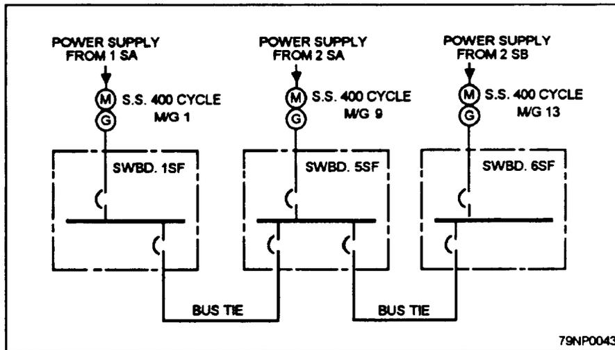
Figure 3-43.—Bus tie connections on 400-hertz ship's service system.
