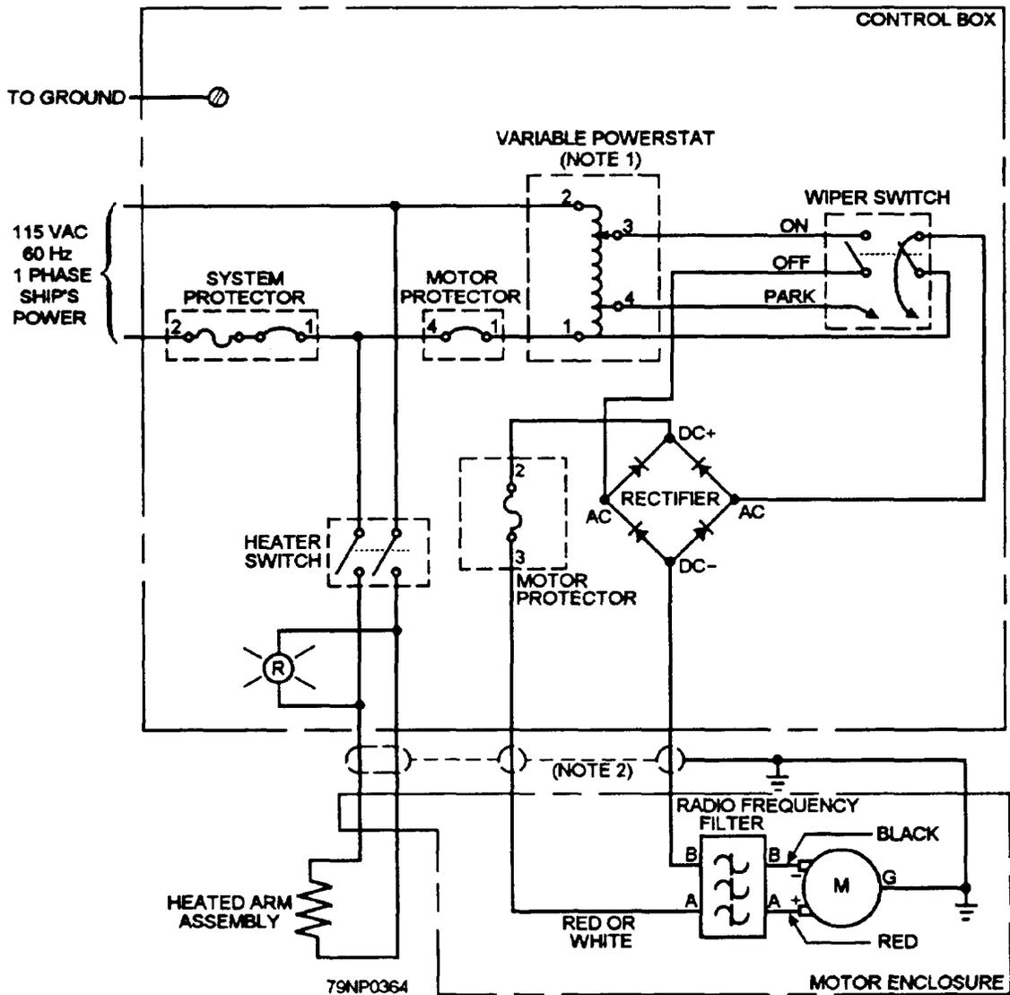
Figure 5-16.—Window wiper schematic.
