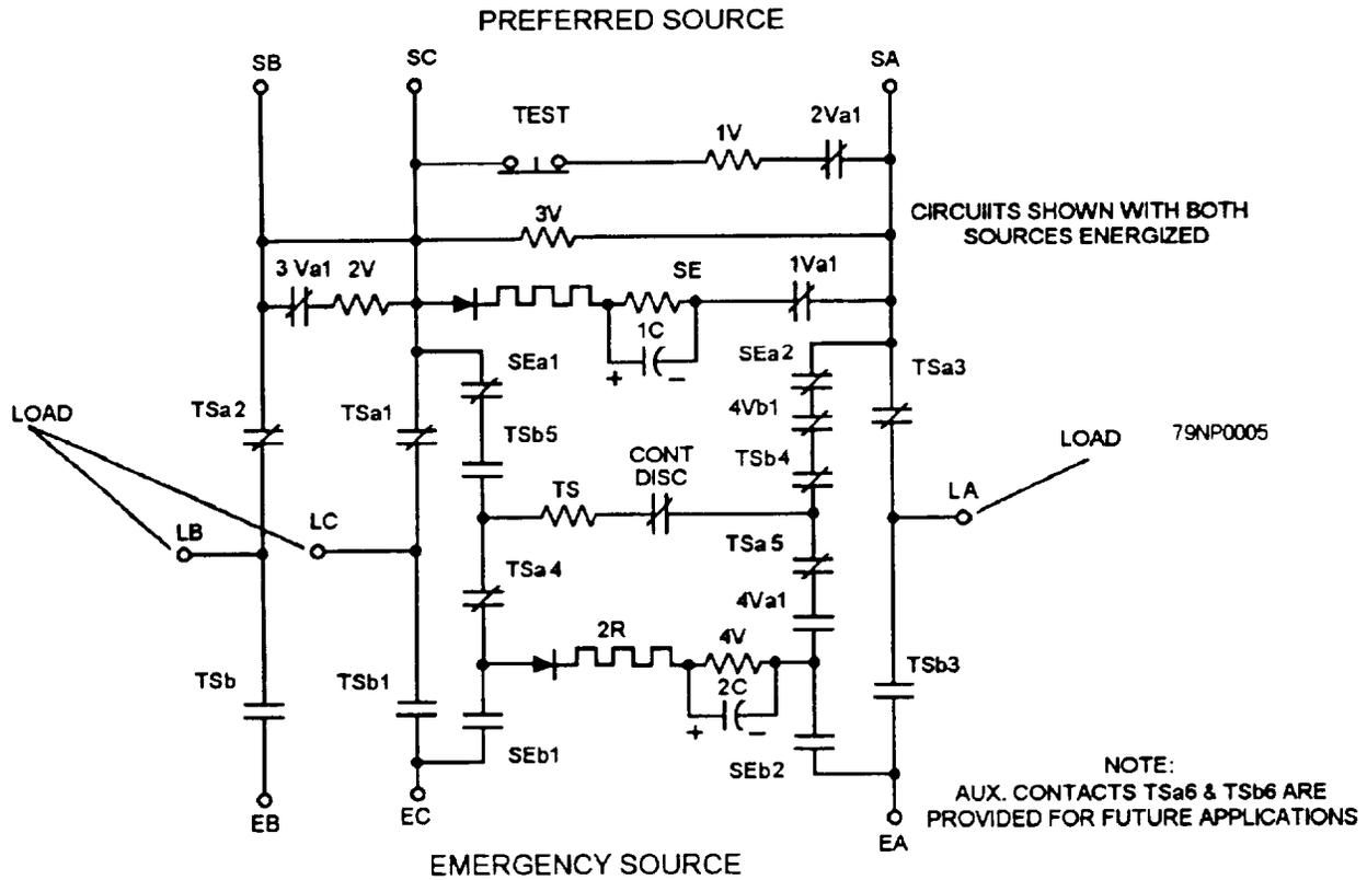
Figure 3-5.—Schematic diagram of the A-2 ABT.
