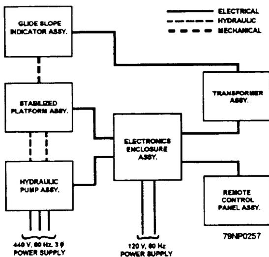
Figure 12-16.—Stabilized glide slope indicator—block diagram.
