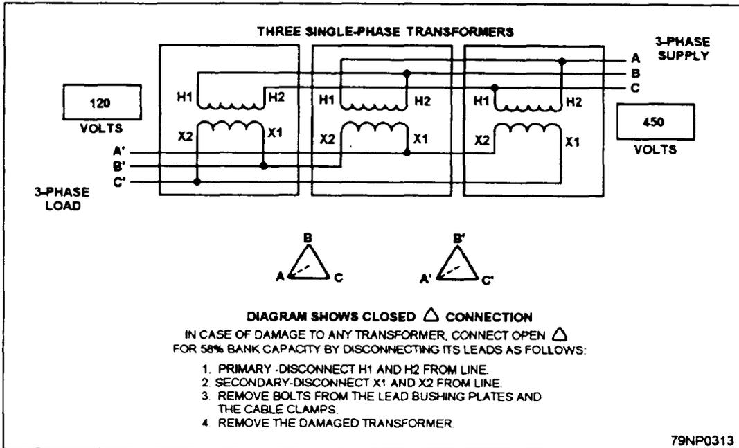
Figure 4-3.—Delta-delta transformer connections.
