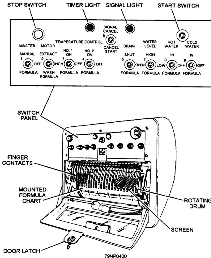
Figure 5-52.—A typical automatic control timer.
