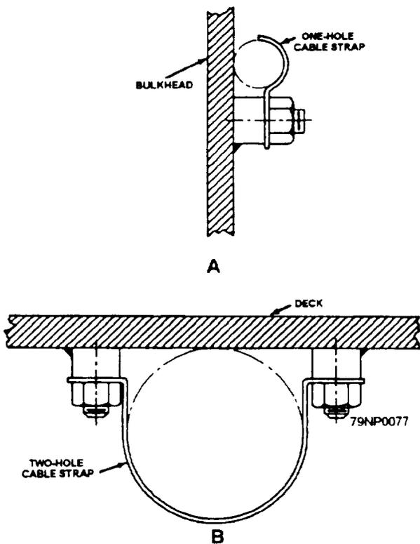
Figure 2-30.—Single cable strap application.
