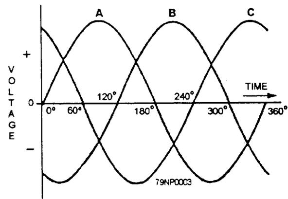
Figure 3-3.—Sine curve for three-phase circuit.
