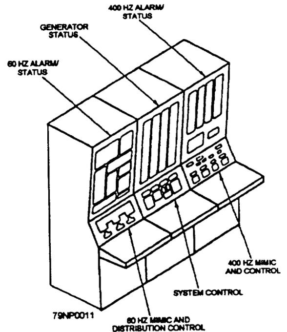
Figure 3-11.—Electric plant control console (EPCC).
