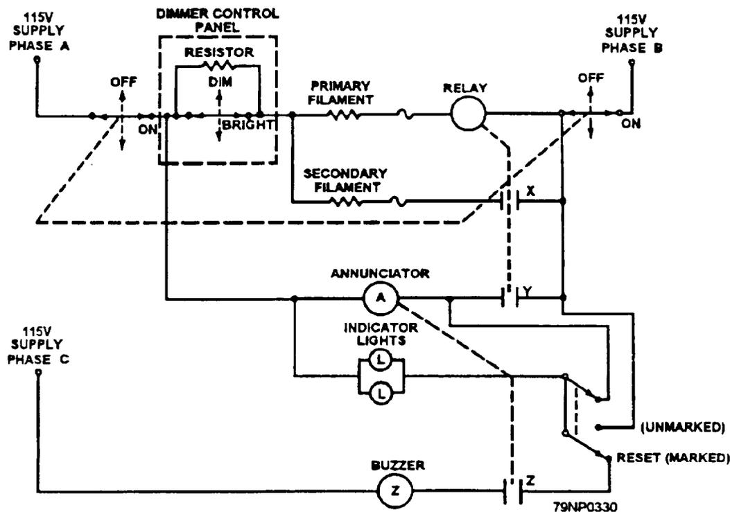
Figure 4-21.—Running light, supply, control, and telltale panel schematic diagram.
