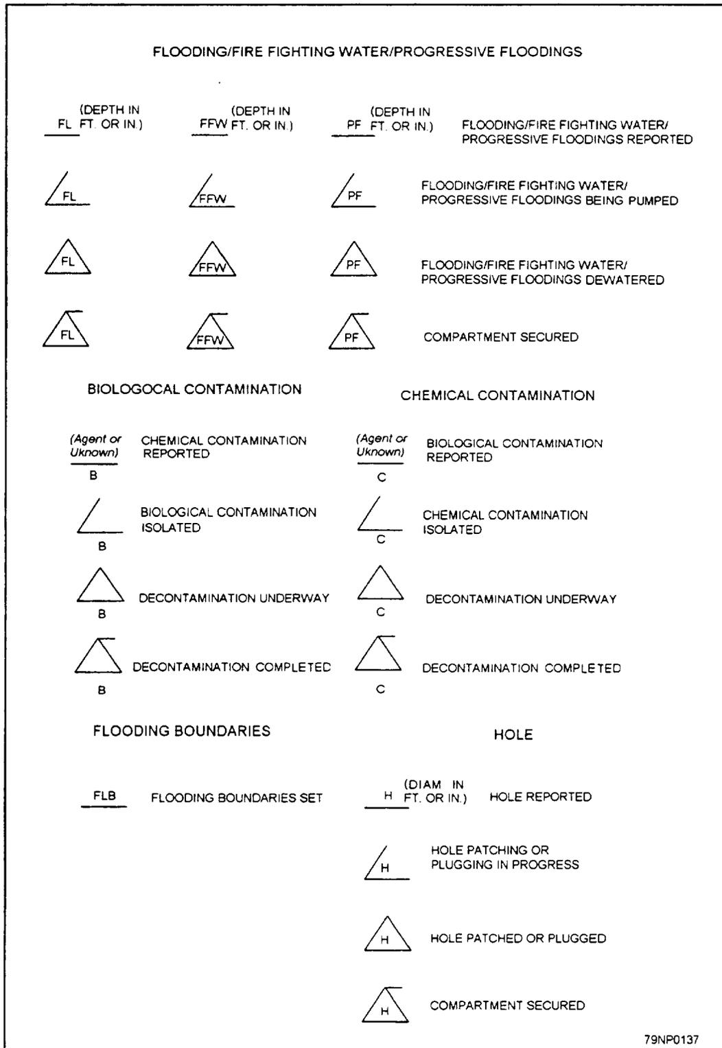
Figure 14-7.—Navy standard damage control symbology.
