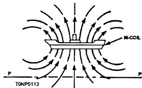
Figure 10-7.—Magnetic field produced by the M coil.
