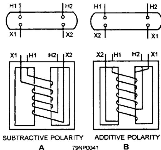
Figure 3-41.—Polarity markings for large transformers.
