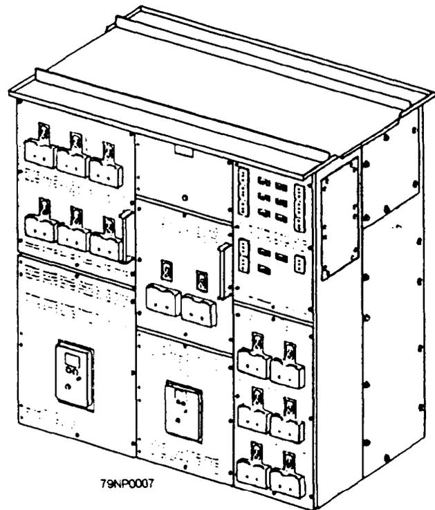
Figure 3-7.—1SA Ship's service switchboard.
