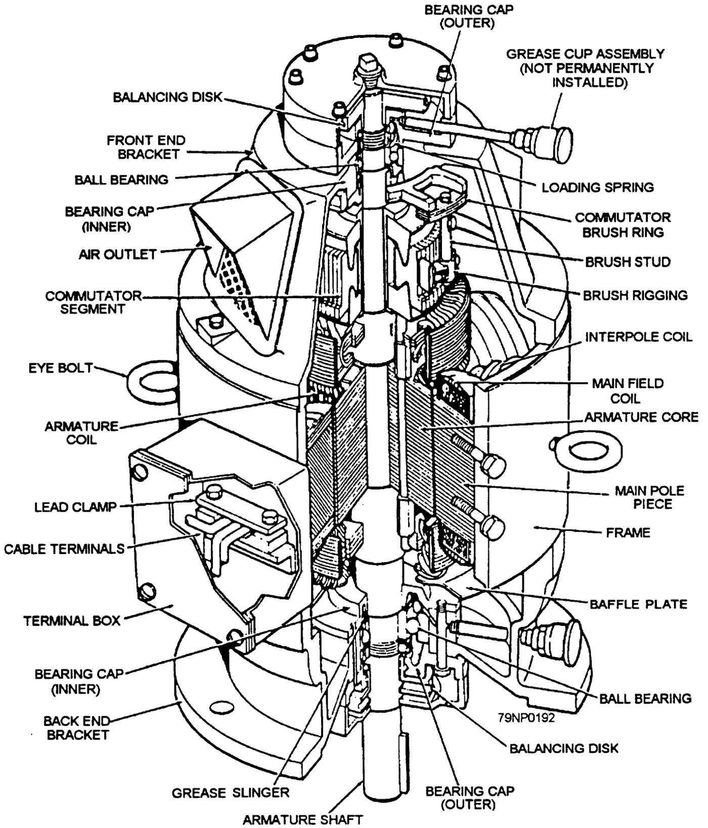
Figure 7-22.—Typical dc Motor.
