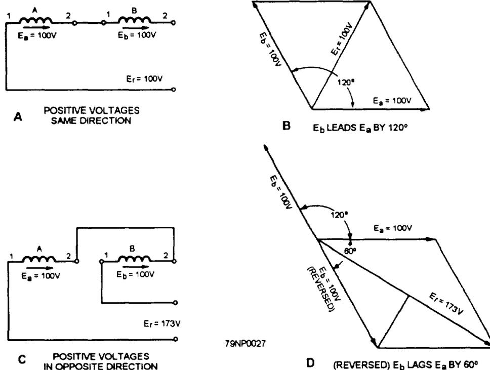
Figure 3-27.—Vector analysis of voltage in series aiding and opposing.
