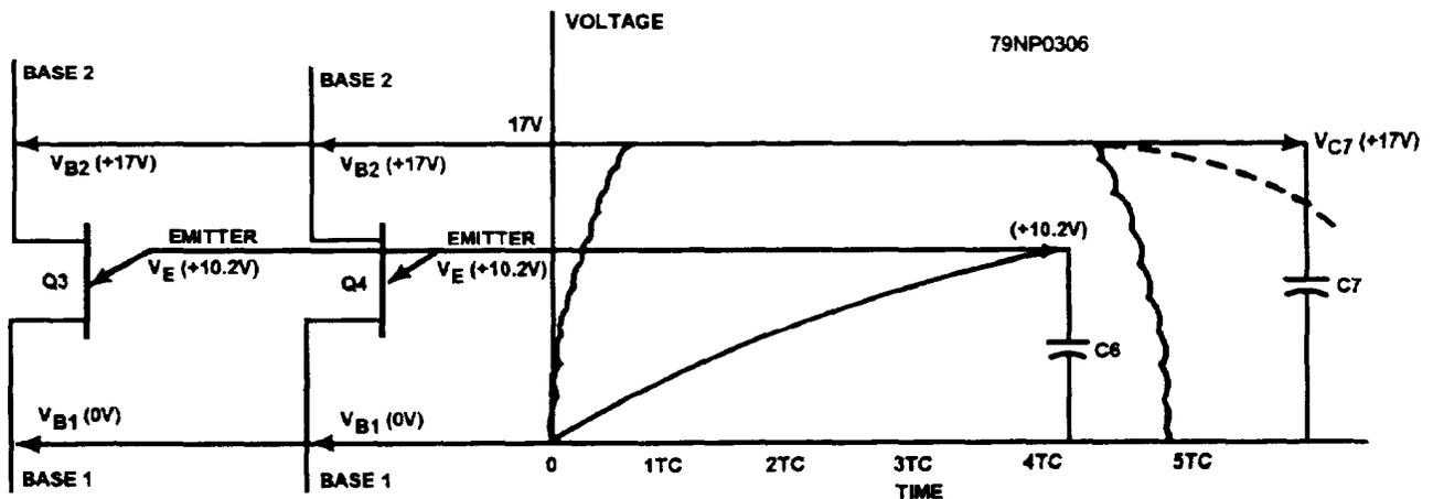
Figure 8-37.—Firing sequence for Q4.
