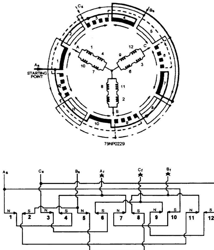
Figure 7-62.—Three-phase, four-pole, parallel-wye winding.
