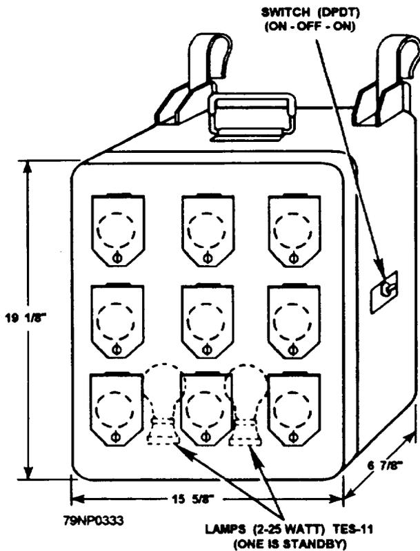
Figure 4-24.—Station marker box, symbol 285.
