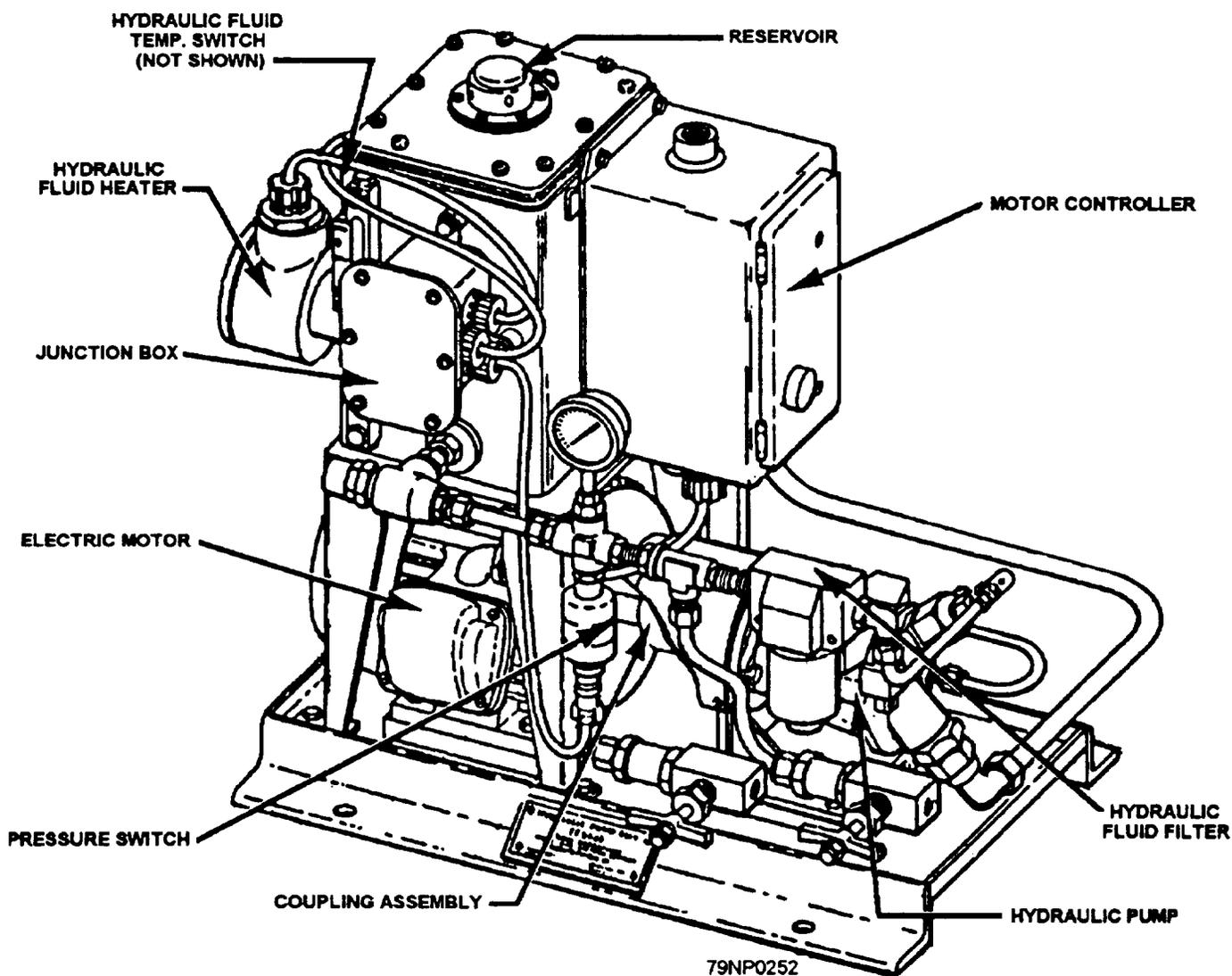
Figure 12-12.—Hydraulic pump assembly.
