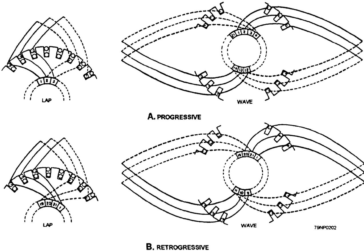
Figure 7-33.—Meaning of coil pitch in armature winding.
