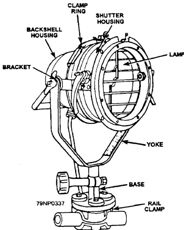
Figure 4-28.—An 8-inch, 60-hertz, sealed-beam searchlight.
