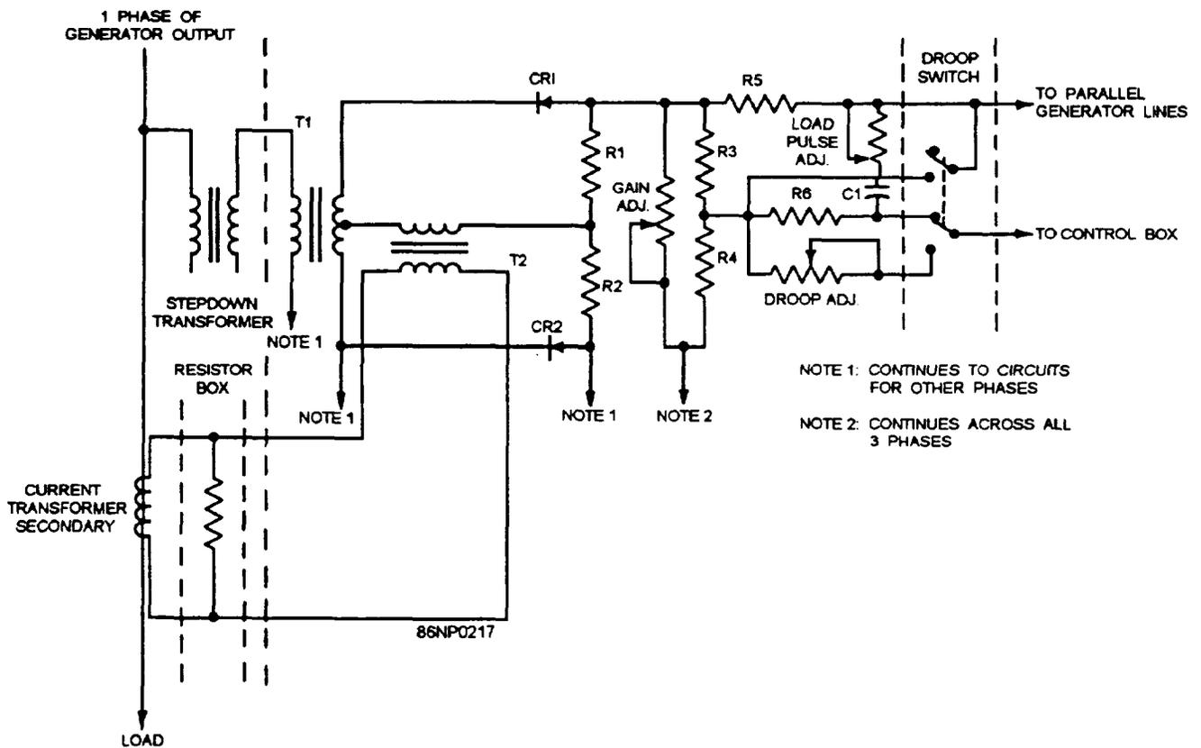
Figure 9-10.—Load signal box, simplified Schematic.
