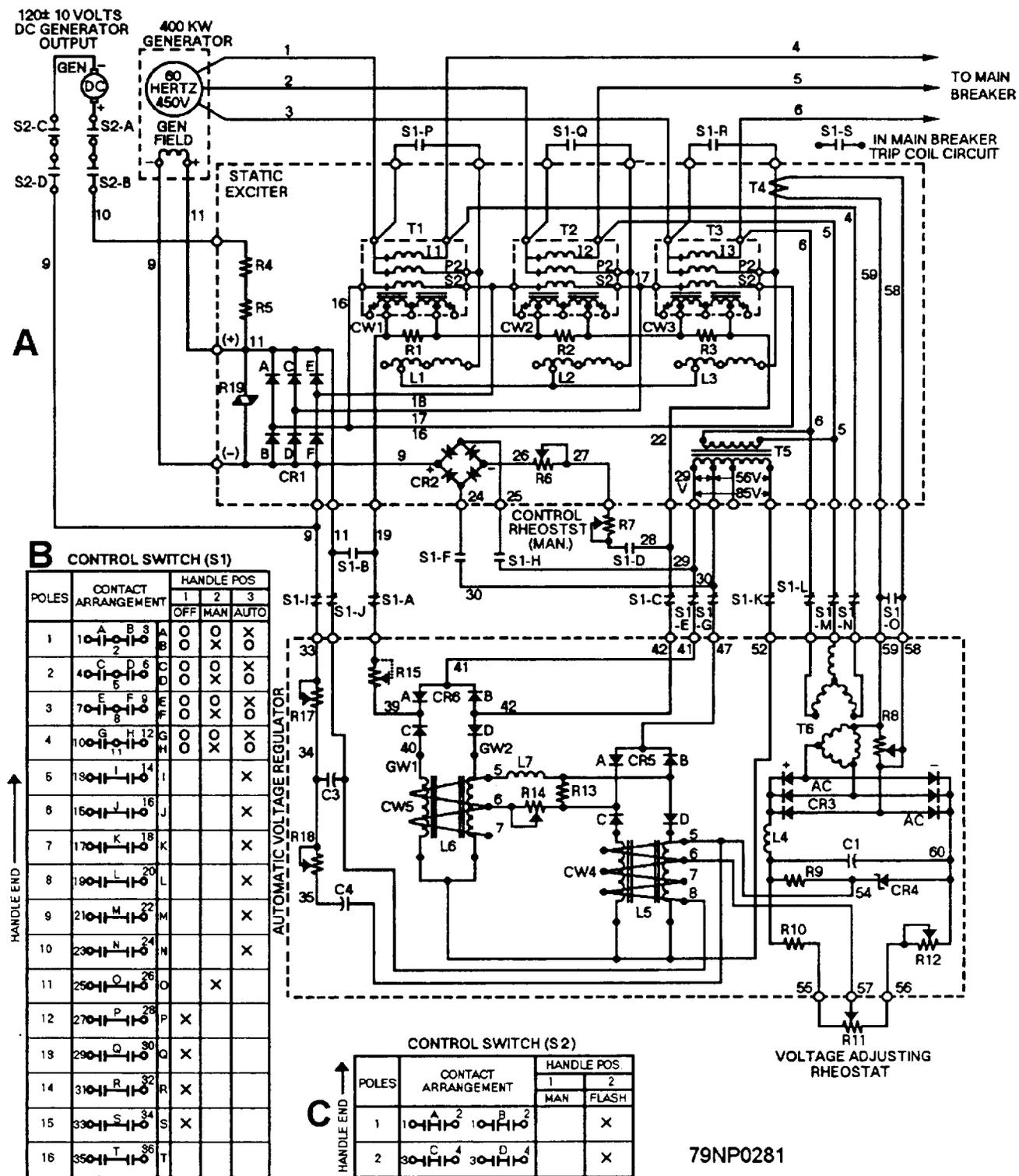
Figure 8-12.—Elementary diagram of static excitation voltage regulator system.
