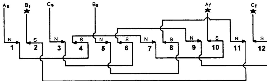
Figure 7-60.—Three-phase, four-pole, series-wye winding.
