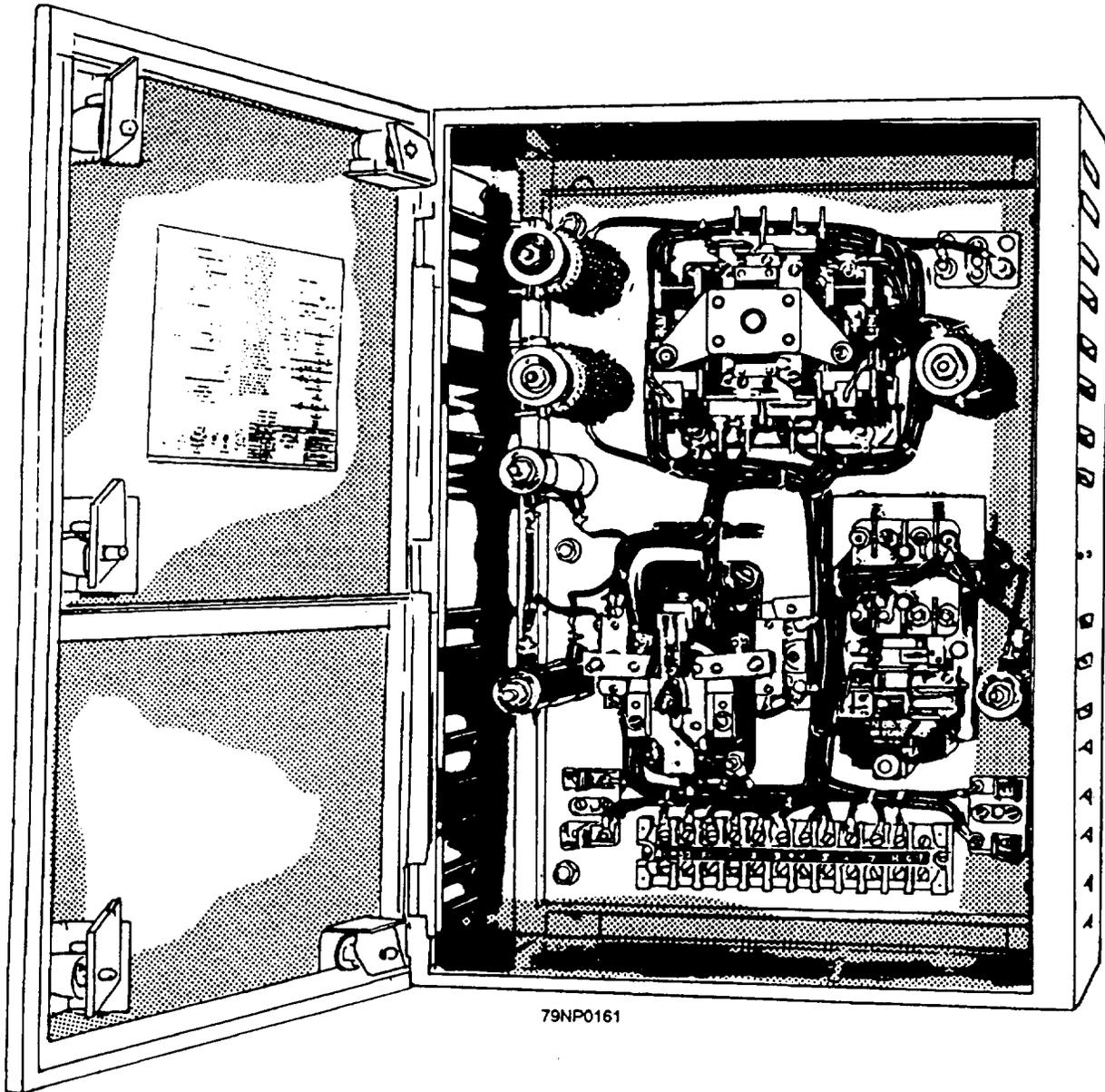
Figure 6-20.—A typical dc controller.
