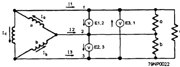
Figure 3-22.—Three-phase, delta-connected system.
