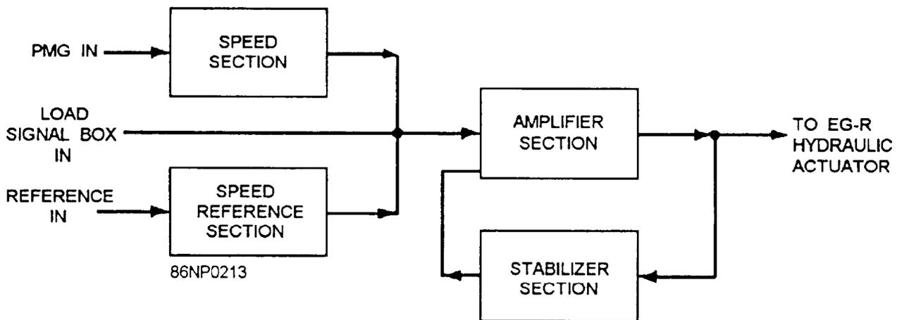
Figure 9-6.—EG-M control box, block diagram.
