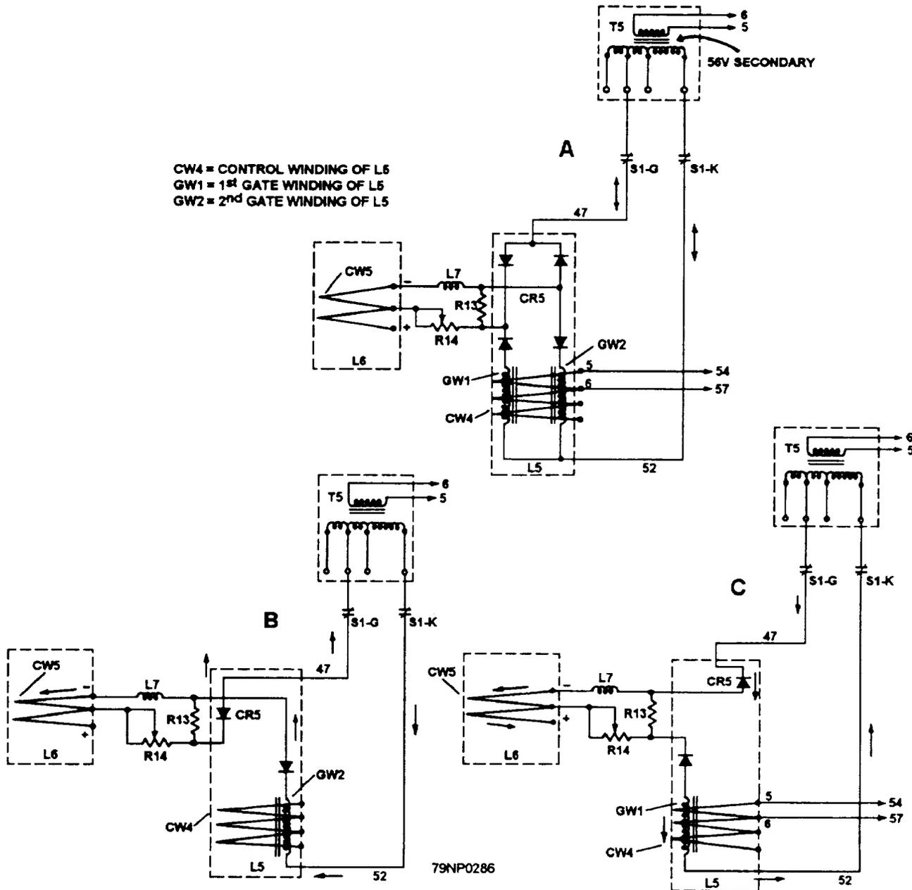
Figure 8-17.—First-stage magnetic amplifier.
