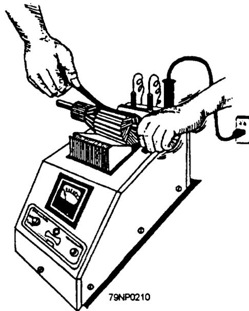
Figure 7-41.—Checking armature shorts with a growler.
