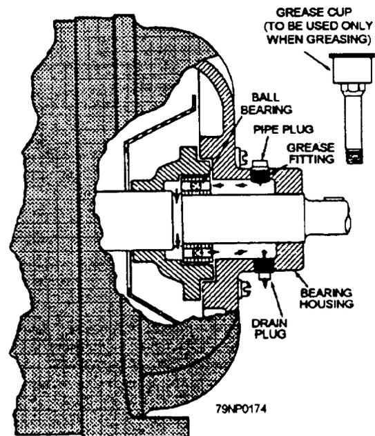
Figure 7-3.—Grease-lubricated ball bearings.
