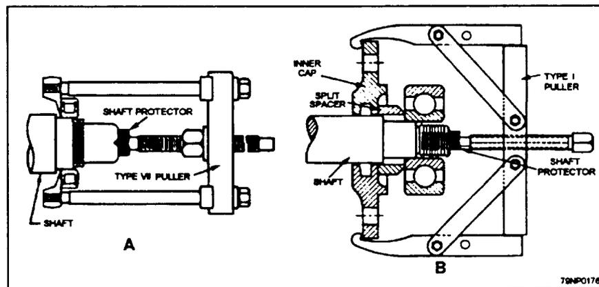
Figure 7-5.—Bearing pullers.
