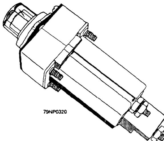
Figure 4-10.—Fuse holder with glow lamp.
