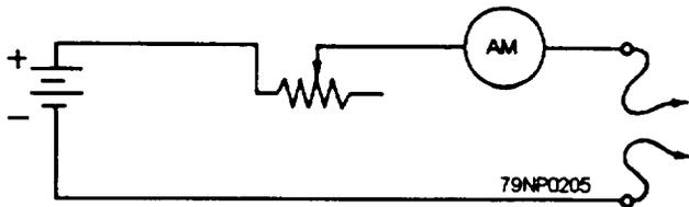
Figure 7-36.—Test circuit for measuring armature resistance.
