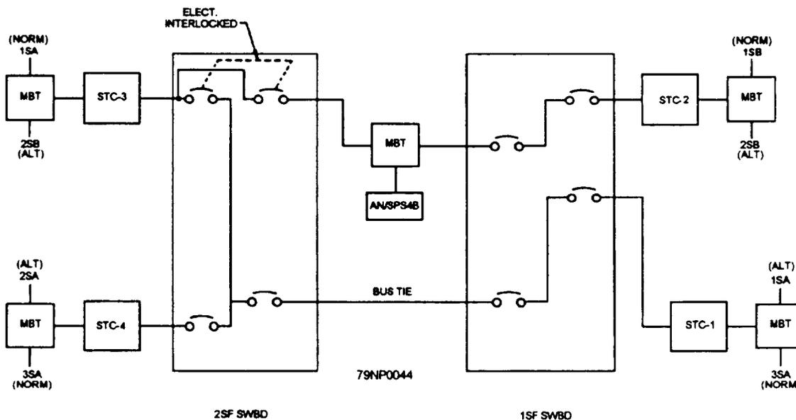
Figure 3-44.—400Hz electric power distribution system aboard a new DDG.
