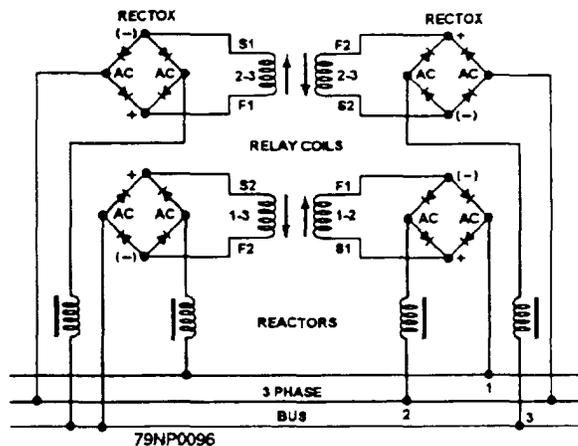
Figure 2-19.—Schematic wiring of a phase-failure relay.
