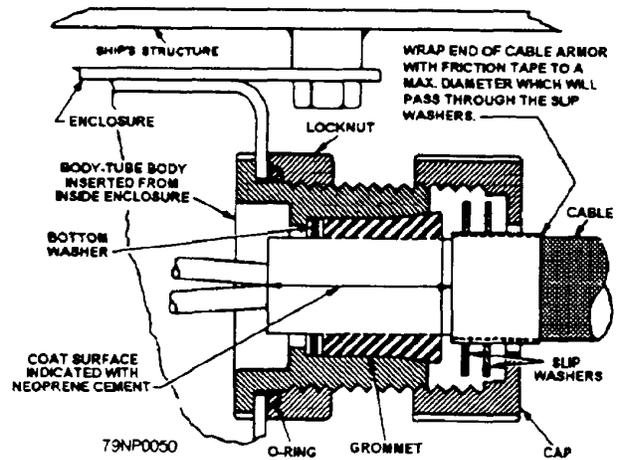
Figure 24.—Representative nylon stuffing tube installations.
