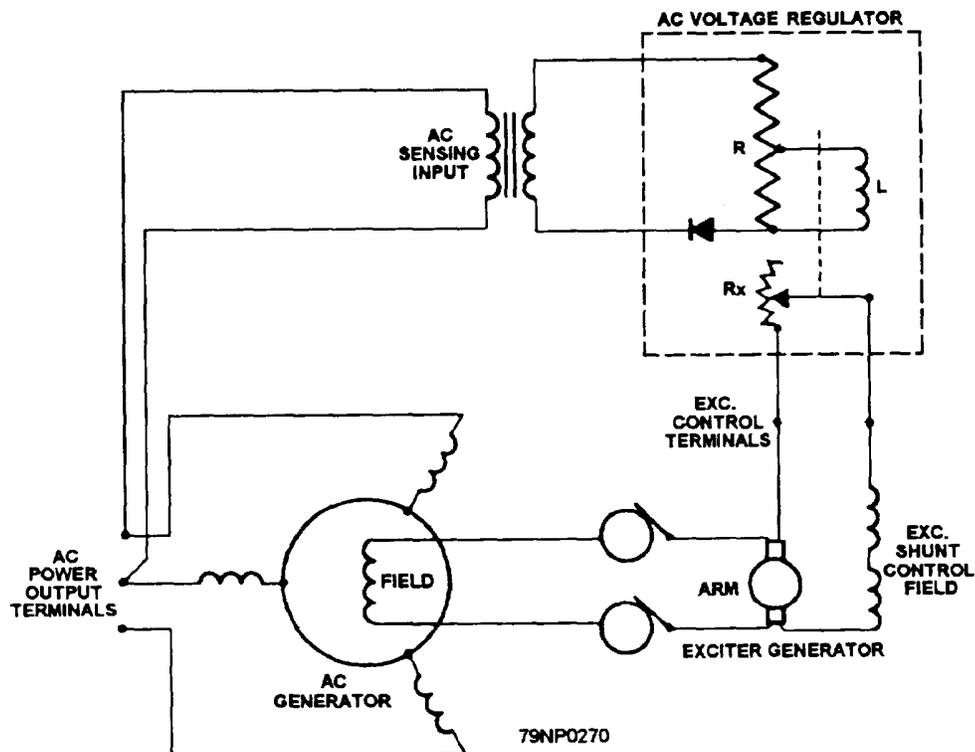
Figure 8-1.—Simplified voltage regulator circuit.
