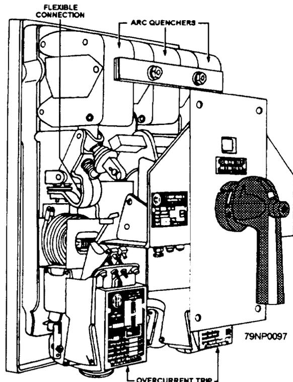
Figure 2-50.—Type ACB circuit breaker.
