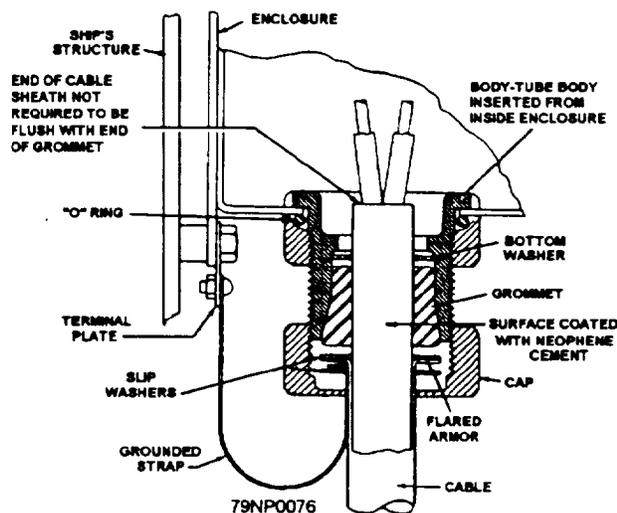
Figure 2-29.—Nylon stuffing tube grounded installation.
