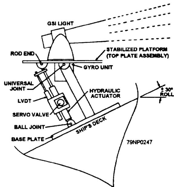
Figure 12-7.—Stabilized platform assembly-functional diagram.
