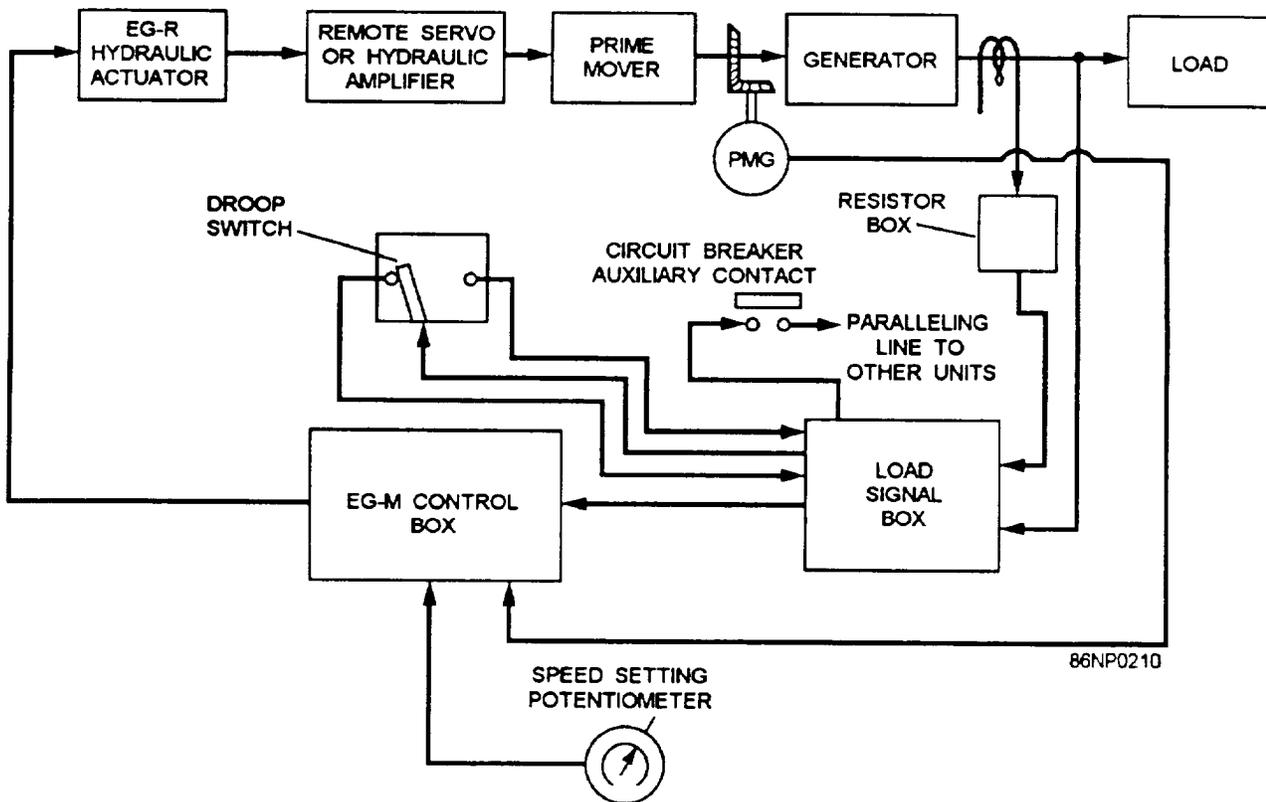
Figure 9-3.—Electrohydraulic load-sensing governor system, block diagram.
