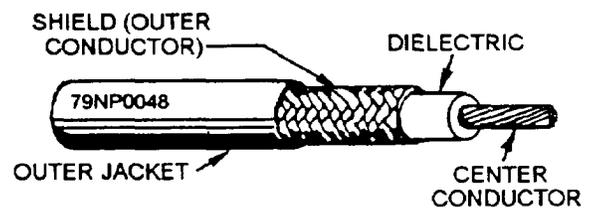
Figure 2-2—Construction of flexible RF transmission line.
