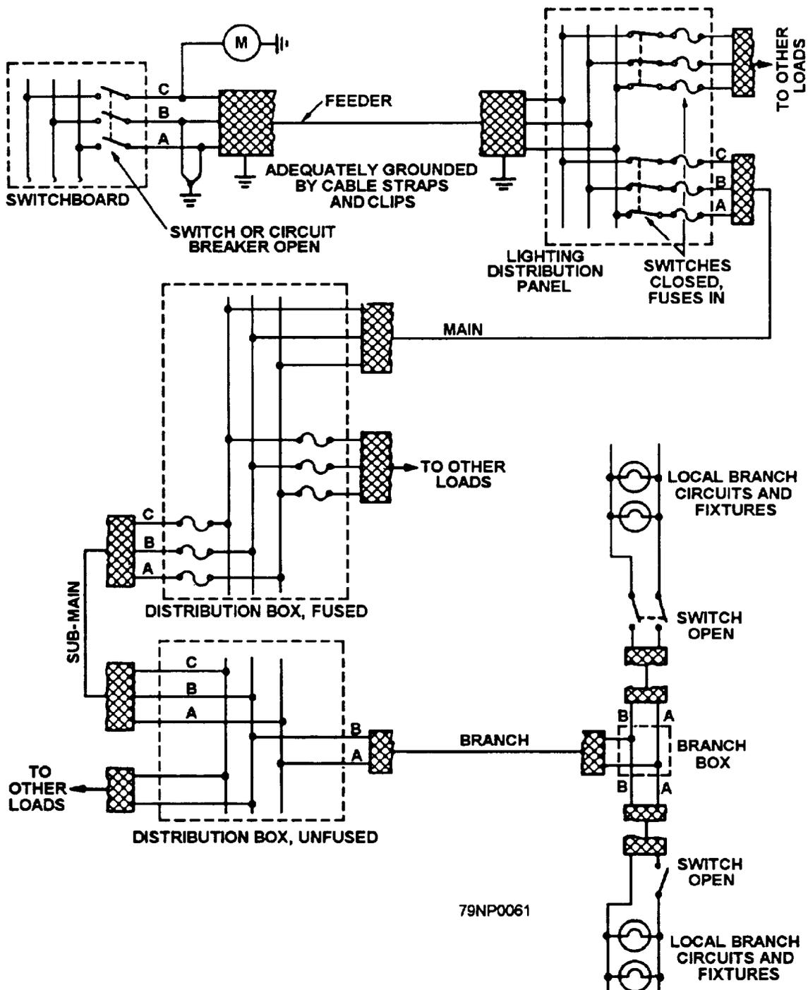
Figure 2-14.—Measuring insulation resistance of a lighting circuit.
