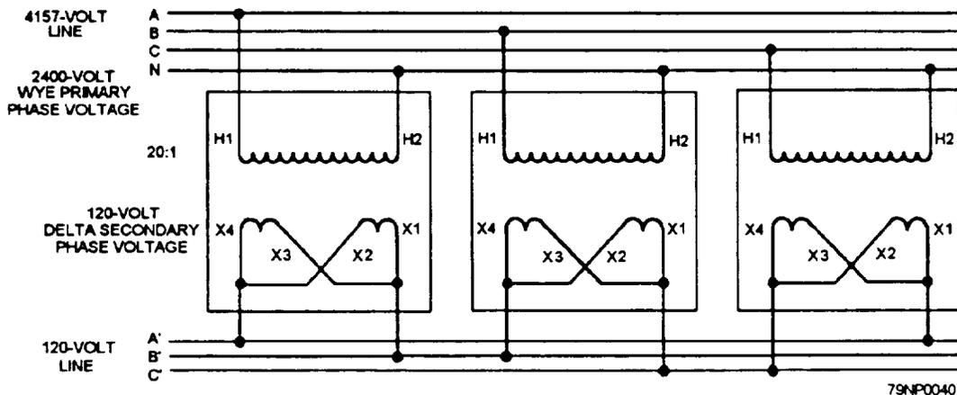
Figure 3-40.—Wye-delta transformer connections.
