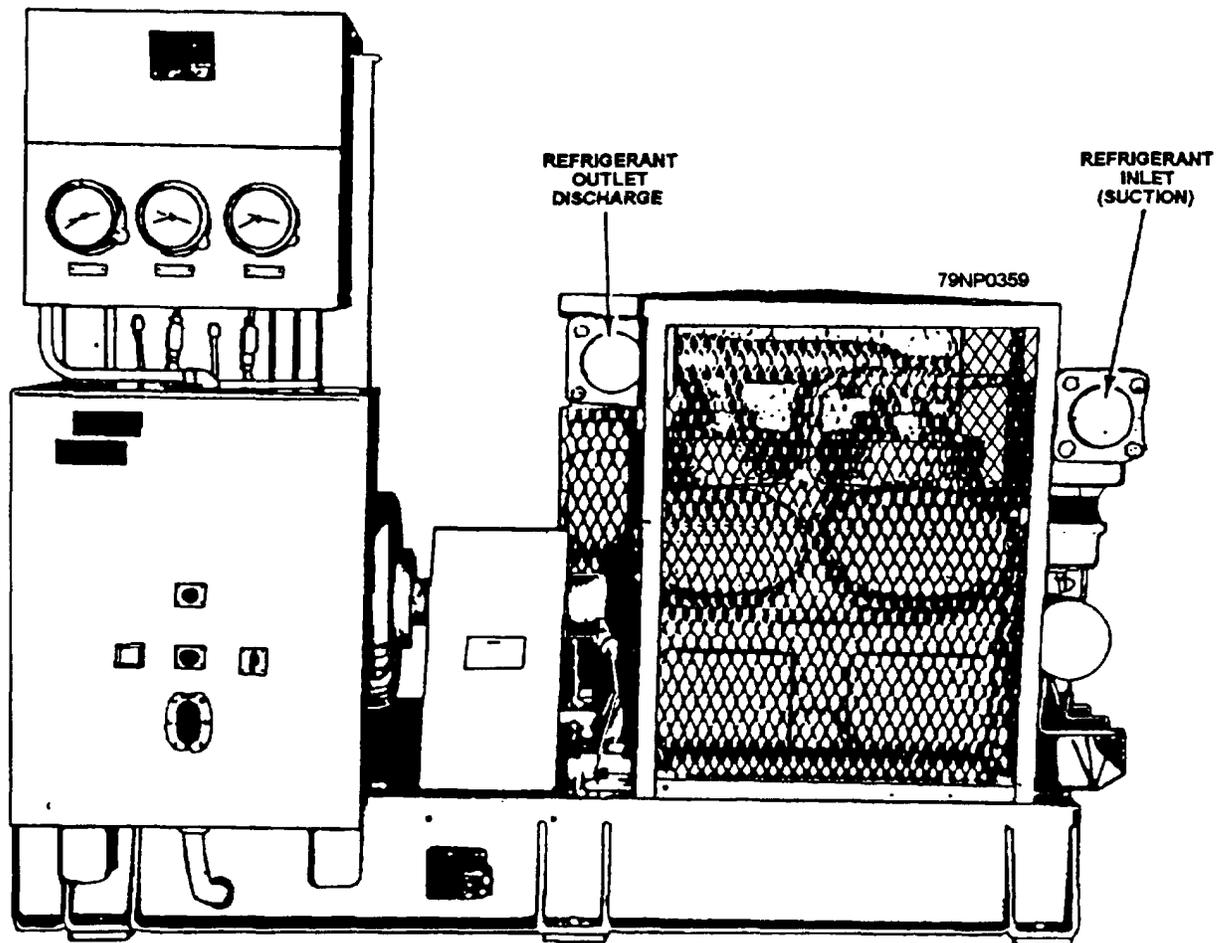
Figure 5-11.—80-ton compressor unit assembly.
