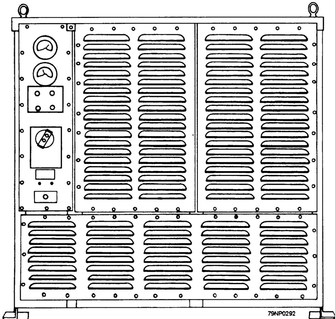
Figure 8-23.—Static converter, front view.
