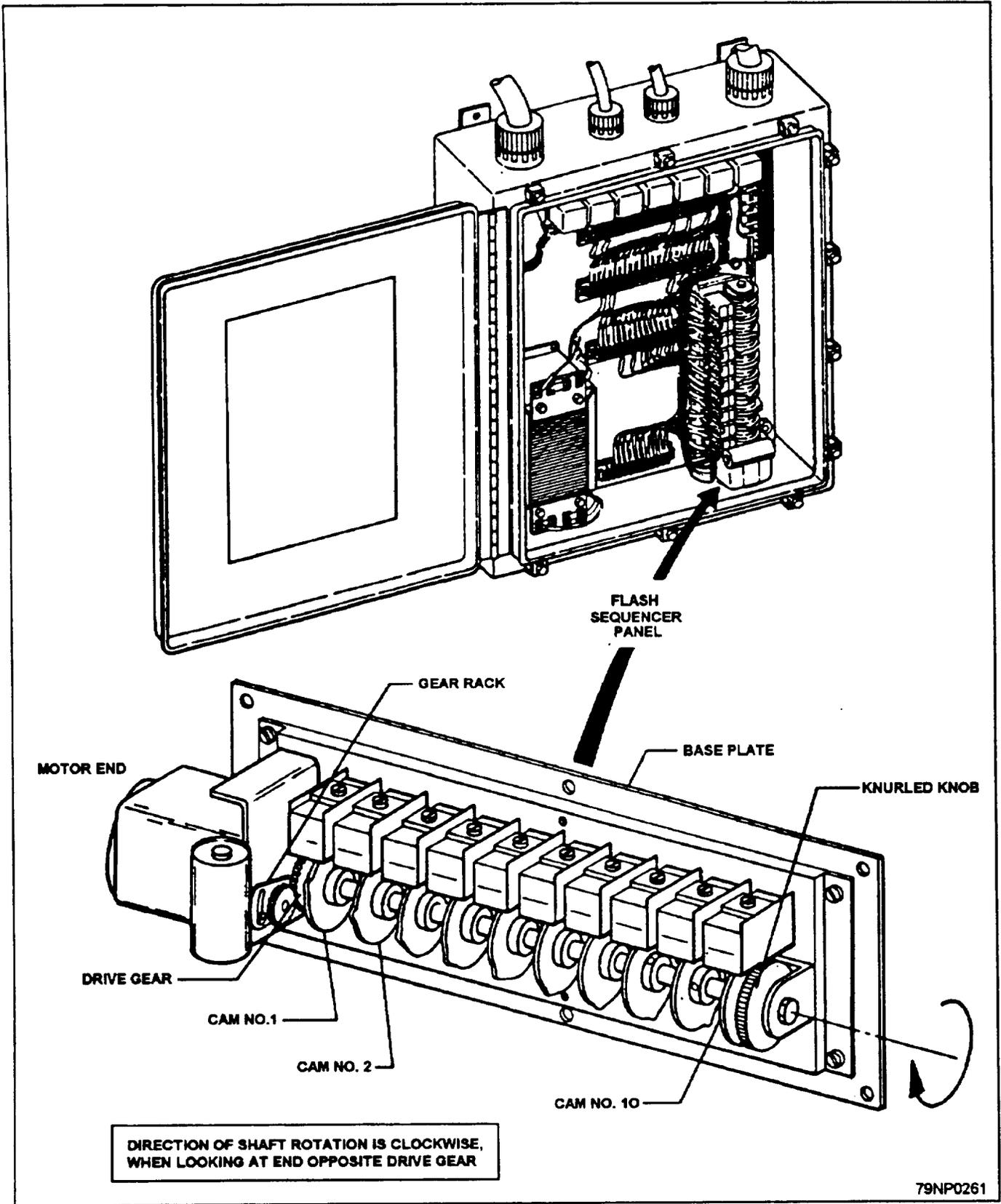
Figure 12-20.—Flash sequencer panel and timer assembly.
