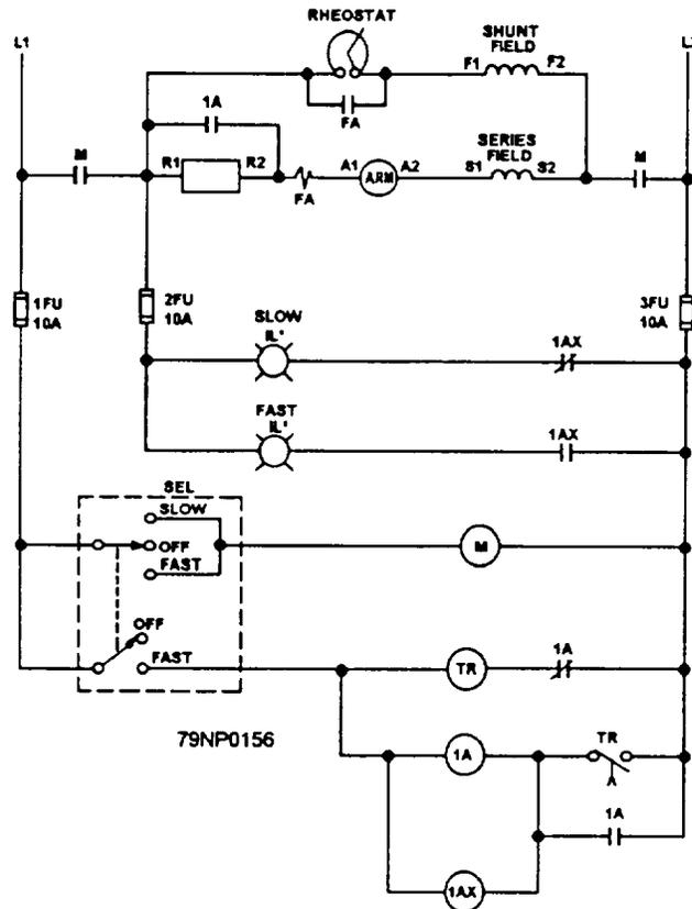
Figure 6-15.—A two-speed dc controller with shunt field rheostat.
