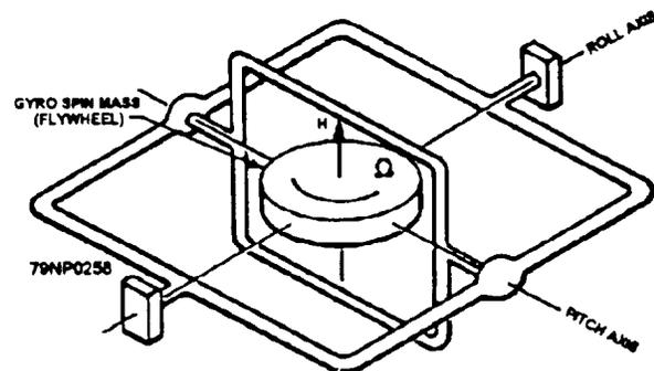
Figure 12-17.—Vertical gyro—simplified schematic.
