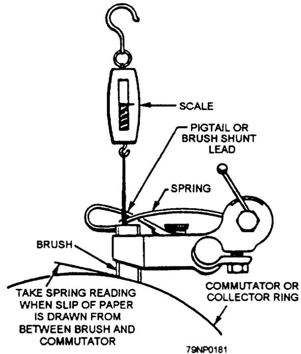
Figure 7-11.—Measuring brush tension.
