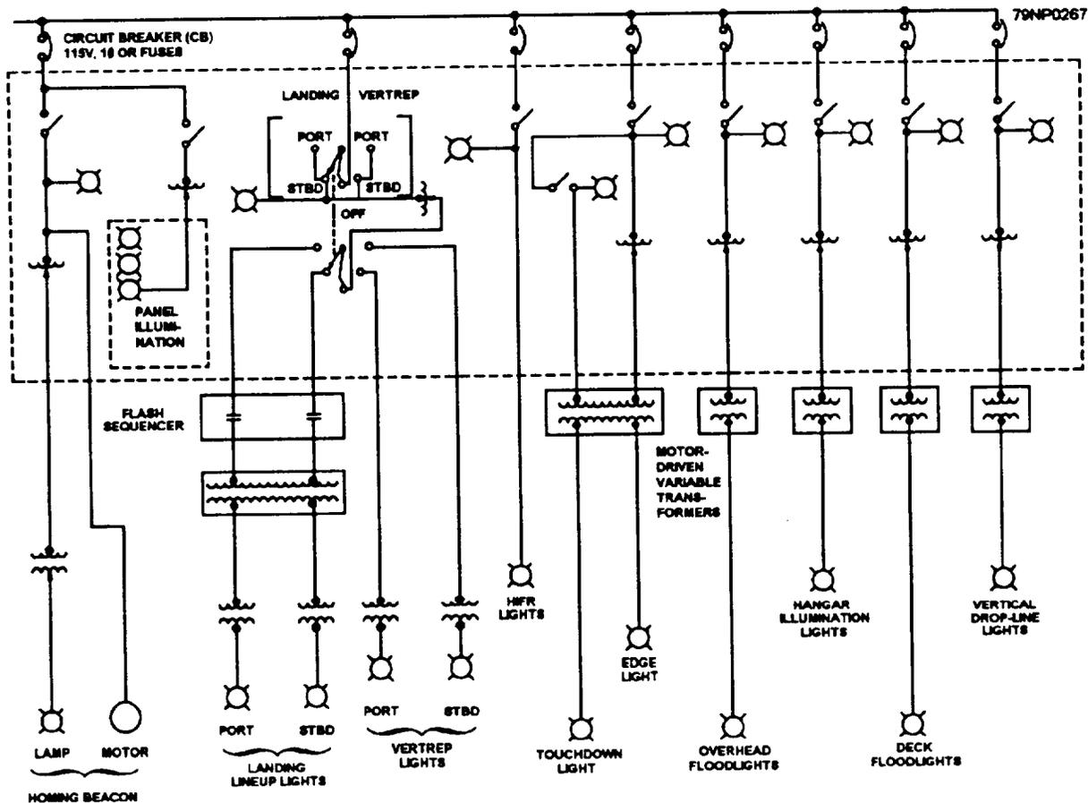
figure 12-26.—Simplified line diagram of the lighting control panel.
