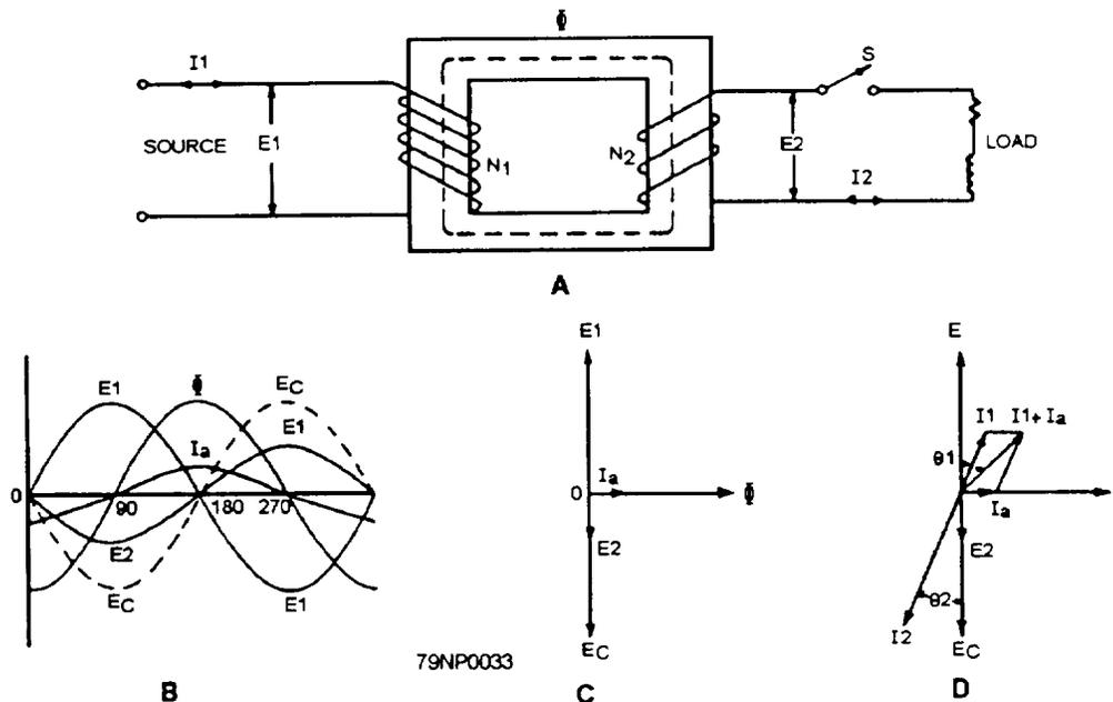
Figure 3-33.—Constant-potential transformer.
