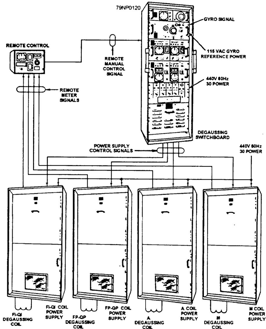
Figure 10-14.—SSM automatic degaussing equipment.
