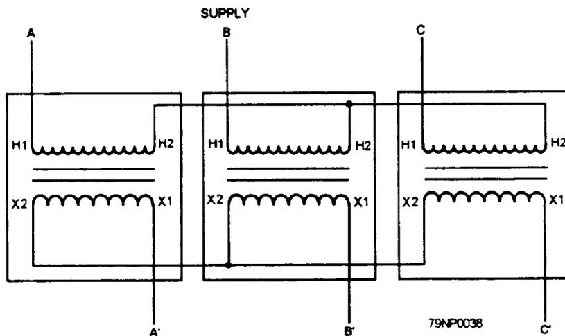
Figure 3-38.—Wye-wye transformer connections.
