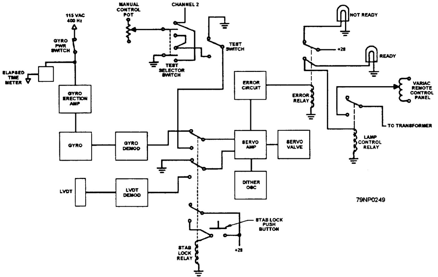
Figure 12-9.—Stabilization control circuits—signal flow.
