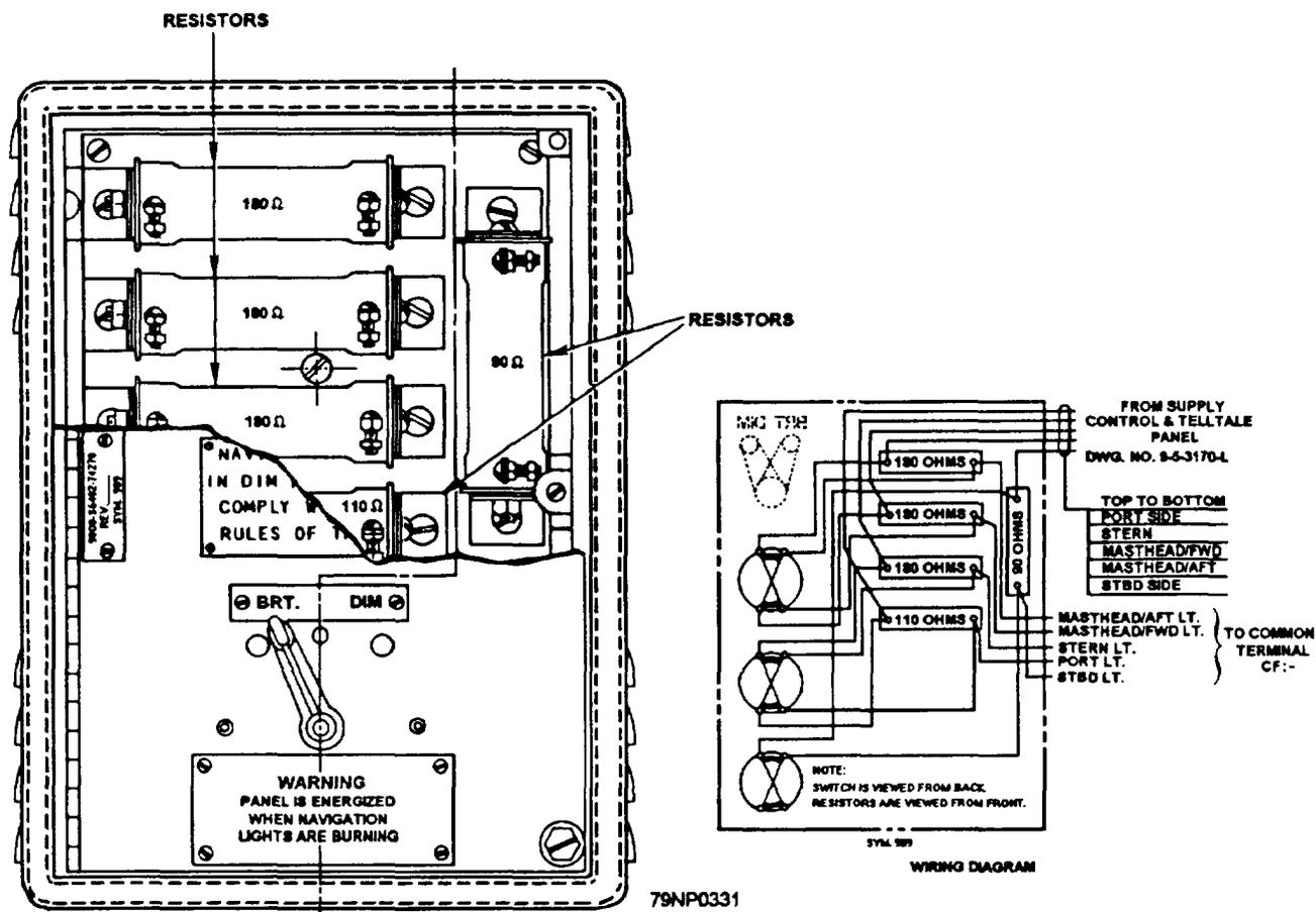
Figure 4-22.—Dimmer control panel, symbol 989.
