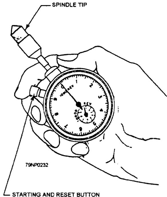
Figure 7-65—A chronometric tachometer.
