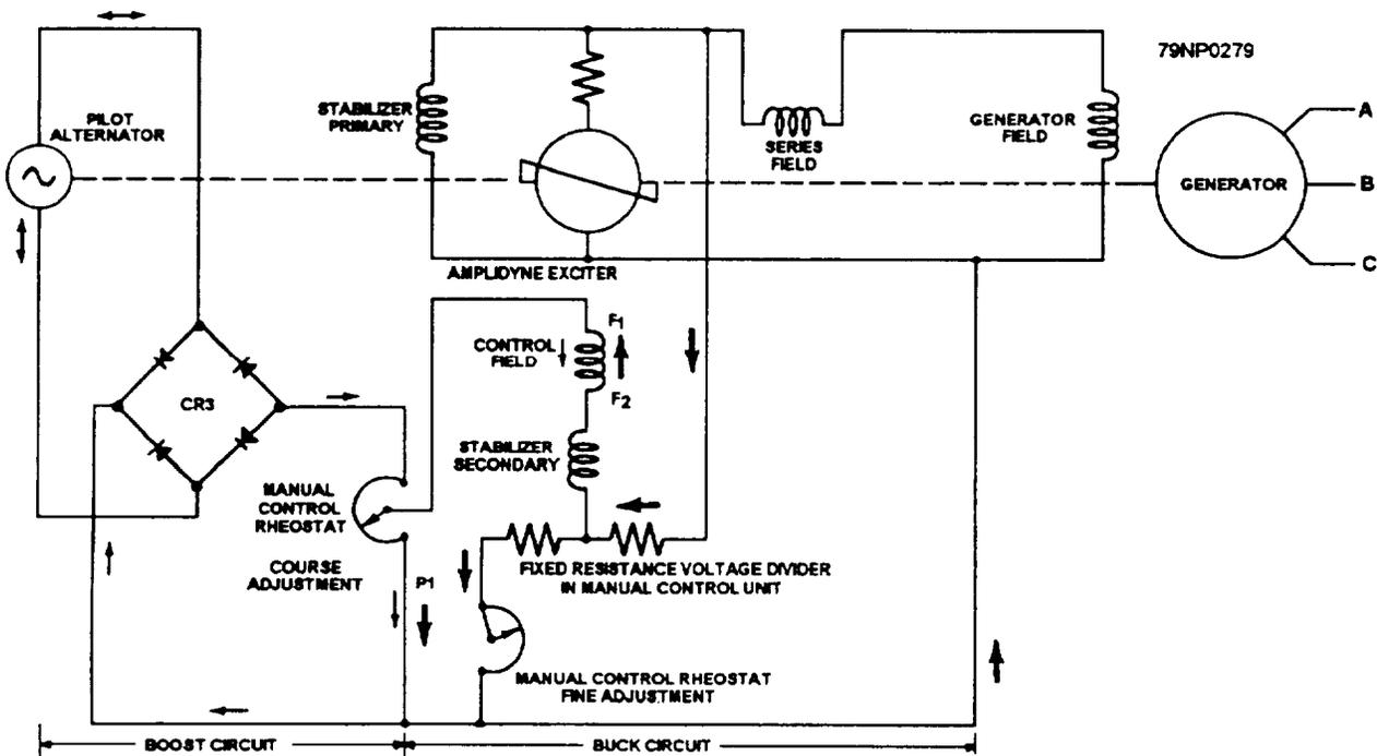
Figure 8-10.—Manual control circuit.
