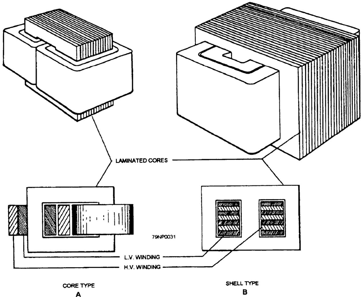
Figure 3-31.—Types transformer construction.
