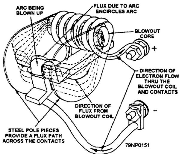
Figure 6-10.—Action of a magnetic blowout coil.
