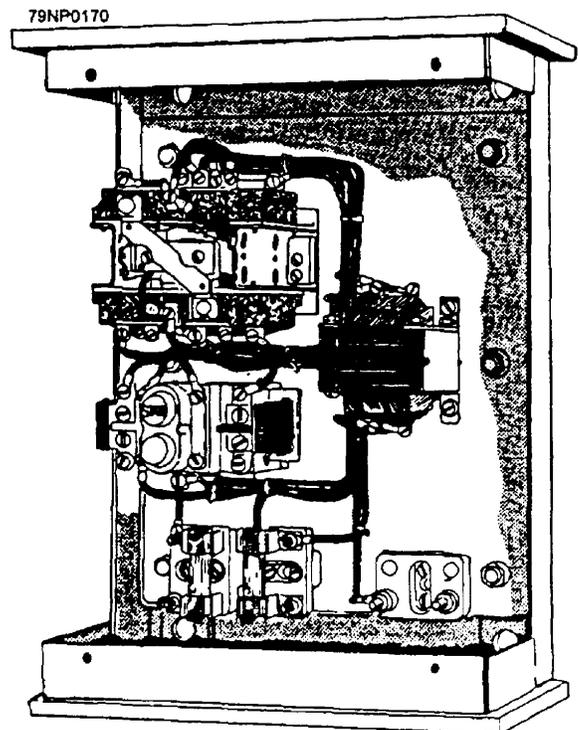
Figure 6-29.—Typical three-phase controller.
