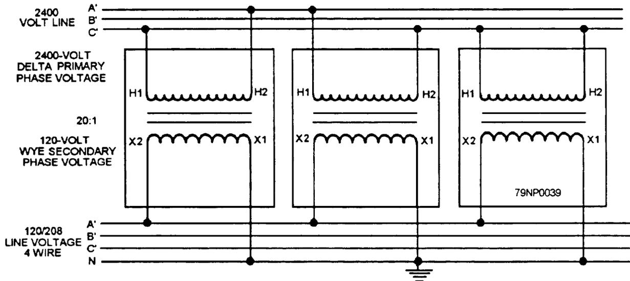
Figure 3-39.—Delta-wye transformer connections.
