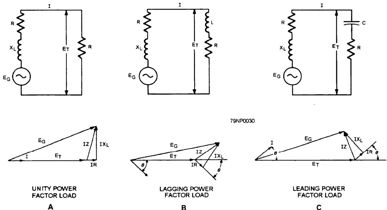
Figure 3-30.—The ac generator voltage characteristics.
