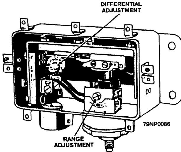
Figure 2-39.—A pressure-operated switch.
