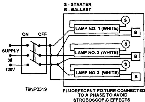
Figure 4-9.—Fluorescent fixture three-phase connections.
