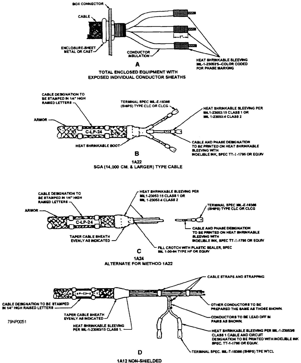
Figure 2-5.—Protecting cable ends.
