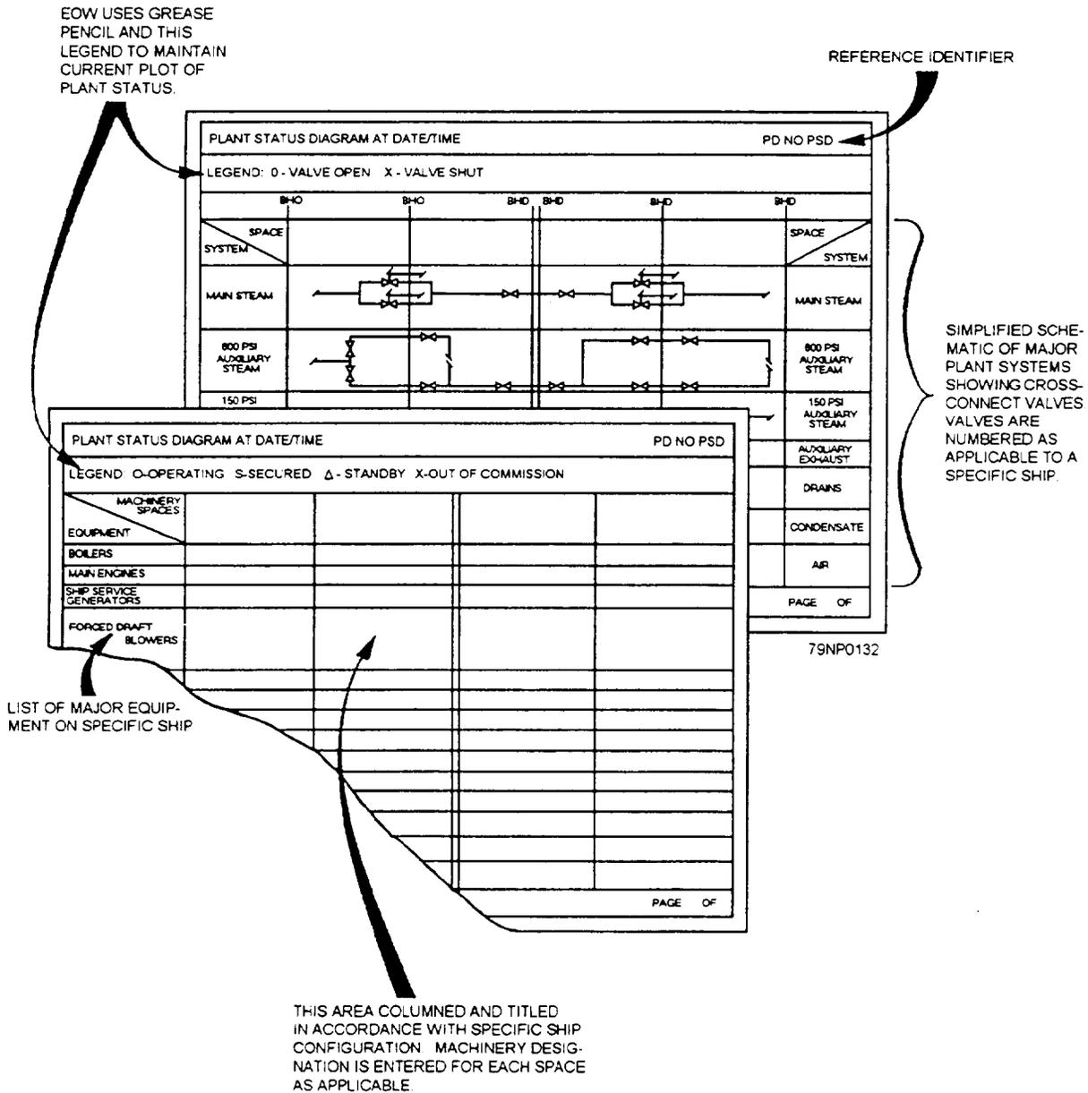
Figure 14-2.-Sample plant status diagram.
