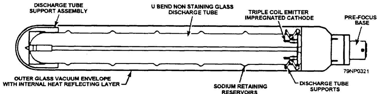
Figure 4-11.—A typical low-pressure sodium (LPS) lamp.
