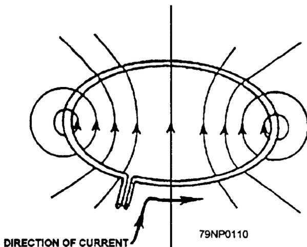
Figure 10-4.—Magnetic field of a current-carrying coil.
