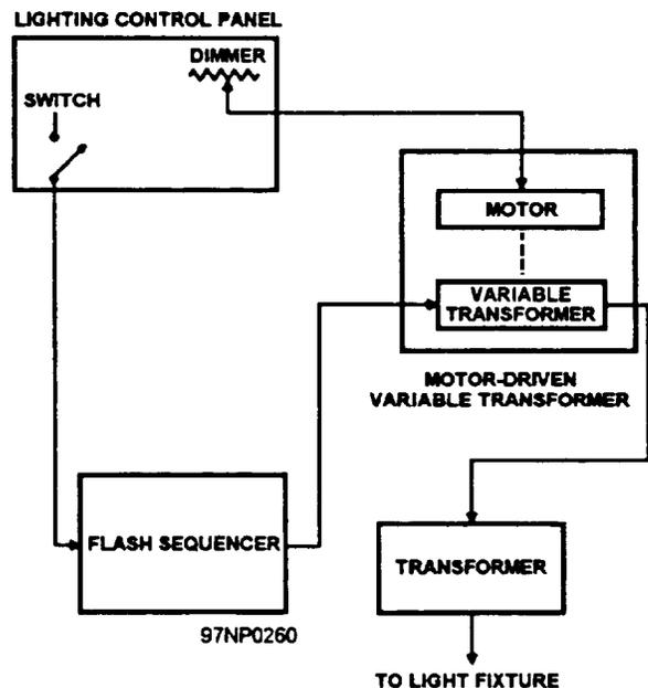
Figure 12-19.—Simplified interconnection of line-up lights.
