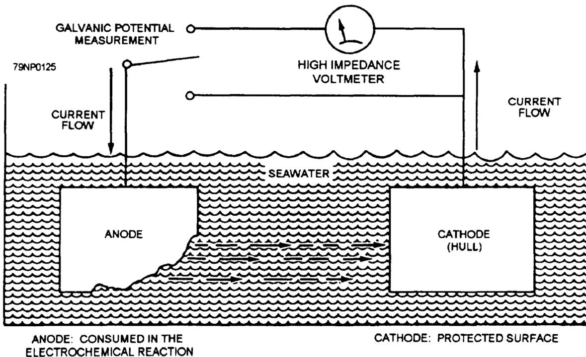
Figure 11-2. Electrochemical corrosion cell.
