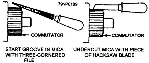
Figure 7-19.—Undercutting mica with a hacksaw blade.
