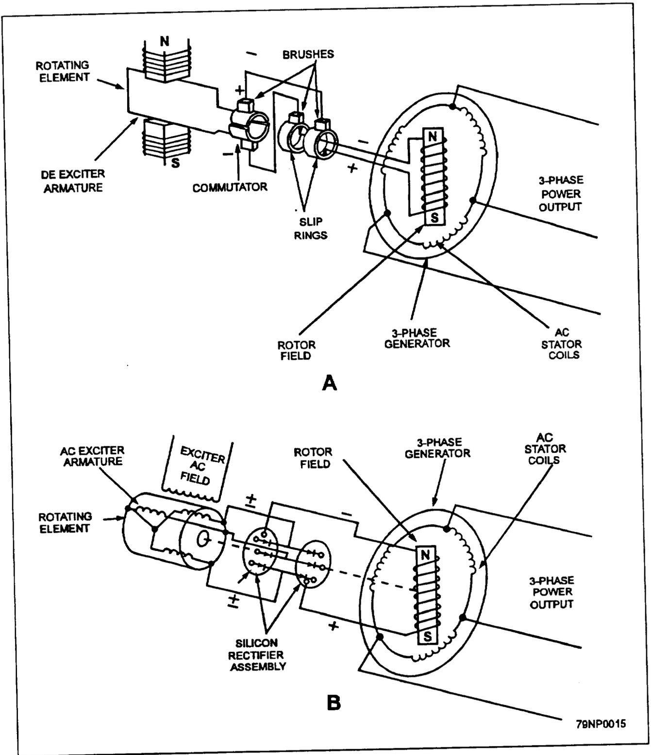
Figure 3-15.—An ac generator: A. Brush type. B. Brushless type.
