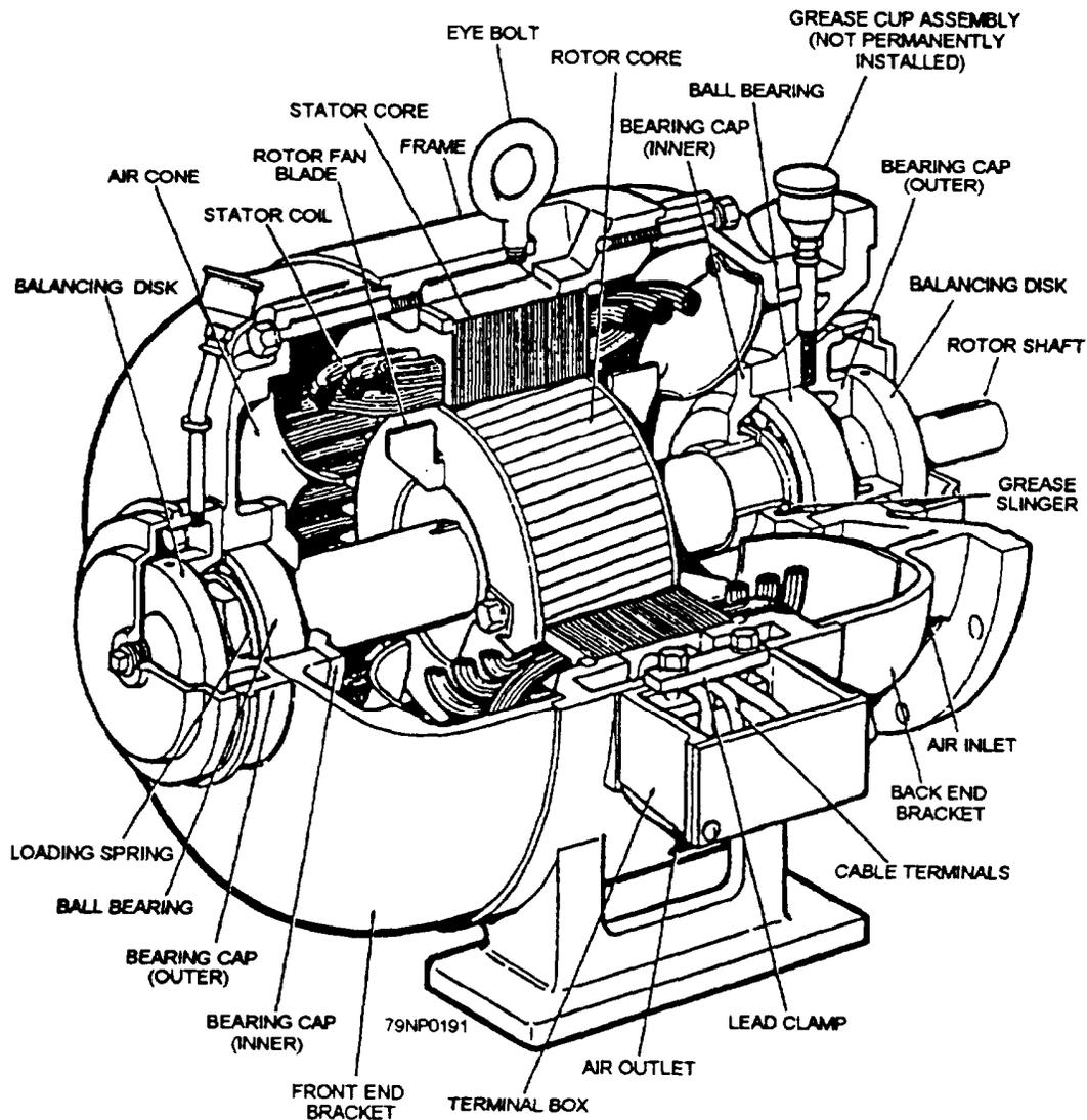
Figure 7-21.—Typical ac motor.
