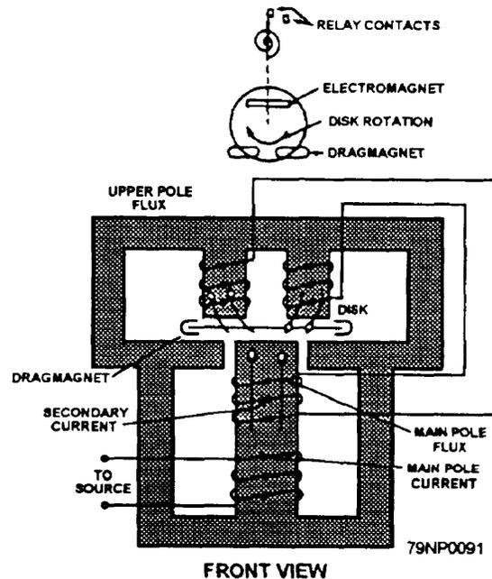
Figure 2-44.—A coil and disk arrangement of an ac reverse-power relay.
