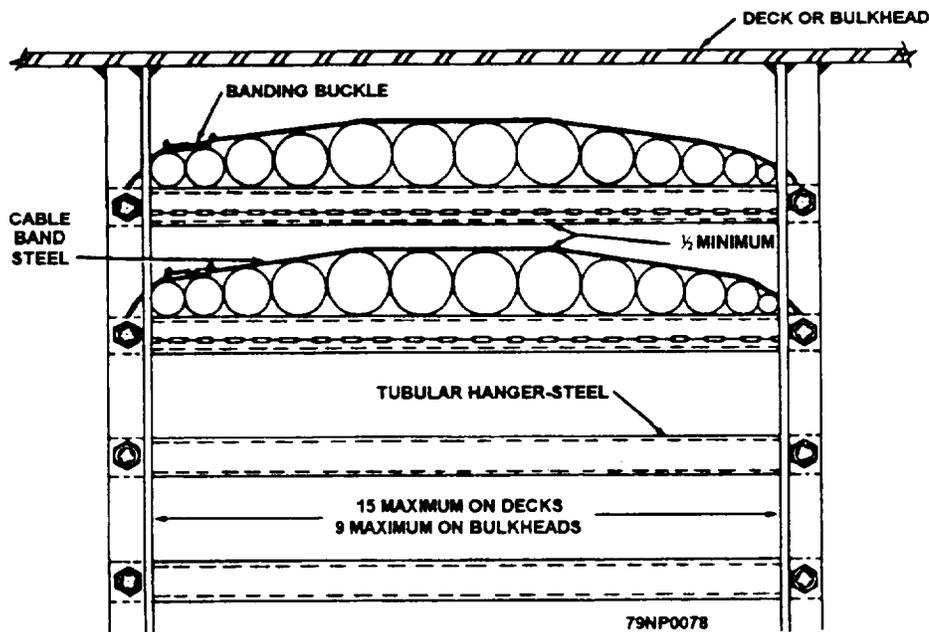
Figure 2-31.—Cables installed in a cable rack.
