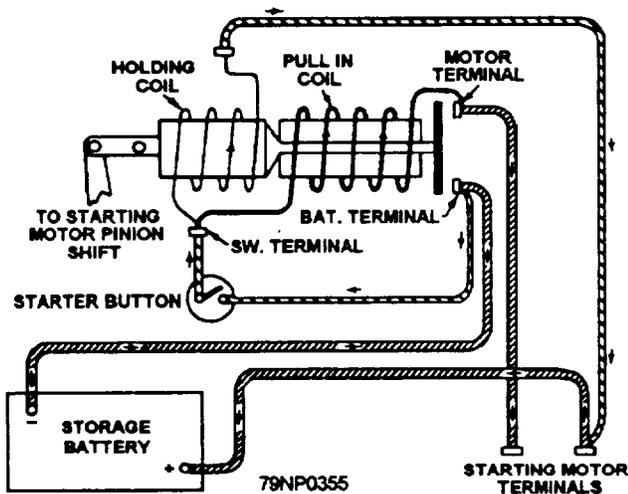
Figure 5-6.—Solenoid switch diagram.
