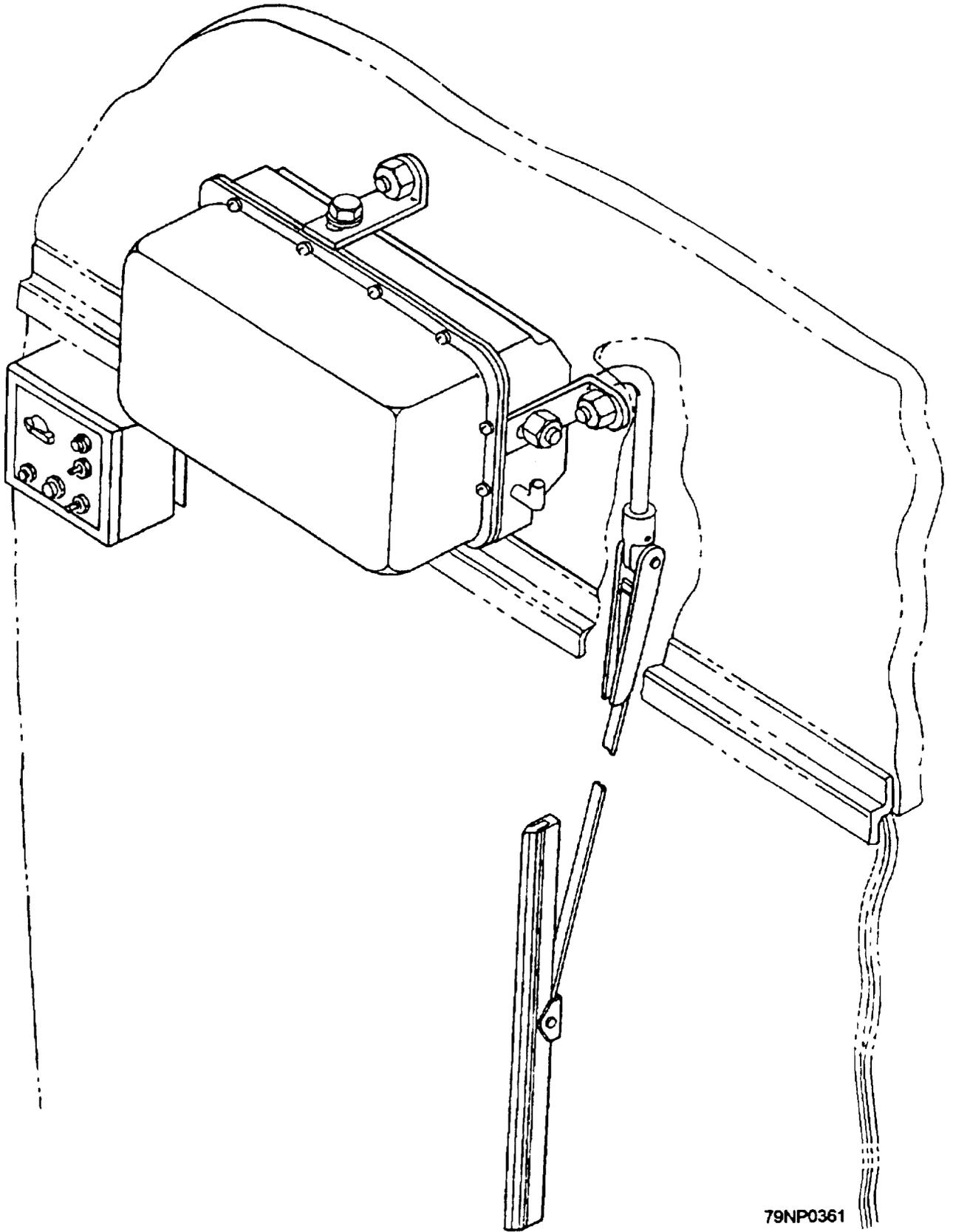
Figure 5-13.—Pendulum window wiper.
