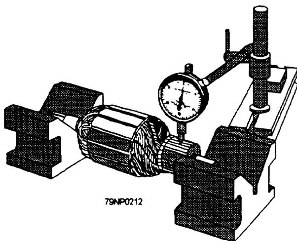
Figure 7-43.—Measuring commutator out-of-round with a dial indicator.
