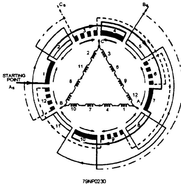
Figure 7-63.—Three-phase, four-pole, series-delta winding.
