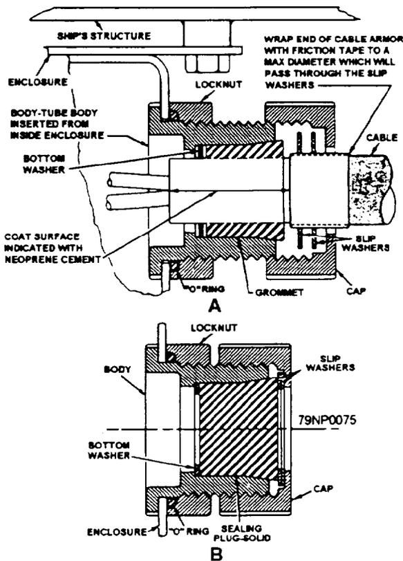
Figure 2-28.—Representative nylon stuffing tube installations.
