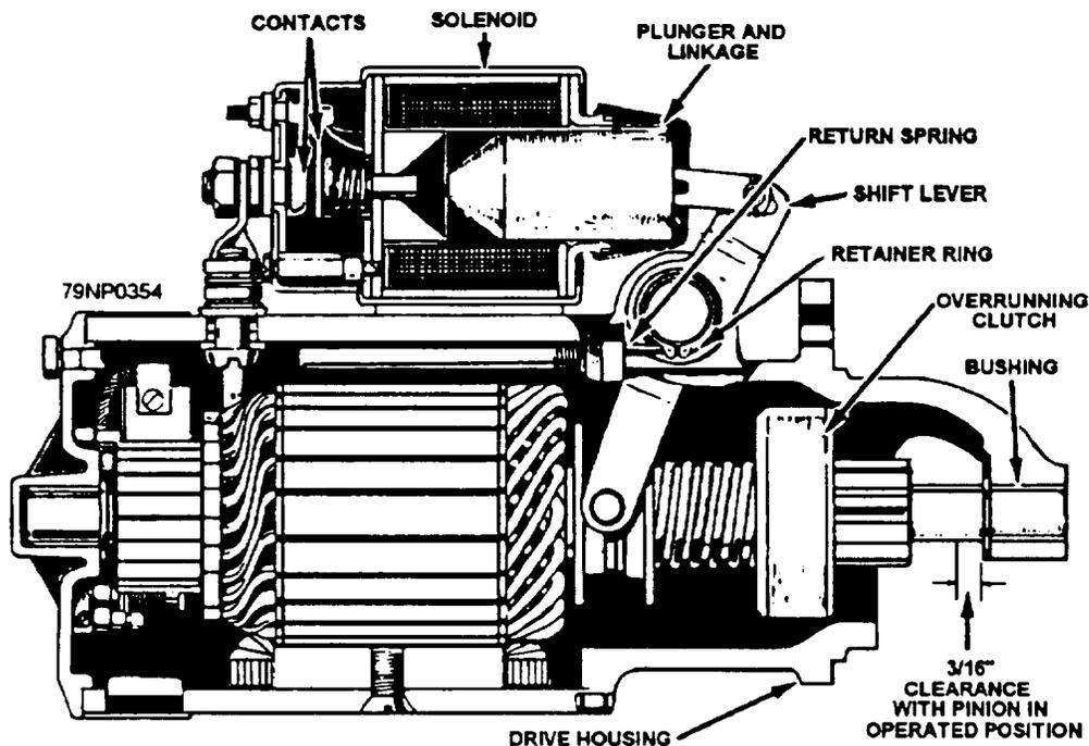
Figure 5-5.—Starting motor with an overrunning clutch drive and a solenoid-operated switch.
