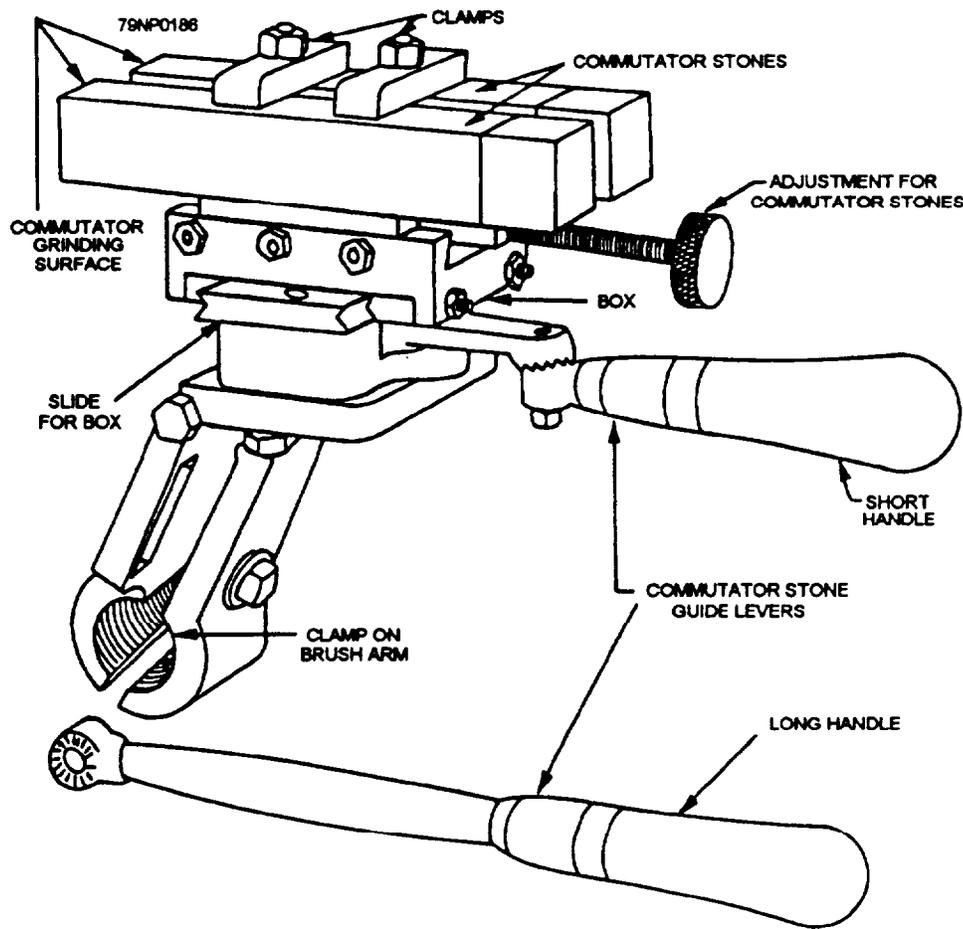
Figure 7-16.—Commutator dressing stone tool.
