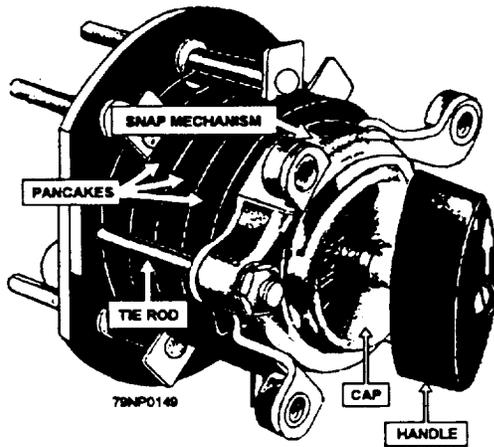
Figure 6-8.—Rotary snap switch.
