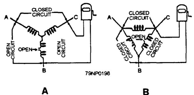
Figure 7-29.—Ohmmeter test for open circuits.
