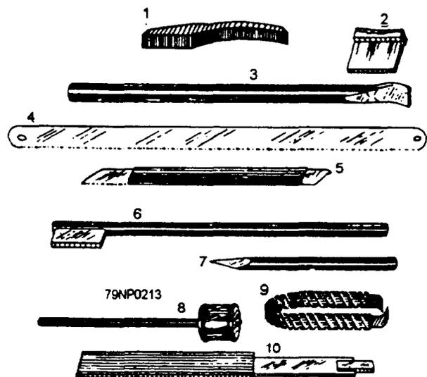
Figure 7-44.—Armature rewinding hand tools.
