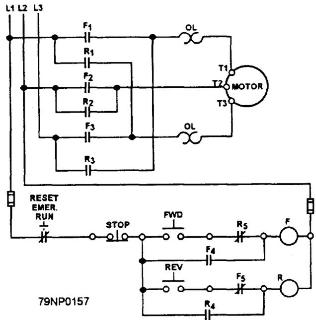
Figure 6-16.—Reversing ac controller.
