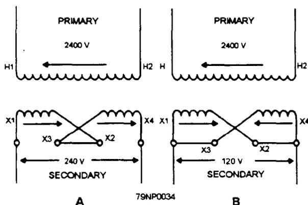
Figure 3-34.—Single-phase transformer connections.
