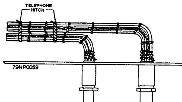
Figure 2-12.—Binding cable groups with the telephone hitch.
