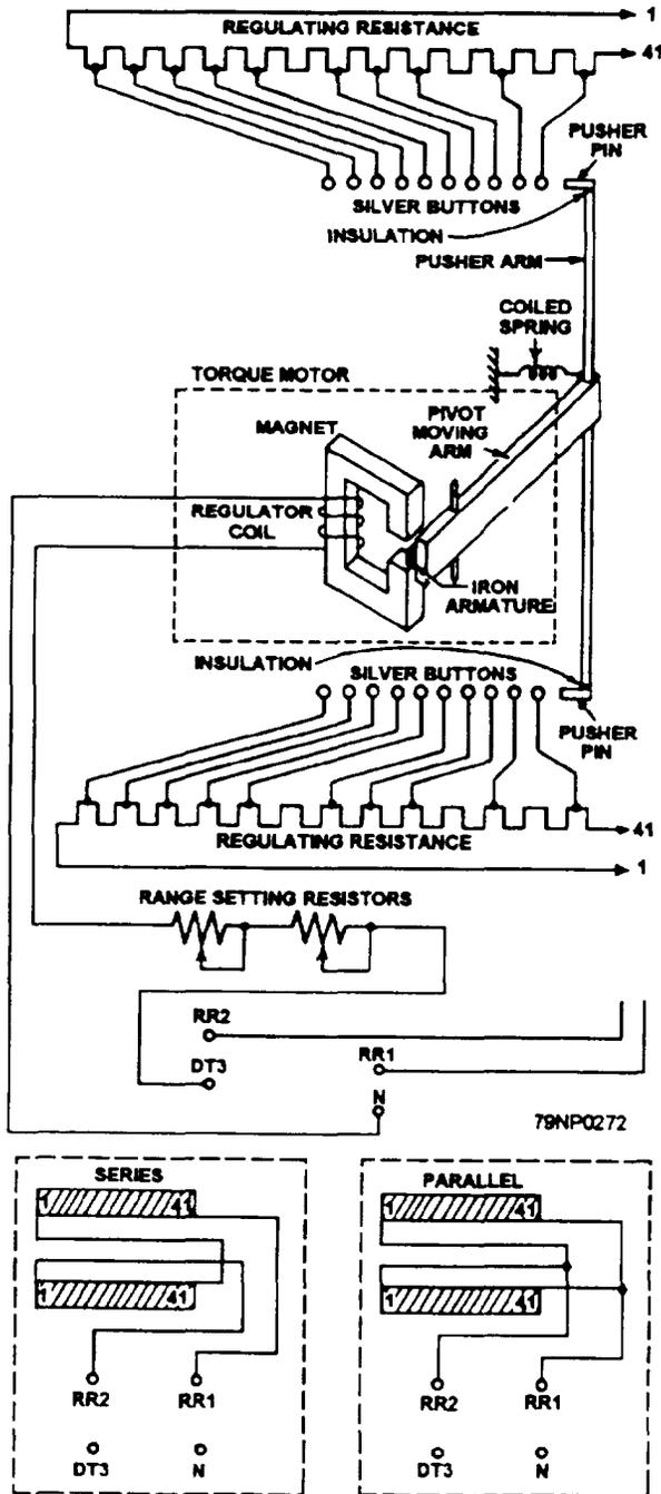
Figure 8-3.—Control element of a direct-acting voltage regulator.
