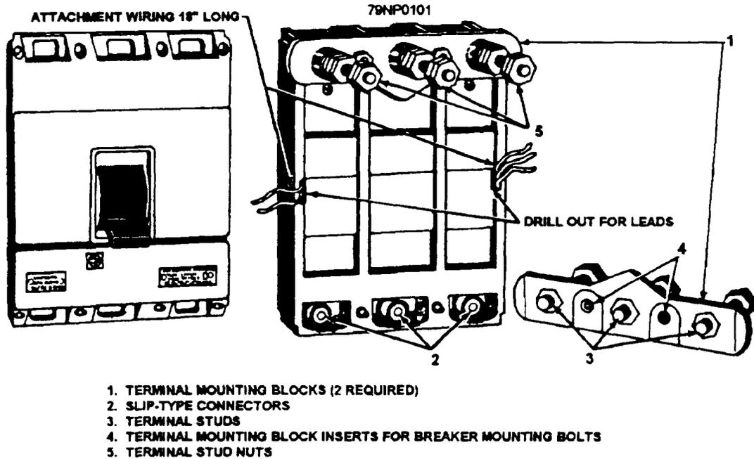
Figure 2-54.—AQB-A250 circuit breaker, rear view, with terminal mounting blocks.
