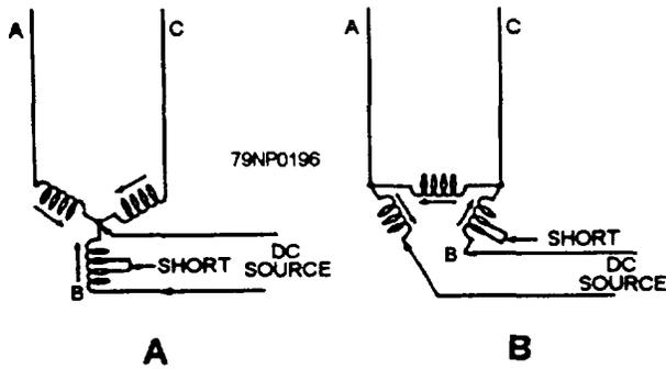
Figure 7-27.—Compass test for shorted pole-phase groups.
