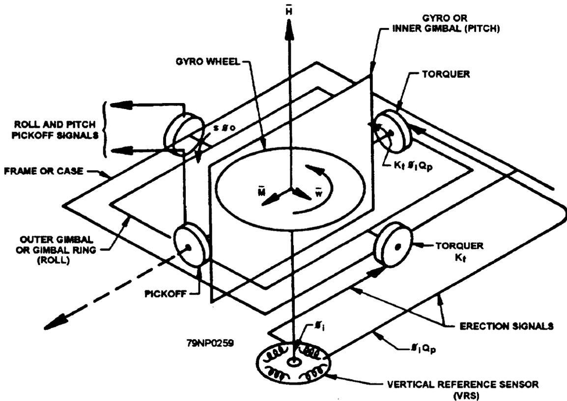
Figure 12-18.—Vertical gyro—line schematic diagram.
