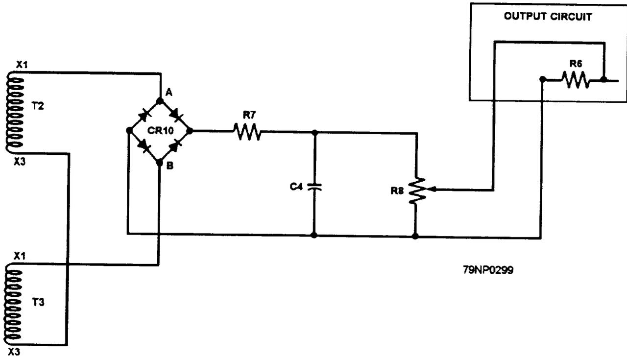
Figure 8-30.—Schematic diagram of a phase difference monitoring circuit.
