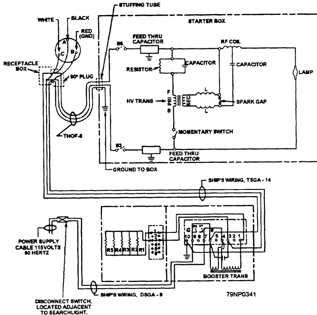
Figure 4-32.—Wiring diagram for a 12-inch mercury-xenon arc searchlight.
