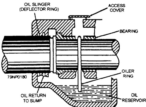
Figure 7-9.—Diagram of an oil-lubricated bearing.
