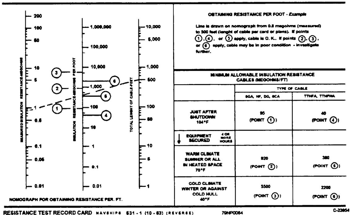
Figure 2-17.—Nomograph for obtaining resistance per foot.
