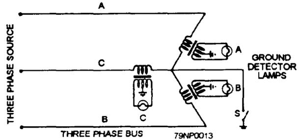
Figure 3-13.—An ac ground detector lamp circuit.
