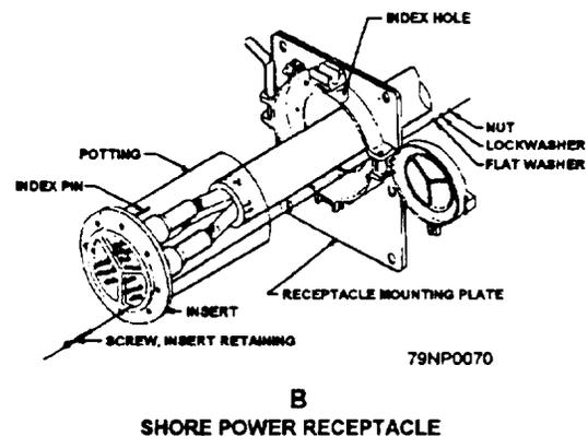
Figure 2-23.—Shore-power station and receptacle assembly.
