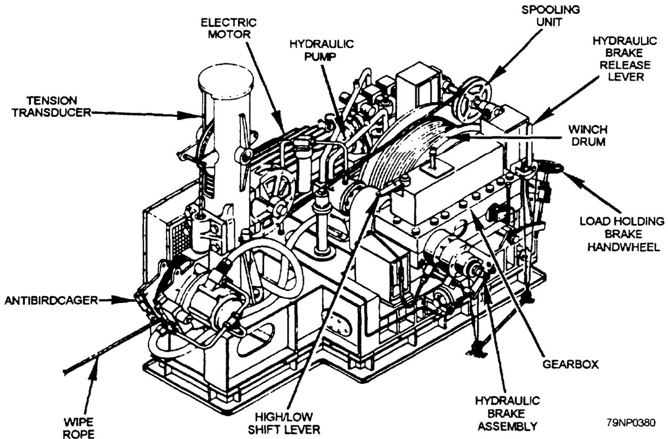
Figure 5-32.—Parts of the inhaul/outhaul winch.
