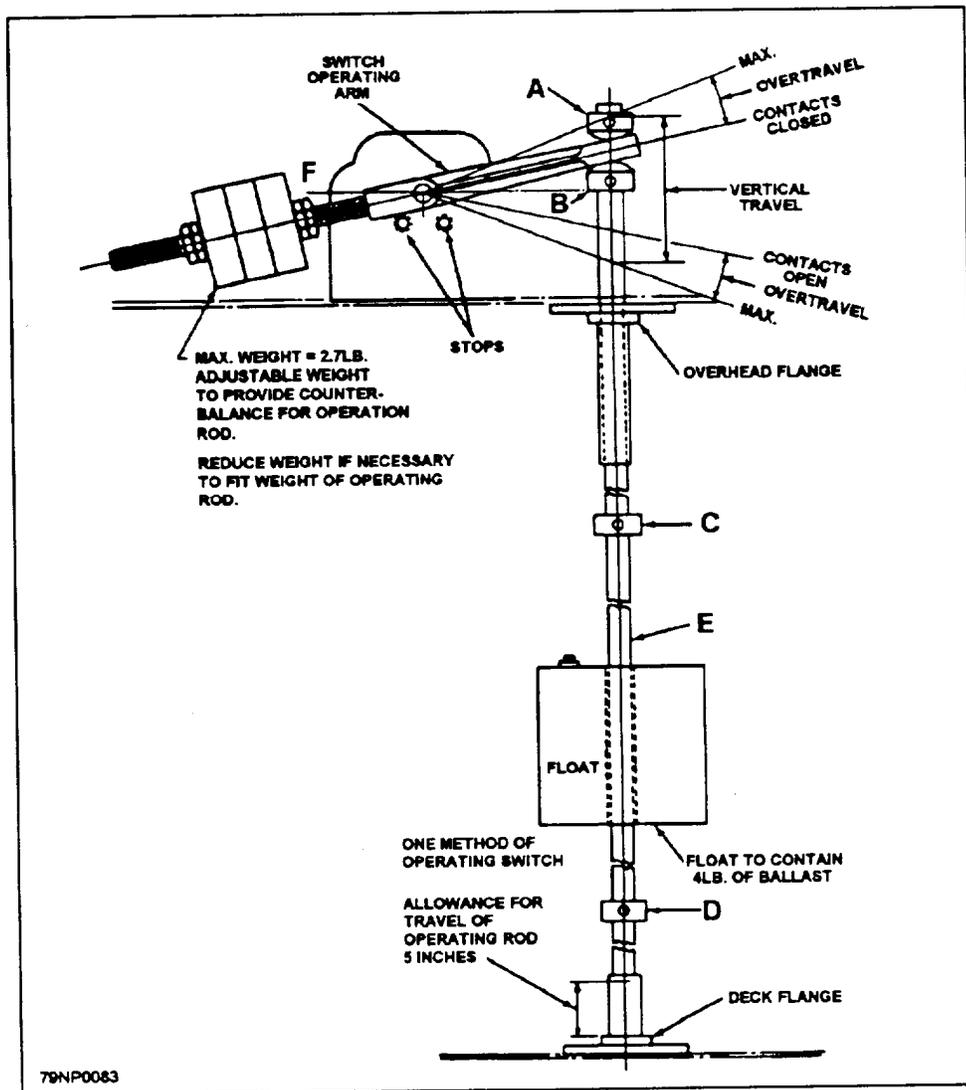
Figure 2-36.—A float switch tank installation.
