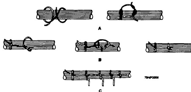
Figure 2-9.—Lacing procedure.
