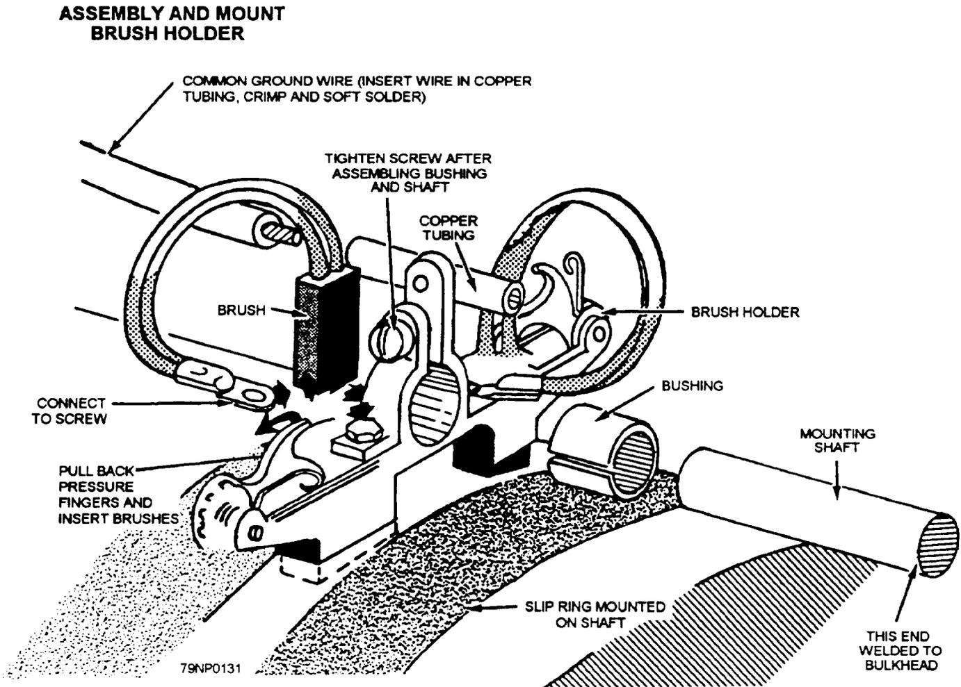
Figure 11-8.—Shaft grounding assembly.
