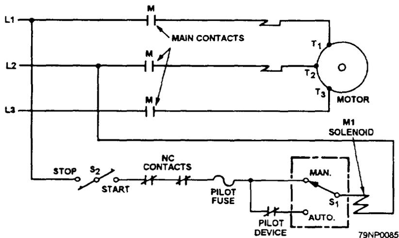
Figure 2-38.—A representative pilot device control circuit.
