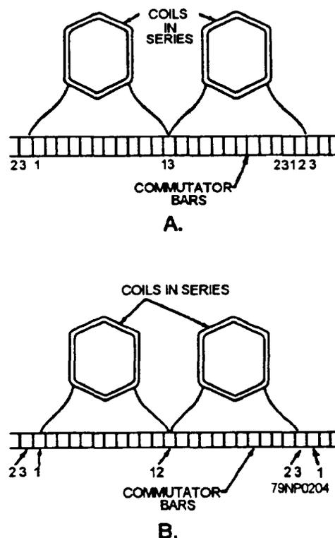
Figure 7-35.—Four-pole simplex wave windings.
