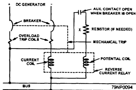
Figure 2-47.—A dc reverse-current connection.
