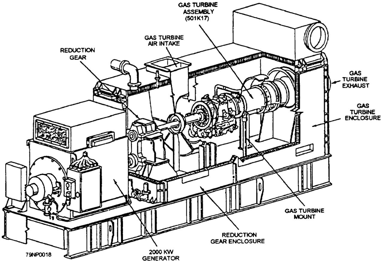
Figure 3-18.—Model 104 gas turbine generator set.
