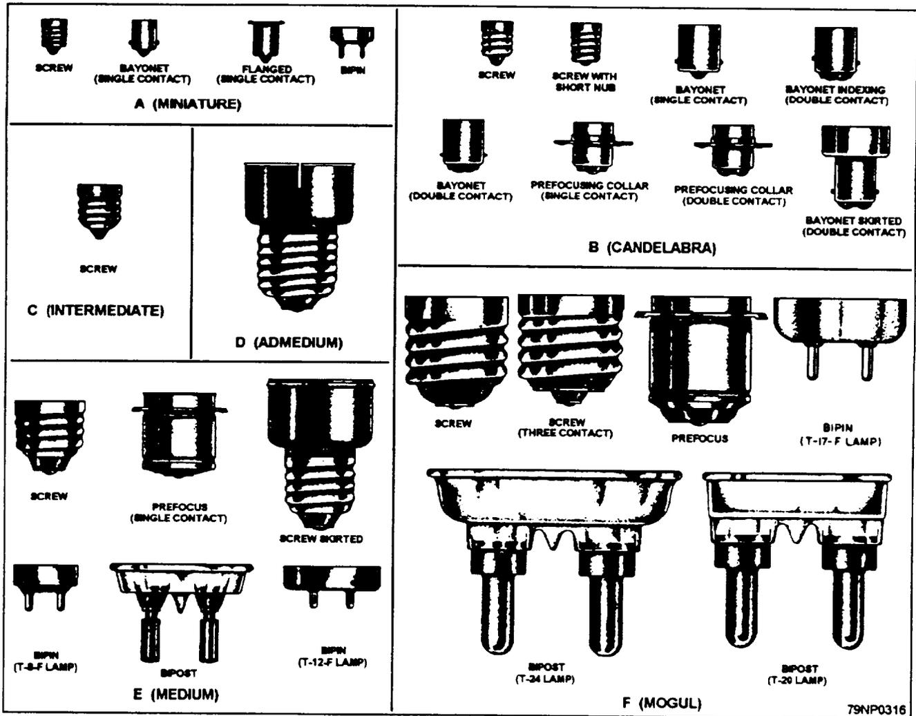
Figure 4-6.—Classification of lamps according to the type of base.
