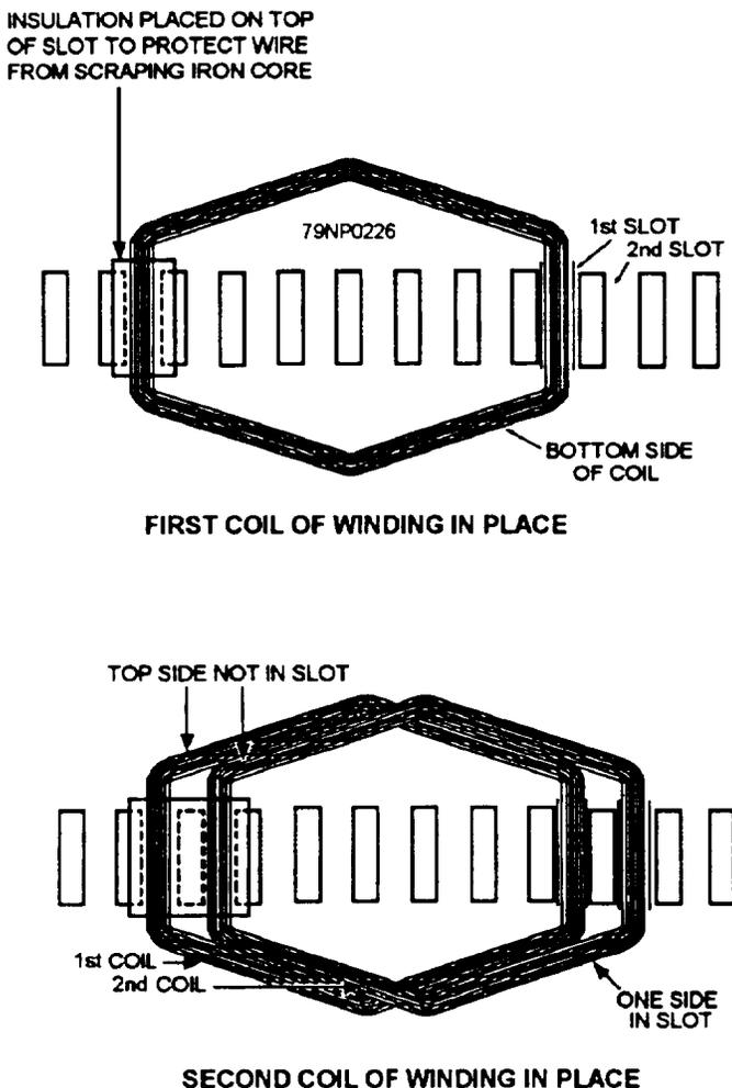
Figure 7-59.—Placing coil sides in slots.
