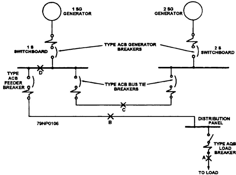
Figure 2-59.—Selected tripping of circuit breakers.
