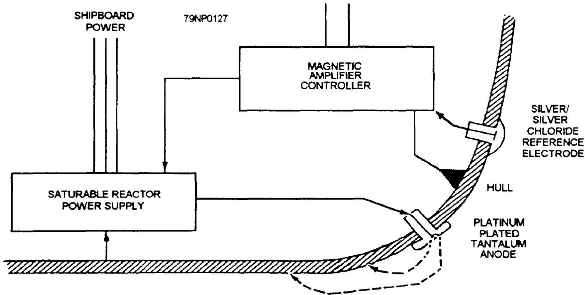
Figure 11-4.—Basic impressed current cathodic protection system.
