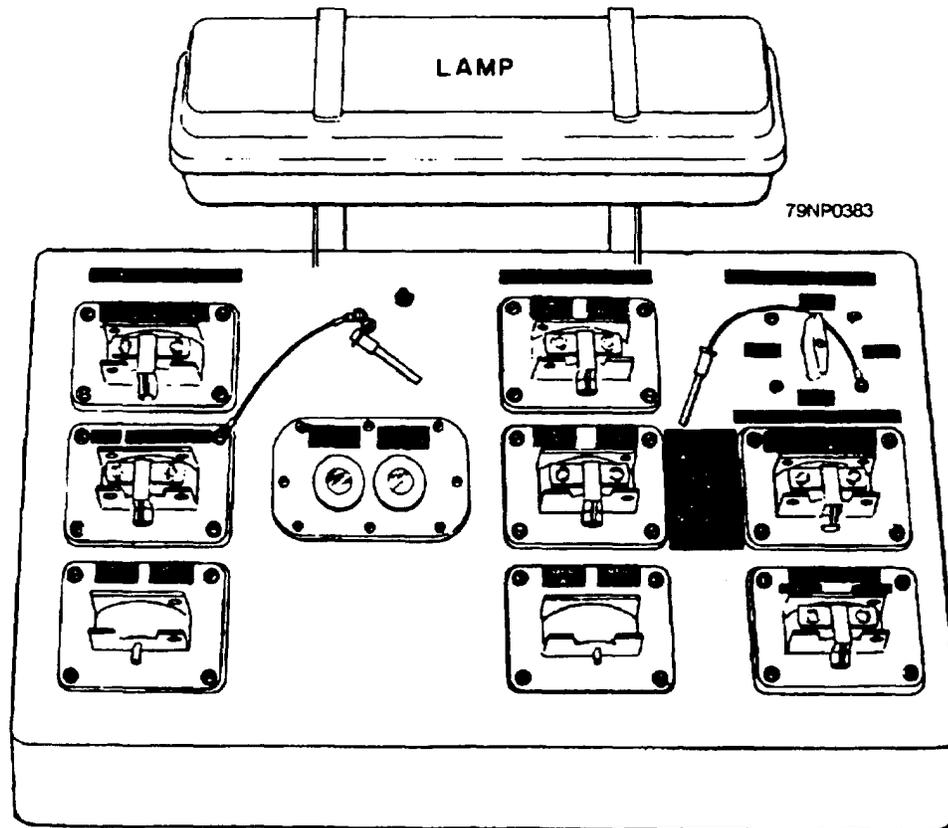
Figure 5-35.—Control console on a receiving ship.
