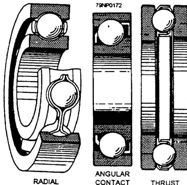
Figure 7-1.—Representative types of ball bearings.
