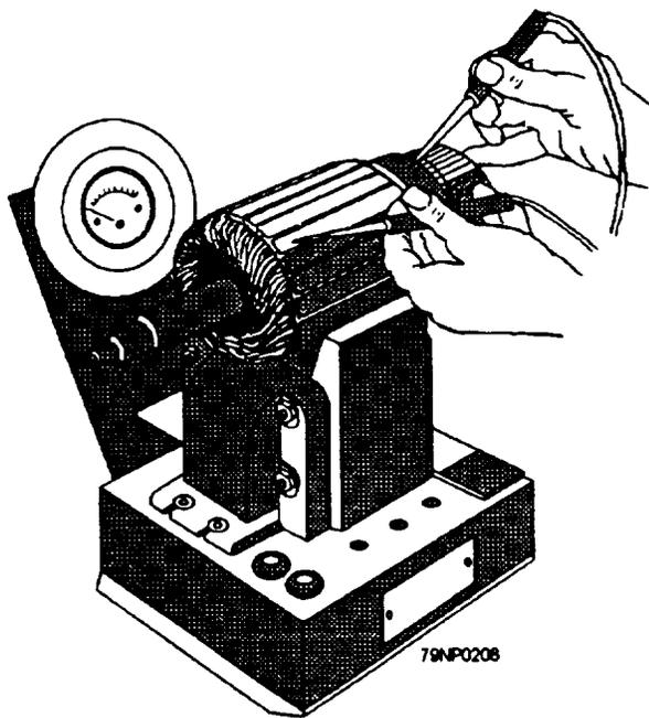
Figure 7-39.—Testing an armature for grounds.
