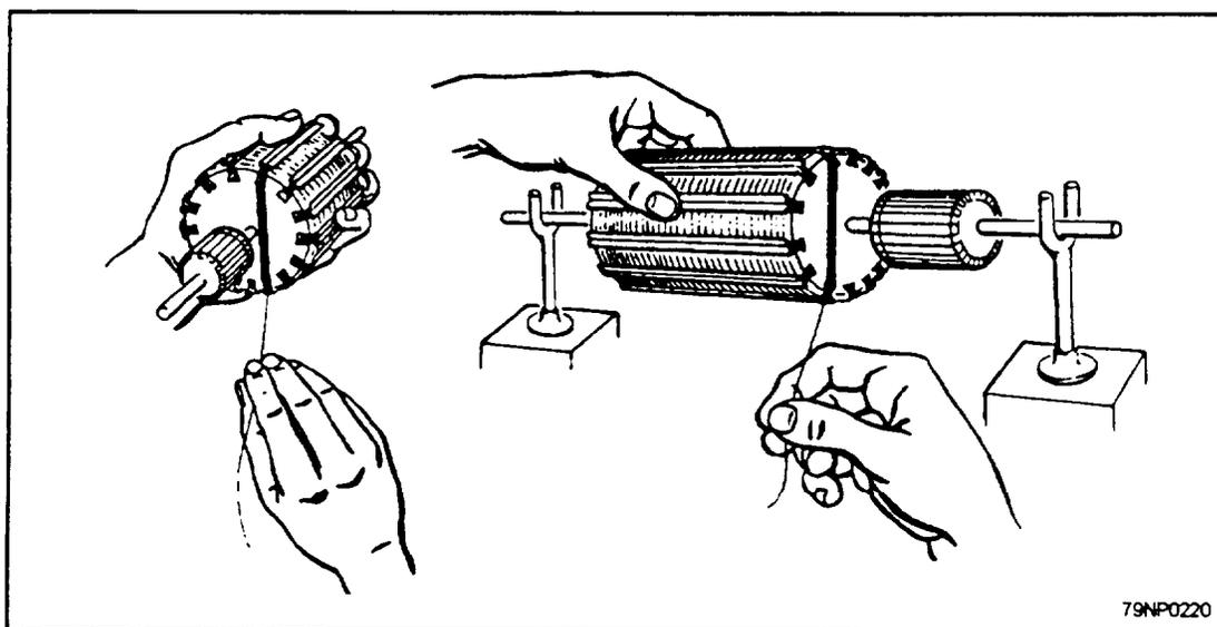
Figure 7-52.—Winding armatures by hand.
