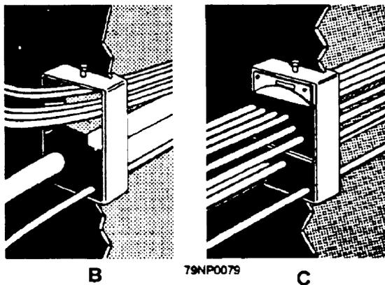
Figure 2-32.—Modular cable supports.
