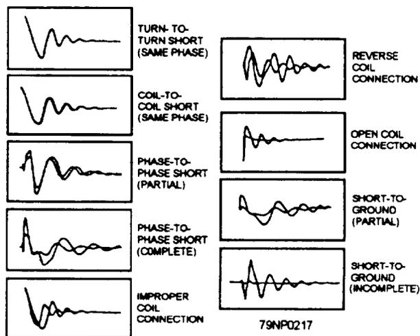
Figure 7-48.—Representative surge test waveforms.
