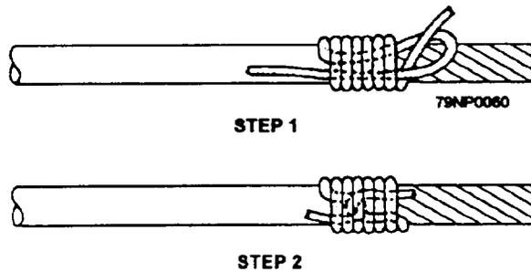
Figure 2-13.—Serving conductor ends.
