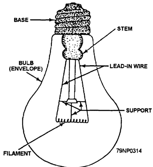
Figure 4-4.—Components of an incandescent lamp.
