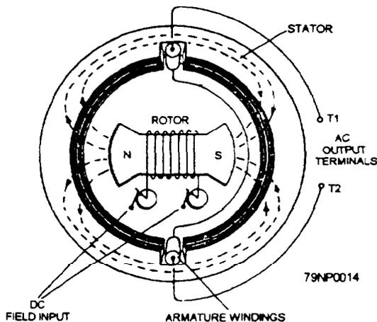
Figure 3-14.—Essential parts of a rotating-field generator.
