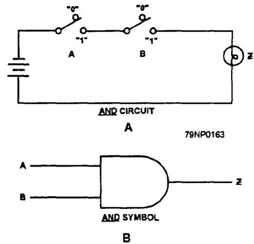
Figure 6-22.—AND symbol and circuit.
