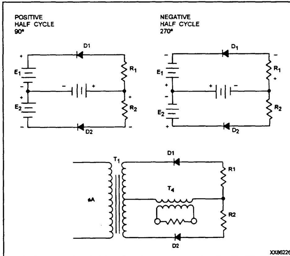
Figure 9.21—Equivalent single-phase circuit. *Reprinted with permission of Woodward Governor Company, 1994*
