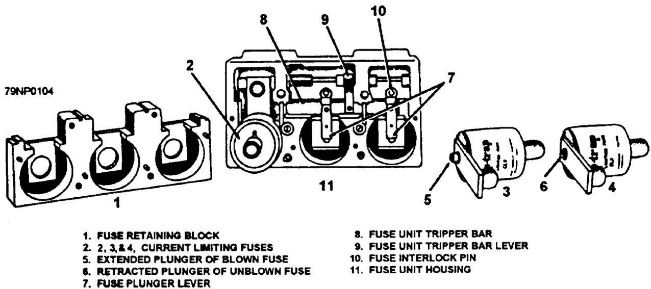
Figure 2-57.—Current-limiting fuse unit assembly.
