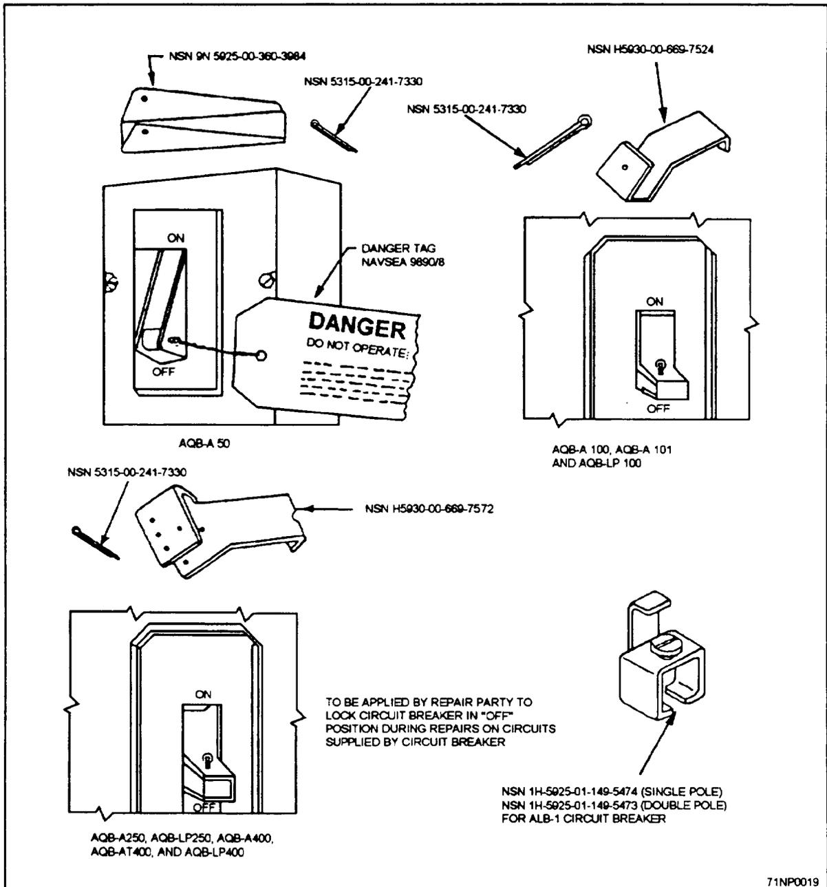
Figure 1-20.—Handle-locking devices for circuit breakers.
