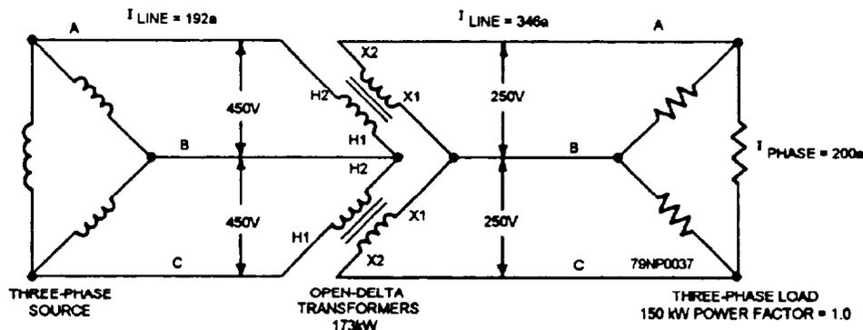
Figure 3-37.—Open-delta transformer connection.
