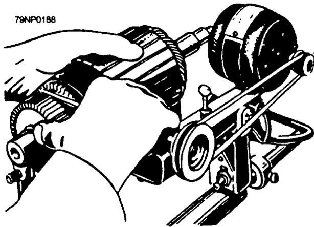
Figure 7-18.—Undercutting commutator mica with undercutter.
