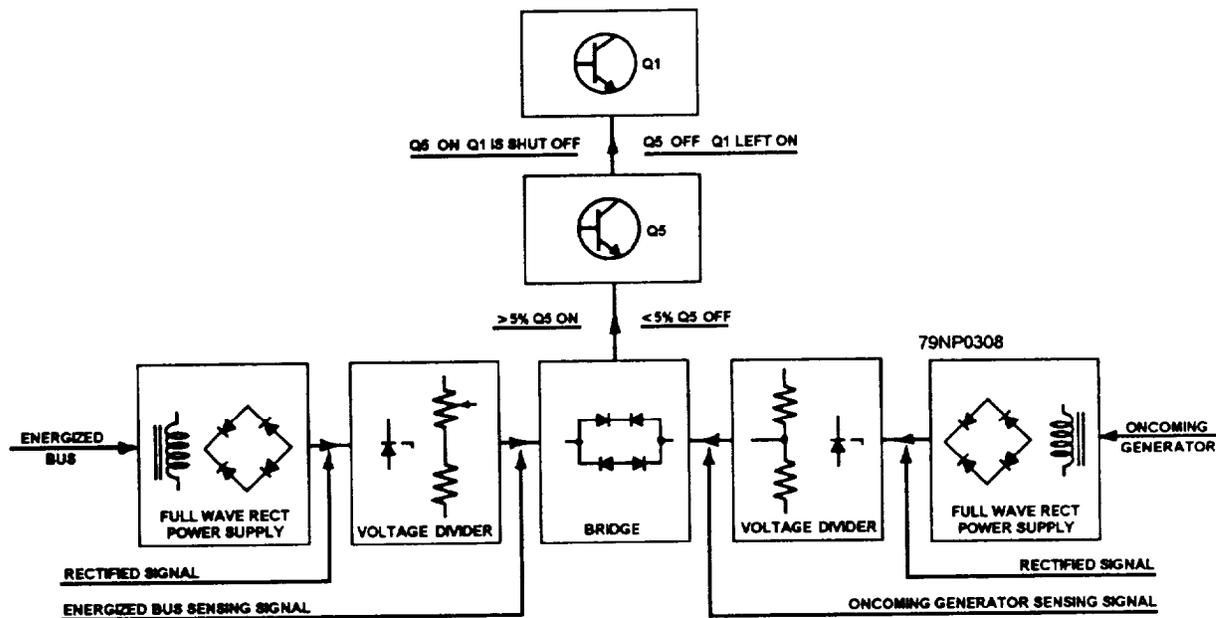
Figure 8-39.—Block diagram of voltage difference monitoring circuit.
