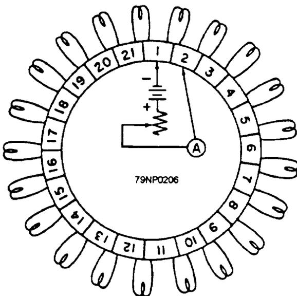
Figure 7-37.—Schematic of a simplex lap winding.
