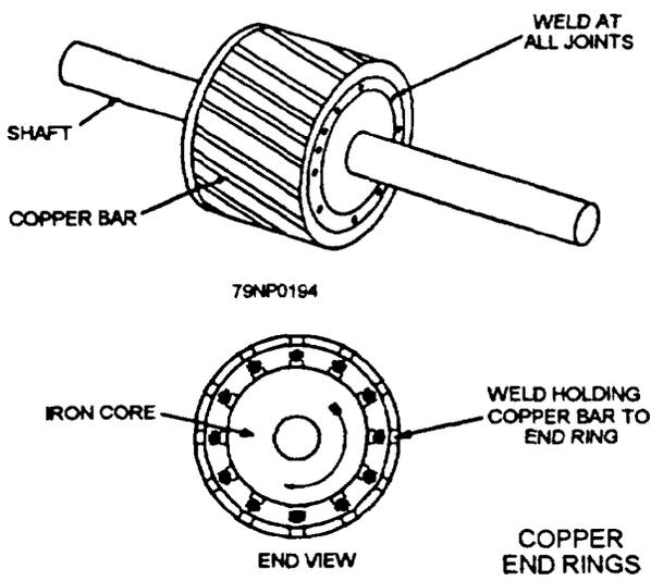
Figure 7-25.—Squirrel-cage rotor.
