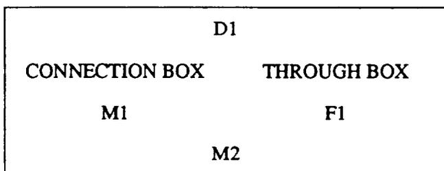
This sample identified the No. 1 degaussing box serving as a connection box for the M1 and M2 loops and as a through box for the F1 loop.
