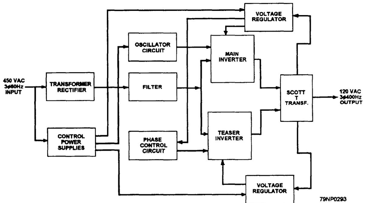
Figure 8-24.—Static converter, simplified block diagram.
