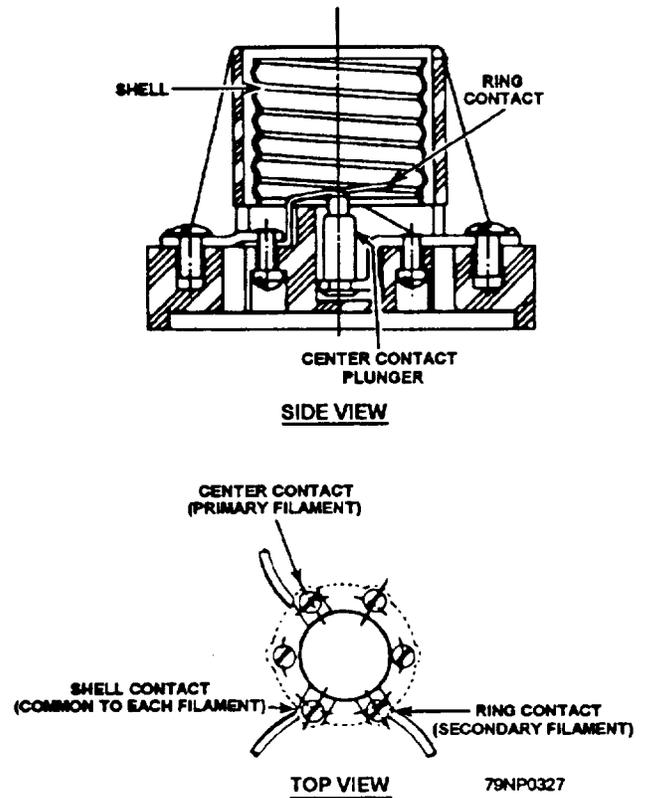
Figure 4-18.—New navigation light fixture lamp holder wiring diagram.
