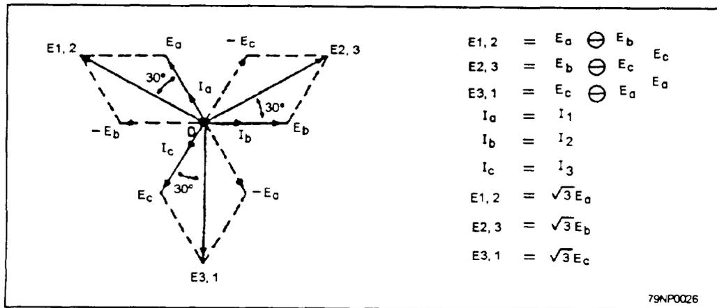
Figure 3-26.—Three-phase, wye-connected system.
