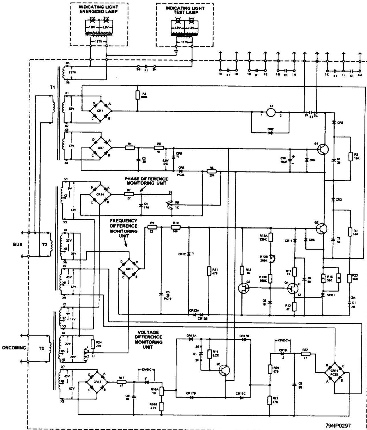
Figure 8-28.—Synchronizing monitor.
