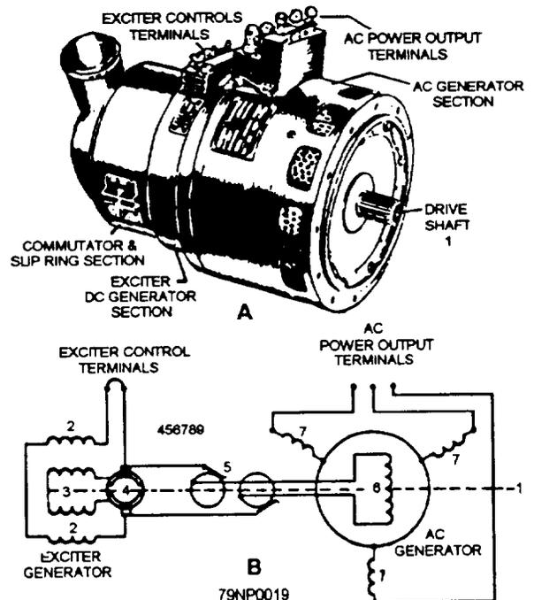
Figure 3-19.—An ac generator and schematic.
