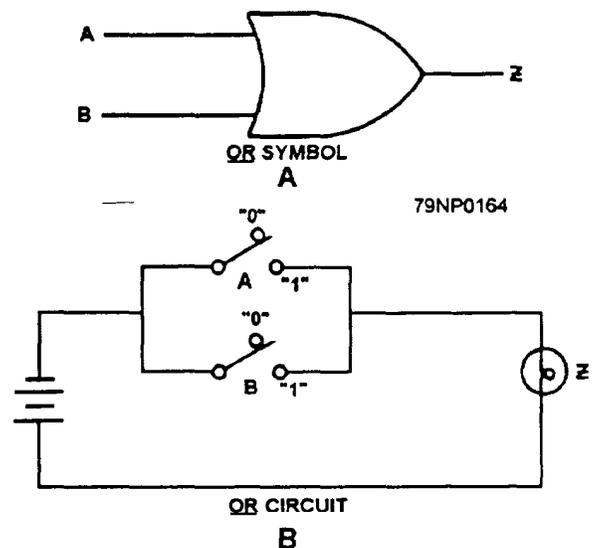
Figure 6-23.—OR symbol and circuit.
