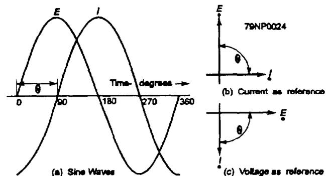
Figure 3-24.—Waves and vectors of alternating current and voltage in a circuit containing only inductance.
