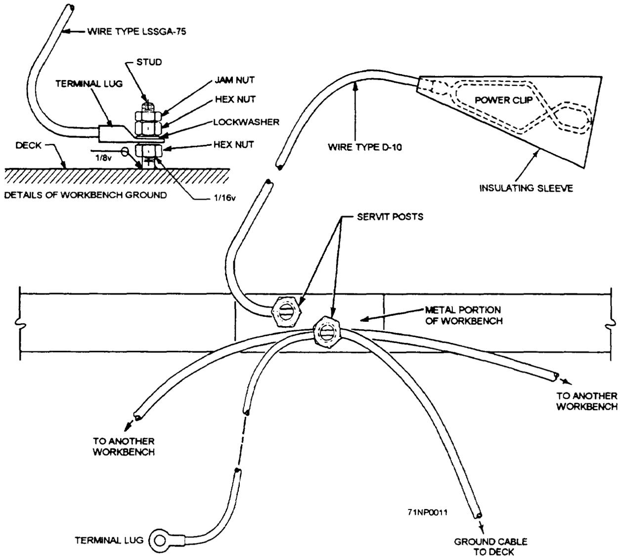
Figure 1-5.—Installation of grounding cable for electric workbench.
