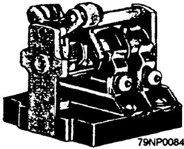
Figure 2-37.—A float switch mechanism.
