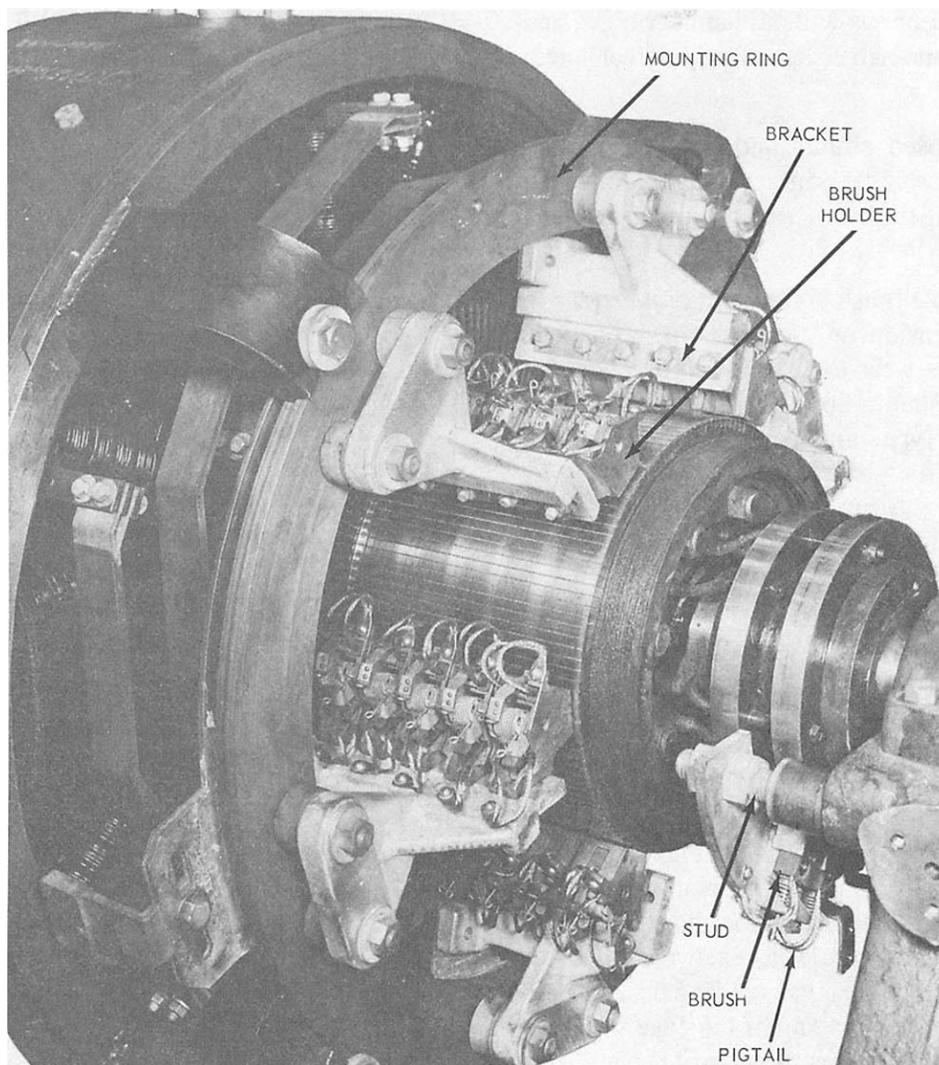
**Figure 7-10.—Brush holder and brush rigging assembly.**
