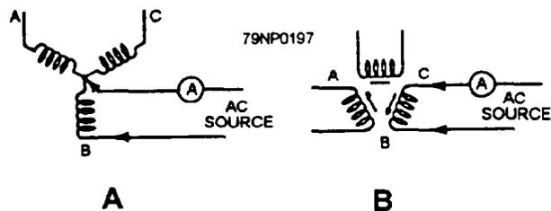
Figure 7-28.—Balanced current test for shorted phase.
