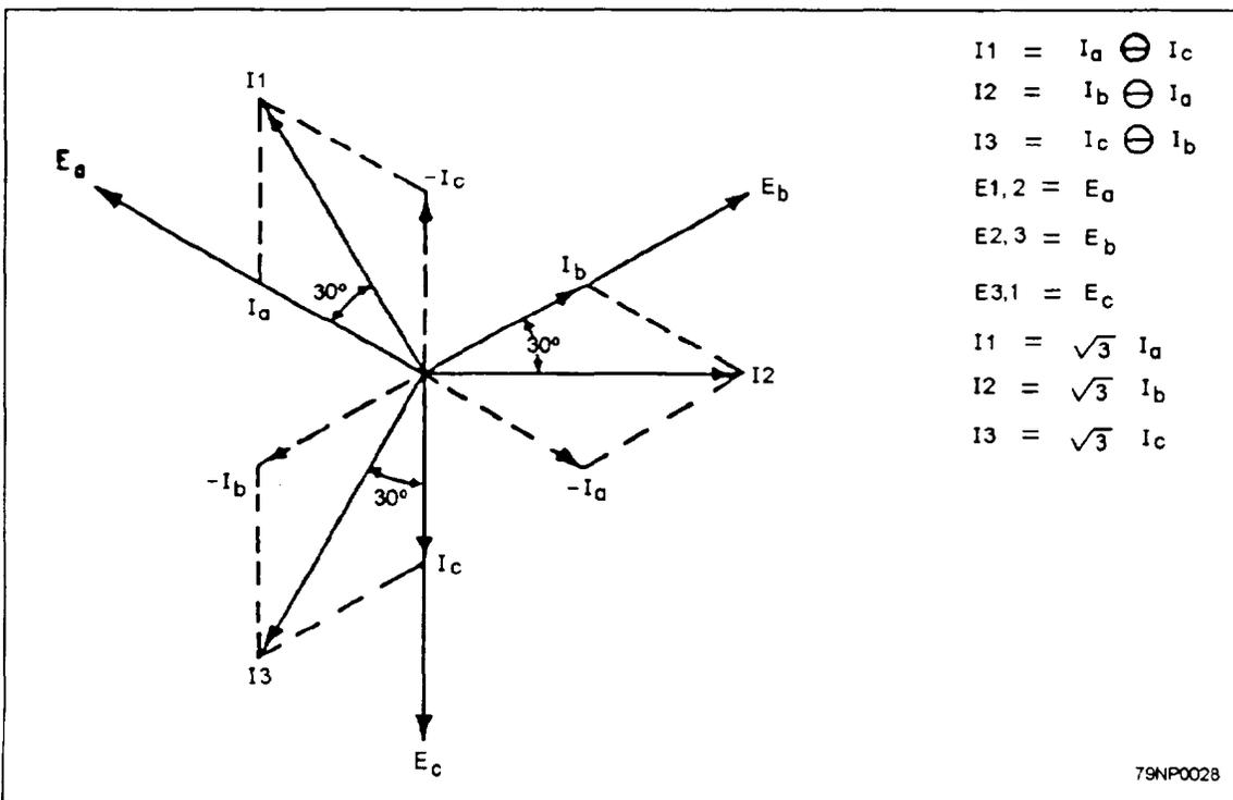
Figure 3-28.—Three-phase delta-connected system.
