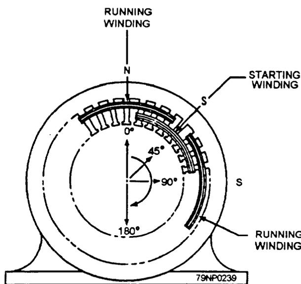
Figure 7-72.—A four-pole, split-phase motor.
