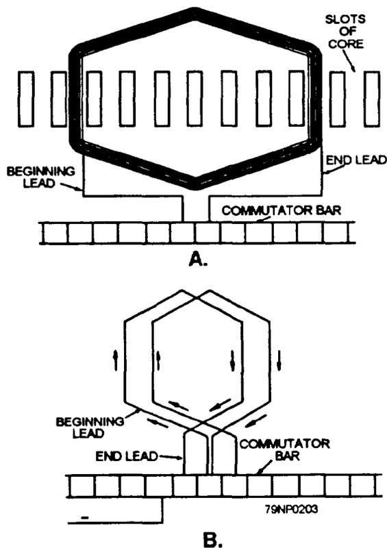
Figure 7-34.—Simplex lap windings.
