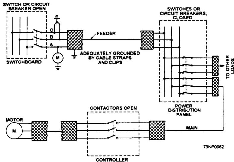
Figure 2-15.—Measuring insulation resistance of a power circuit.
