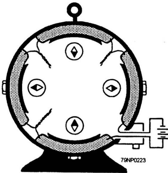
Figure 7-55.—Testing the polarity of field coils.
