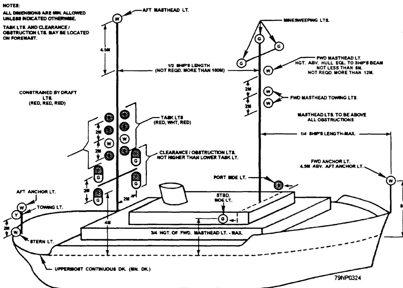
Figure 4-15.—General arrangement of lights for navigation.
