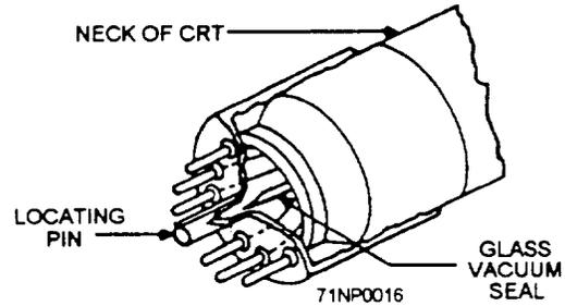
Figure 1-17.—Cathode-ray tube base structure.
