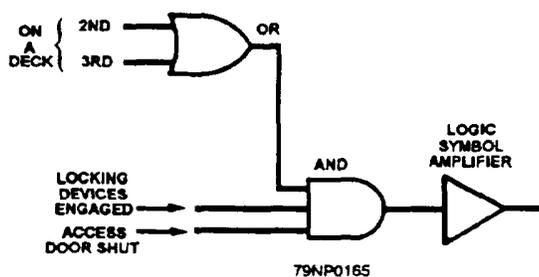
Figure 6-24.—Basic logic circuit.
