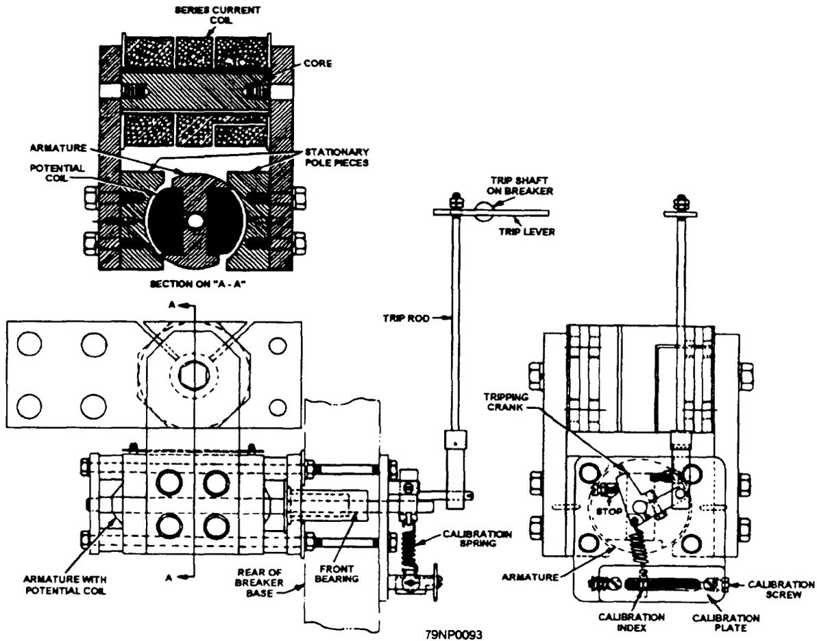
Figure 2-46.—Mechanical construction of an dc reverse-current relay.
