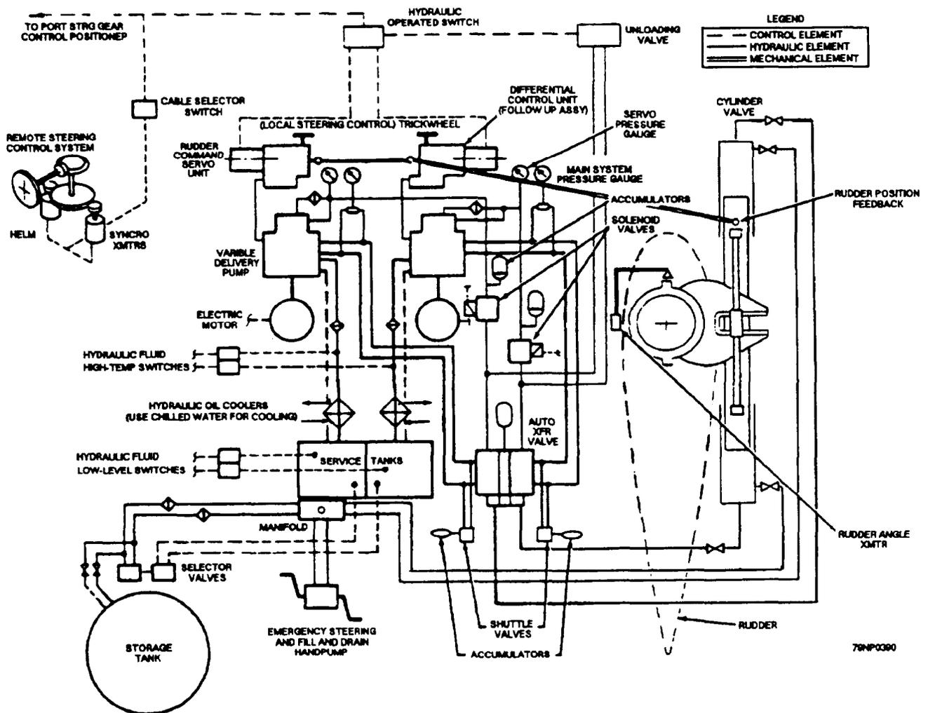
Figure 5-42.—Steering gear functional block diagram.
