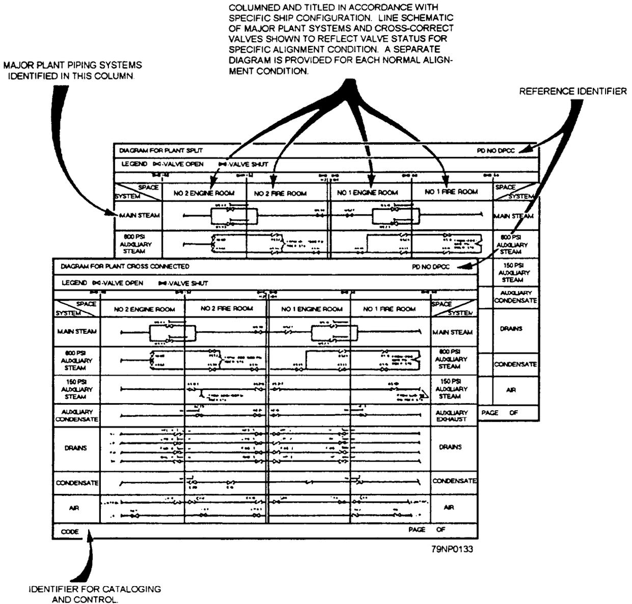
Figure 14-3.—Sample preferred alignment diagrams.
