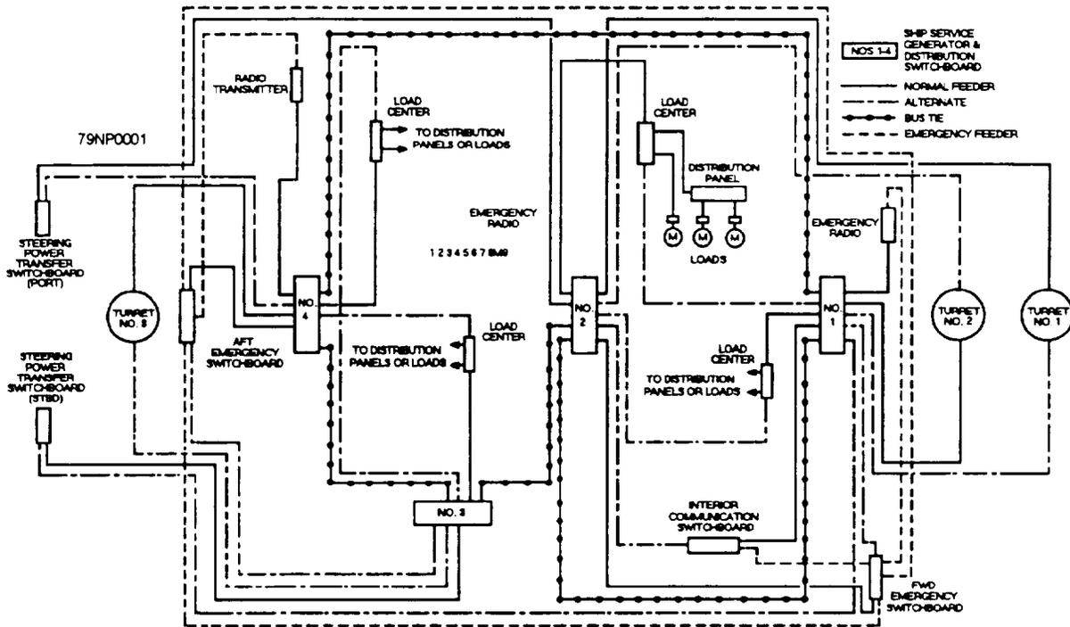
Figure 3-1.—Power distribution in a large combatant ship.
