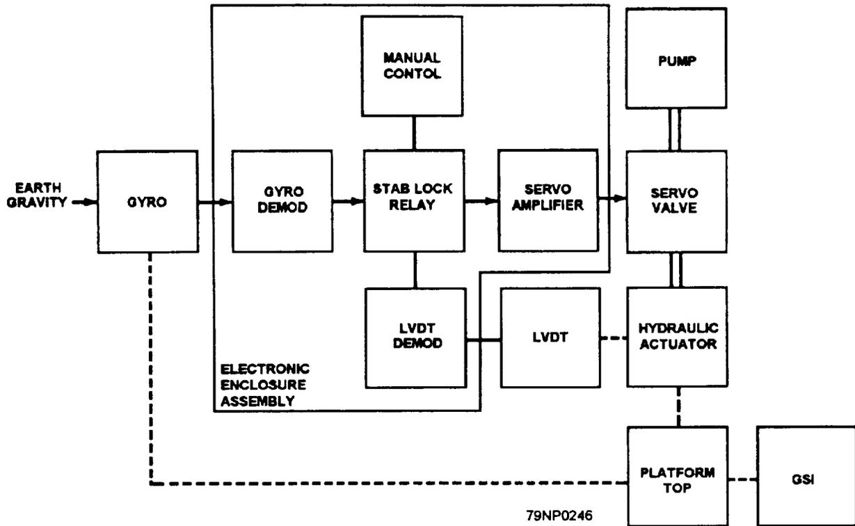
Figure 12-6.—Block diagram-stabilization circuits.
