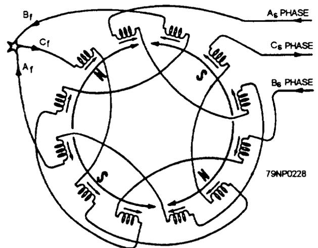
Figure 7-61.—Three-phase, four-pole, series-wye winding showing the four poles.
