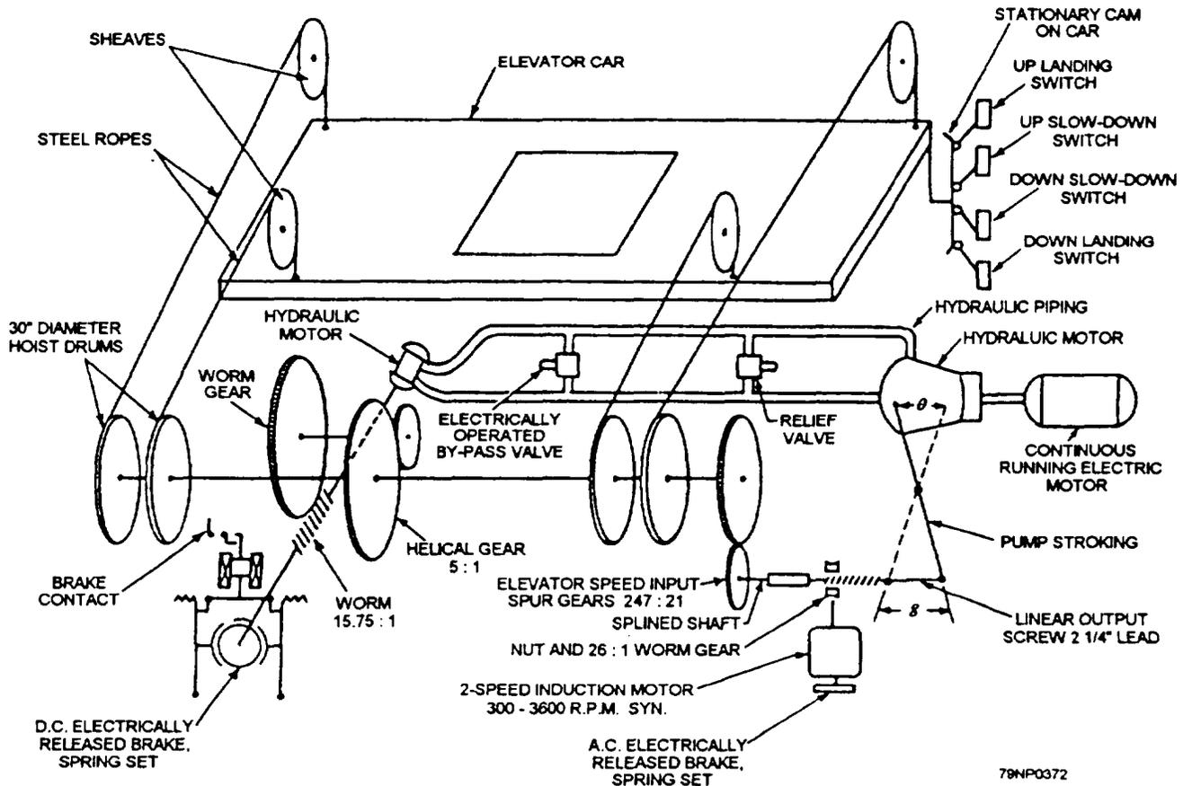
Figure 5-24.—Bomb elevator power plant and control scheme.
