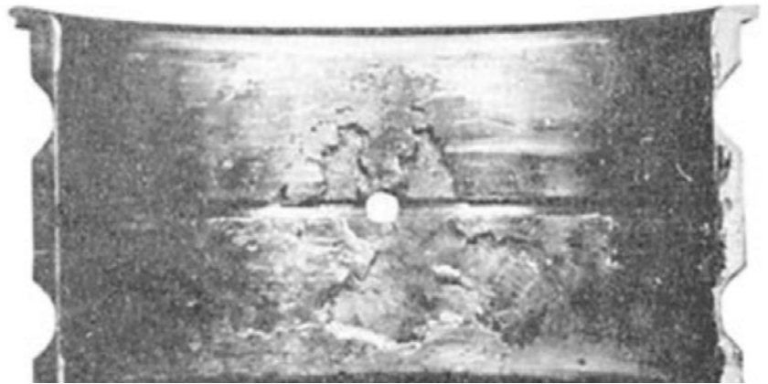
Figure 21-21 — Bearing failure resulting from wiping and excessive temperatures.
