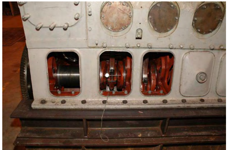
Figure 4-42 — Using a strain or deflection gauge between crank webs.
