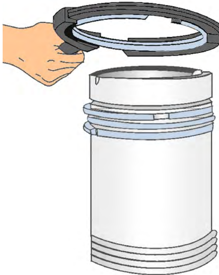
Figure 4-32 — Piston ring tools used for removal or installation.
