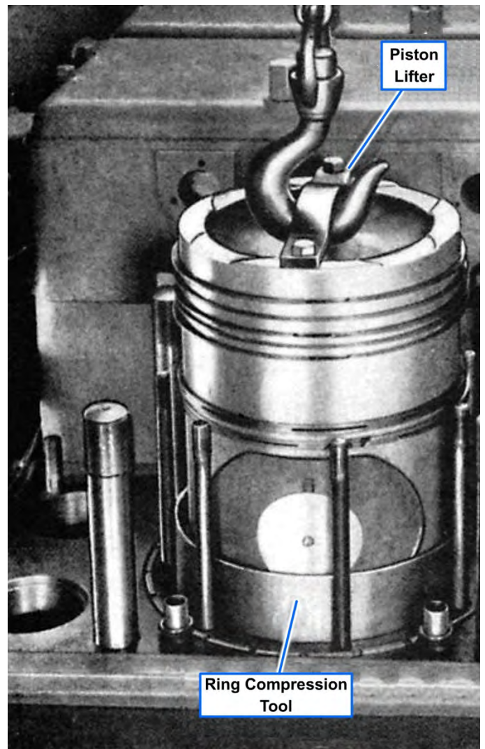
Figure 4-37 — Installing a piston in a cylinder bore with a funnel-type ring compressor.
