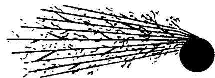
B SPARKS PRODUCED FROM HIGH-CARBON STEEL
