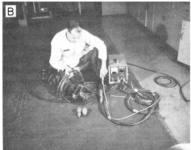
Figure 11-8.—Longitudinal magnetization—coil method.
