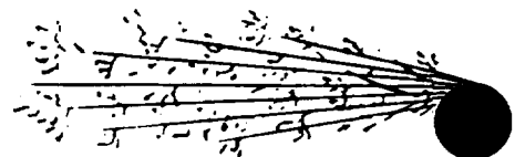
C SPARKS PRODUCED FROM GRAY CAST IRON
