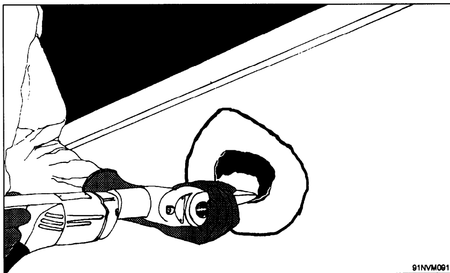
Figure 4-11.—Damaged area being cut away.
