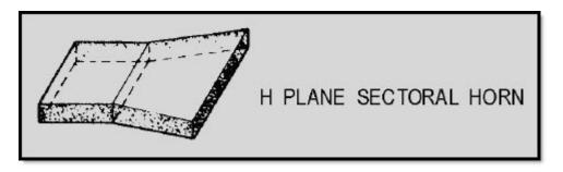
Figure 1-44B Waveguide horns. H PLANE SECTORAL HORN
