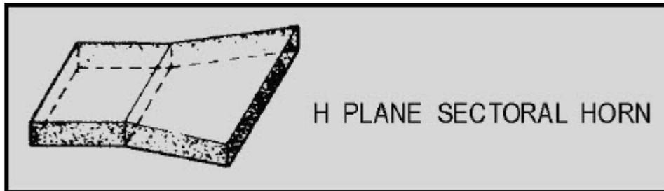
Figure 1-44B Waveguide horns. H PLANE SECTORAL HORN
