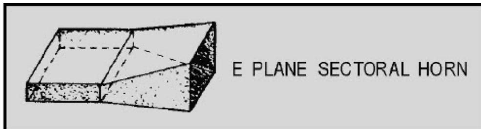
Figure 1-44A Waveguide horns. E PLANE SECTORAL HORN
