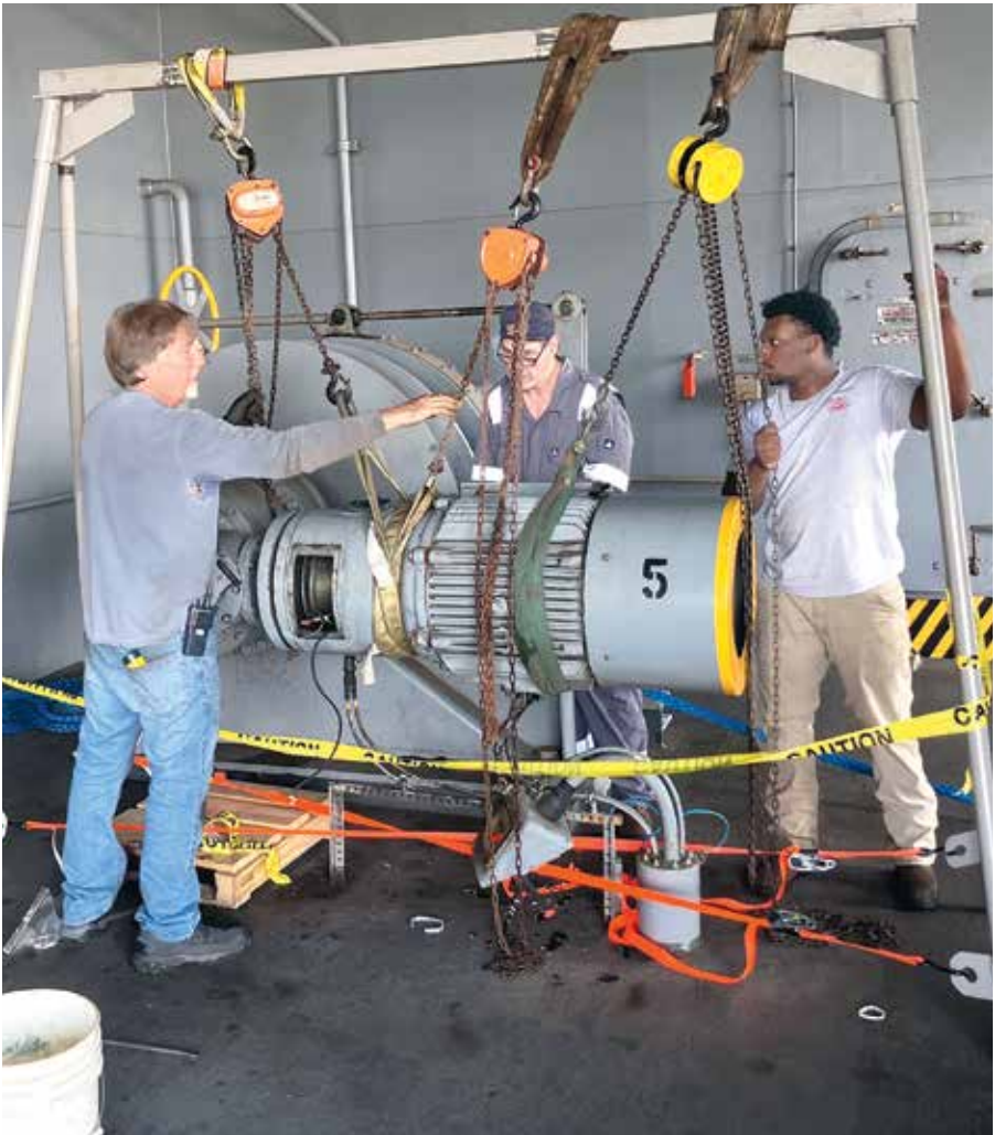
USNS Pomeroy QMED-Oiler D’Averyon Bloodworth, non-seniority, assisting engineers repairing the brake on #5 mooring winch in Baltimore, Maryland.
