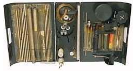
"Belly-buster", a hand-cranked audio drill strapped to an agent's stomach. It was used during the late 1950s and early 1960s to covertly drill holes into masonry for implanting audio devices, such as microphones.
