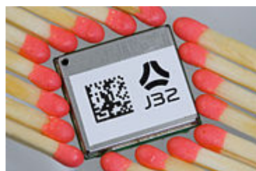
A typical OEM GPS receiver module measuring 15 mm × 17 mm (0.6 in × 0.7 in)
