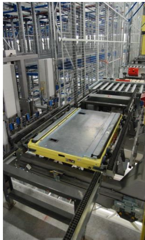
At the P&D stations, pallets are moved on and off the crane using chain conveyor
