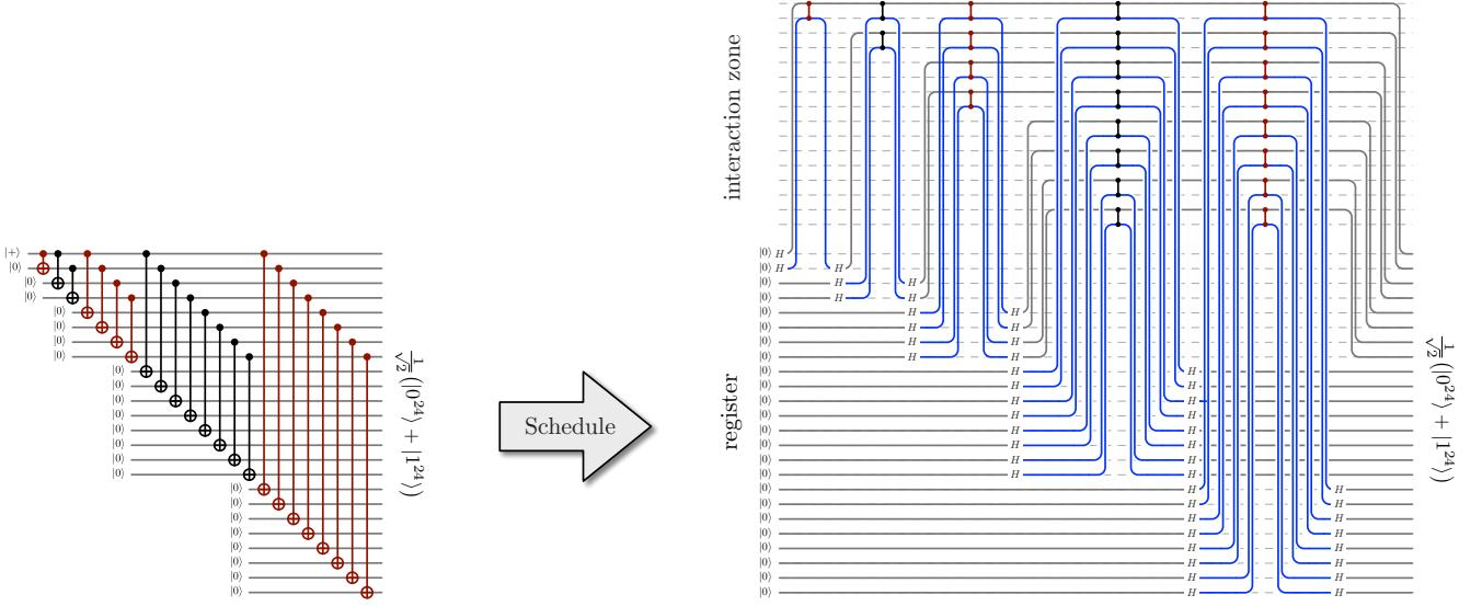
FIG. 6. Circuit to prepare a 24-qubit cat state, unencoded. One-qubit gates are applied at an atom's home register location.
