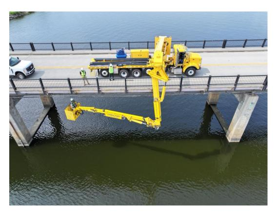
The **Paxton-Mitchell Snooper 260** is a high-reach under-bridge inspection and maintenance platform designed to meet the demanding needs of bridge engineers, DOT personnel, and infrastructure contractors. Known for its robust capabilities, the 260 model combines reliability, versatility, and safety for efficient bridge access.
