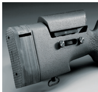
THUMBWHEEL ADJUSTABLE CHEEKPIECE, with locking thumbscrews. This is recommended for competition rifles with iron or receiver sights where frequent changes are necessary. Shown with spacer system and presentation recoil pad.
