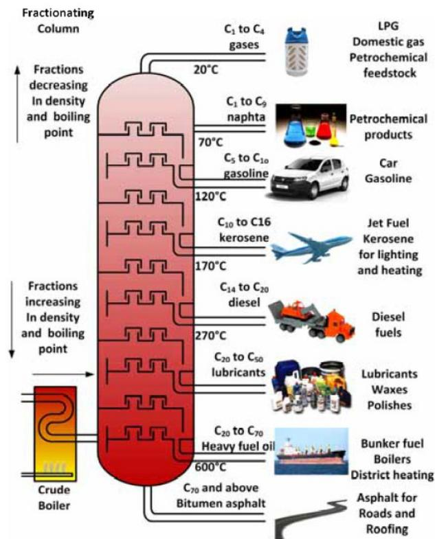
Crude oil exists basically in two types – high viscosity or heavy crude and low viscosity or light crude. In the US light crude is preferred since it yields more gasoline than heavy crude. In Europe heavy crude is preferred because it yield more diesel fuel. Because the input feed are different outputs from the initial distillation tower will differ.
