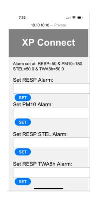
**DOWNLOADING DATALOG** – Immediate download of the datalog using smart device or PC. They can then immediately be e-mailed or shared. Logs are in CSV format and can be easily graphed using excel
