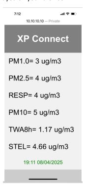
**MODE MENU** – specific for silica exposure measurement, the function uses the SDS of the material (e.g., engineered stone) to realistically estimate silica dust exposure.
