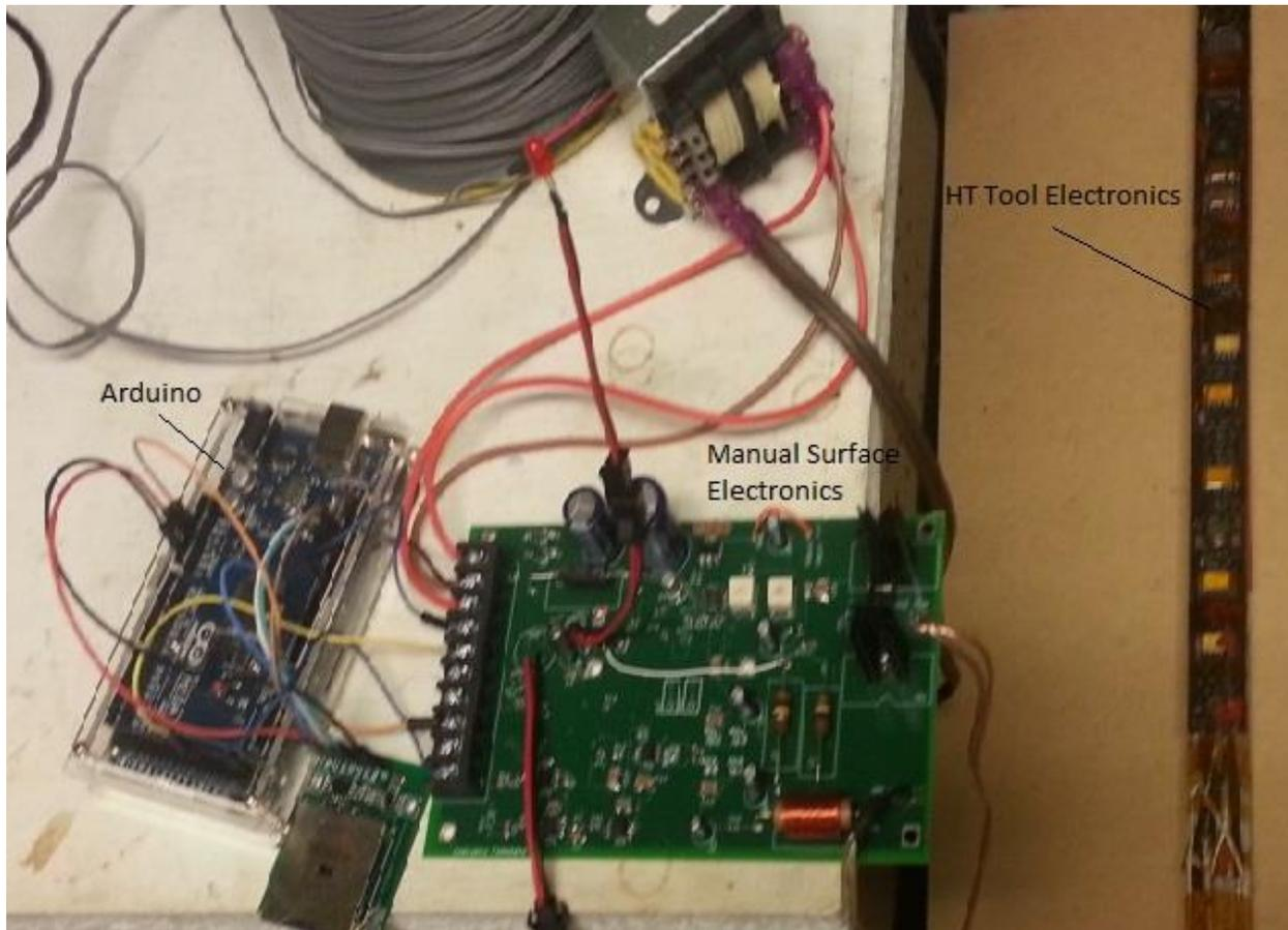
Figure 1 First use of an Arduino system to operate the surface electronics for monitoring a geothermal well monitoring tool.
