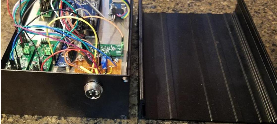
Figure 6. Shows is the circuit mounted and wired inside  $\frac{1}{2}$  of the extruded aluminum “clam” shell enclosure. One of the end plates was mounted to the lower clamshell with the circuit to mount a 5 pin connector.
