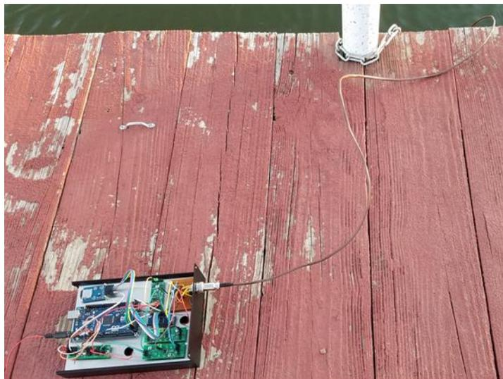
Figure 11. The custom built data collection system is working on the dock. The 50 meter sensor cable is in about 10ft of water.
