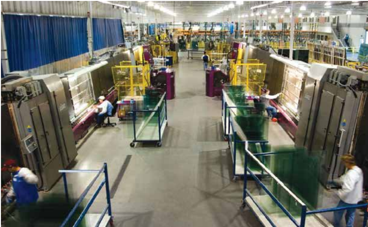
Two of our three multimillion dollar automated (robotic) glass insulating lines
