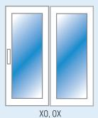
Monte Verde Patio Doors are available in Standard (2 1/2" wide rails) and French-style (4 1/2" rails), and in widths from 5' to 12' wide by 8' high. (Illustrations to left depict 4 1/2" rails.)
