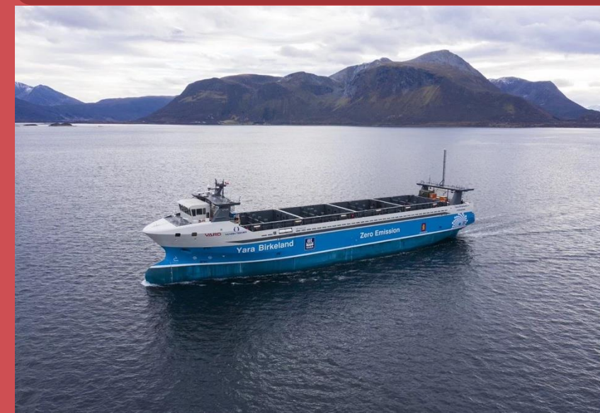
Yara Birkeland – First autonomous and all electric cargo ship under long-term trials in Norway
