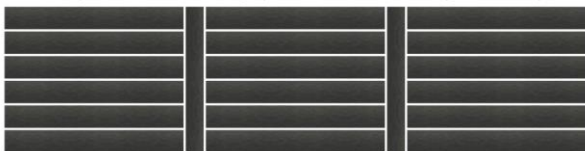
Example of breaker board design (recommended for decks longer than 5.4m):
