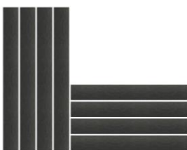
Another recommended option is to change the direction of the boards at the corner of the house:
