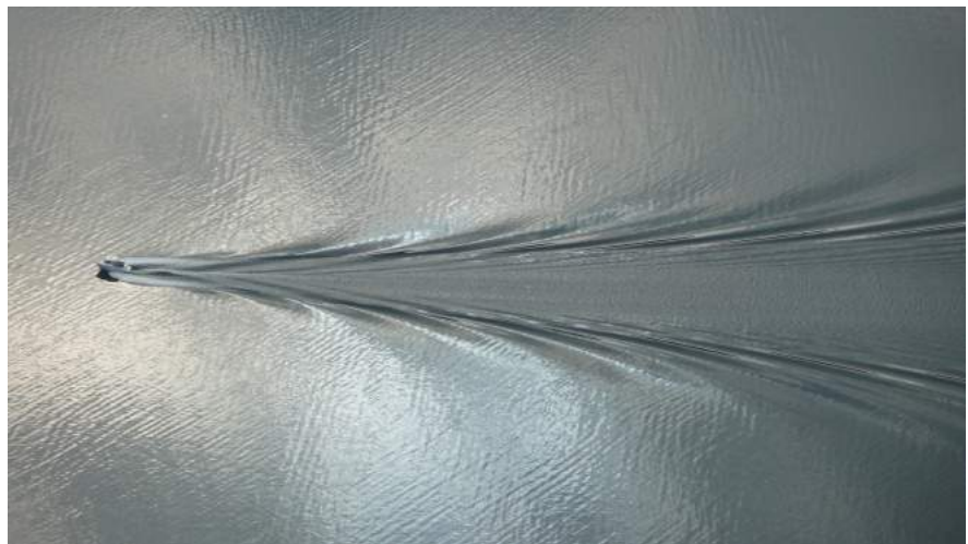
Figure 2. Typical wave pattern of a planning craft.
