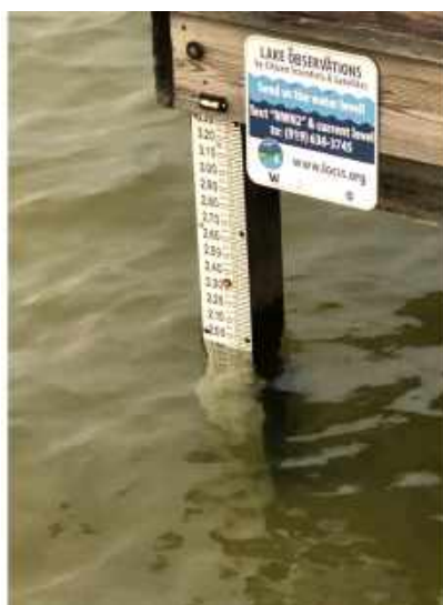
Figure LL 2. Lake level gauge installed by the Lake Observations by Citizen Scientists and Satellites program at the University of North Carolina-Chapel Hill, located at Goldston's Motel Pier (1608 White Lake Drive). Photo taken January 16, 2020.
