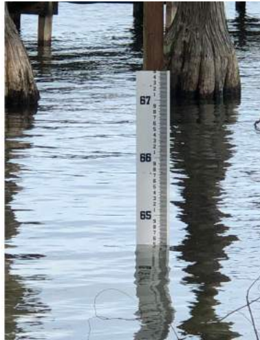
Figure LL 1. Lake elevation gauge installed by Walker Surveying Company at Turtle Cove. Elevations are given in the NAVD 88 Vertical Datum. Photo taken January 16, 2020.
