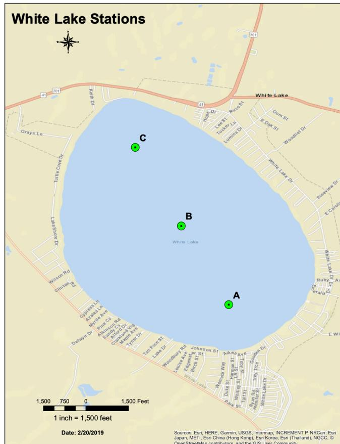
WL-C1, WL-B1, and WL-A1 are taken at 0.5 meters below the lake surface, while WL-C2, WL-B2, and WL-A2 are taken at 2.0 meters depth.
