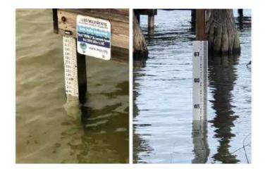
Figure 8. (Left) Lake level gauge installed by the Lake Observations by Citizen Scientists and Satellites program at the University of North Carolina-Chapel Hill, located at Goldston's Motel Pier (1608 White Lake Drive), and (right) lake elevation gauge installed by Walker Surveying Company at Turtle Cove. Elevations are given in the NAVD 88 Vertical Datum. Photos taken January 16, 2020.
