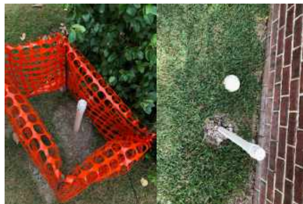
Figure N2. Top photo: groundwater well at Timberlodge Lane, located in a landscaped island that is popular with dogs—the fencing was added by Town staff when they rehabbed the well. Bottom photo: groundwater well at Godwin Road that was also rehabbed by Town staff. The top pipe is a wastewater line cleanout. Recent attempts to collect well water from these sites have been unsuccessful (Bill Stafford, Town of White Lake, personal communication).
