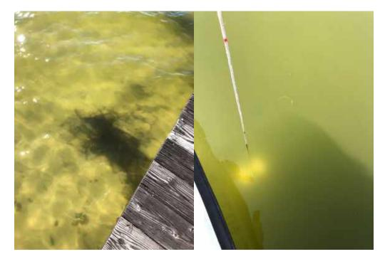
Photo on the left taken February 24, 2021 from the same pier as above. Photo on the right is a view of a Secchi Disk at a station in the middle of the lake on February 25, with clarity = 4 feet.
