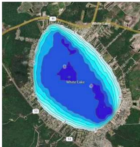
Figure 9. A bathymetric map of White Lake created from BioBase software, using depth measurements obtained with a Lowrance sonar receiver. The depth contours reflect conditions in 2019, when lake levels were approximately 1 foot lower than in 2017.
