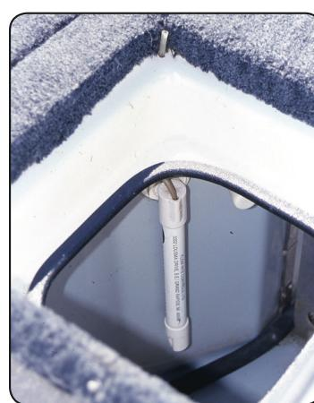
these systems can be easily improved by inserting a length of the appropriate-diameter aquarium air tubing into the vent hole on the top of the aspirator and routing the tubing to fresh air.
