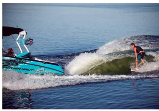
Figure 1. A typical, stern-heavy wake boat creates a large surfable wake. Photo from Pinsdaddy.
