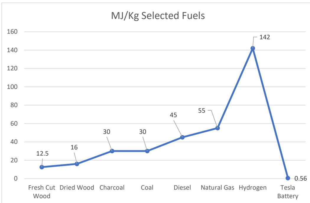
Adapted from [https://www.engineeringtoolbox.com/fuels-higher-calorific-values-d\\_169.html](https://www.engineeringtoolbox.com/fuels-higher-calorific-values-d_169.html)
