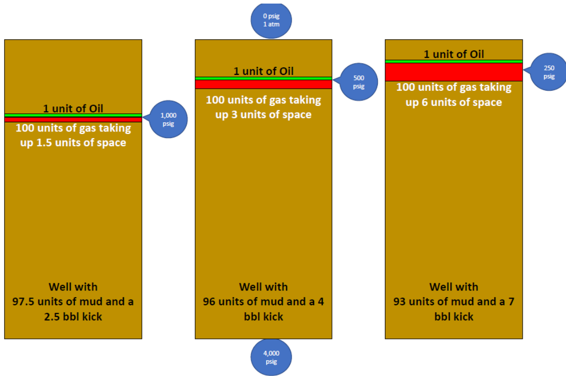
Figure 2: The remaining gas in solution leaves the oil and continues expanding at a much more noticeable rates as it comes close to surface.
