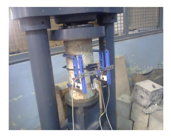
The above Photo shows dual Axial extensometer of Fixed Gauge Length of 100 MM with 5 MM compression stroke and can be fitted on square or Round samples. Whether the extensometers are to be fitted on the Thickness or width has to be specified by the user as it is factory set.( i.e. 50 MM thickness or 100 /150 mm width )
