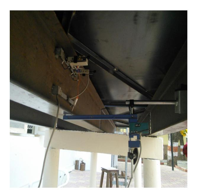
REUSABLE STRAIN TRANSDUCER FITTED TO A STEEL I-BEAM AND DEFLECTOMETER ATTACHED FOR DEFLECTION MEASUREMENT.
