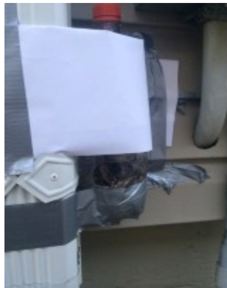
Soda bottle, (can tape a piece of paper to the outside for shade AFTER the bottle is affixed to the surface).
