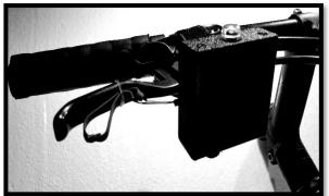
Pictures above show how the Mini-Hamster™ is installed on bicycles, e-bikes or other vehicles. As you can see, the elastic band is attached to the brake lever so whenever you press the brake the wire attached to the elastic band senses the movement and activates the brake light. This system is designed to avoid interference with the braking system of your bicycle, scooter or vehicle.
