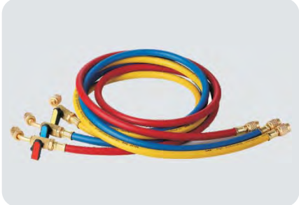
Hose with 1/4" (7/16 - 20) Female flare on manifold connection and 5/16" (1/2 - 20) Female flare angled on service end Standard fitting without ball valve
