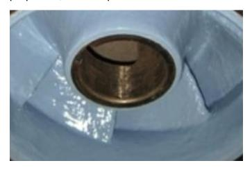
No more time consuming, painstaking, taking entire heavy impellers apart, moving them awkwardly around to repair the impeller wear surfaces. Just repair your impellers in place where access is practical. Repair patch and smooth the surfaces to efficient wear surfaces With Pro-Seal Aero-Graft®.
