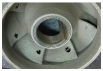
When this happens, above, repair in place with Pro-Seal Aero-Graft, used extensively by PSE for repair of their hydroelectric water impeller properties, below repaired.
