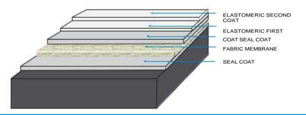
LMS nano polycarbon/polycarbonate Cool Roofs was specifically designed to extend the life of built-up, metal, concrete and single-ply roofs by providing a high tensile strength and ultra-bright white reflective topcoat system. The high reflectivity LMS Cool Roofs' rich consistency forms a permanently flexible monolithic membrane it can also be a stand-alone over insulation. It provides protection from normal weathering, aging and ultraviolet exposure.
