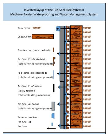
This is a (not to scale) schematic of the Pro-Seal FlexSystem II Methane Barrier System as laid up in the inverted format to accommodate the installation of concrete pour, Shotcrete or Gunite (the latter two only with manufactures
