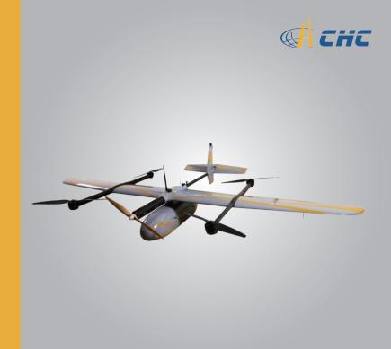
P310 is a innovative VTOL composite wing UAV, using fixed wing with four rotors of composite wing layout form can achieve both long fixed wing UAV navigation time, high speed and far distance features and the function of the rotorcraft UAV.
